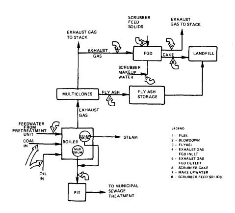
Figure 2. Diagram of boiler and flue gas desulfurization system showing sampling locations.
