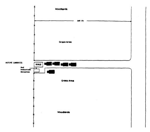
State survey personnel discover that the source is not in the truck that was originally thought to be the problem. It is a truck that is third in line, about 100 feet away from the scales. Gamma levels at this distance are 11 mR/hr. This is why the alarm failed to clear when the first truck was diverted. Gamma survey results will be provided to the State personnel as follows.
