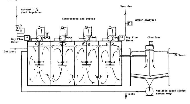
FIG. 2 MIDDLESEX COUNTY SEWAGE TREATMENT PLANT "UNOX" PILOT FACILITY SCHEMATIC
