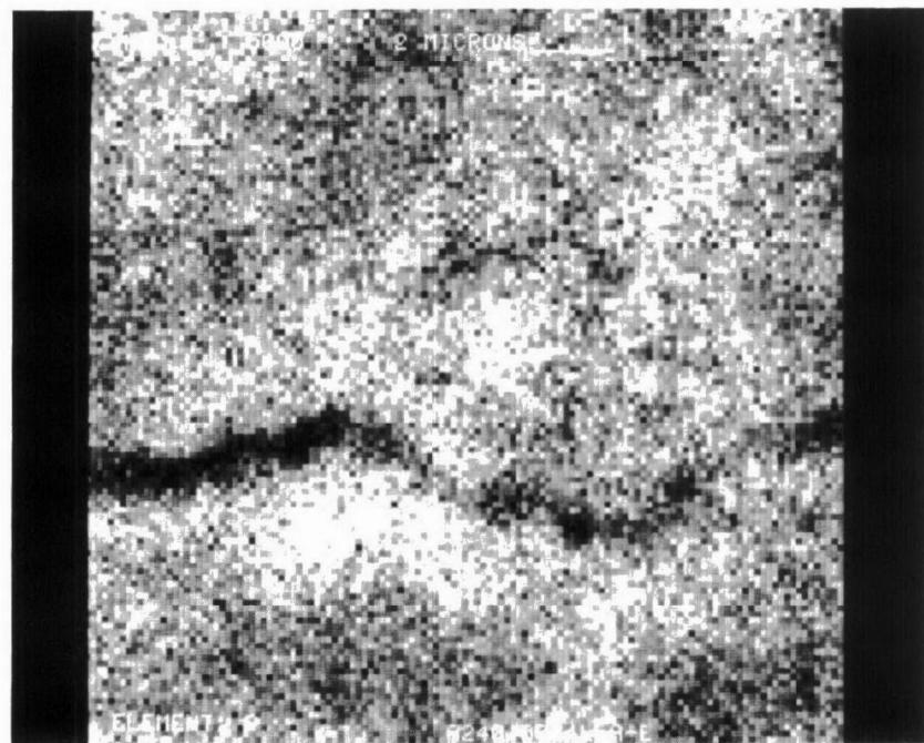
Figure D-170. Phosphorus Dot Map at X5000 of Converter A240/0334L
