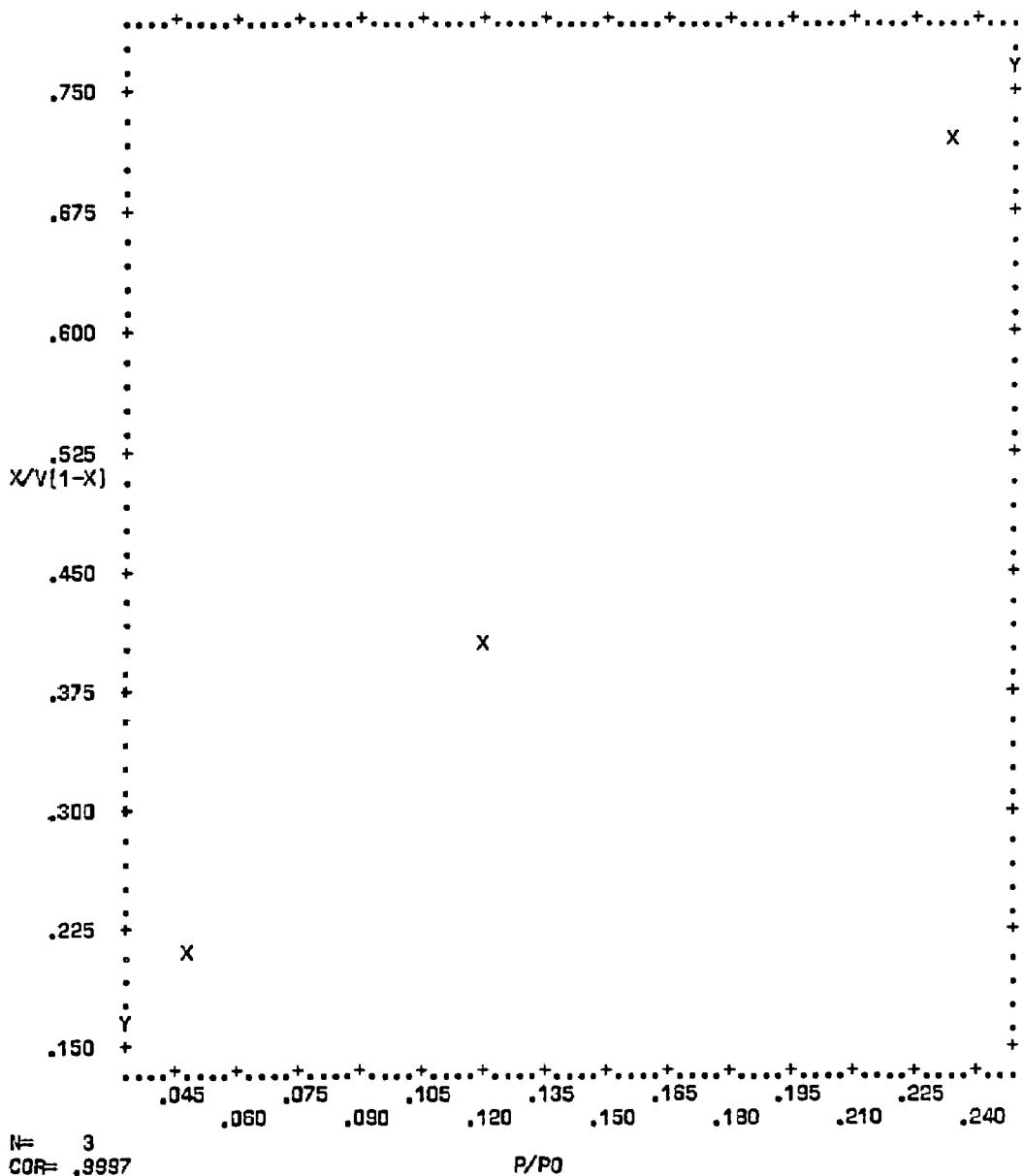
**Figure C-87.** Plot of BET equation versus relative pressure for Converter A249/0169-3-B - Bulk
