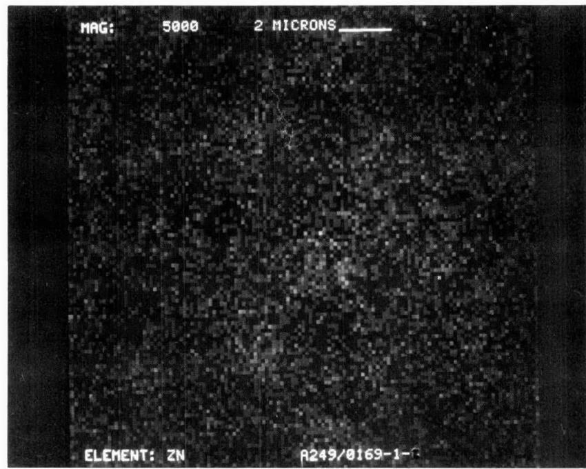
Figure D-179. Zinc Dot Map at X5000 of Converter A249/0169-1
