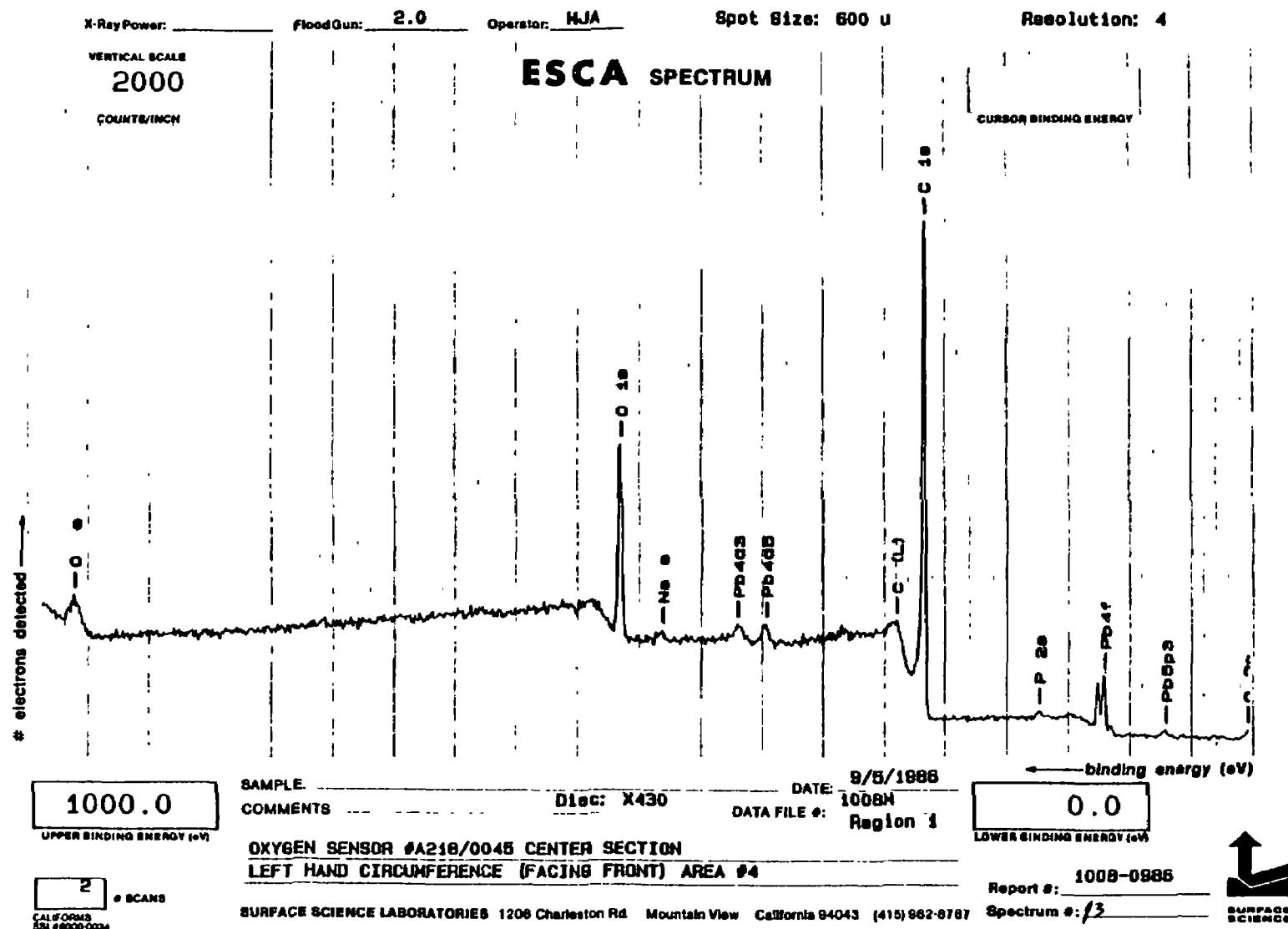
Figure I-18. ESCA Spectrum of Oxygen Sensor A218/0045 from 0 eV to 1000 eV (Location 9)
