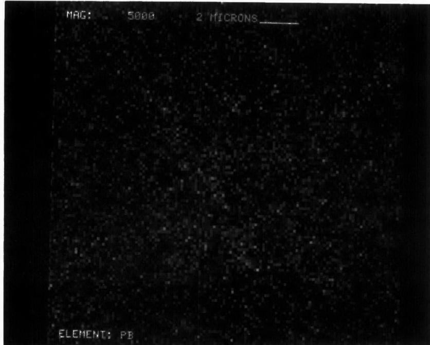
Figure D-37. Lead Dot Map at X5000 of Converter A218/0045X
