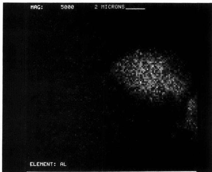
Figure D-145. Aluminum Dot Map at X5000 of Converter A240/0141L
