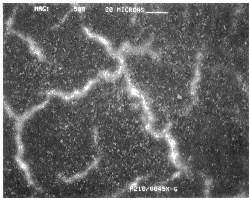
Figure D-242. Scanning Electron Micrograph at X500 of Converter A218/0045X-Rear Face
