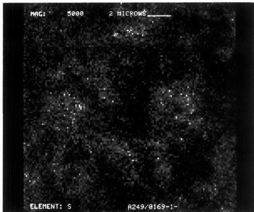
Figure D-178. Sulfur Dot Map at X5000 of Converter A249/0169-1
