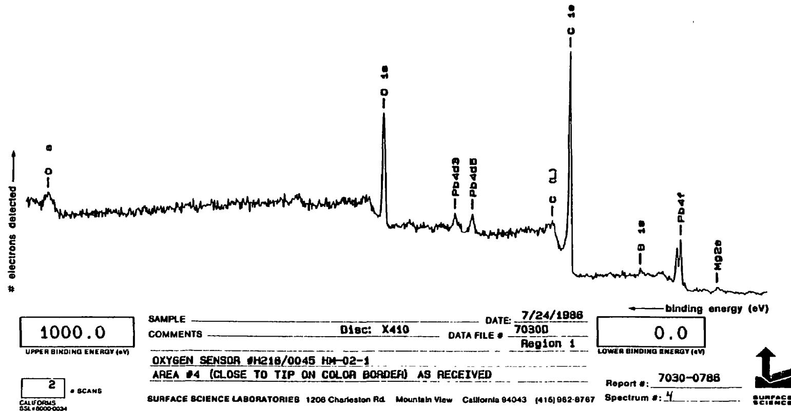
Figure I-8. ESCA Spectrum of Oxygen Sensor A218/0045 from 0 eV to 1000 eV (Location 4)
