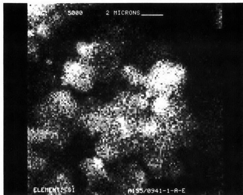
Figure D-216. Silicon Dot Map at X5000 of Converter A155/0941-1
