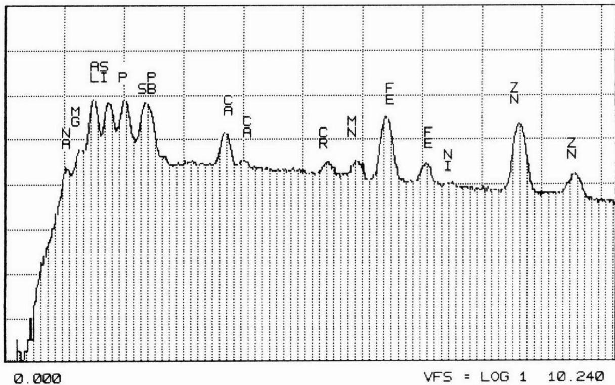
Figure D-221. SEM/EDX Spectrum of Converter A155/0941-2
