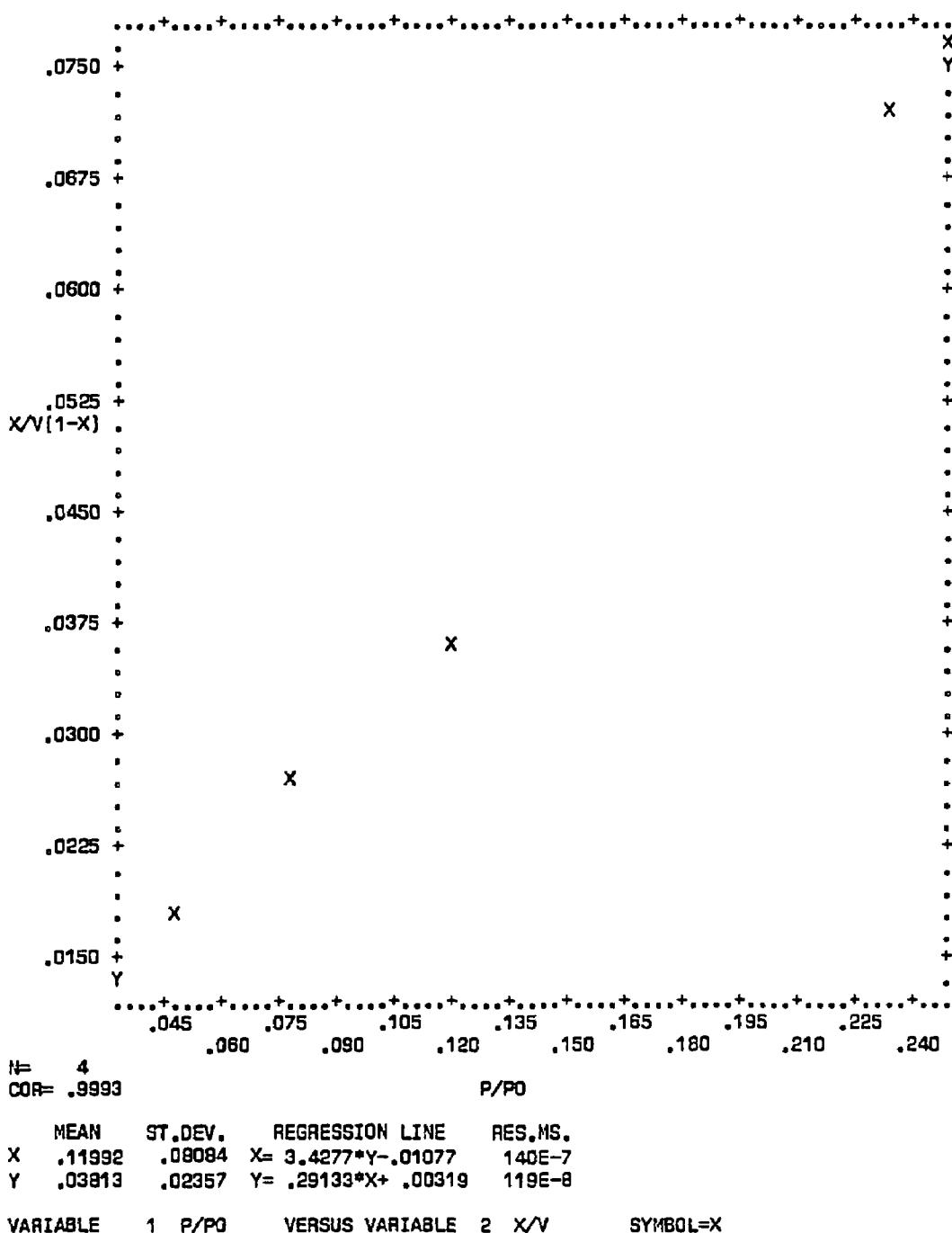
**Figure C-44. Plot of BET equation versus relative pressure for Converter A230/0177X-A - Front Face**
