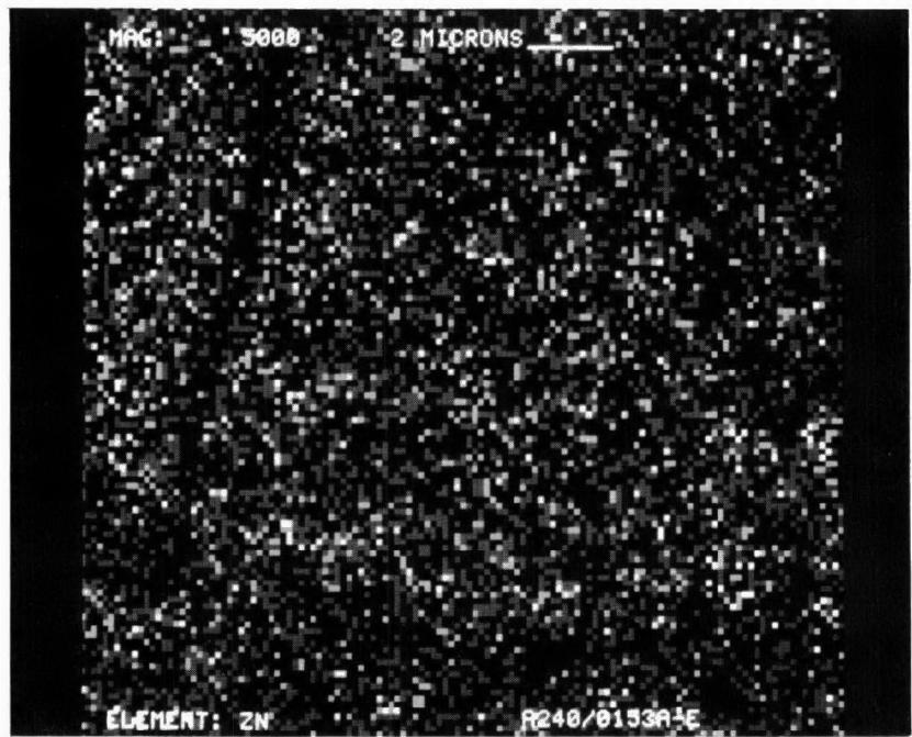
Figure D-159. Zinc Dot Map at X5000 of Converter A240/0153
