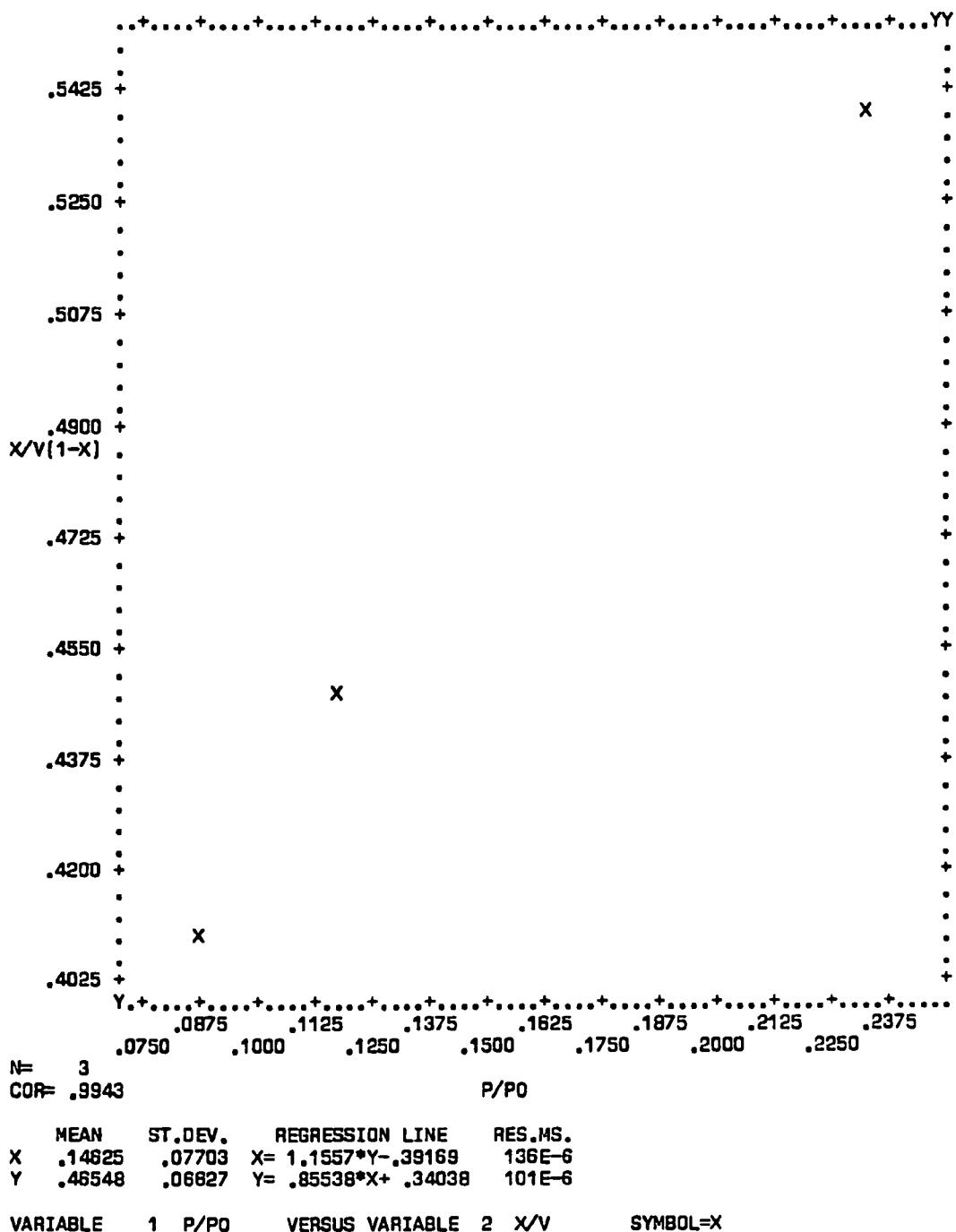
**Figure F-11.** Plot of BET equation versus relative pressure for Oxygen Sensor A218/0045X
