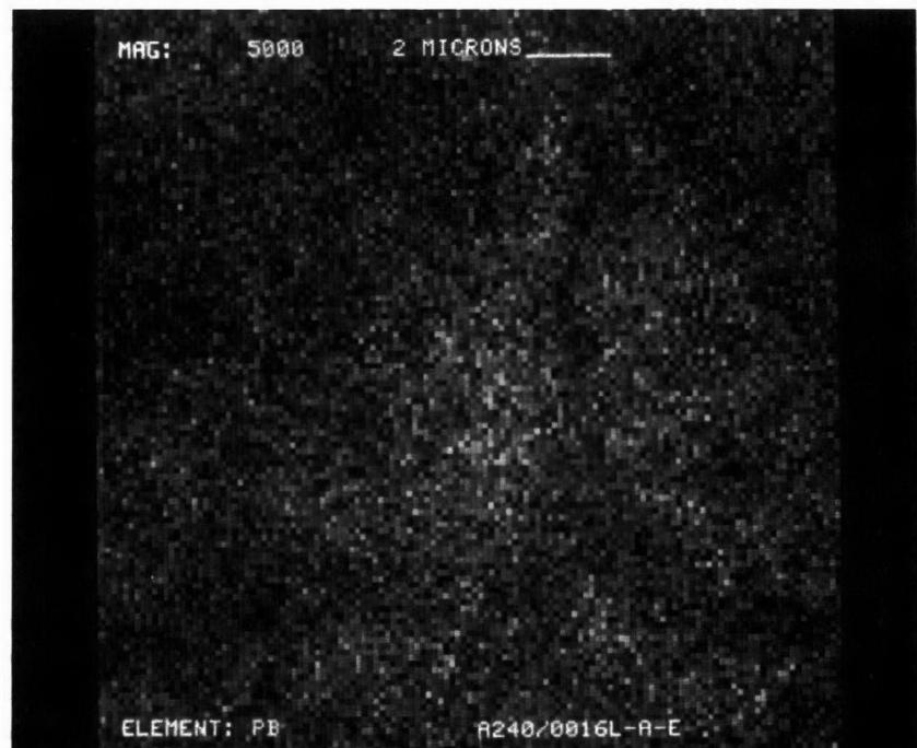
Figure D-127. Lead Dot Map at X5000 of Converter A240/0016L
