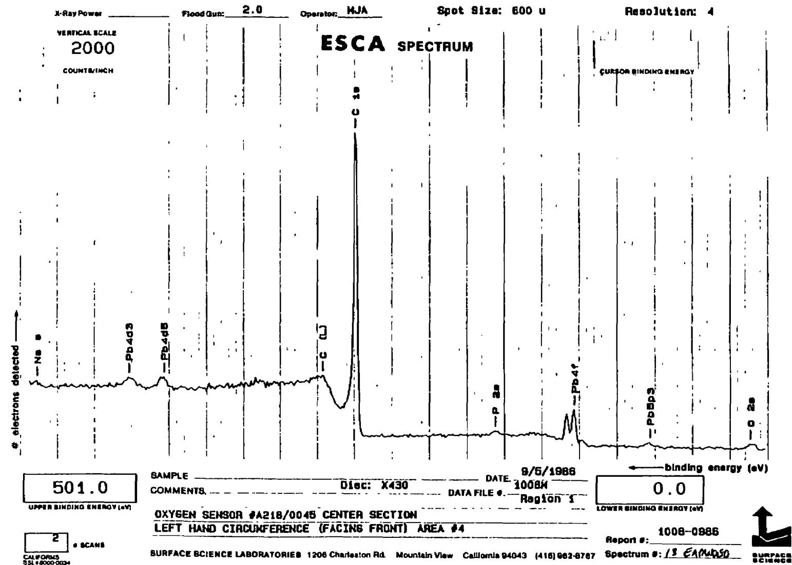
Figure I-19. ESCA Spectrum of Oxygen Sensor A218/0045 from 0 eV to 510 eV (Location 9)
