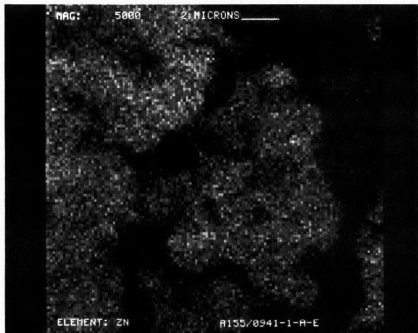
Figure D-219. Zinc Dot Map at X5000 of Converter A155/0941-1
