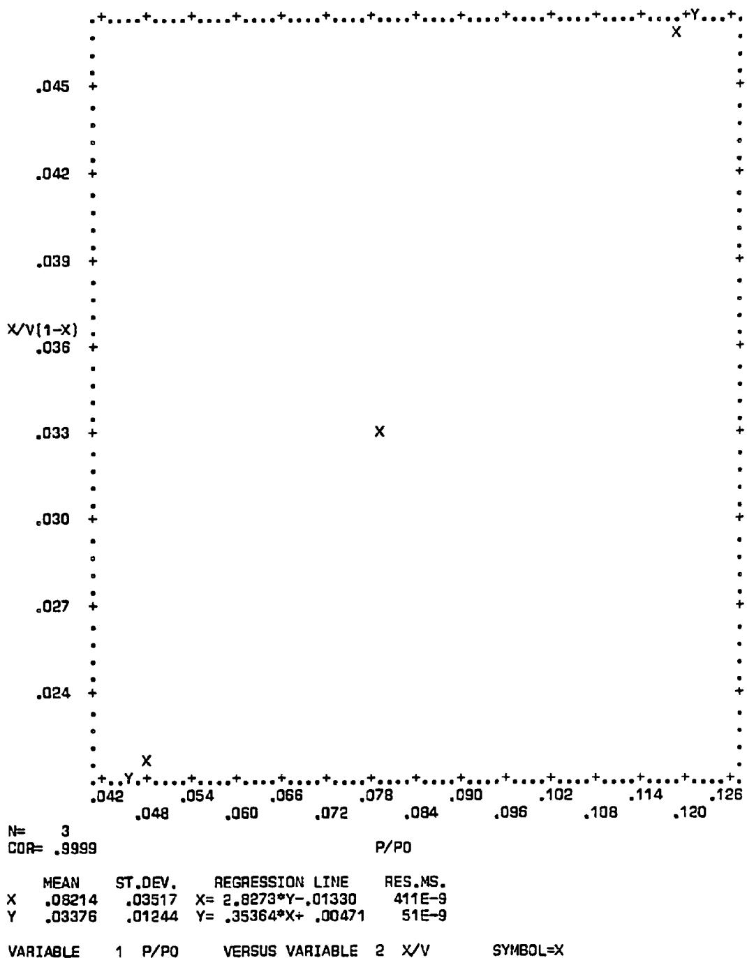
Figure C-22. Plot of BET equation versus relative pressure for Converter A220/0392-B - Front Face
