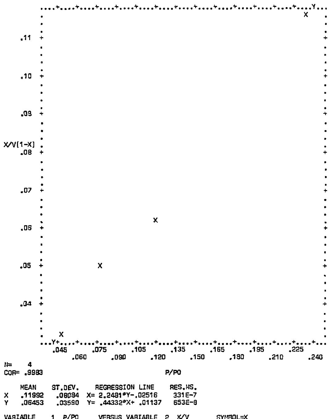
Figure C-42. Plot of BET equation versus relative pressure for Converter A221/0447-B - Front Face
