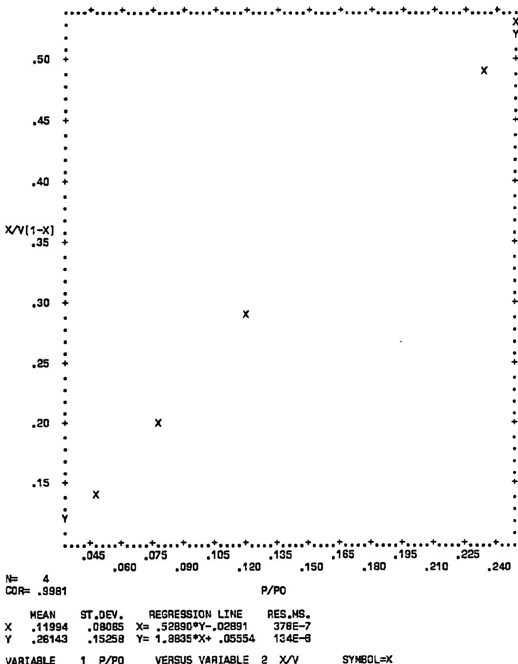
Figure C-81. Plot of BET equation versus relative pressure for Converter A249/0169-2 - Bulk
