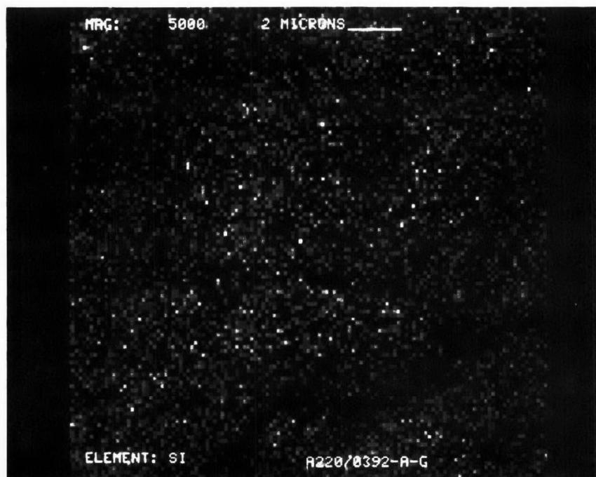
Figure D-256. Silicon Dot Map at X5000 of Converter A220/0392-Rear Face
