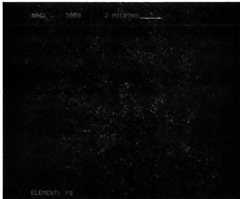
Figure D-87. Lead Dot Map at X5000 of Converter A221/0204
