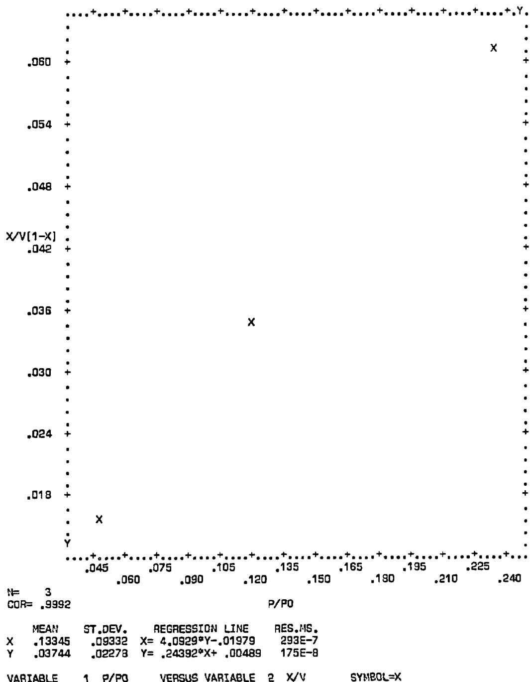
**Figure C-57. Plot of BET equation versus relative pressure for Converter A240/0016L-B - Front Face**
