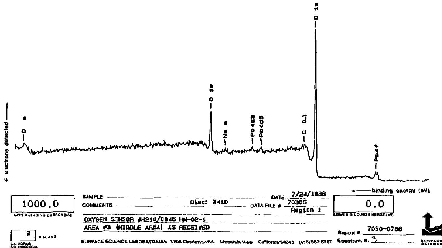
Figure G-20. ESCA Spectrum of Oxygen Sensor A218/0045 from 0 eV to 1000 eV (Exterior Surface)
