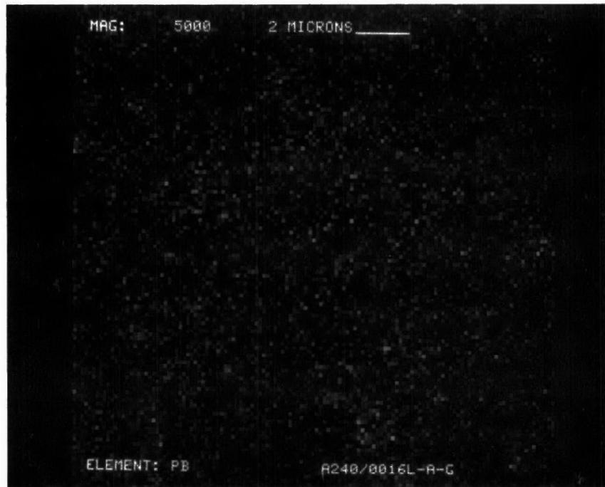
Figure D-287. Lead Dot Map at X5000 of Converter A240/0016L-Rear Face
