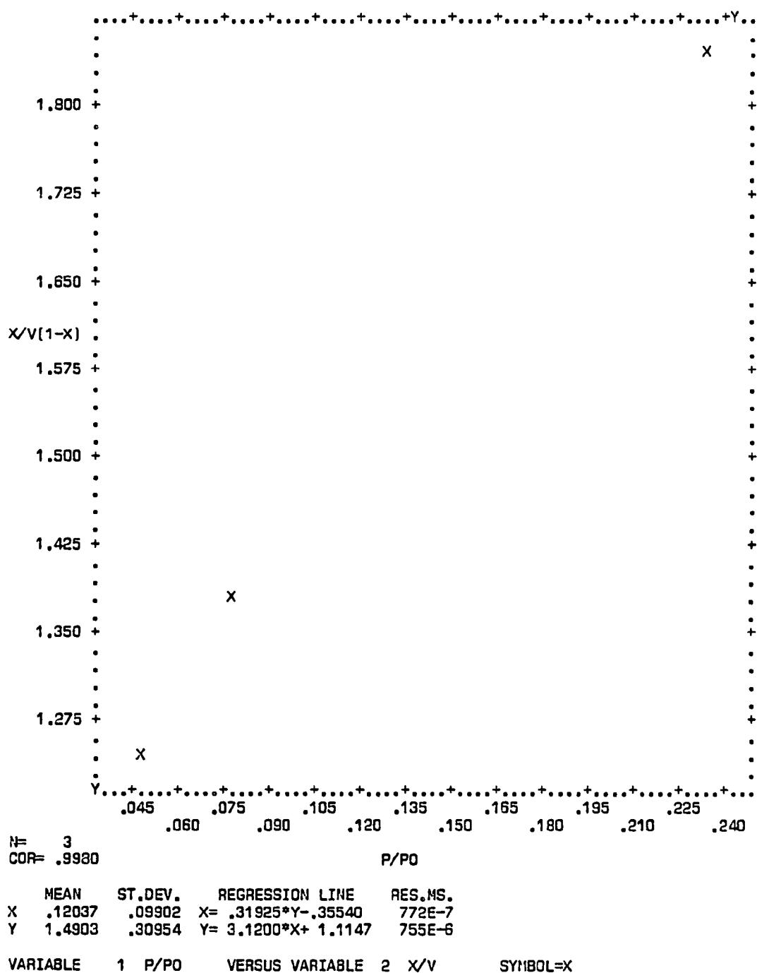
**Figure F-8.** Plot of BET equation versus relative pressure for Oxygen Sensor A251/0467
