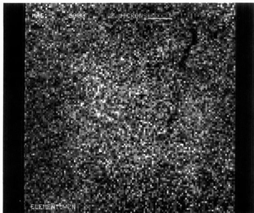
Figure D-89. Zinc Dot Map at X5000 of Converter A221/0204
