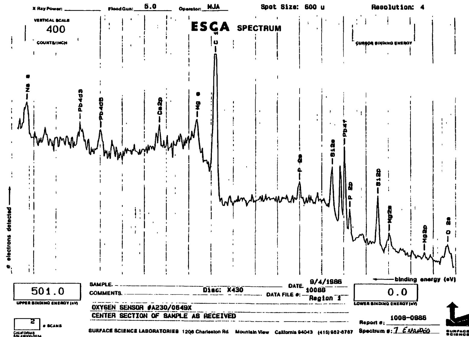
Figure G-12. ESCA Spectrum of Oxygen Sensor A230/0649X from 0 eV to 501 eV (Exterior Surface)
