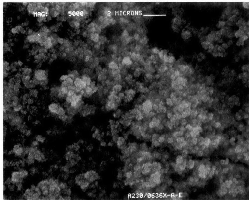
Figure D-114. Scanning Electron Micrograph at X5000 of Converter A230/0636X
