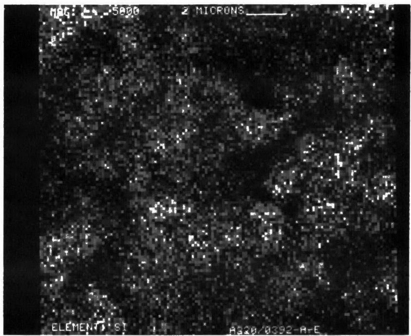
Figure D-56. Silicon Dot Map at X5000 of Converter A220/0392
