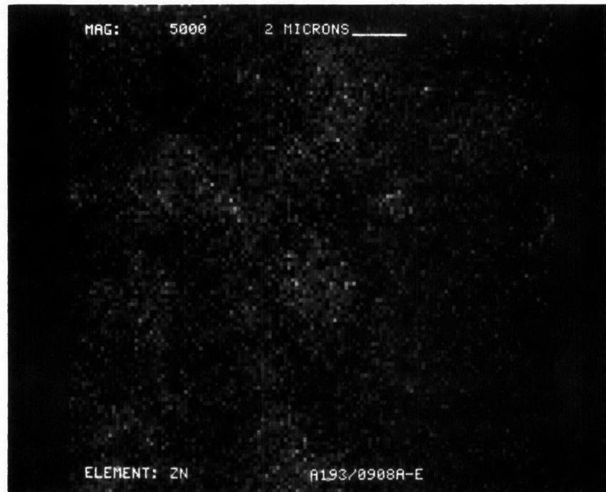
Figure D-19. Zinc Dot Map at X5000 of Converter A193/0908
