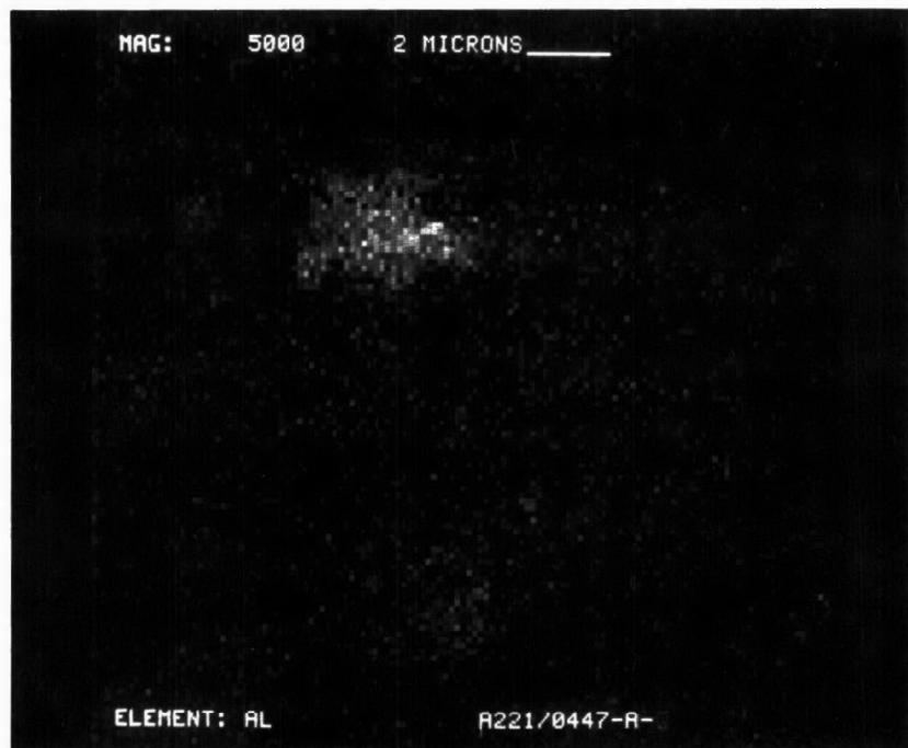
Figure D-95. Aluminum Dot Map at X5000 of Converter A221/0447
