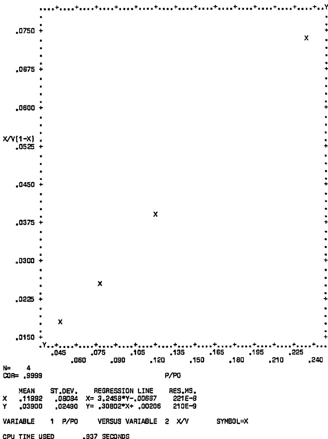
**Figure C-10.** Plot of BET equation versus relative pressure for Converter A218/0045 - Front Face
