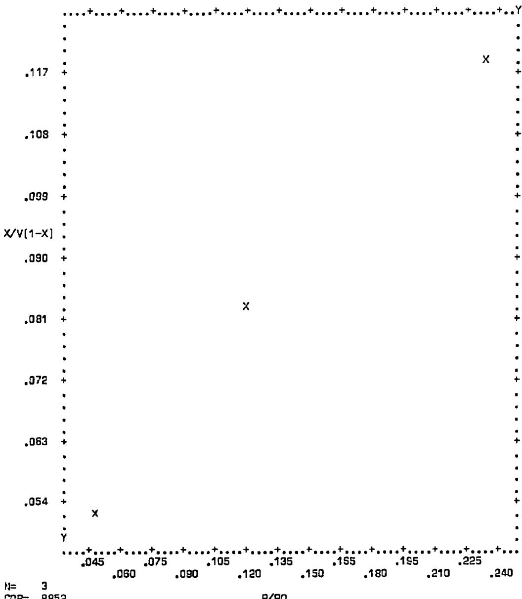
**Figure C-5. Plot of BET equation versus relative pressure for Converter A193/0908-A - Front Face**
