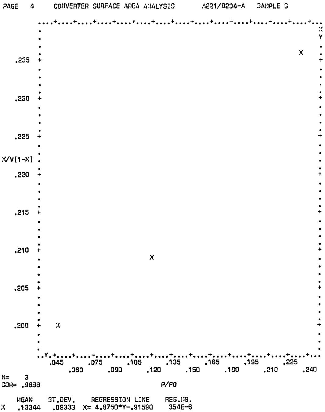
Figure C-35. Plot of BET equation versus relative pressure for Converter A221/0204-A - Rear Face
