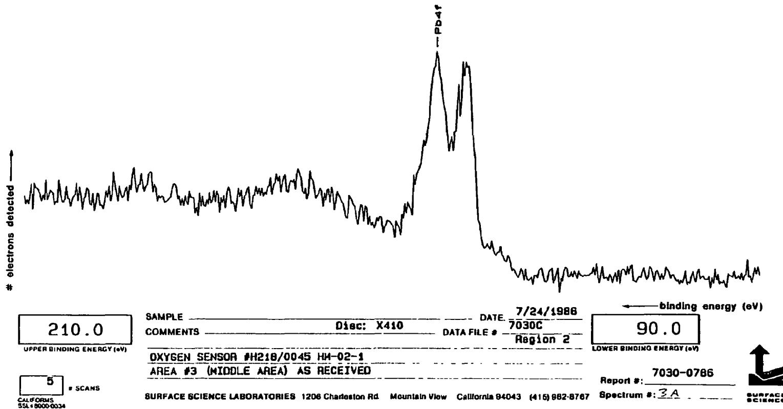
Figure I-7. ESCA Spectrum of Oxygen Sensor A218/0045 from 90 eV to 210 eV (Location 3)
