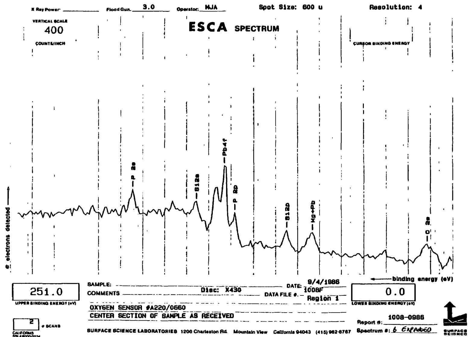
Figure G-2. ESCA Spectrum of Oxygen Sensor A220/0660 from 0 eV to eV 251 (Exterior Surface)
