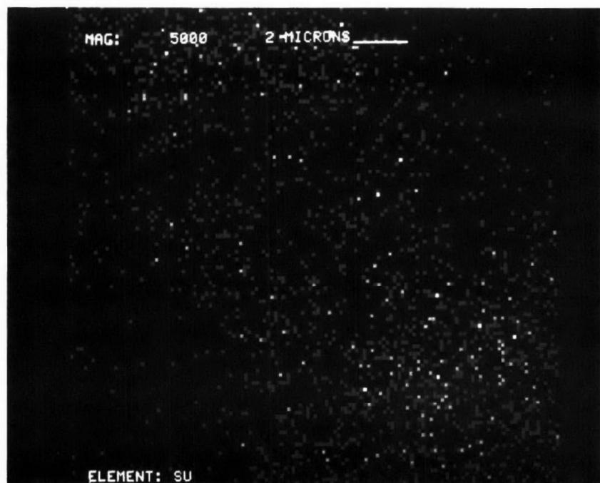
Figure D-188. Sulfur Dot Map at X5000 of Converter A249/0169-2
