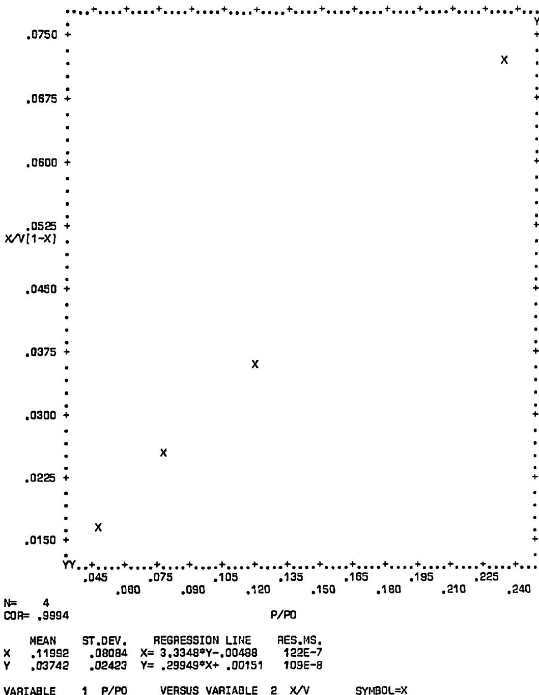
**Figure C-21.** Plot of BET equation versus relative pressure for Converter A220/0392-B - Bulk
