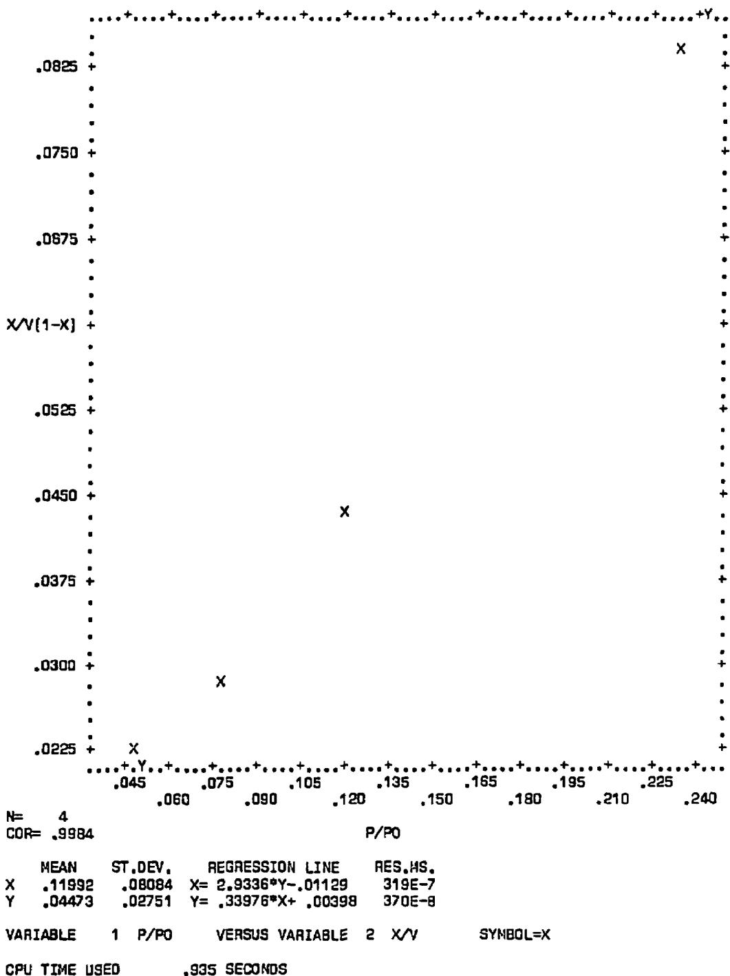
Figure C-13. Plot of BET equation versus relative pressure for Converter A218/0045X - Front Face
