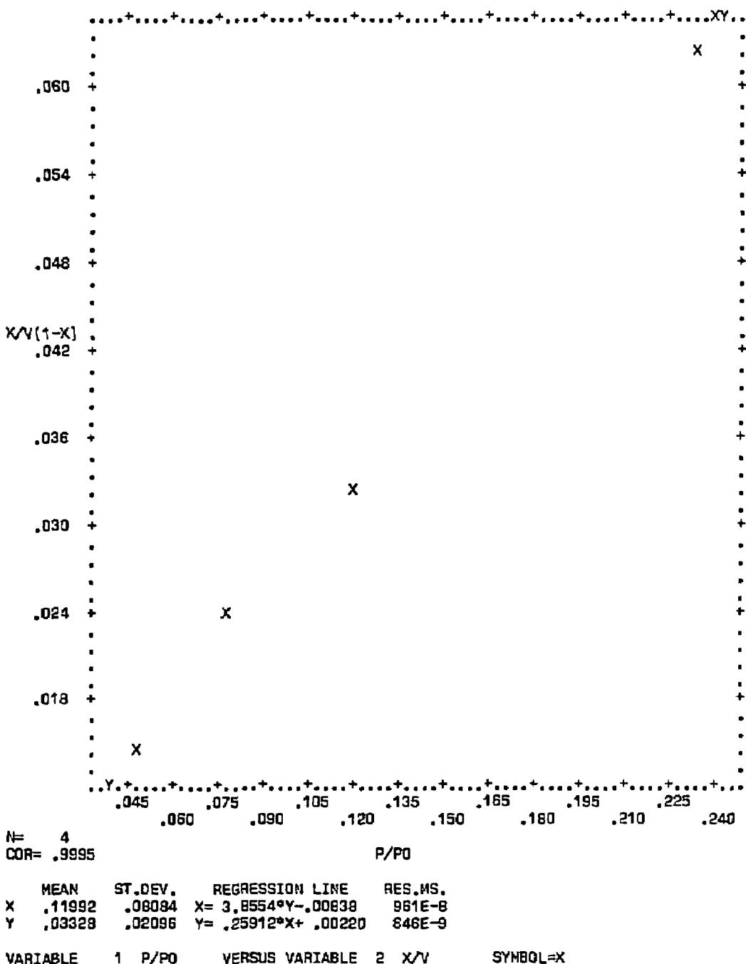
**Figure C-9. Plot of BET equation versus relative pressure for Converter A218/0045 - Bulk**
