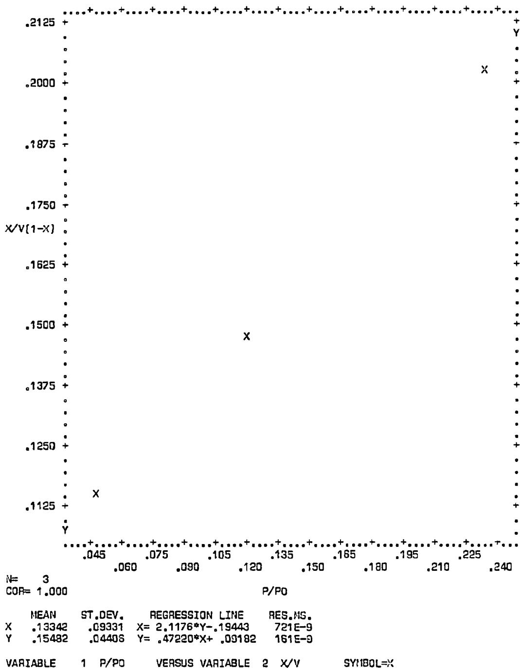
Figure C-6. Plot of BET equation versus relative pressure for Converter A193/0908-A - Rear Face
