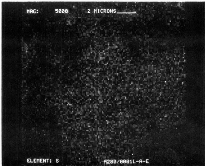
Figure D-208. Sulfur Dot Map at X5000 of Converter A280/0001L
