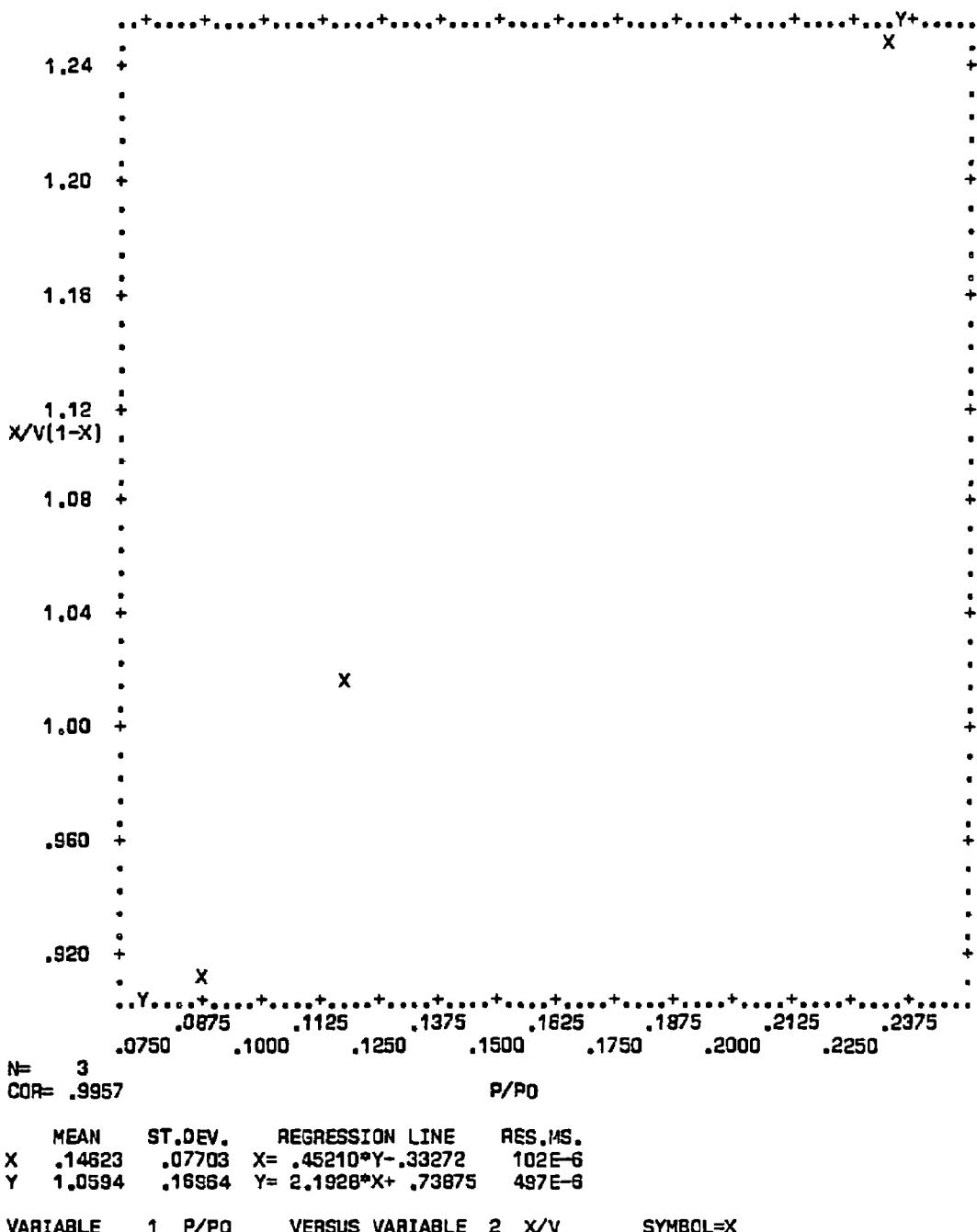
**Figure F-6.** Plot of BET equation versus relative pressure for Oxygen Sensor A230/0649X
