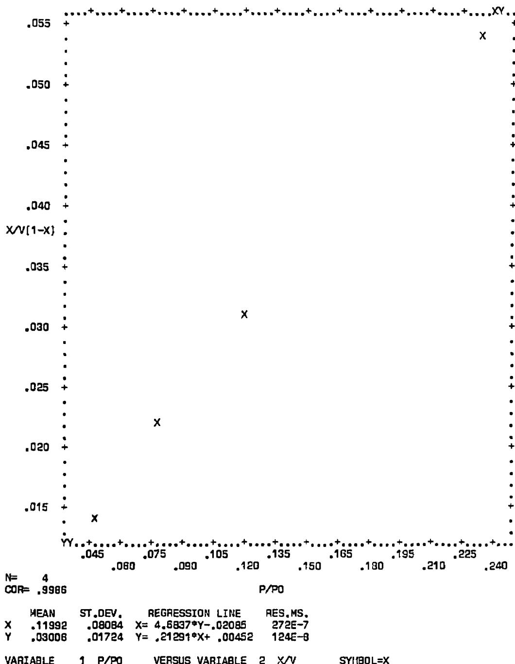
Figure C-65. Plot of BET equation versus relative pressure for
