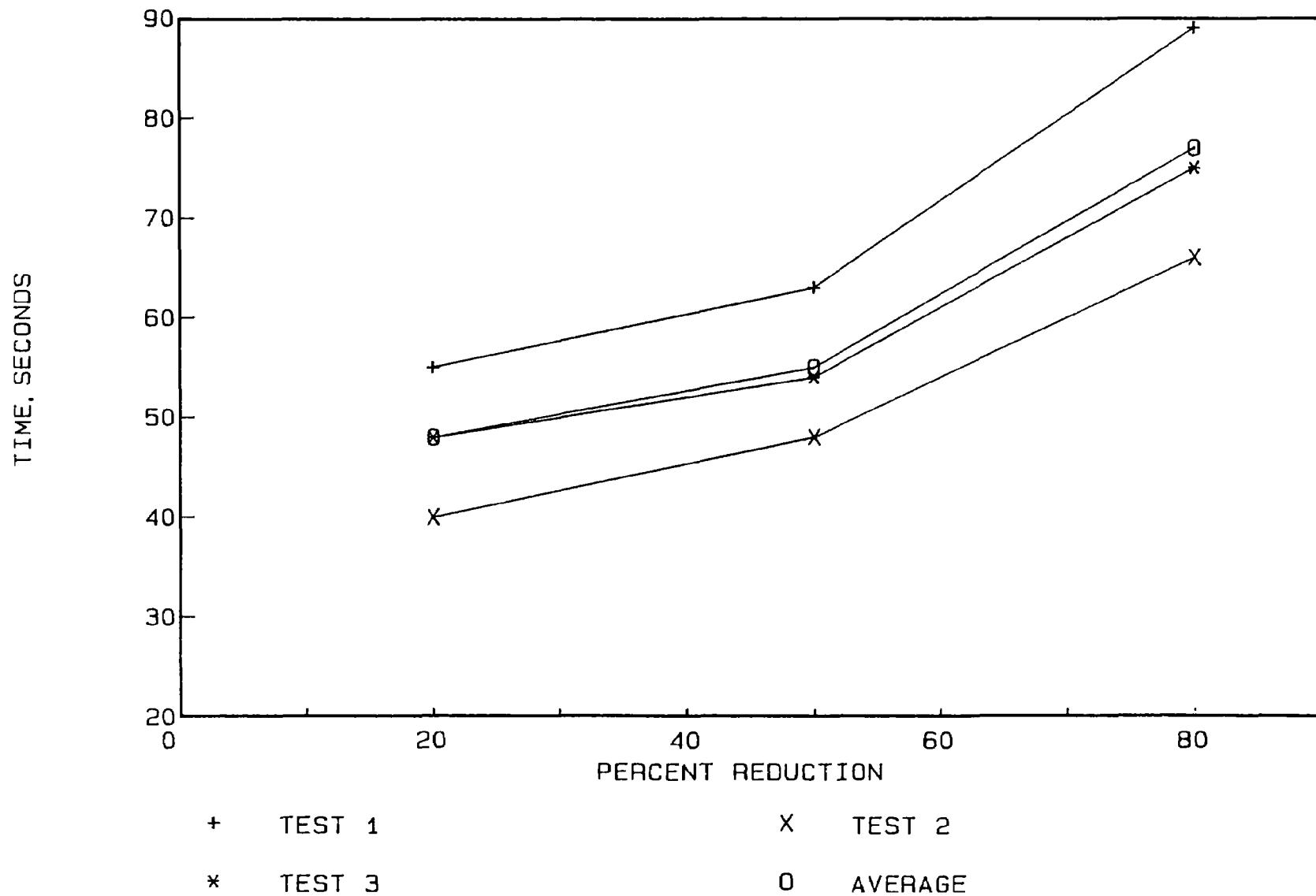
Figure 4. Percent reduction of HC from the light-off test for Converter EPA 1174R
