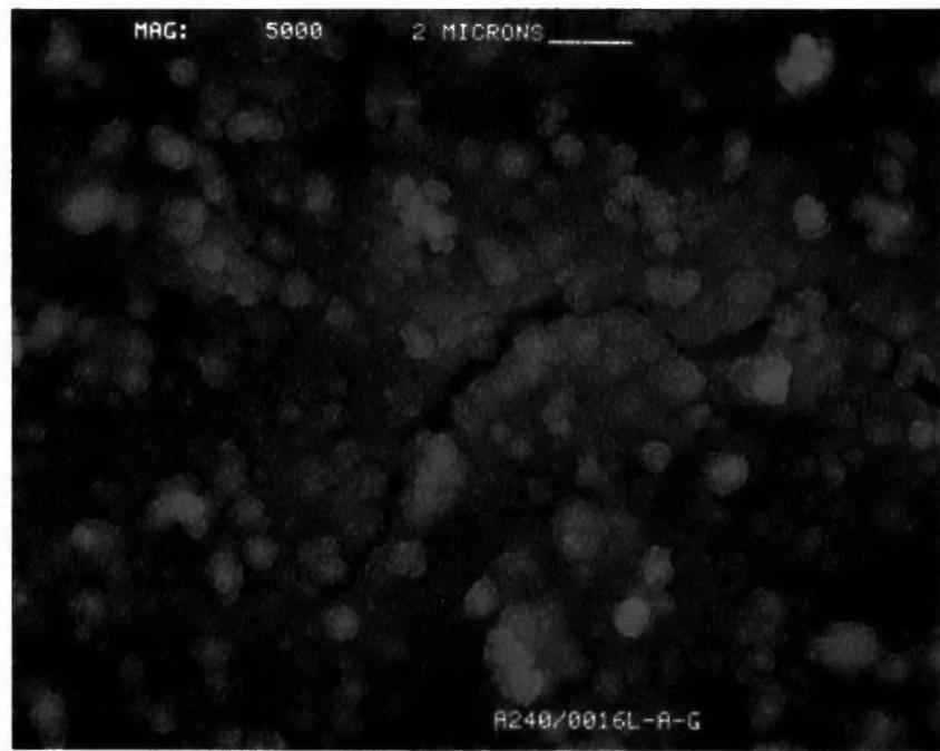
Figure D-284. Scanning Electron Micrograph at X5000 of Converter A240/0016L-Rear Face
