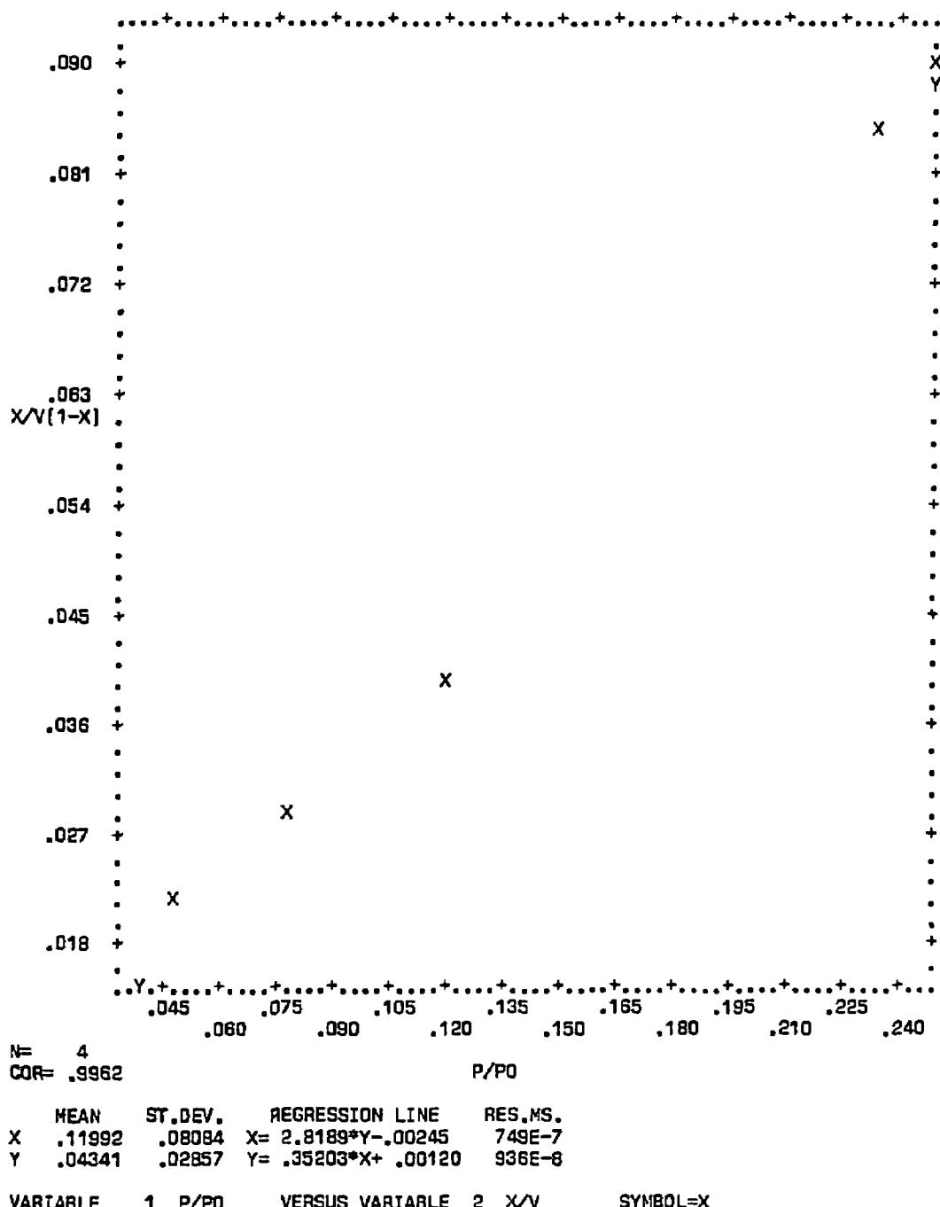
Figure C-67. Plot of BET equation versus relative pressure for Converter A240/0141L-B - Front Face
