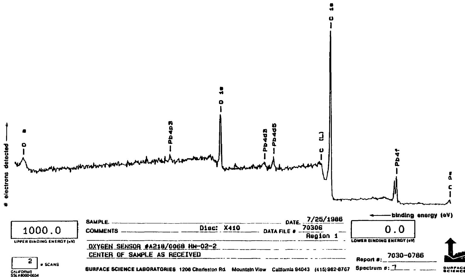
Figure G-26. ESCA Spectrum of Oxygen Sensor A218/0068 from 0 eV to 1000 eV (Exterior Surface)
