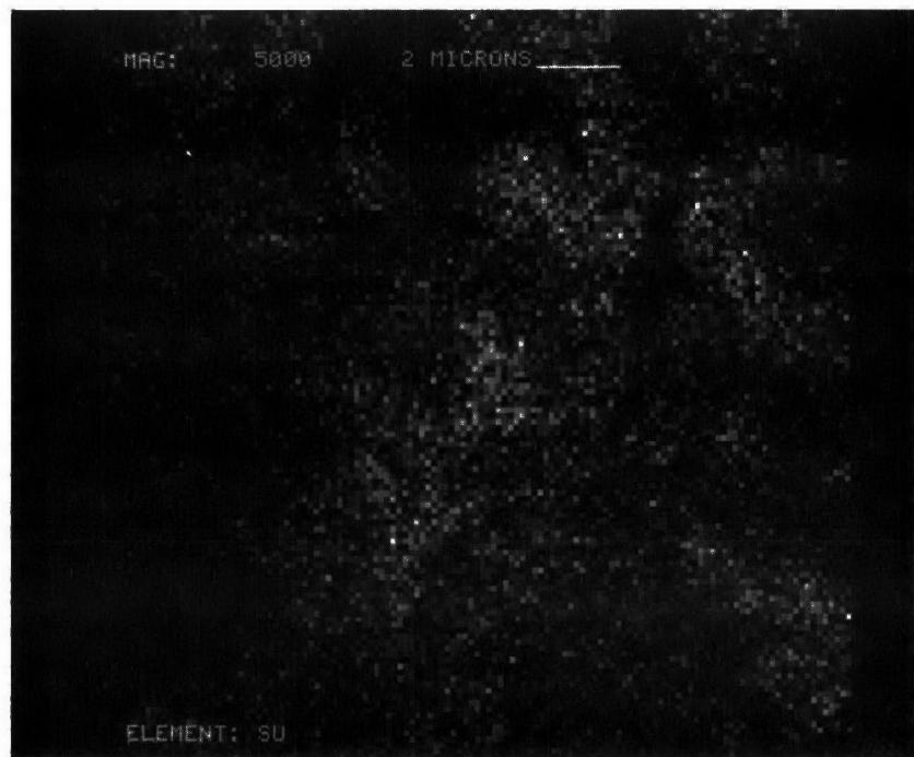
Figure D-88. Sulfur Dot Map at X5000 of Converter A221/0204
