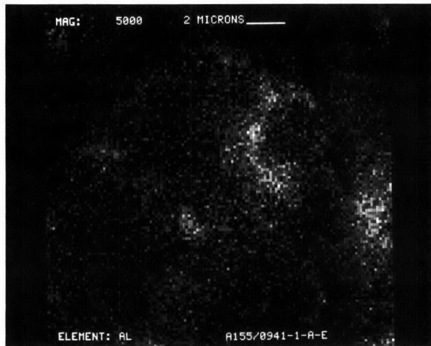
Figure D-215. Aluminum Dot Map at X5000 of Converter A155/0941-1
