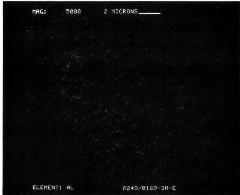
Figure D-195. Aluminum Dot Map at X5000 of Converter A249/0169-3
