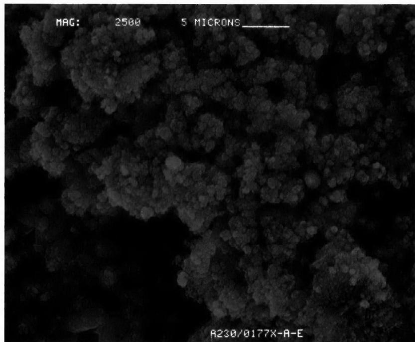
Figure D-103. Scanning Electron Micrograph at X2500 of Converter A230/0177X
