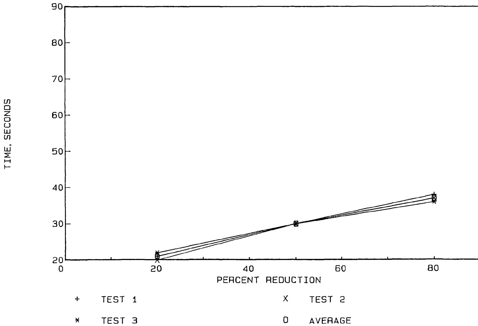
Figure 3. Percent reduction of CO from the light-off test for Converter A215/0201R
