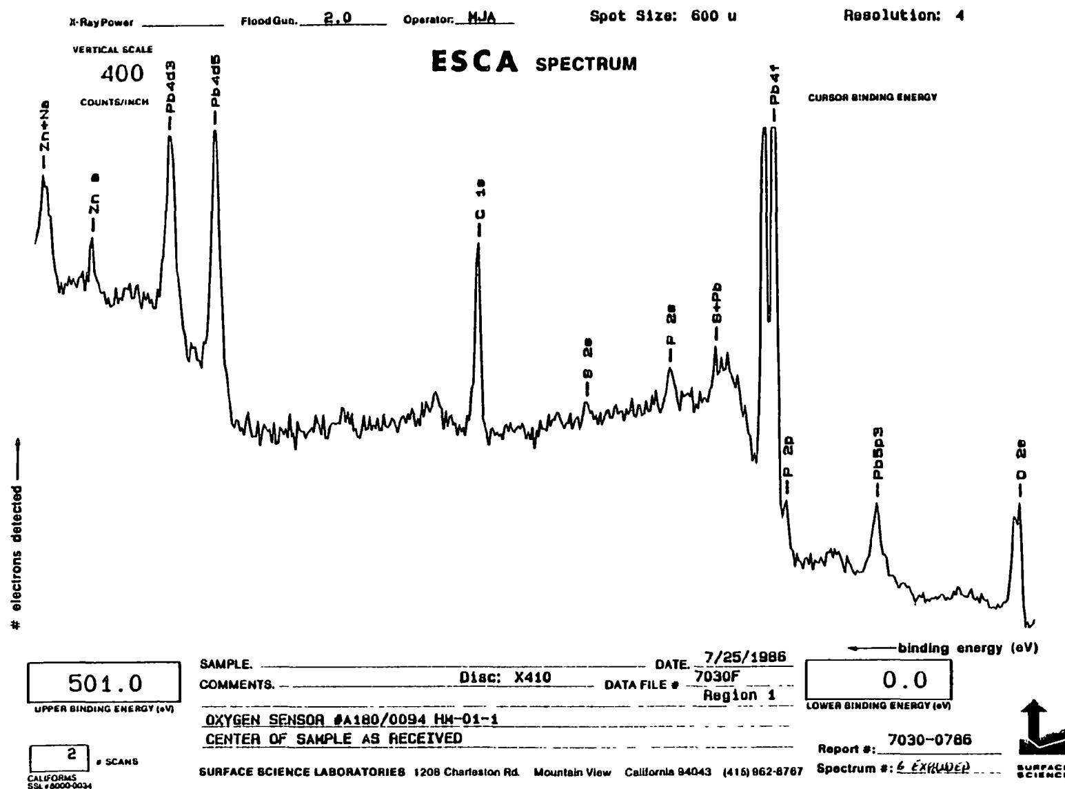
Figure G-18. ESCA Spectrum of Oxygen Sensor A180/0094 from 0 eV to 501 eV (Exterior Surface)
