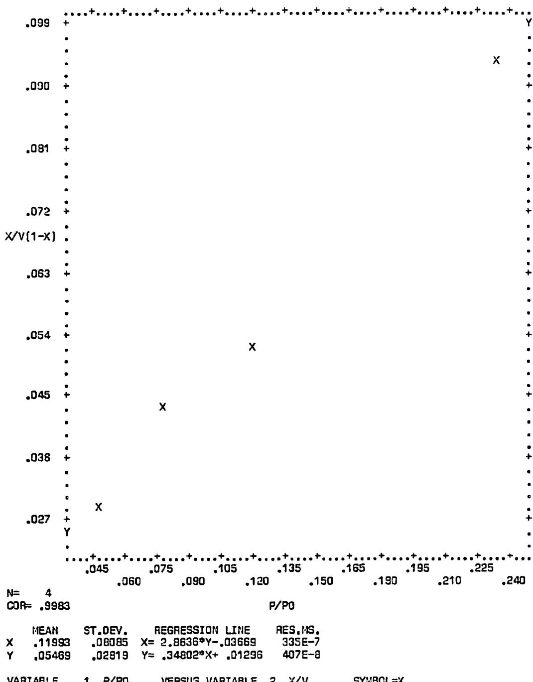
**Figure C-32. Plot of BET equation versus relative pressure for Converter A221/0152-B - Front Face**
