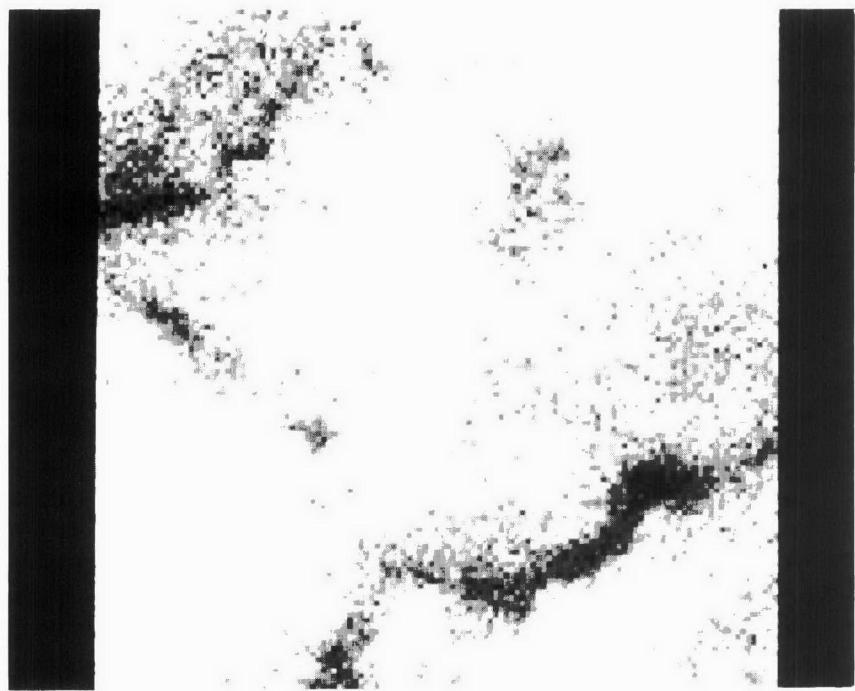
Figure D-257. Lead Dot Map at X5000 of Converter A220/0392-Rear Face
