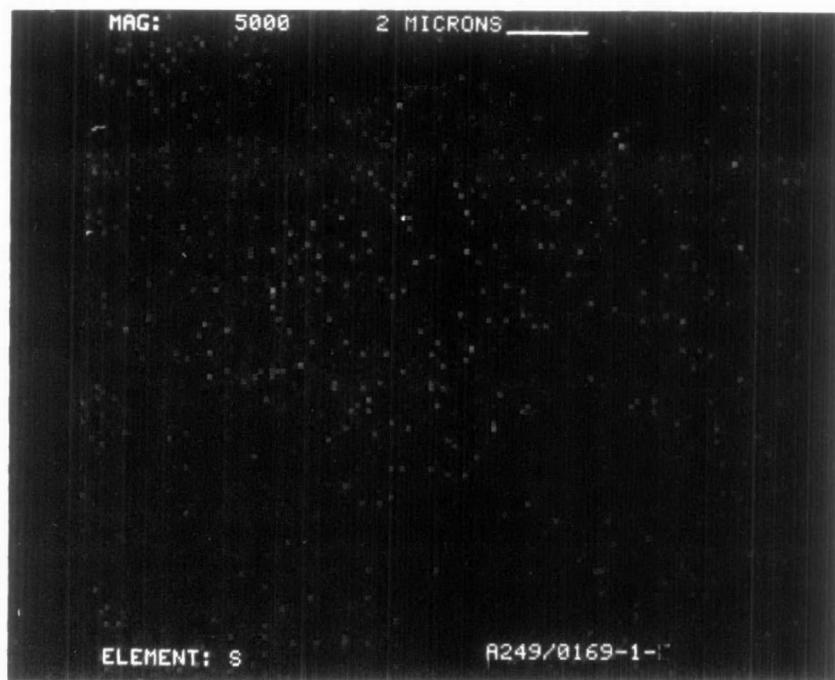
Figure D-288. Sulfur Dot Map at X5000 of Converter A249/0169-1-Rear Face
