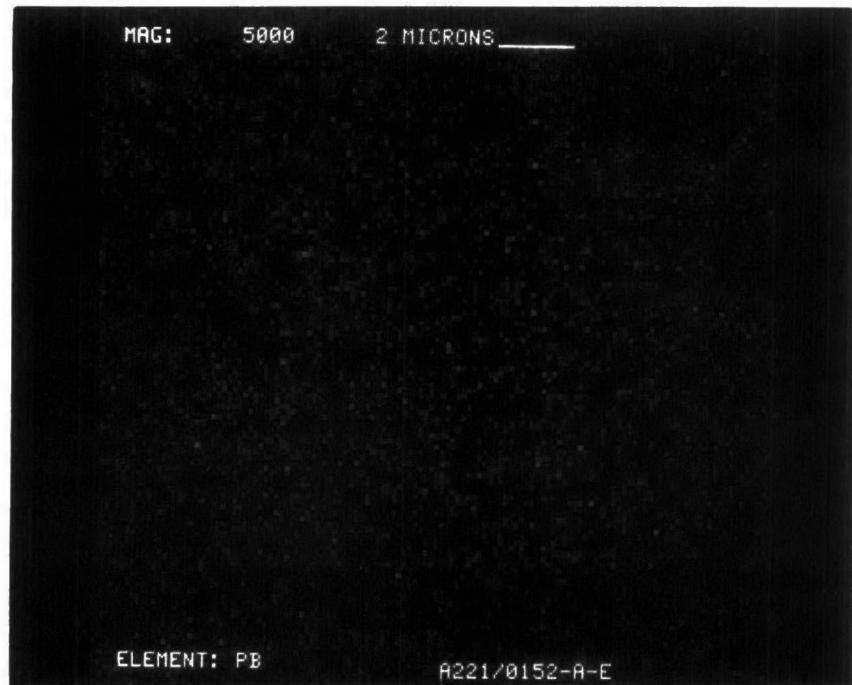
Figure D-77. Lead Dot Map at X5000 of Converter A221/0152
