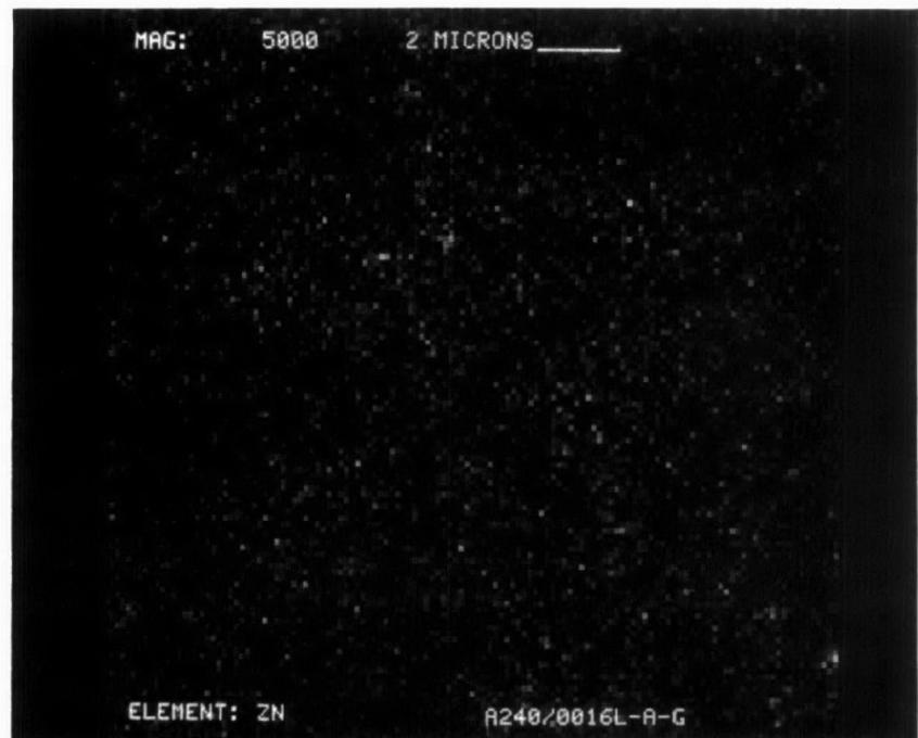
Figure D-289. Zinc Dot Map at X5000 of Converter A240/0016L-Rear Face
