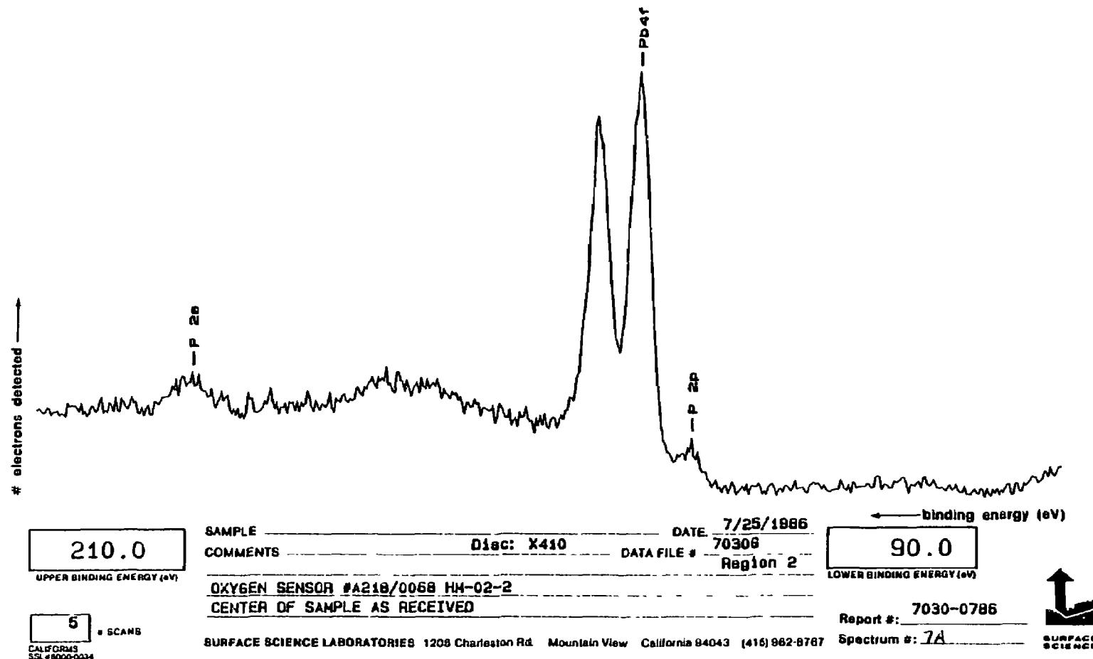
Figure G-28. ESCA Spectrum of Oxygen Sensor A218/0068 from 90 eV to 210 eV (Exterior Surface)
