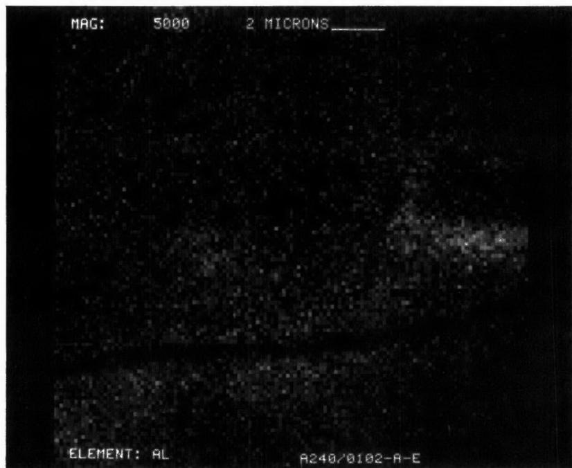
Figure D-135. Aluminum Dot Map at X5000 of Converter A240/0102
