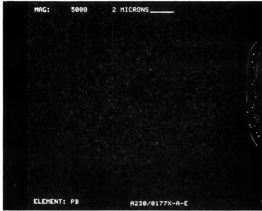
Figure D-107. Lead Dot Map at X5000 of Converter A230/0177X
