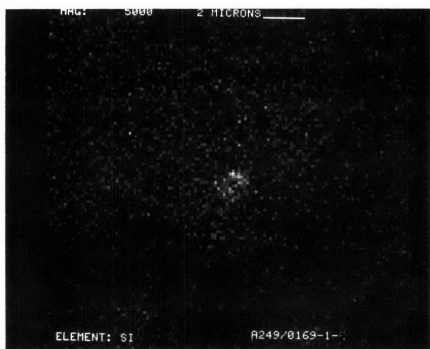
Figure D-286. Silicon Dot Map at X5000 of Converter A249/0169-1-Rear Face
