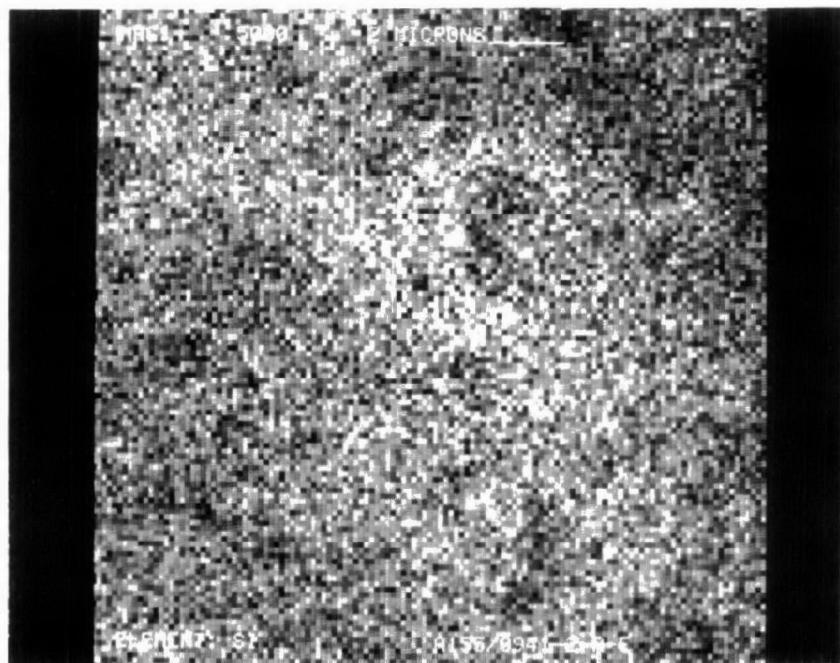
Figure D-226. Silicon Dot Map at X5000 of Converter A155/0941-2
