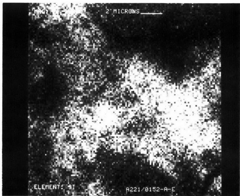
Figure D-76. Silicon Dot Map at X5000 of Converter A221/0152
