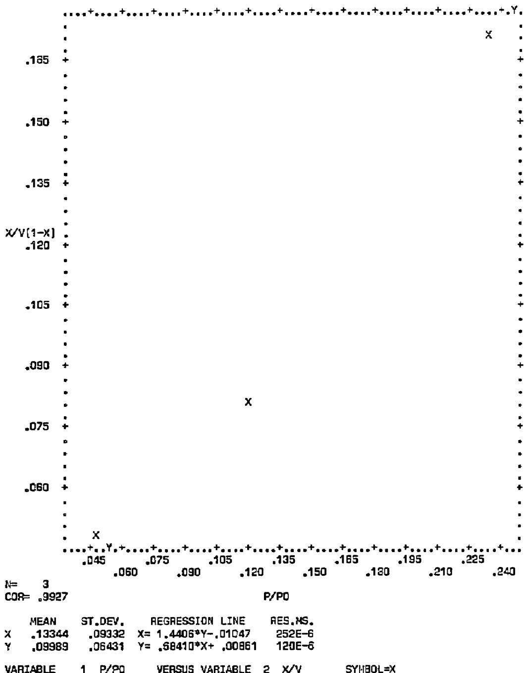
Figure C-36. Plot of BET equation versus relative pressure for Converter A221/0204-B - Bulk
