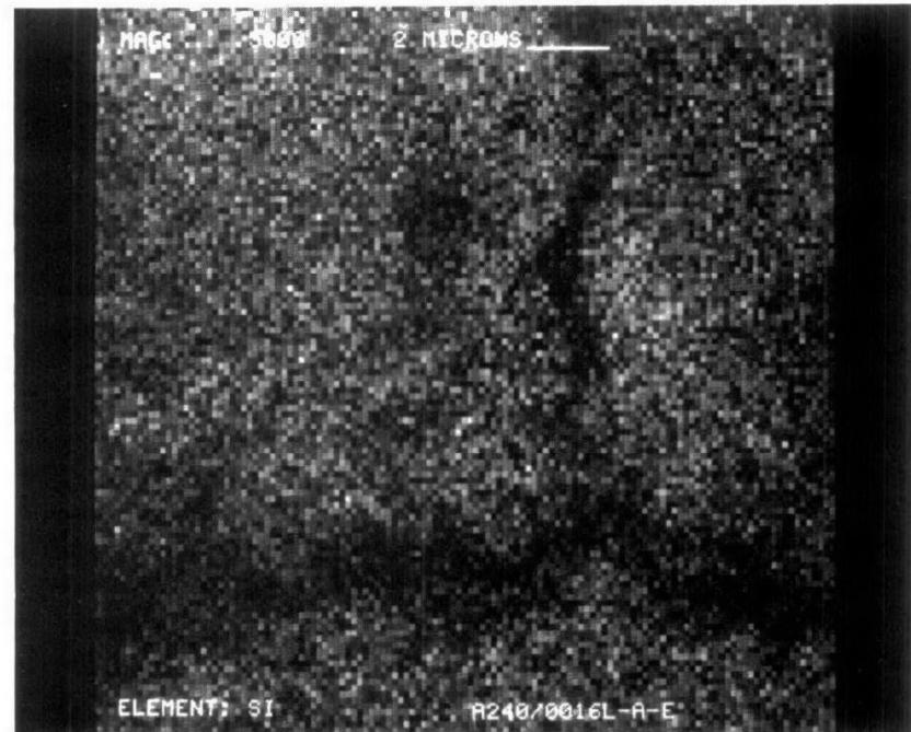
Figure D-126. Silicon Dot Map at X5000 of Converter A240/0016L
