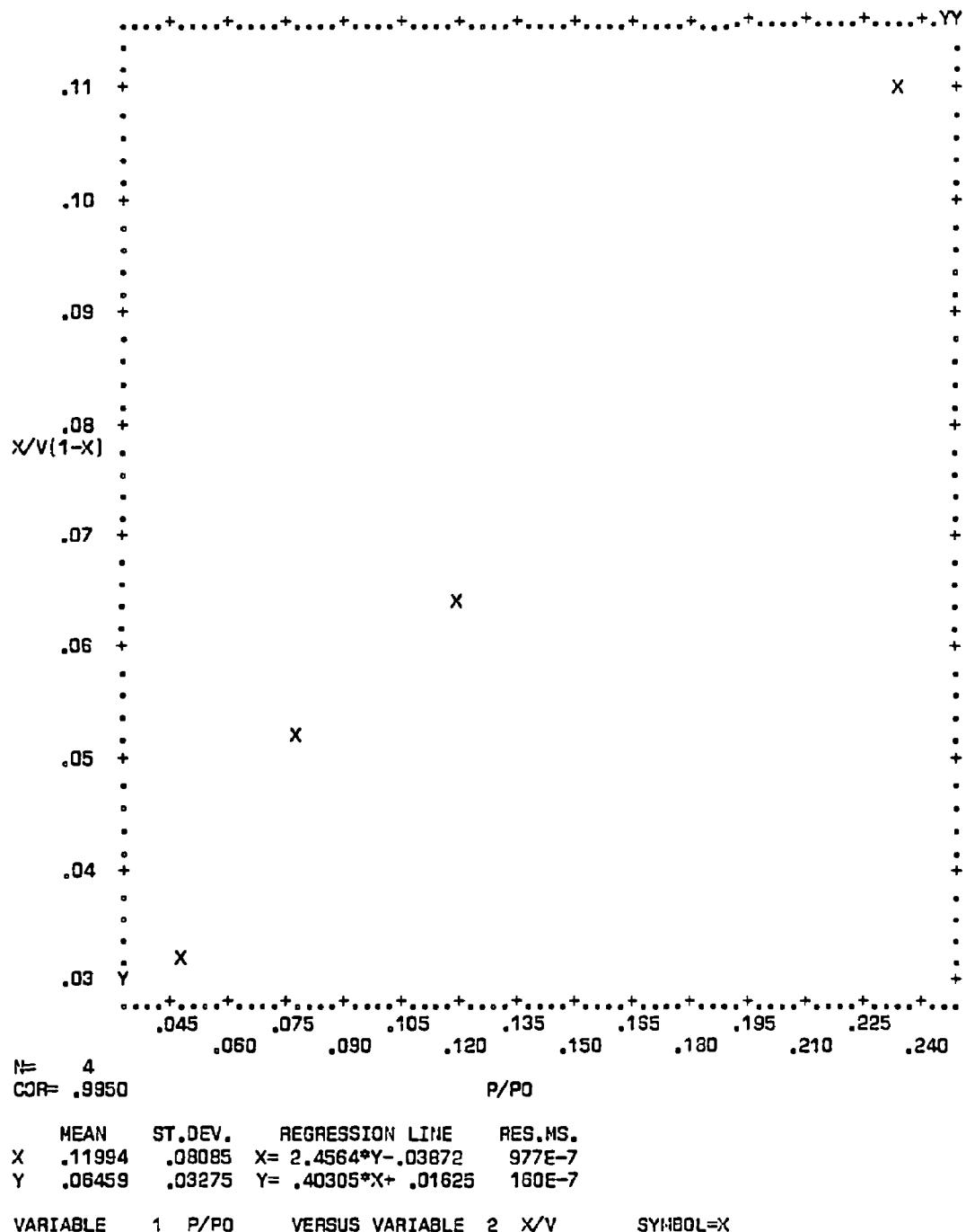
Figure C-28. Plot of BET equation versus relative pressure for Converter A221/0152-A - Bulk
