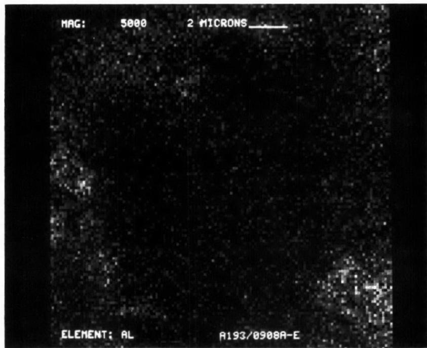
Figure D-15. Aluminum Dot Map at X5000 of Converter A193/0908
