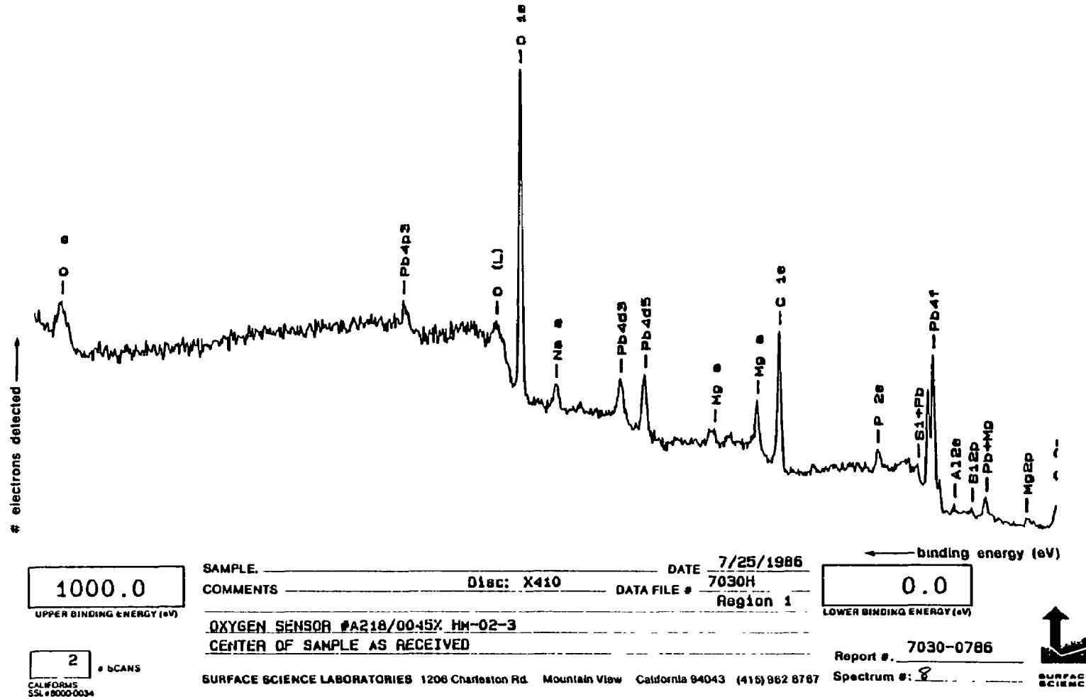
Figure G-23. ESCA Spectrum of Oxygen Sensor A218/0045X from 0 eV to 1000 eV (Exterior Surface)
