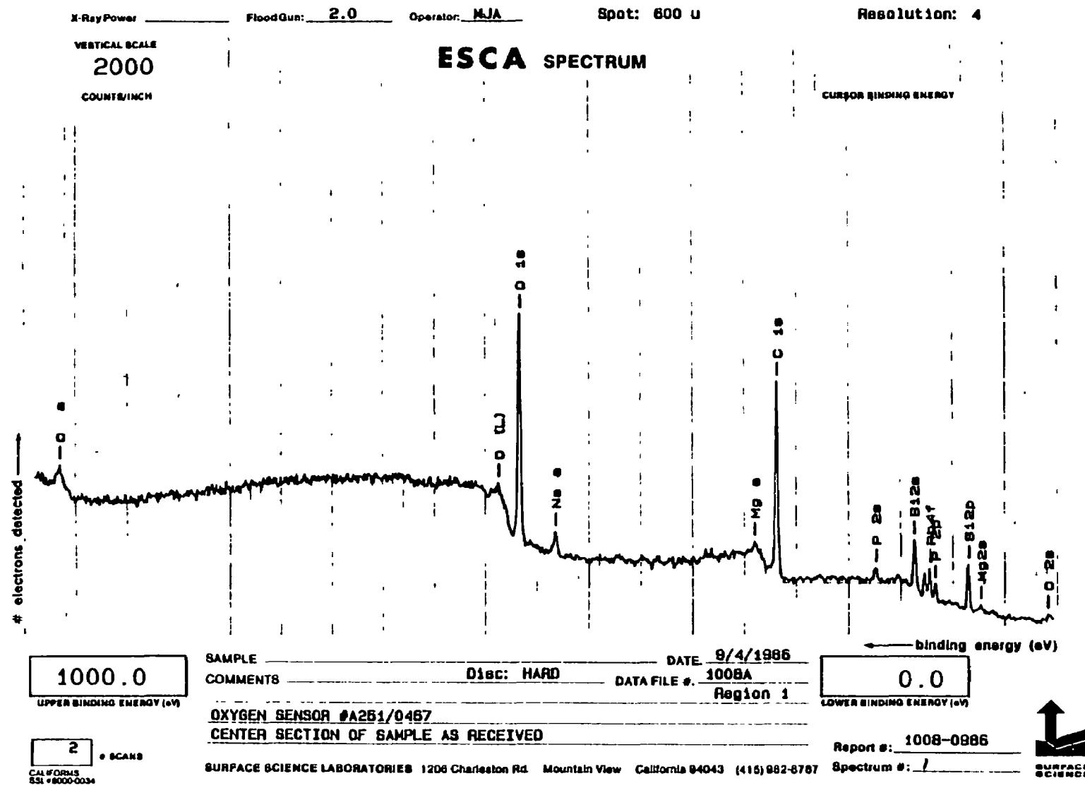
Figure G-15. ESCA Spectrum of Oxygen Sensor A251/0467 from 0 eV to 1000 eV (Exterior Surface)
