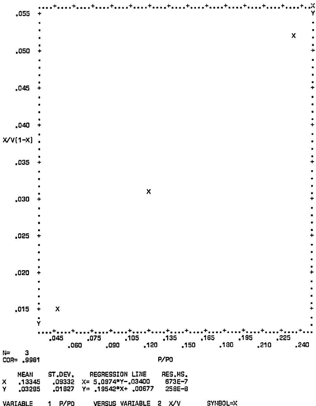
Figure C-55. Plot of BET equation versus relative pressure for Converter A240/0016L-A - Rear Face
