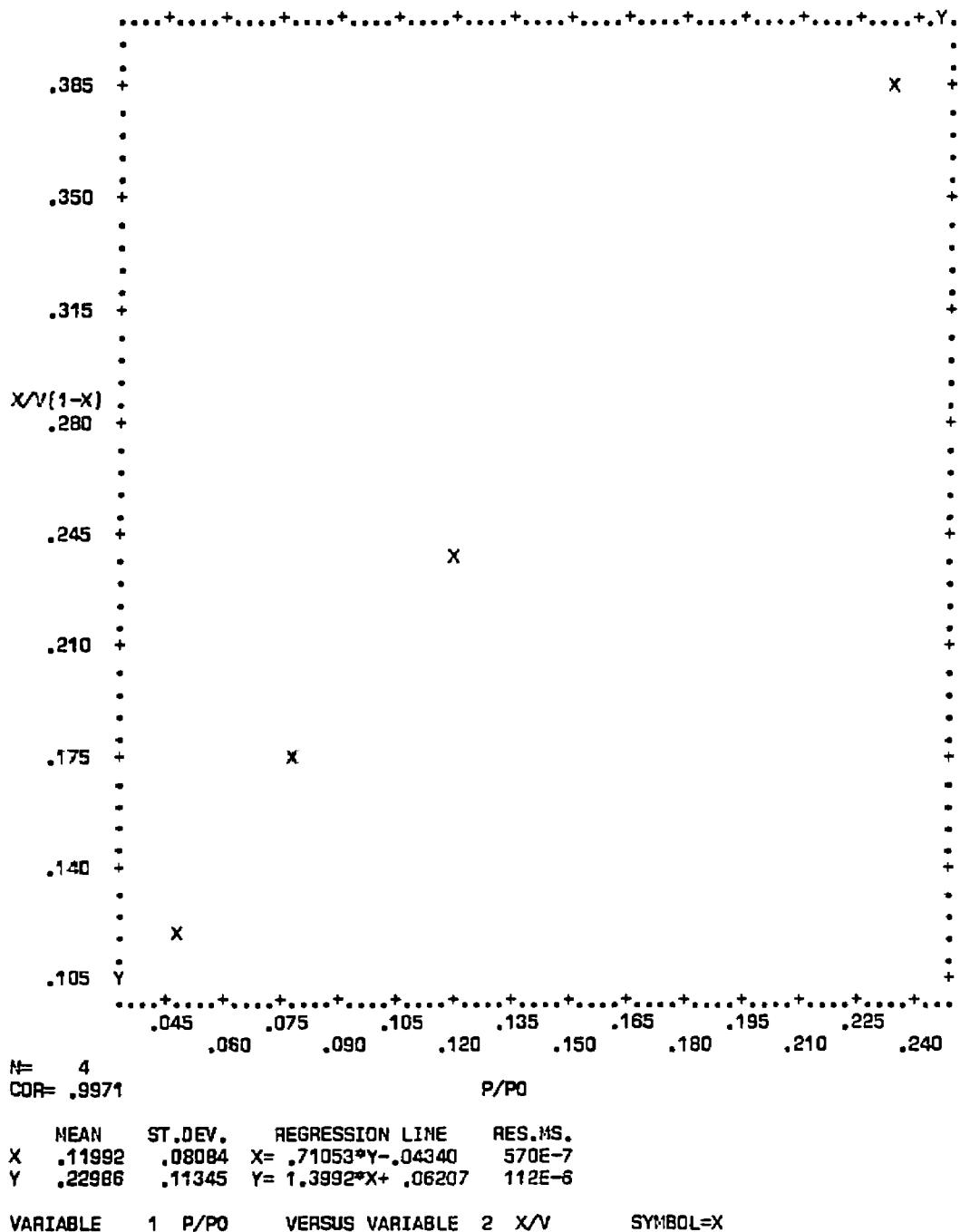
Figure C-33. Plot of BET equation versus relative pressure for Converter A221/0204-A - Bulk
