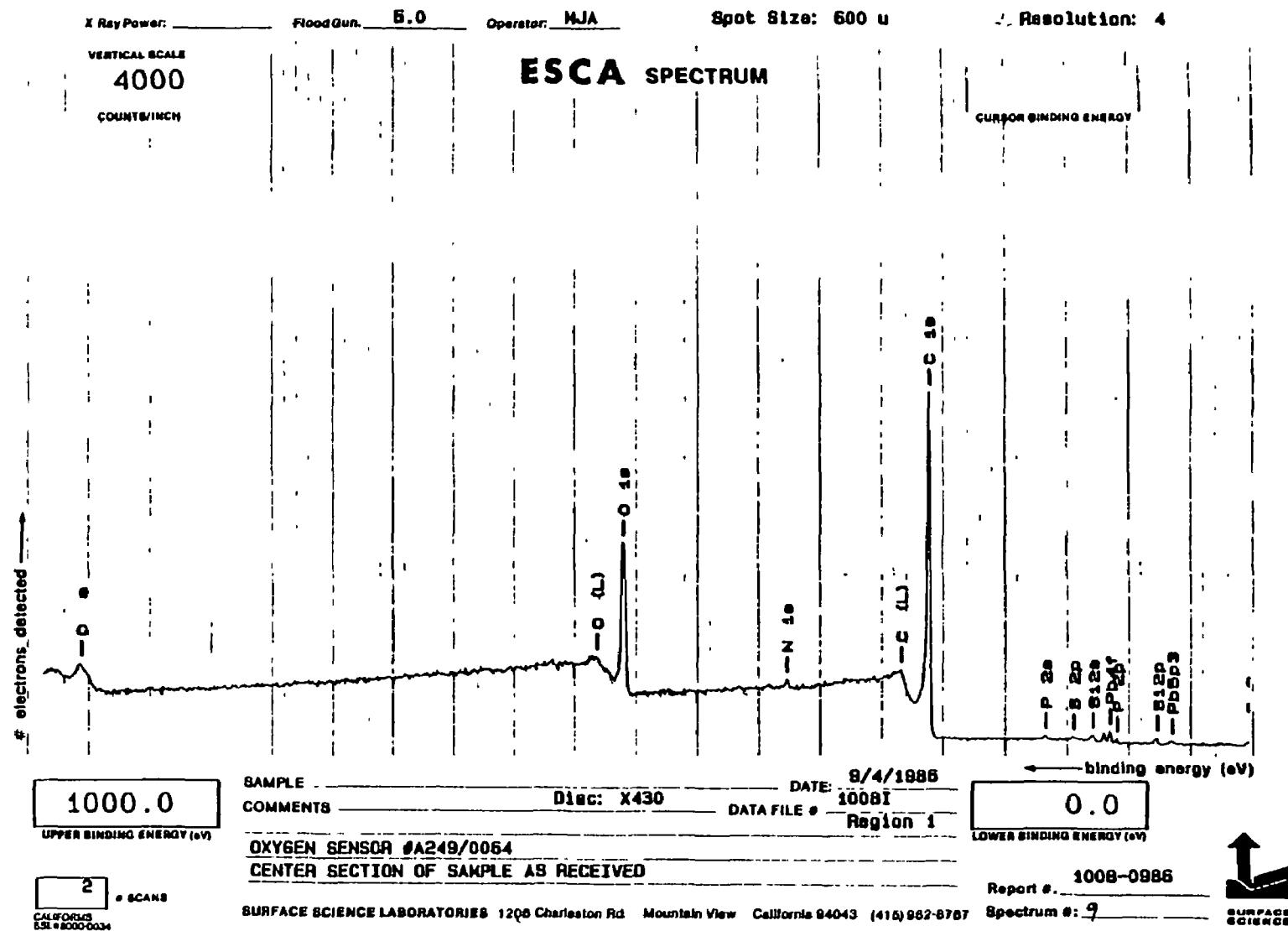
Figure G-13. ESCA Spectrum of Oxygen Sensor A249/0064 from 0 eV to 1000 eV (Exterior Surface)
