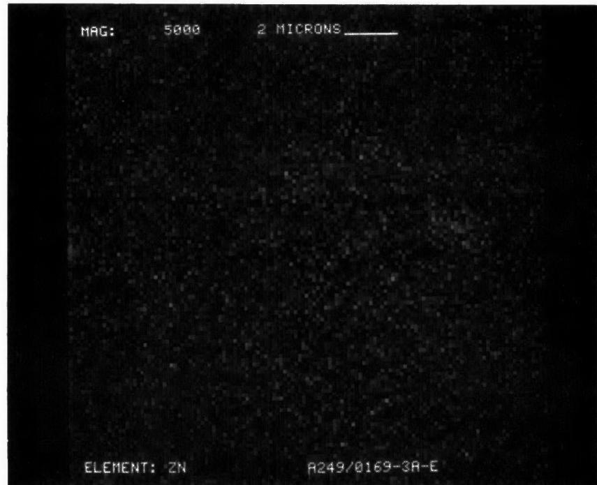
Figure D-199. Zinc Dot Map at X5000 of Converter A249/0169-3
