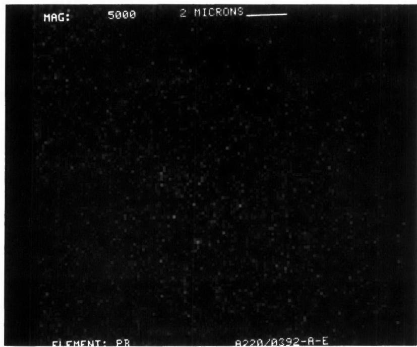
Figure D-57. Lead Dot Map at X5000 of Converter A220/0392
