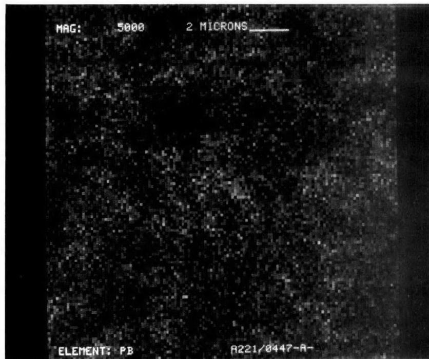
Figure D-97. Lead Dot Map at X5000 of Converter A221/0447
