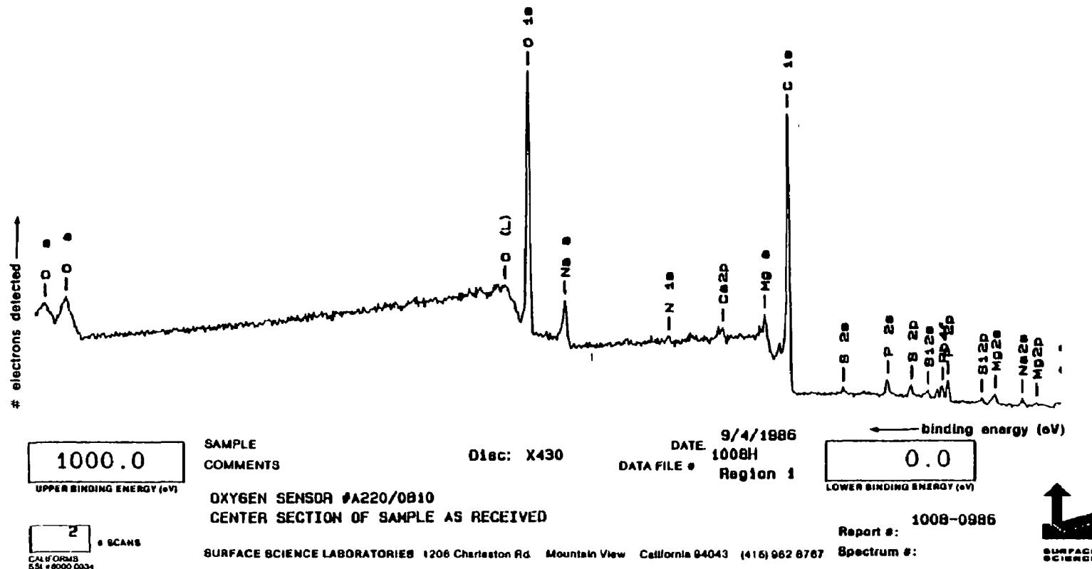
Figure G-3. ESCA Spectrum of Oxygen Sensor A220/0810 from 0 eV to 1000 eV (Exterior Surface)
