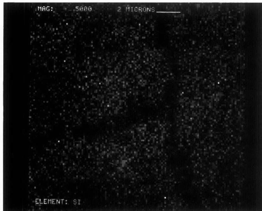
Figure D-26. Silicon Dot Map at X5000 of Converter A218/0045
