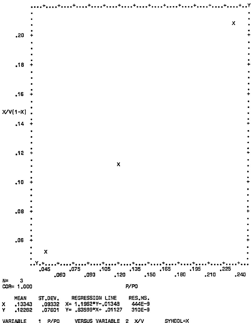
Figure C-89. Plot of BET equation versus relative pressure for Converter A280/0001L-A - Bulk
