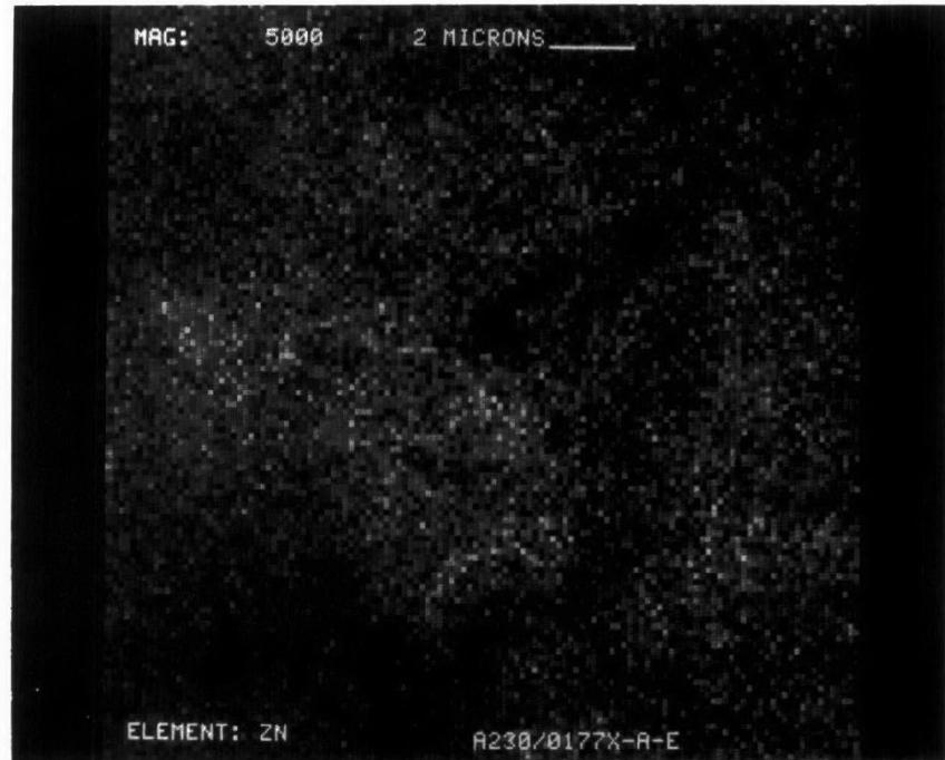
Figure D-109. Zinc Dot Map at X5000 of Converter A230/0177X
