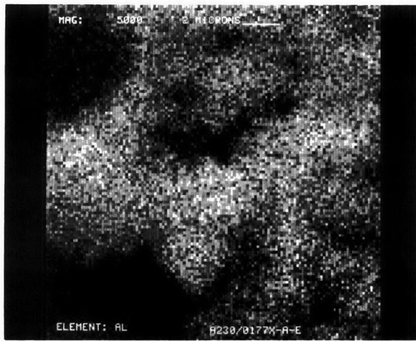
Figure D-105. Aluminum Dot Map at X5000 of Converter A230/0177X
