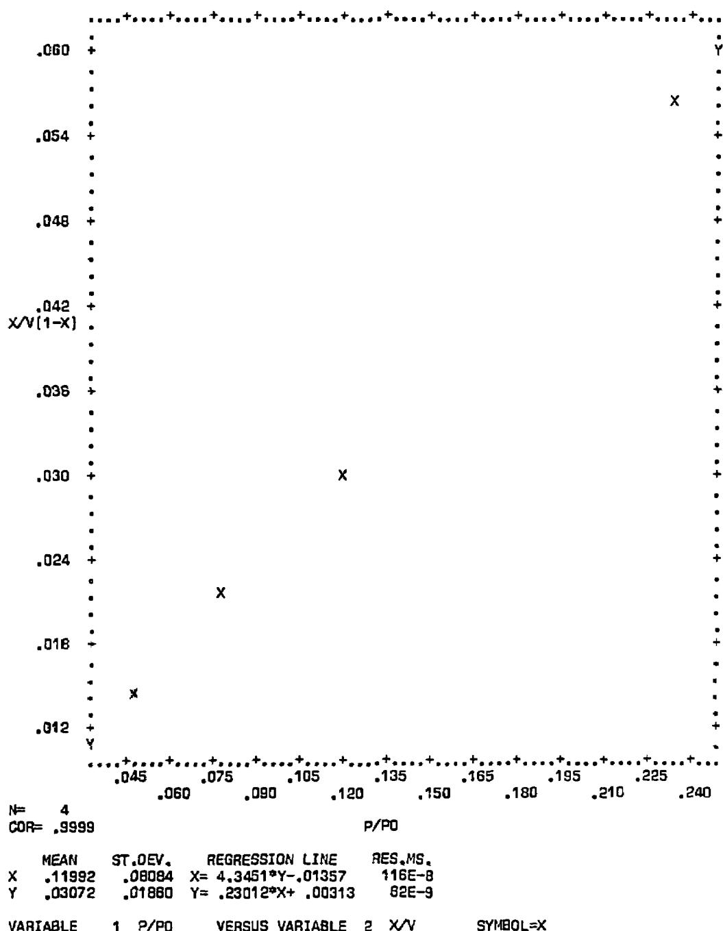
Figure C-63. Plot of BET equation versus relative pressure for Converter A240/0141L-A - Bulk
