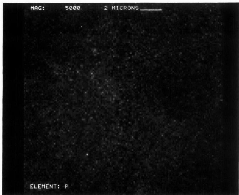
Figure D-150. Phosphorus Dot Map at X5000 of Converter A240/0141L
