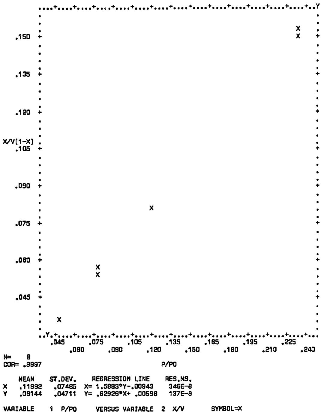
Figure C-78. Plot of BET equation versus relative pressure for Converter A249/0169-1 - Bulk
