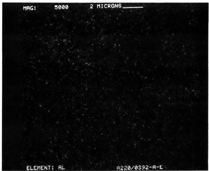
Figure D-55. Aluminum Dot Map at X5000 of Converter A220/0392
