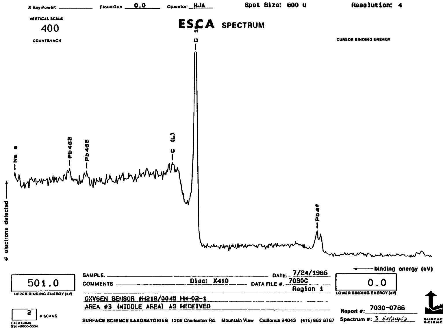
Figure G-21. ESCA Spectrum of Oxygen Sensor A218/0045 from 0 eV to 501 eV (Exterior Surface)
