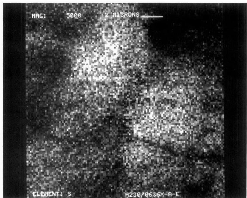
Figure D-118. Sulfur Dot Map at X5000 of Converter A230/0636X
