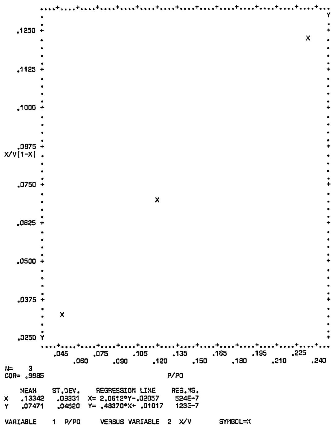
Figure C-98. Plot of BET equation versus relative pressure for Converter A155/0941-1-B - Front Face
