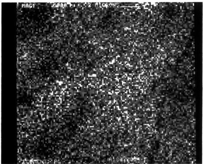
Figure D-10. Phosphorus Dot Map at X5000 of Converter A180/0094
