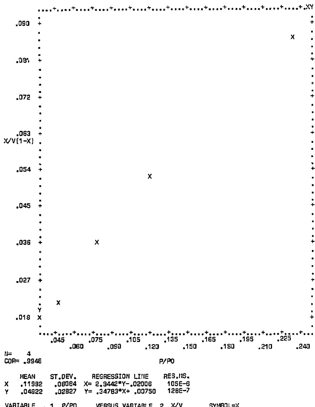
Figure C-30. Plot of BET equation versus relative pressure for Converter A221/0152-A - Rear Face
