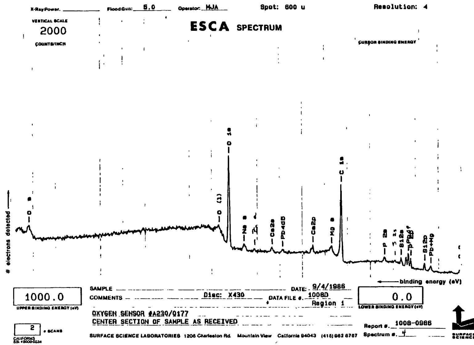
Figure G-9. ESCA Spectrum of Oxygen Sensor A230/0177 from 0 eV to 1000 eV (Exterior Surface)
