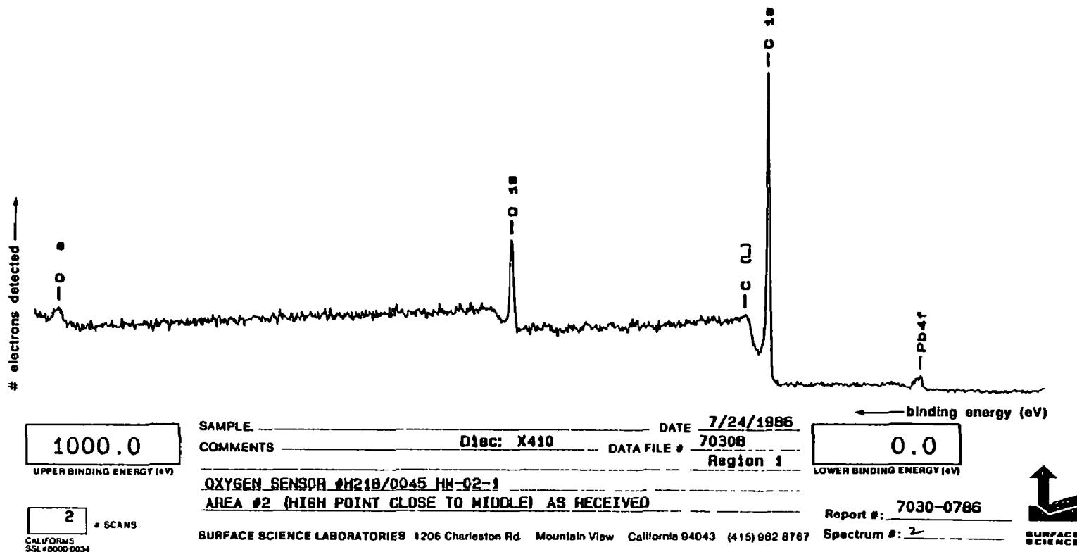
Figure I-3. ESCA Spectrum of Oxygen Sensor A218/0045 from 0 eV to 1000 eV (Location 2)
