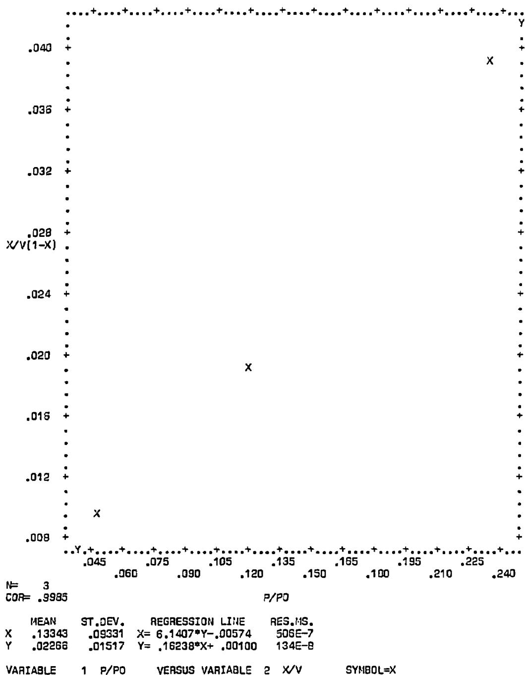
Figure C-69. Plot of BET equation versus relative pressure for Converter A240/0153-A - Front Face
