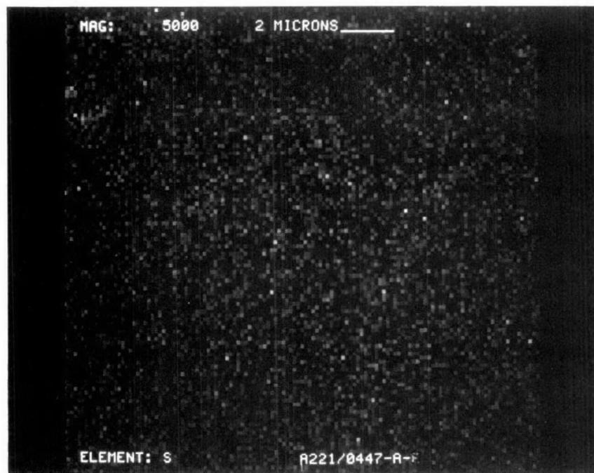
Figure D-268. Sulfur Dot Map at X5000 of Converter A221/0447-Rear Face
