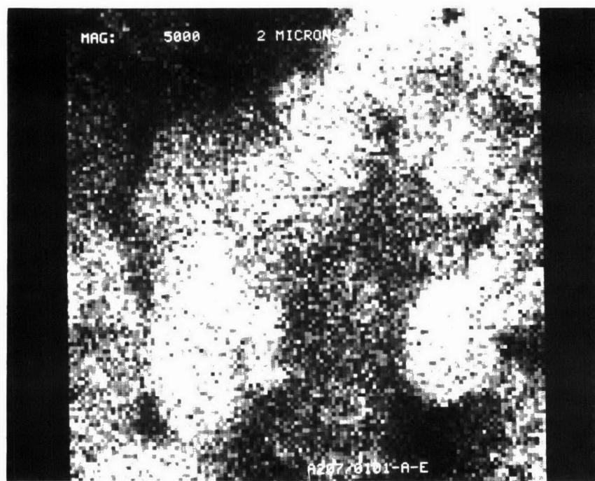
Figure D-240. Phosphorus Dot Map at X5000 of Converter A207/0101
