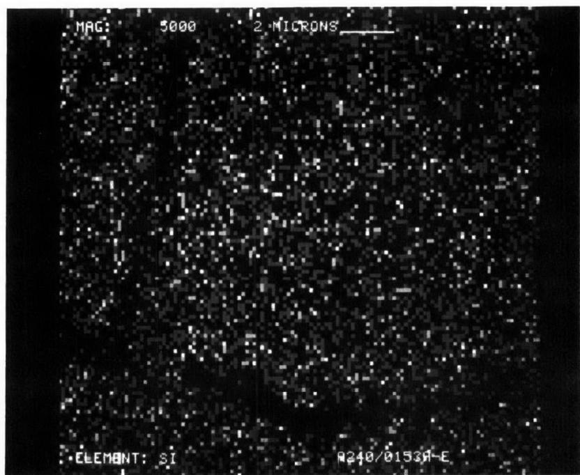
Figure D-156. Silicon Dot Map at X5000 of Converter A240/0153
