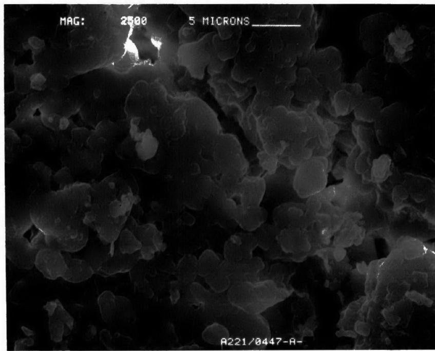
**Figure D-263.** Scanning Electron Micrograph at X2500 of Converter A221/0447-Rear Face
