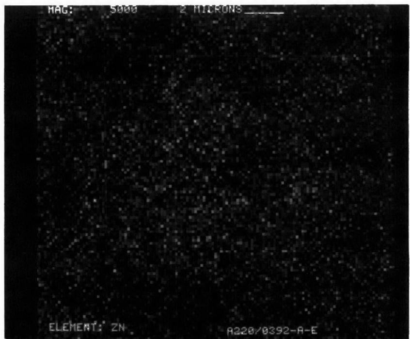
Figure D-59. Zinc Dot Map at X5000 of Converter A220/0392
