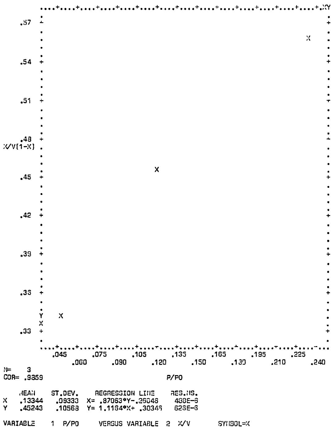
Figure F-12. Plot of BET equation versus relative pressure for Oxygen Sensor A218/0063
