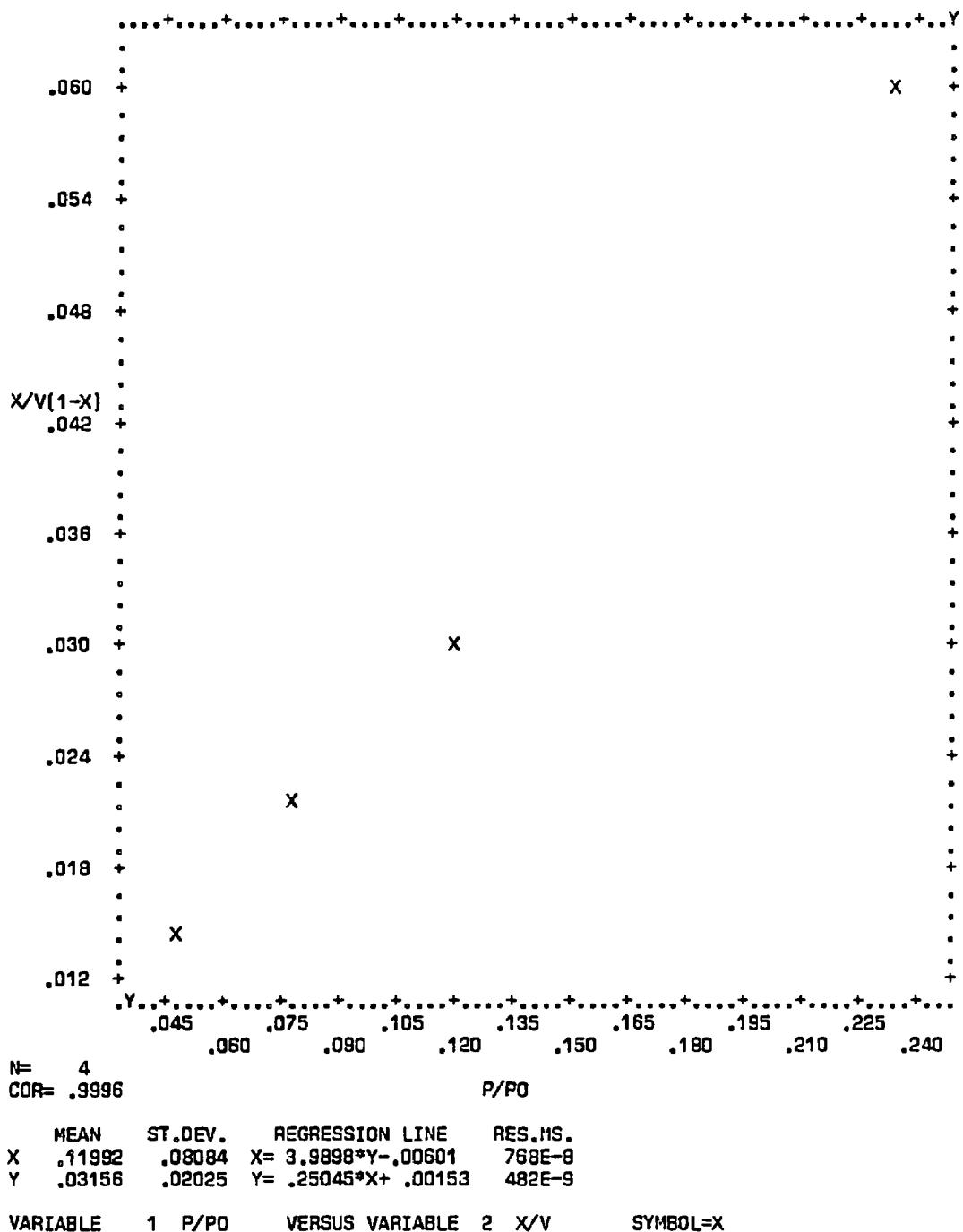
**Figure C-18.** Plot of BET equation versus relative pressure for Converter A220/0392-A - Bulk
