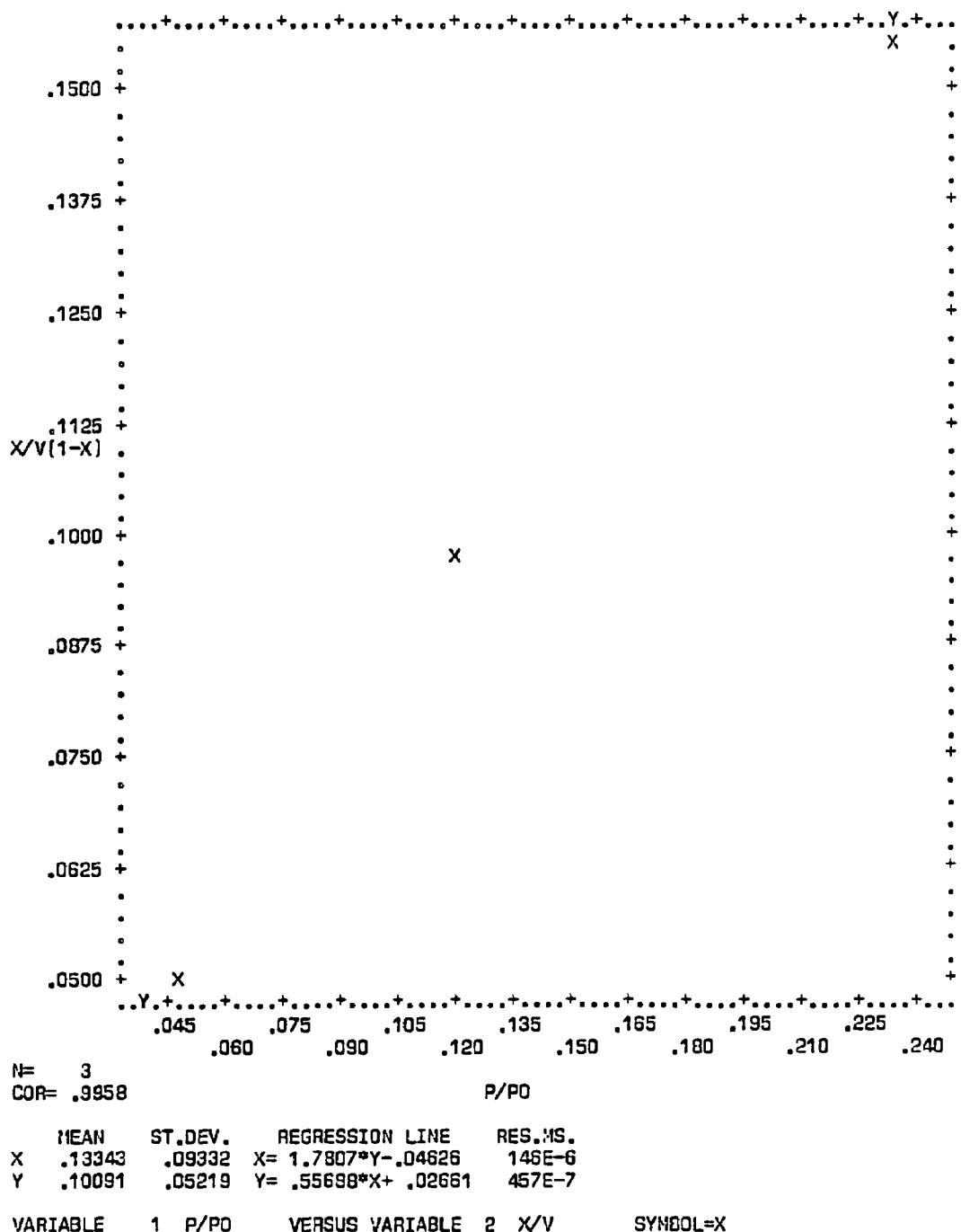
**Figure C-90. Plot of BET equation versus relative pressure for Converter A280/0001L-A - Front Face**
