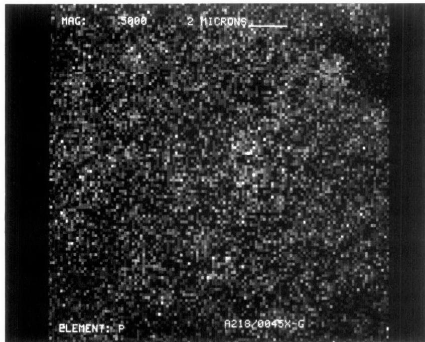
Figure D-250. Phosphorus Dot Map at X5000 of Converter A218/0045X-Rear Face
