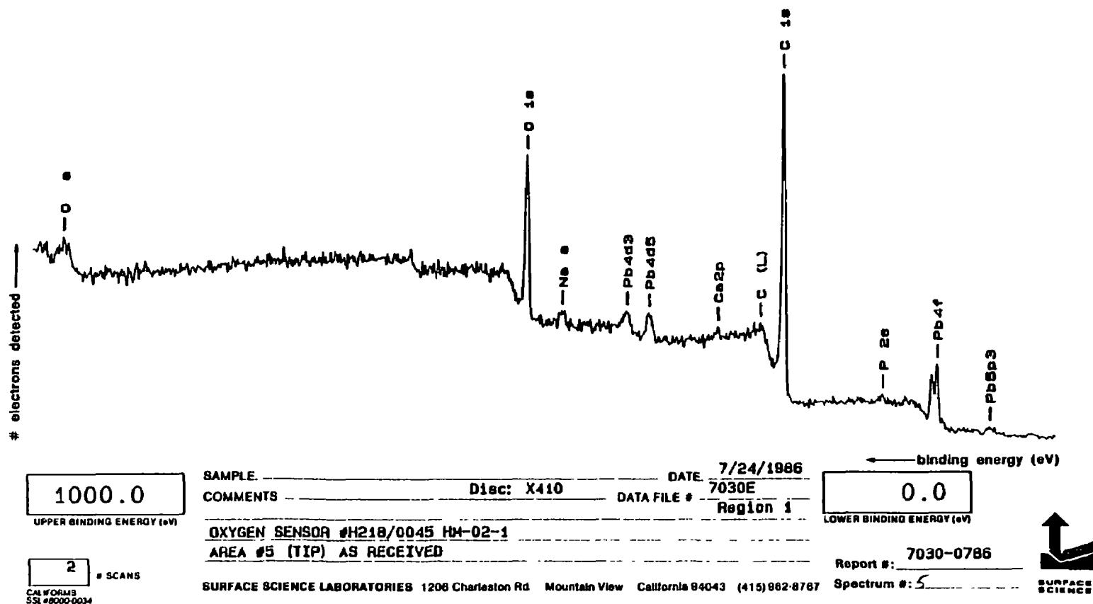
Figure I-10. ESCA Spectrum of Oxygen Sensor A218/0045 from 0 eV to 1000 eV (Location 5)
