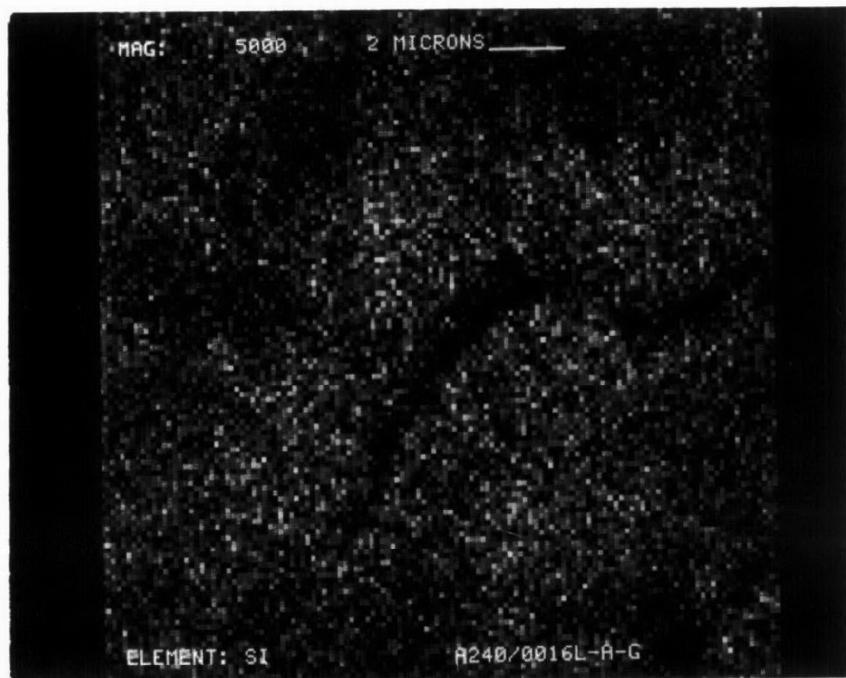
Figure D-286. Silicon Dot Map at X5000 of Converter A240/0016L-Rear Face
