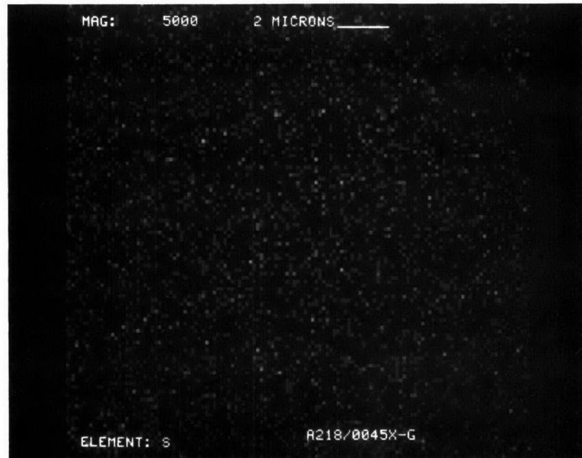
Figure D-248. Sulfur Dot Map at X5000 of Converter A218/0045X-Rear Face
