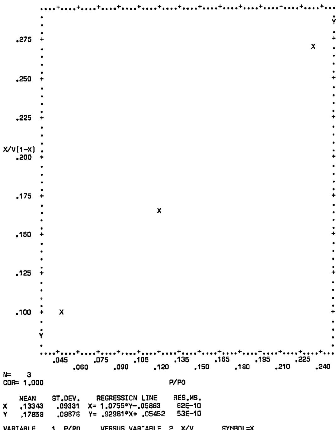
Figure C-100. Plot of BET equation versus relative pressure for Converter A155/0941-2-A - Front Face
