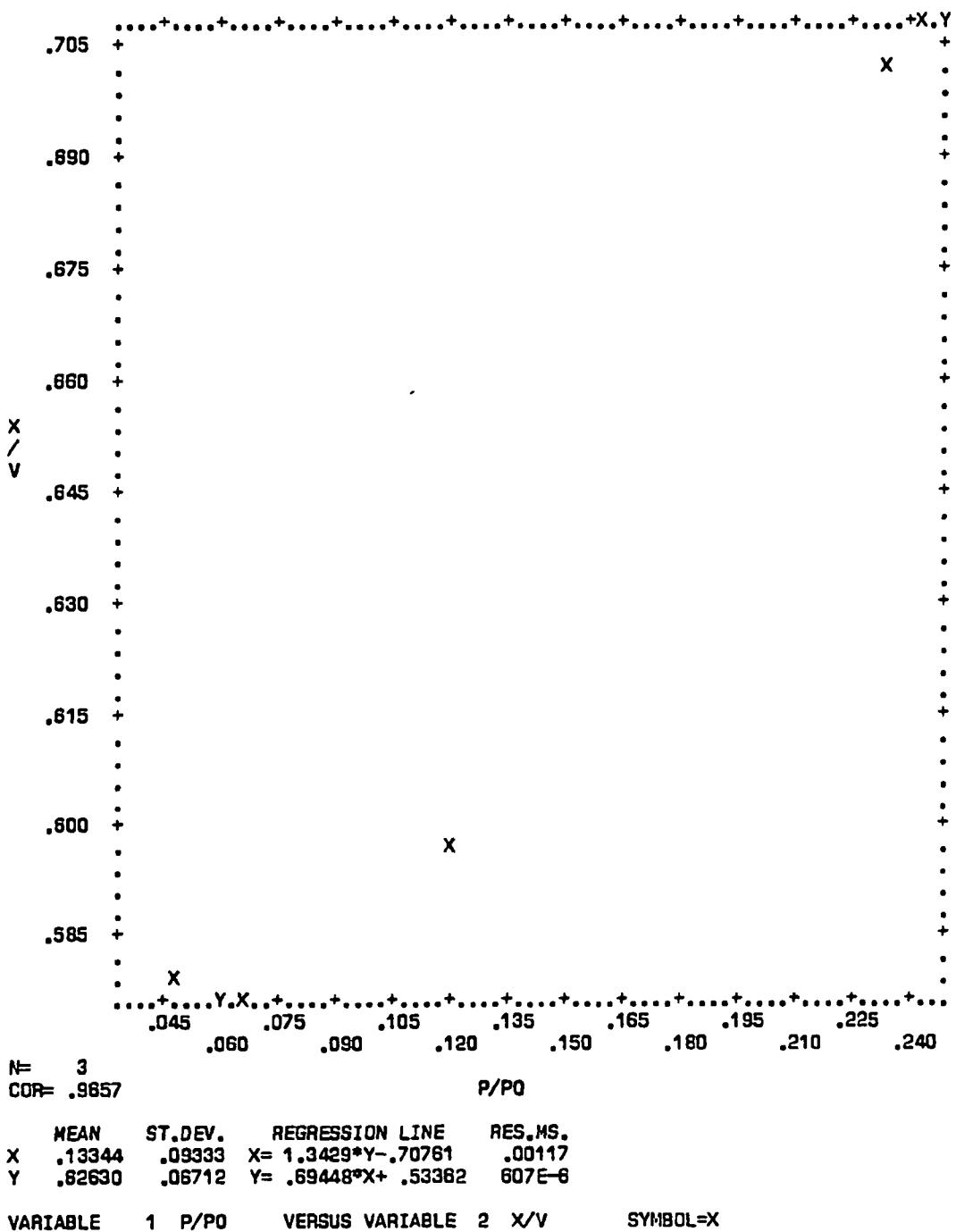
Figure F-9. Plot of BET equation versus relative pressure
