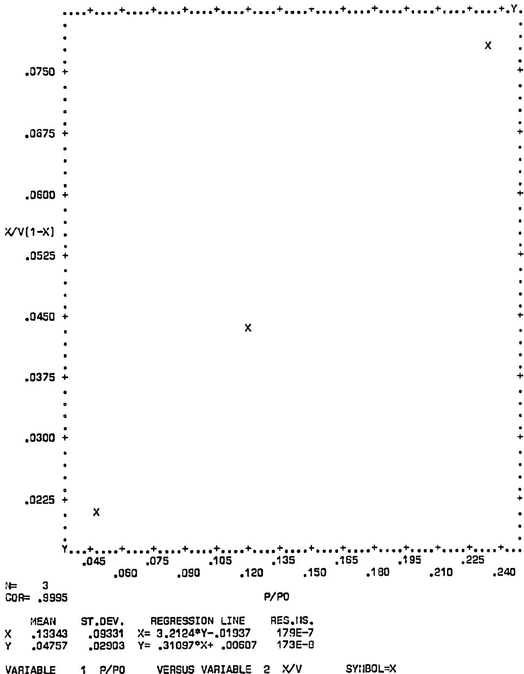
Figure C-72. Plot of BET equation versus relative pressure for Converter A240/0153-B - Front Face
