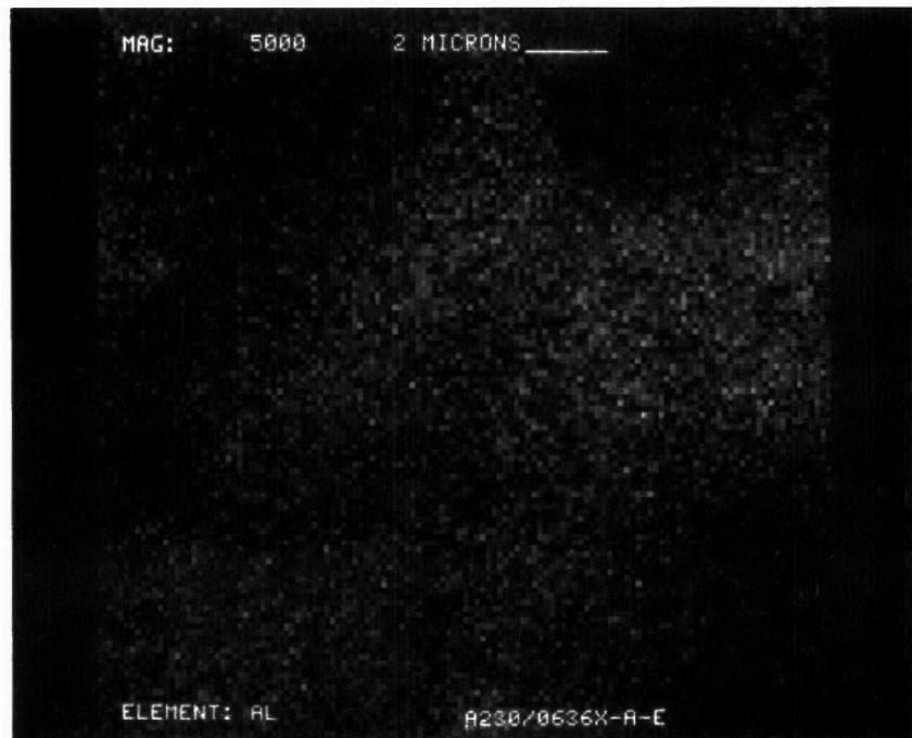
Figure D-115. Aluminum Dot Map at X5000 of Converter A230/0636X
