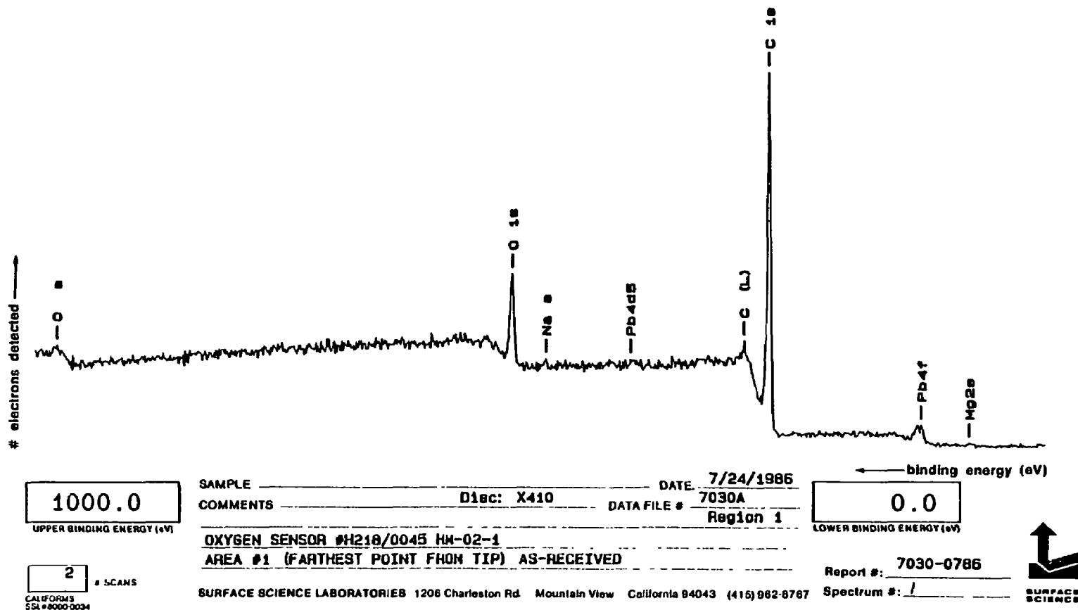
Figure I-1. ESCA Spectrum of Oxygen Sensor A218/0045 from 0 eV to 1000 eV (Location 1)
