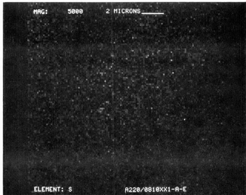
Figure D-68. Sulfur Dot Map at X5000 of Converter A220/0810
