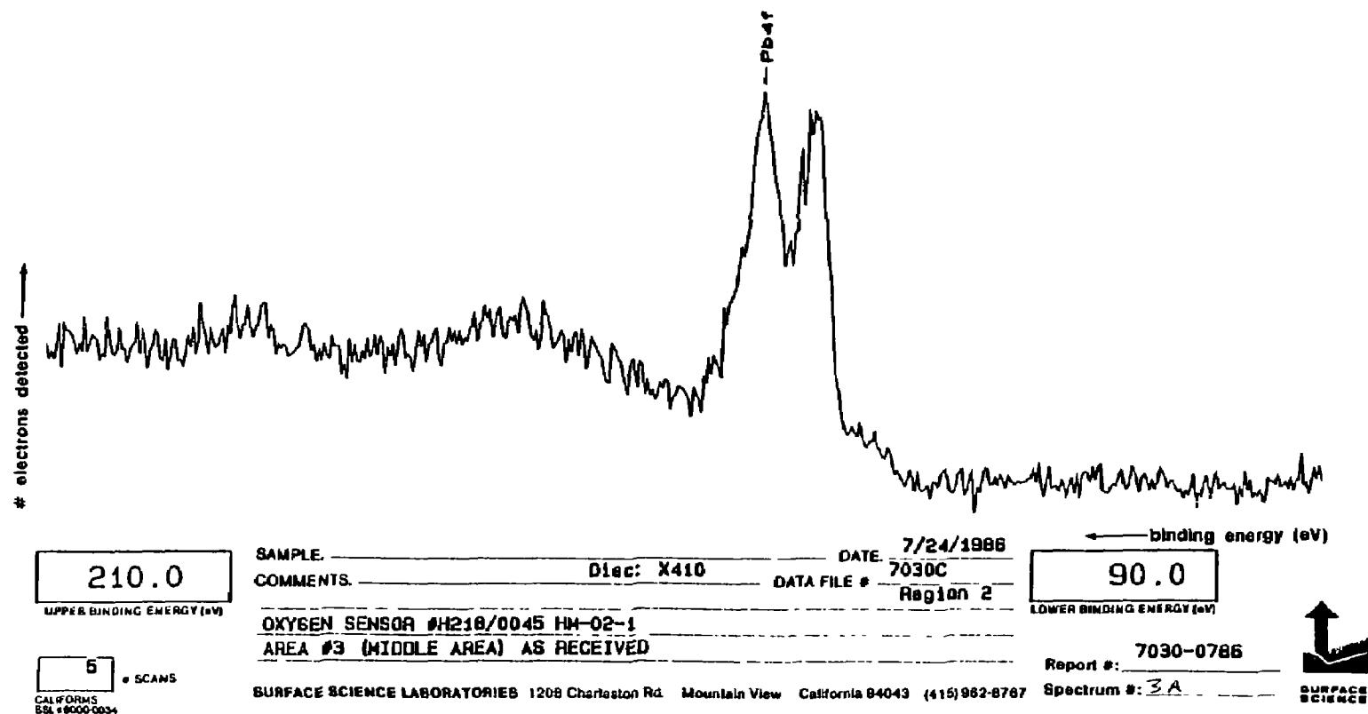
Figure G-22. ESCA Spectrum of Oxygen Sensor A218/0045 from 90 eV to 210 eV (Exterior Surface)
