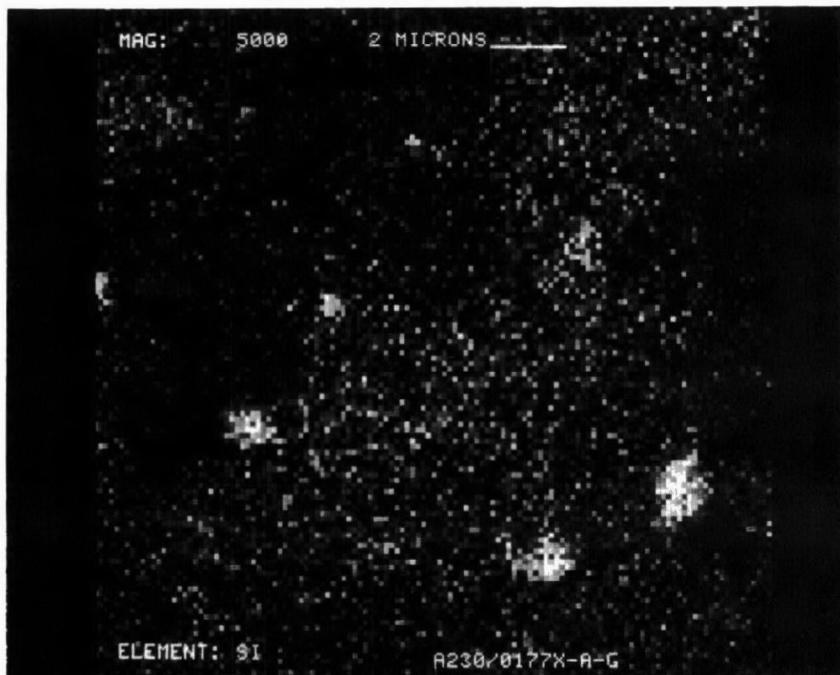
Figure D-276. Silicon Dot Map at X5000 of Converter A230/0177X-Rear Face
