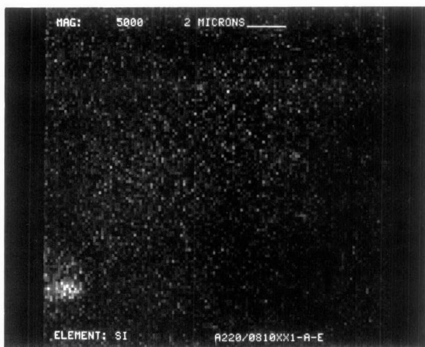
Figure D-66. Silicon Dot Map at X5000 of Converter A220/0810
