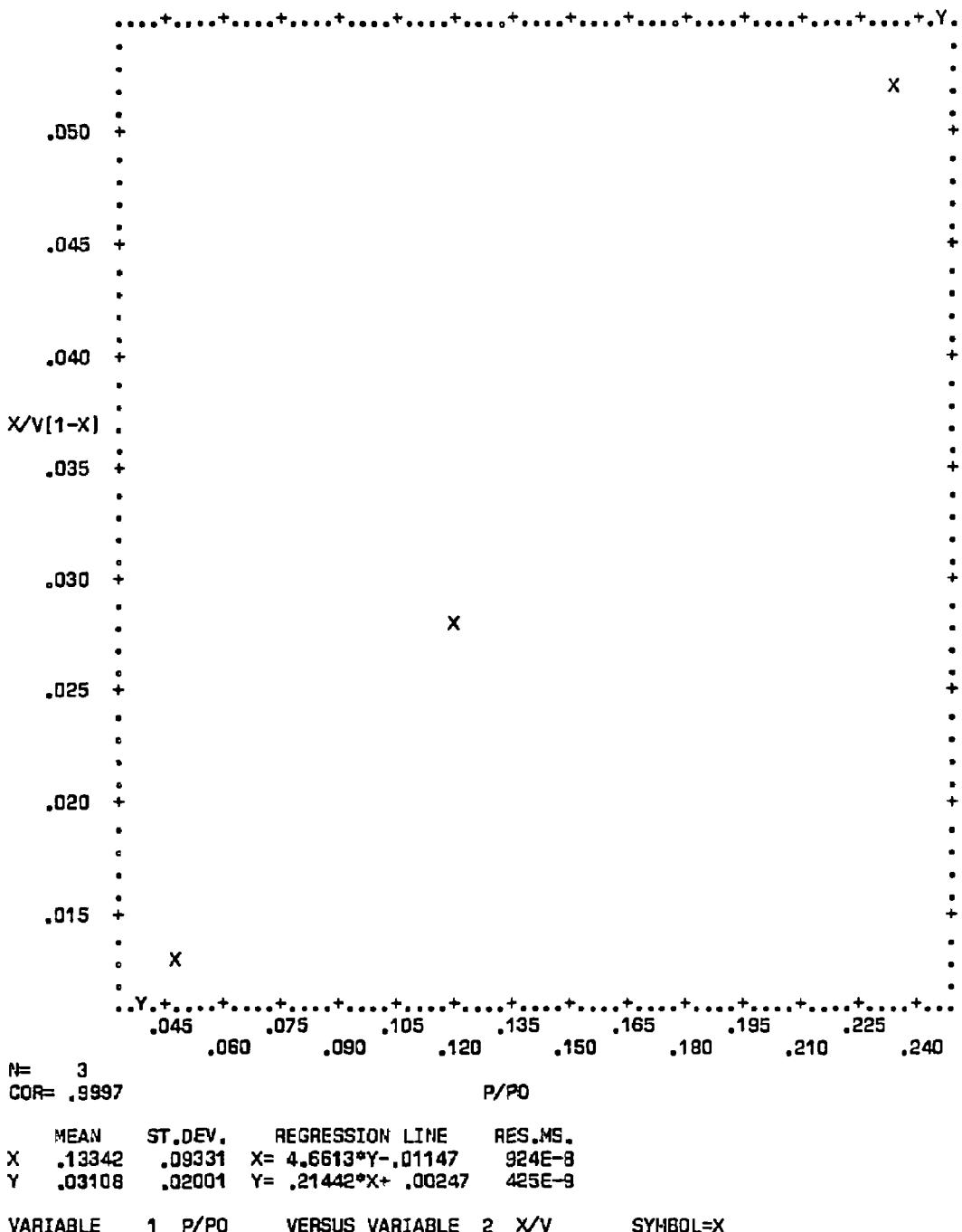
**Figure C-68.** Plot of BET equation versus relative pressure for Converter A240/0153-A - Bulk
