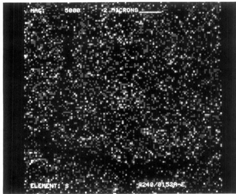
Figure D-158. Sulfur Dot Map at X5000 of Converter A240/0153
