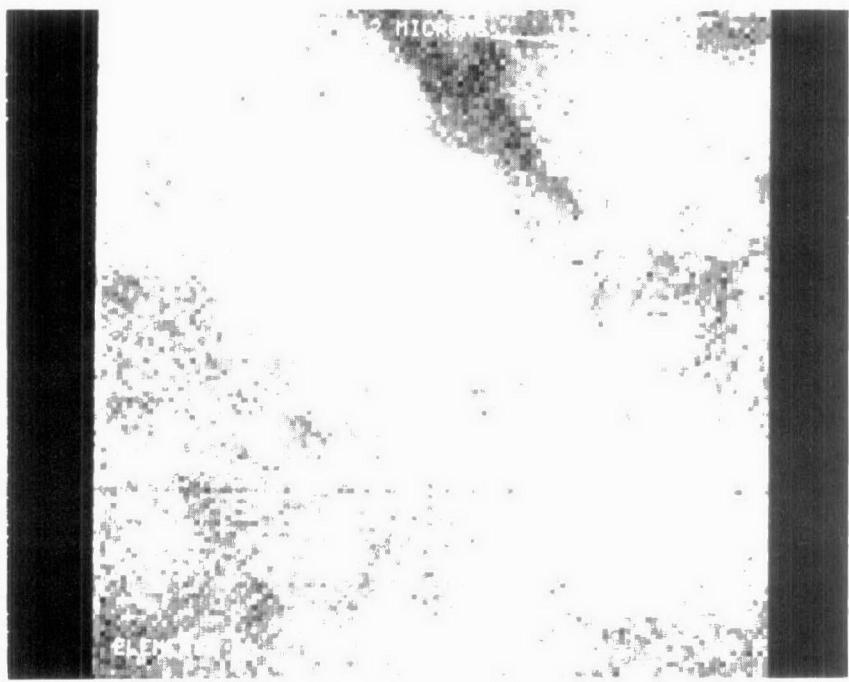
Figure D-265. Aluminum Dot Map at X5000 of Converter A221/0447-Rear Face
