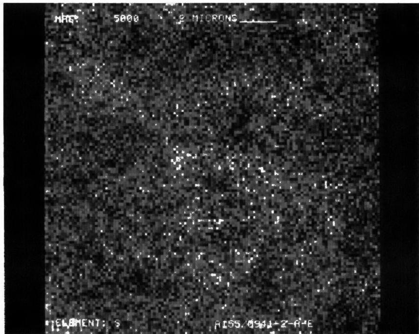
Figure D-228. Sulfur Dot Map at X5000 of Converter A155/0941-2
