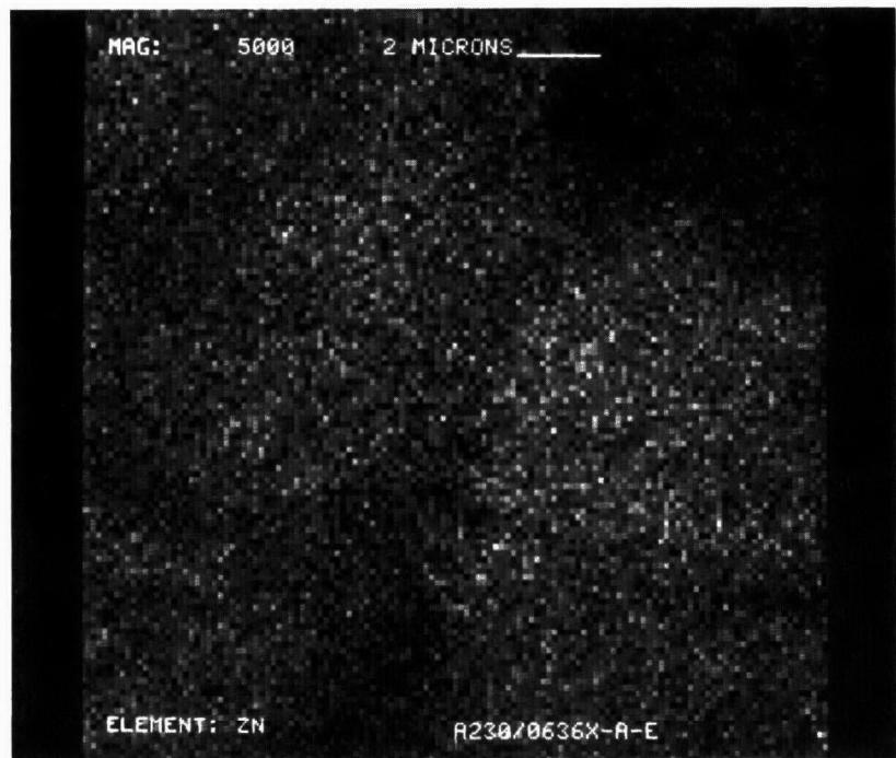
Figure D-119. Zinc Dot Map at X5000 of Converter A230/0636X
