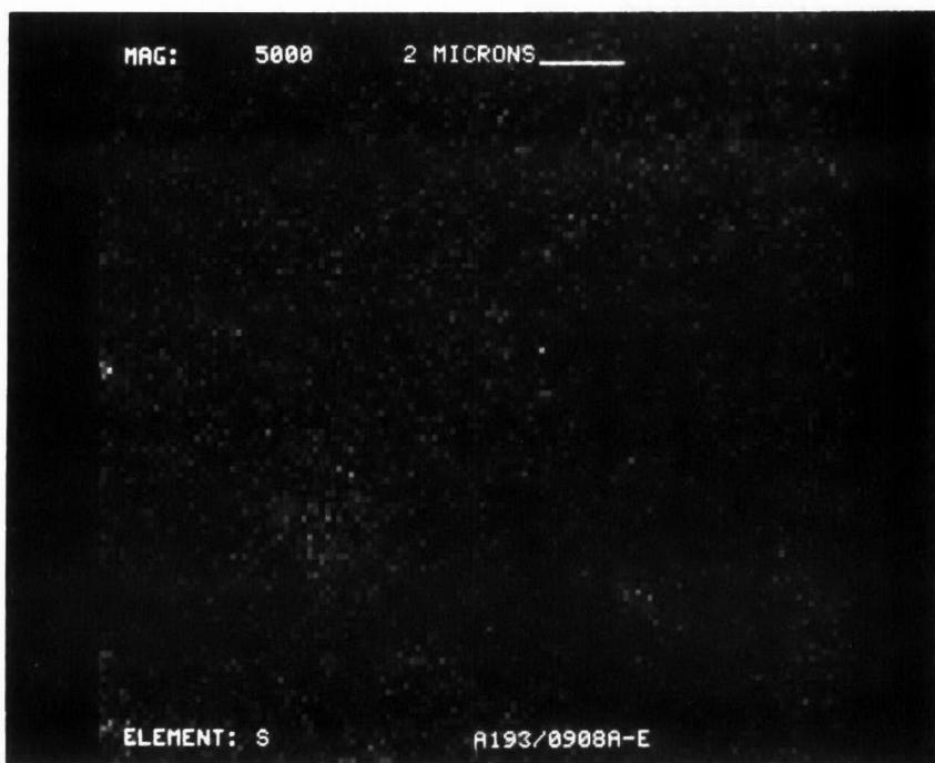
Figure D-18. Sulfur Dot Map at X5000 of Converter A193/0908
