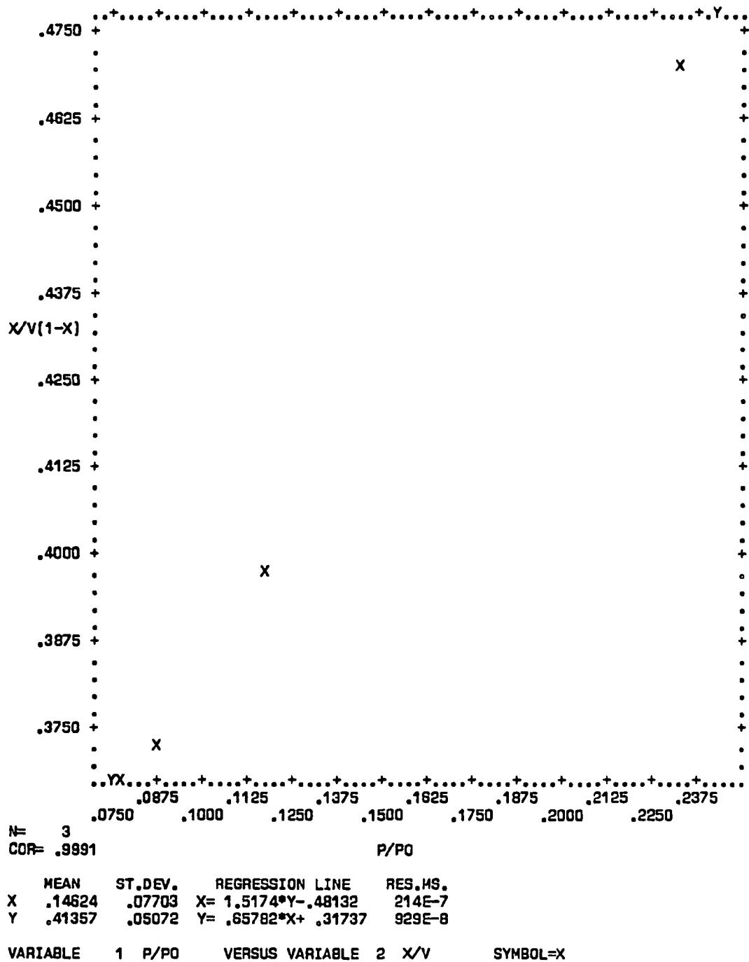
Figure F-10. Plot of BET equation versus relative pressure for Oxygen Sensor A218/0045
