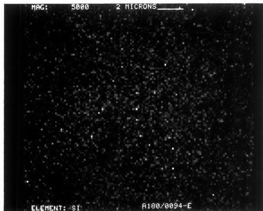
Figure D-6. Silicon Dot Map at X5000 of Converter A180/0094
