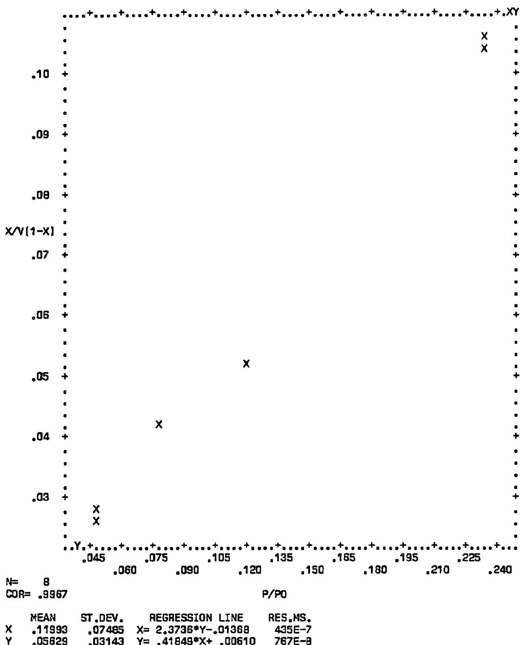
Figure C-80. Plot of BET equation versus relative pressure for Converter A249/0169-1 - Rear Face
