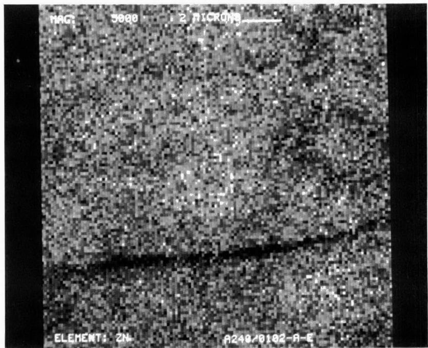
Figure D-139. Zinc Dot Map at X5000 of Converter A240/0102
