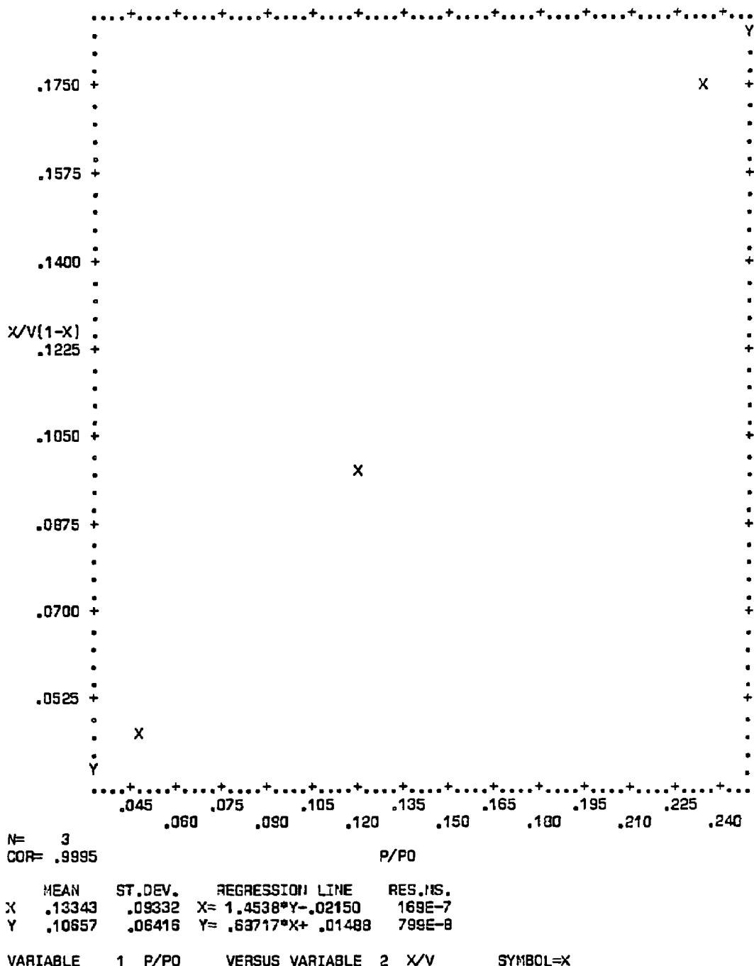
Figure C-104. Plot of BET equation versus relative pressure for Converter A207/0101-A - Bulk
