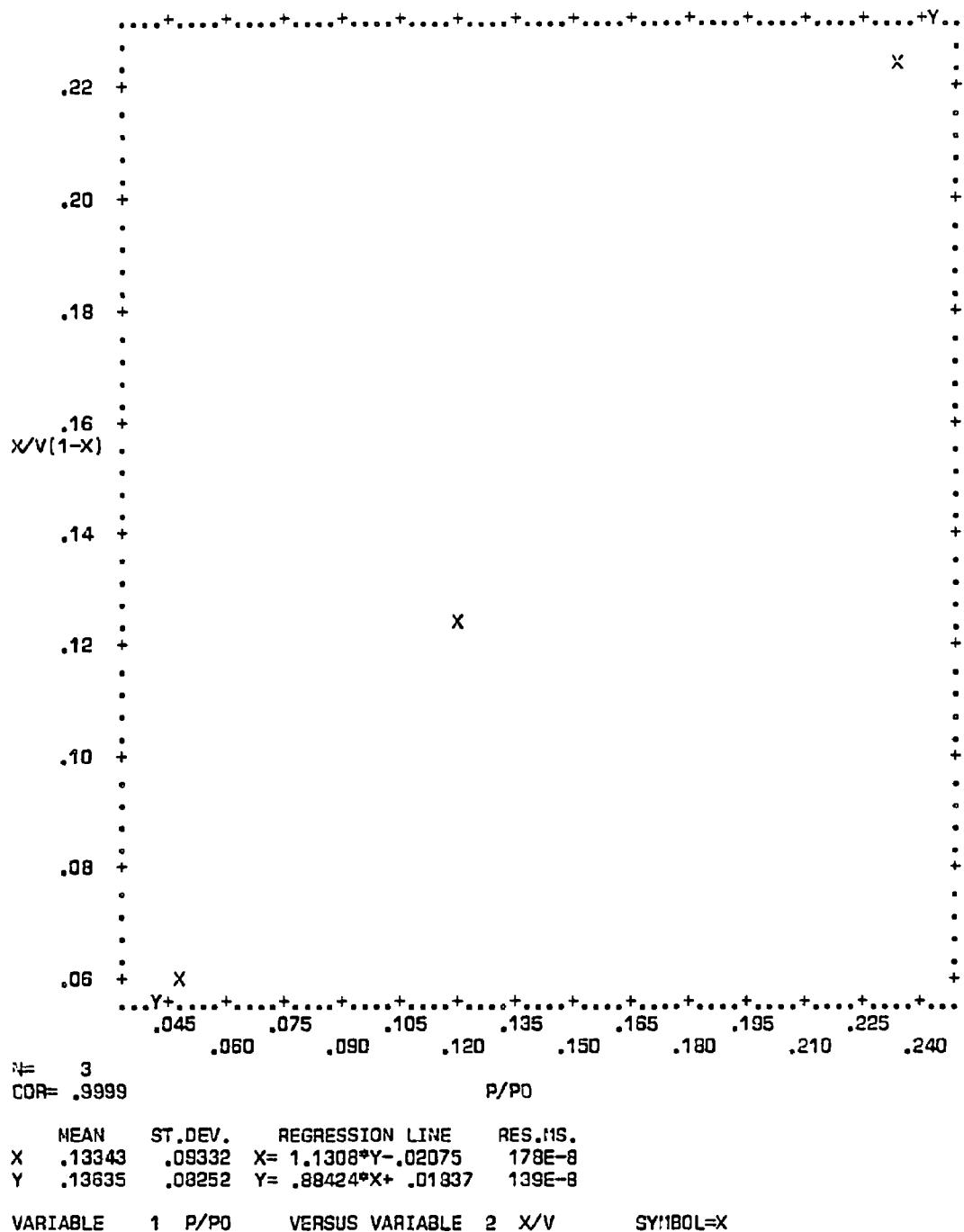
Figure C-84. Plot of BET equation versus relative pressure for Converter A249/0169-3-A - Bulk
