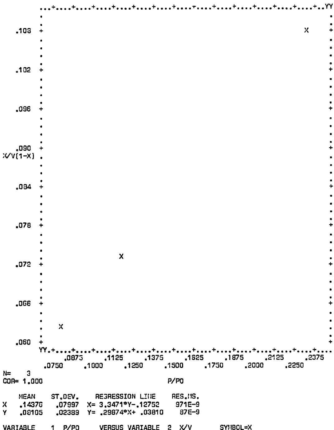
Figure C-40. Plot of BET equation versus relative pressure for Converter A221/0447-A - Rear Face
