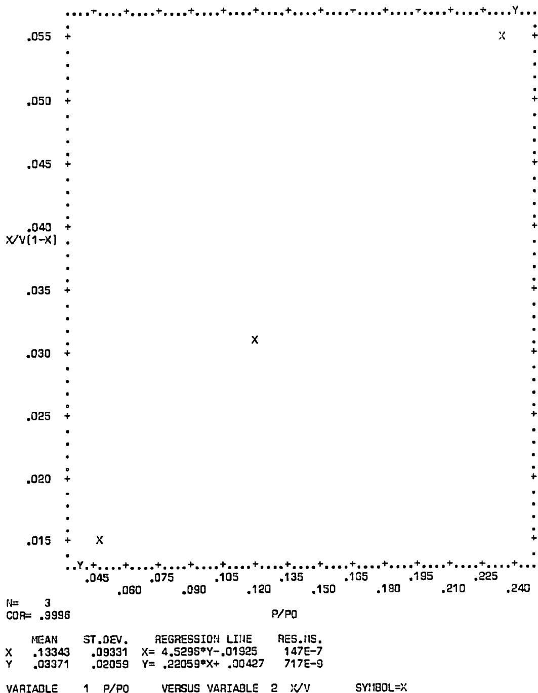
Figure C-75. Plot of BET equation versus relative pressure for Converter A240/0334L-A - Rear Face
