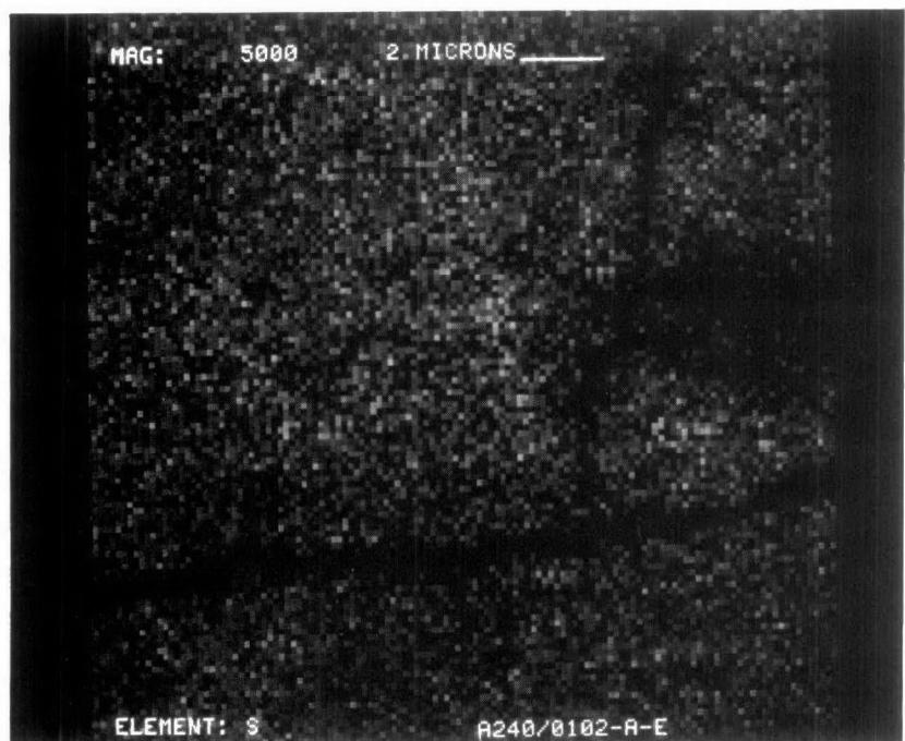
Figure D-138. Sulfur Dot Map at X5000 of Converter A240/0102
