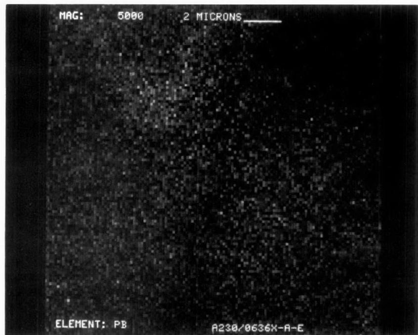
Figure D-117. Lead Dot Map at X5000 of Converter A230/0636X
