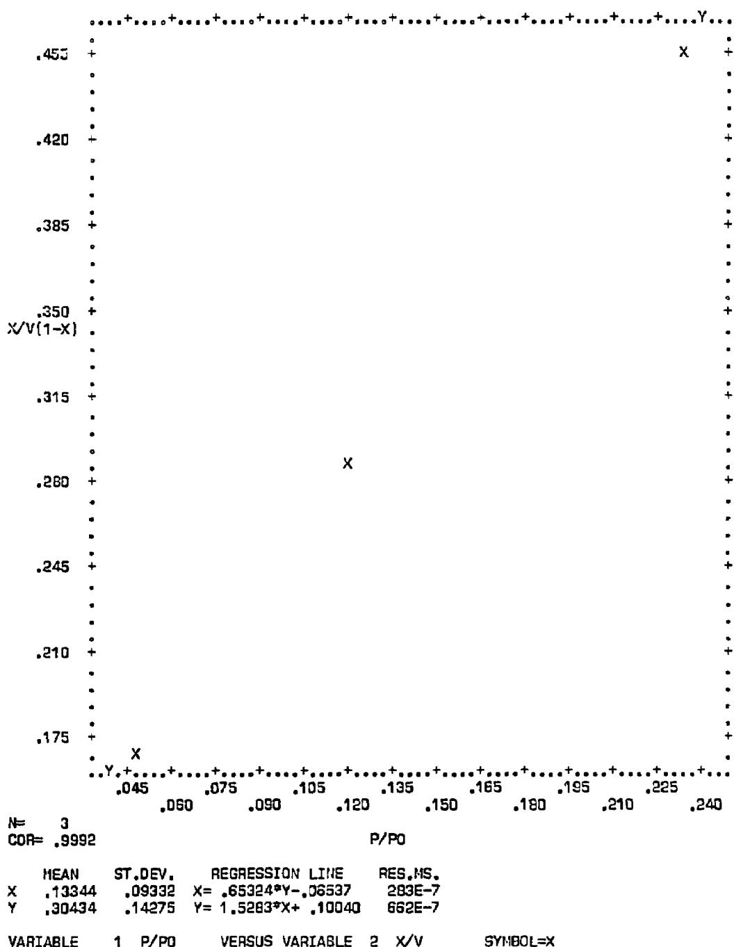
Figure C-4. Plot of BET equation versus relative pressure for Converter A193/0908-A - Bulk
