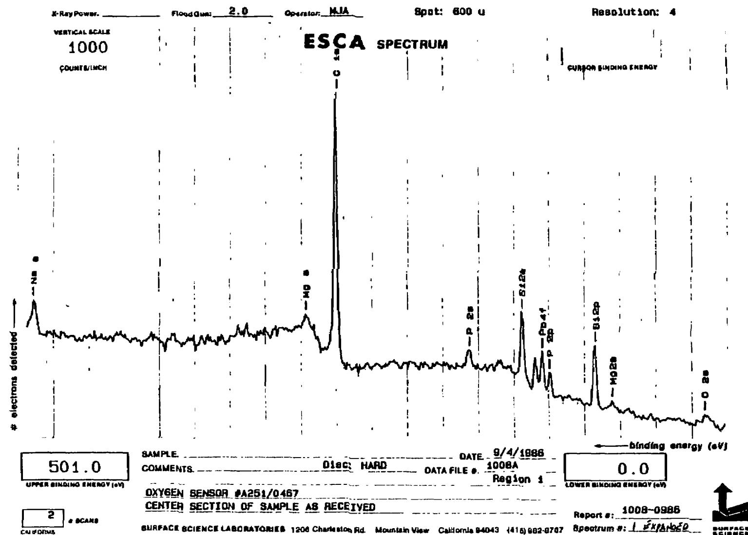
Figure G-16. ESCA Spectrum of Oxygen Sensor A251/0467 from 0 eV to 501 eV (Exterior Surface)
