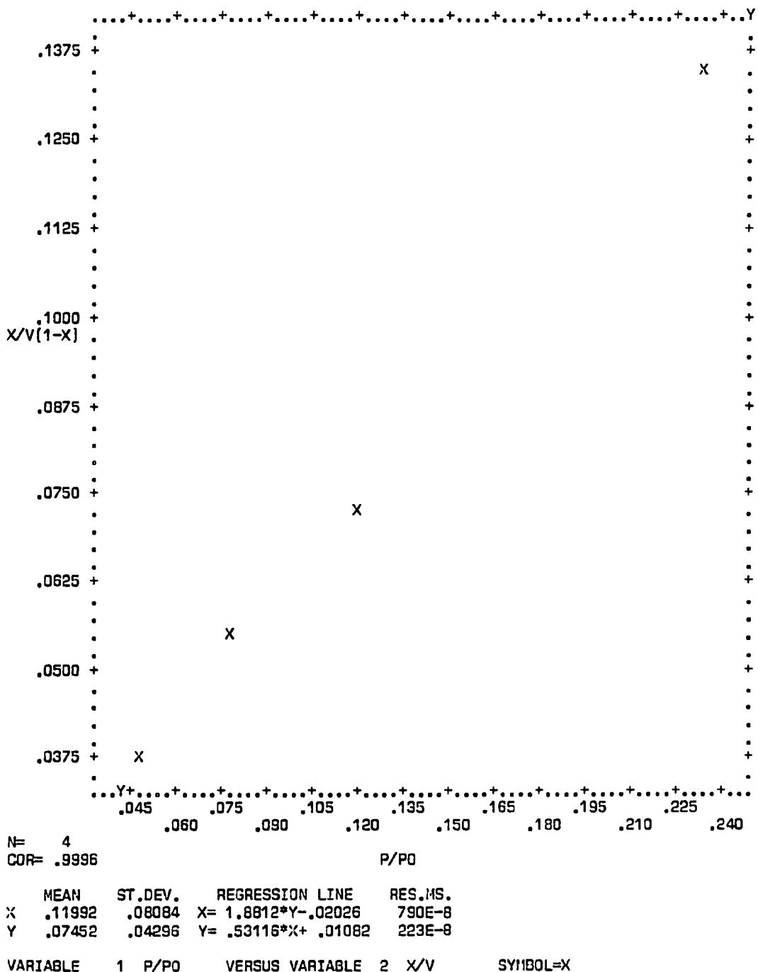
Figure C-41. Plot of BET equation versus relative pressure for Converter A221/0447-B - Bulk
