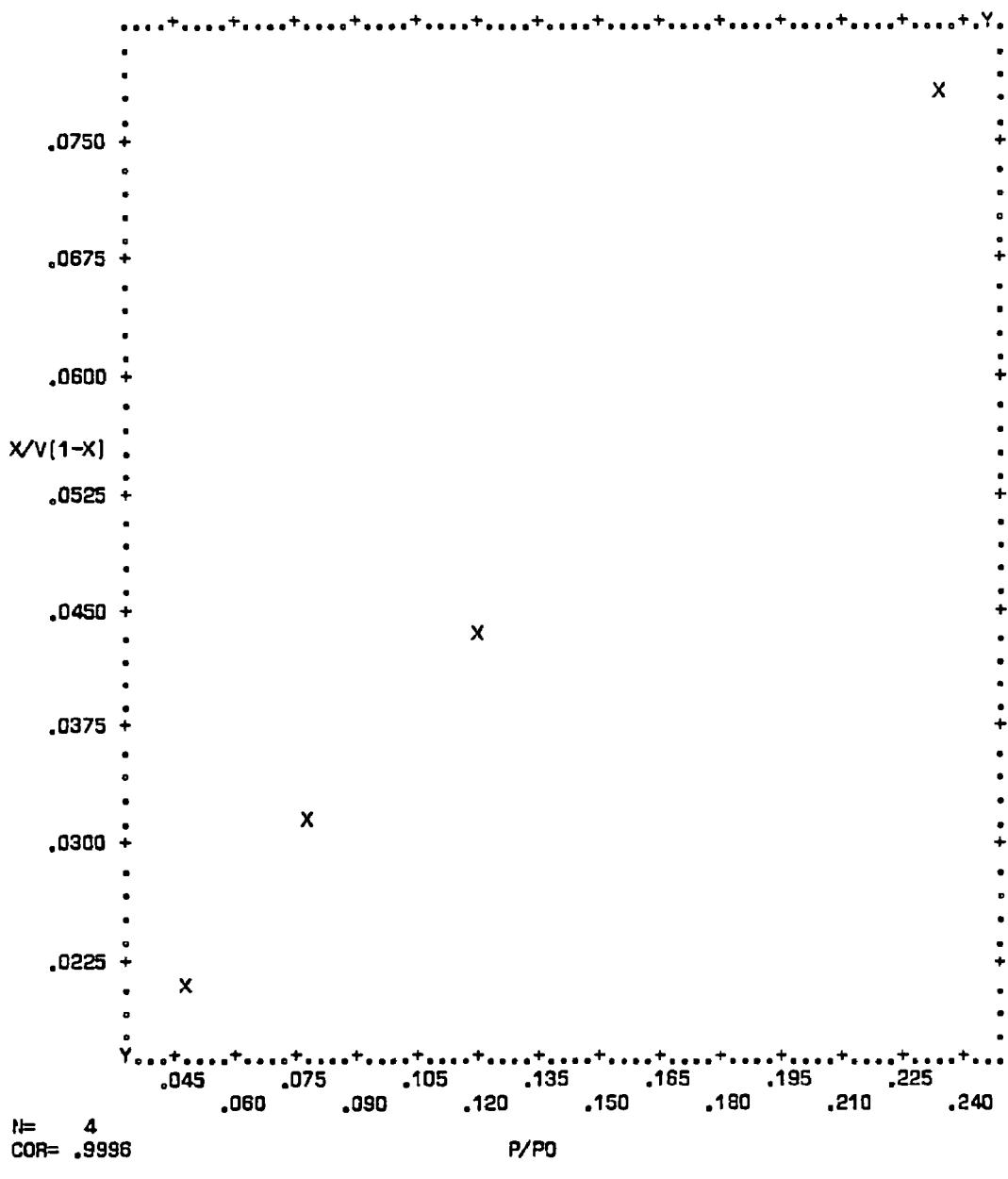
**Figure C-52. Plot of BET equation versus relative pressure for Converter A230/0636X-B - Front Face**
