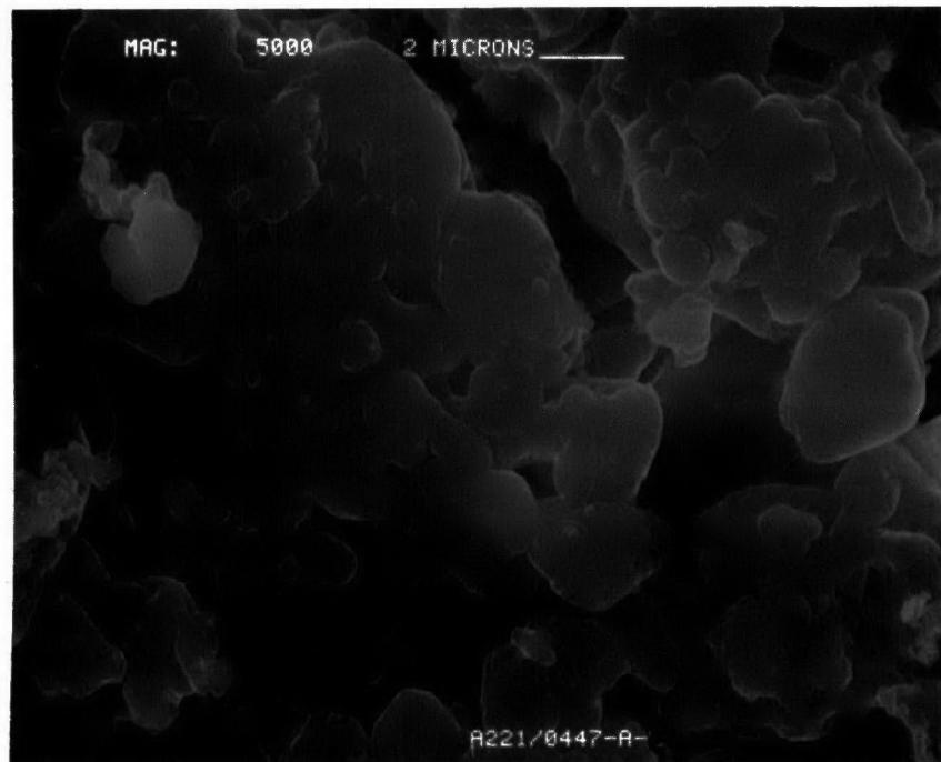
**Figure D-264.** Scanning Electron Micrograph at X5000 of Converter A221/0447-Rear Face
