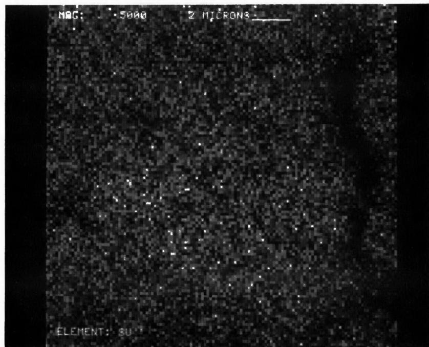
Figure D-48. Sulfur Dot Map at X5000 of Converter A218/0068
