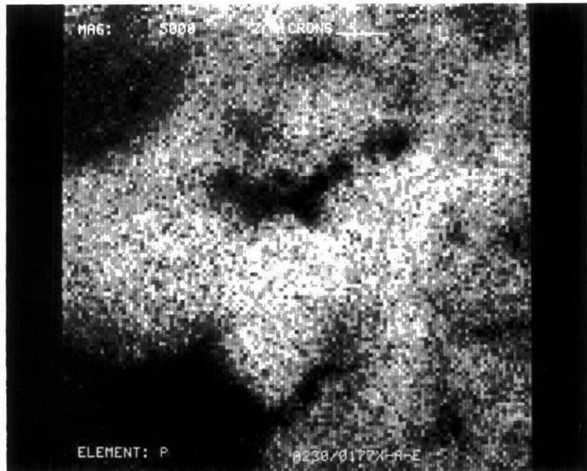
Figure D-110. Phosphorus Dot Map at X5000 of Converter A230/0177X
