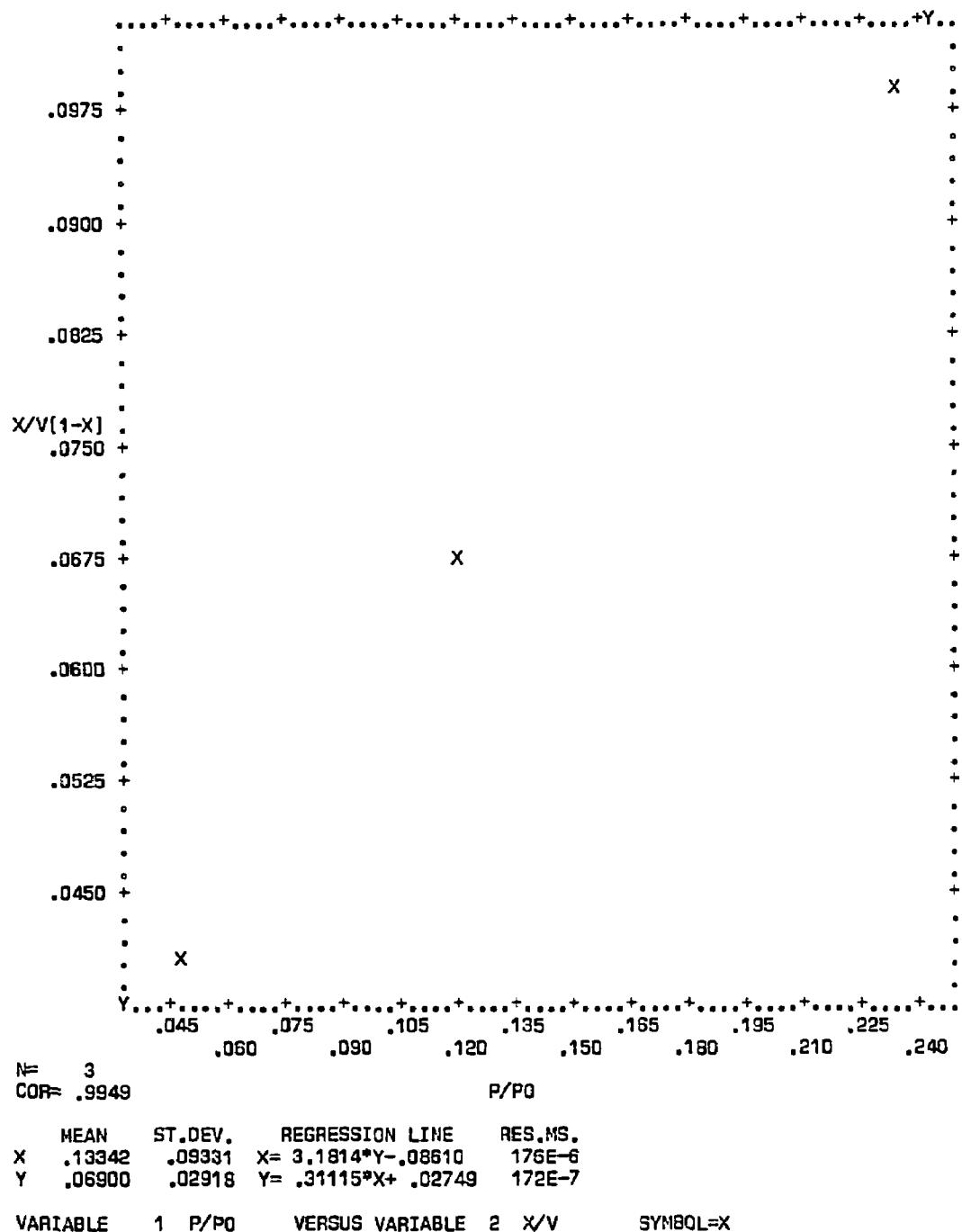
Figure C-62. Plot of BET equation versus relative pressure for Converter A240/0102-B - Front Face
