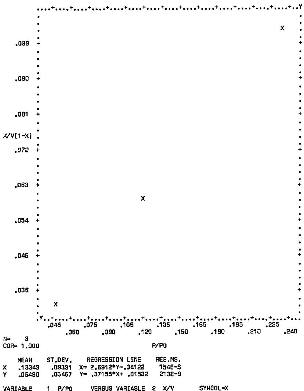
Figure C-25. Plot of BET equation versus relative pressure for Converter A220/0810-A - Rear Face
