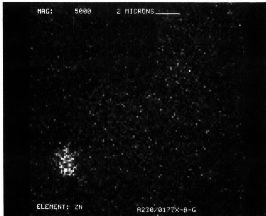
Figure D-279. Zinc Dot Map at X5000 of Converter A230/0177X-Rear Face
