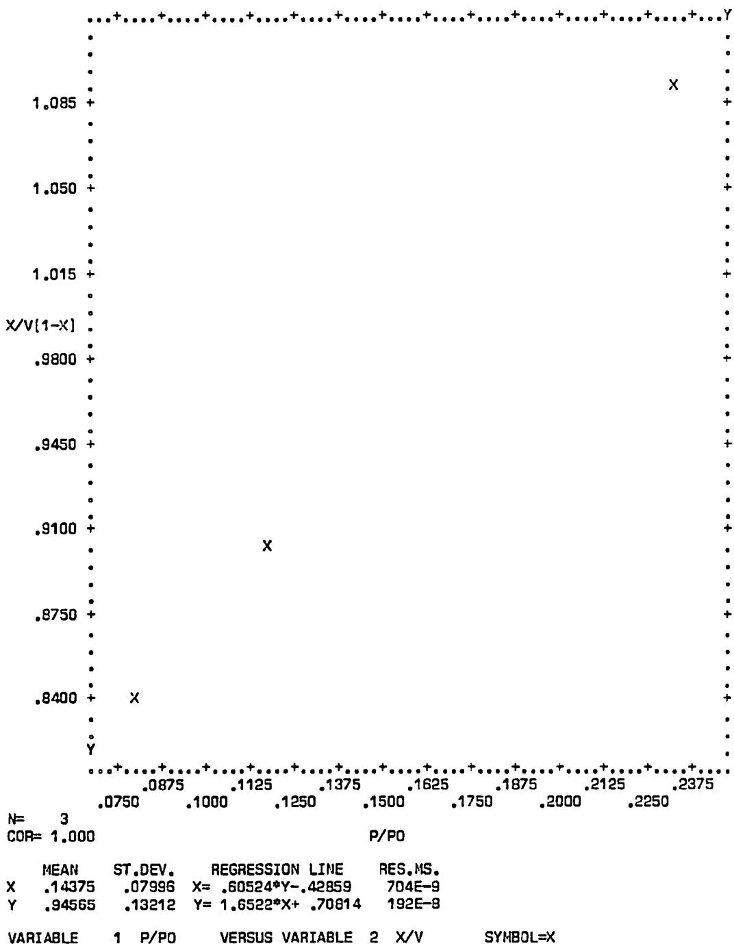
**Figure F-4.** Plot of BET equation versus relative pressure
