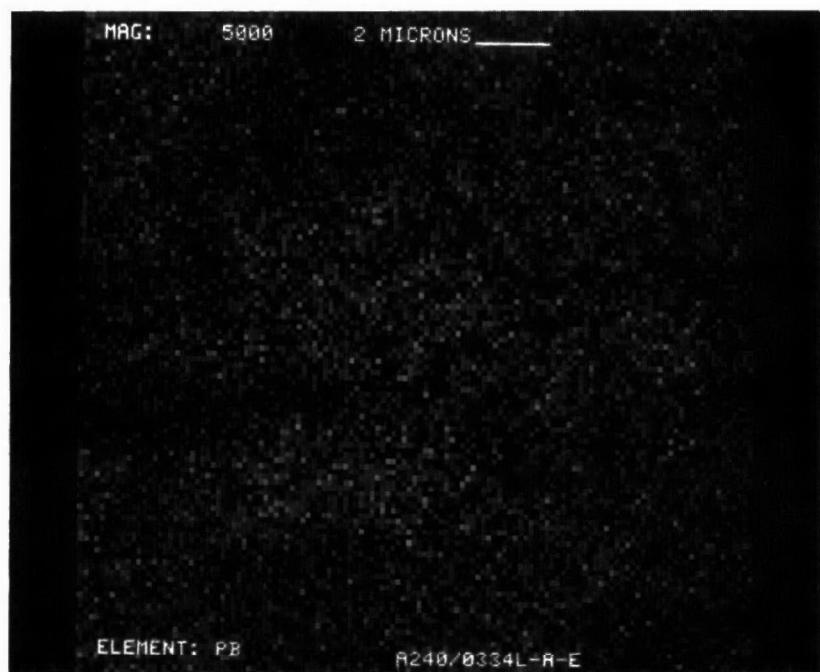
Figure D-167. Lead Dot Map at X5000 of Converter A240/0334L
