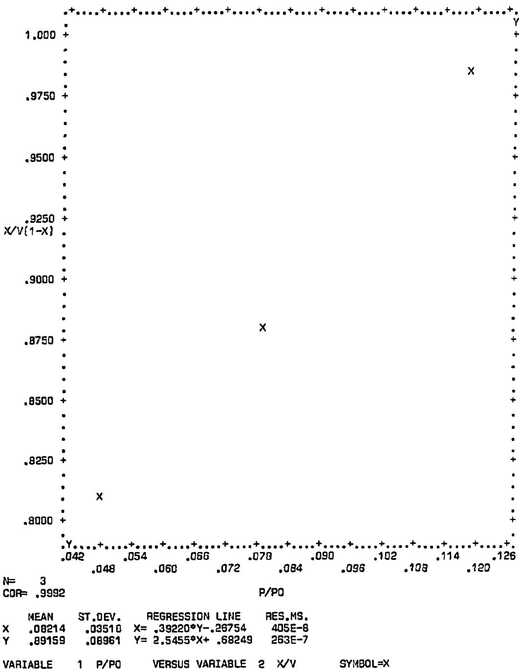
**Figure F-3.** Plot of BET equation versus relative pressure for Oxygen Sensor A221/0146
