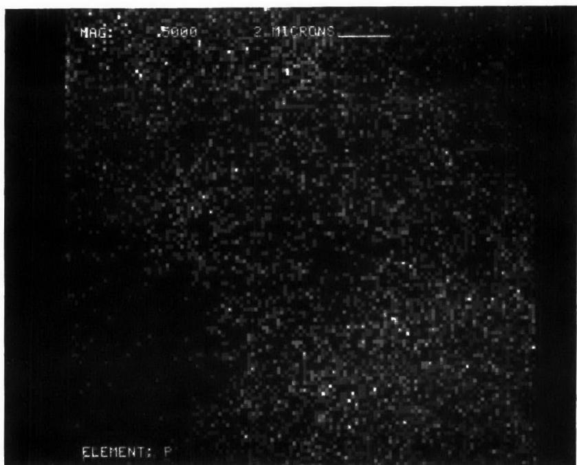
Figure D-190. Phosphorus Dot Map at X5000 of Converter A249/0169-2
