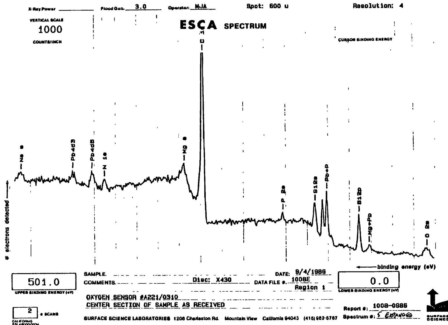
Figure G-8. ESCA Spectrum of Oxygen Sensor A221/0310 from 0 eV to 501 eV (Exterior Surface)
