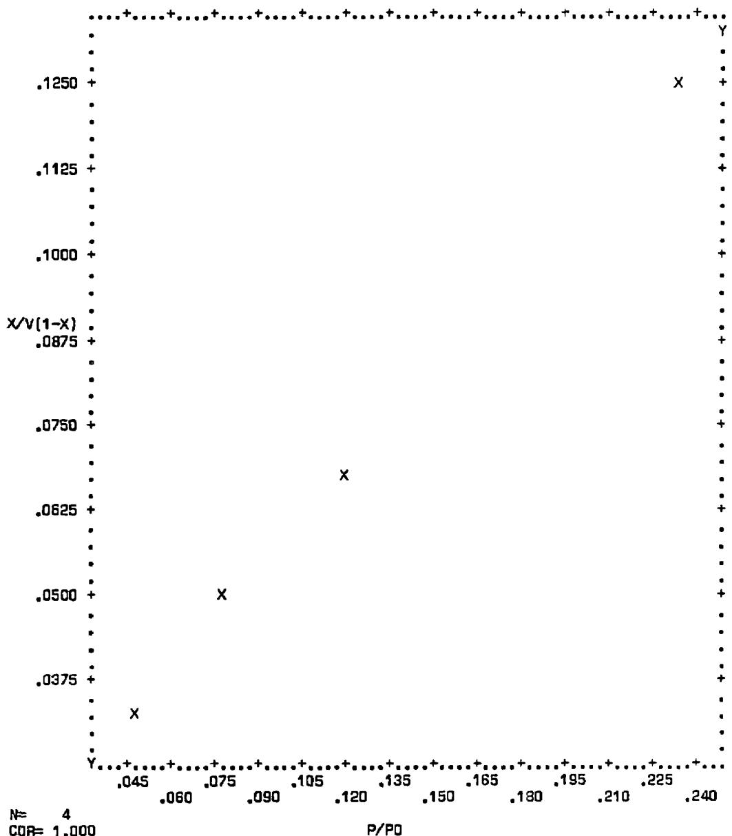
**Figure C-31. Plot of BET equation versus relative pressure for Converter A221/0152-B - Bulk**
