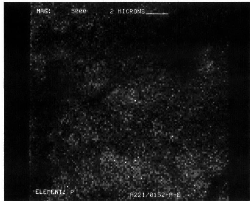
Figure D-80. Phosphorus Dot Map at X5000 of Converter A221/0152
