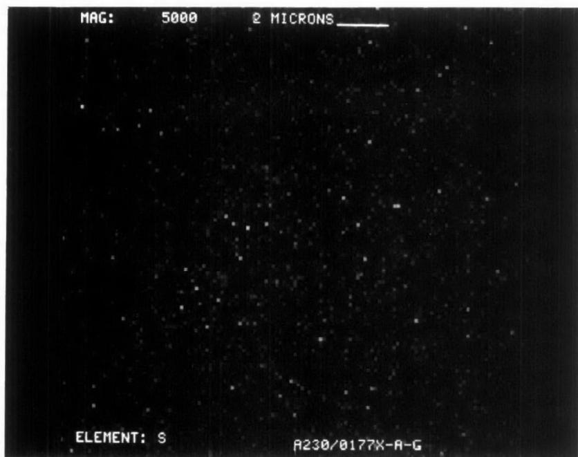
Figure D-278. Sulfur Dot Map at X5000 of Converter A230/0177X-Rear Face
