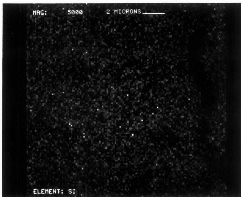
Figure D-46. Silicon Dot Map at X5000 of Converter A218/0068
