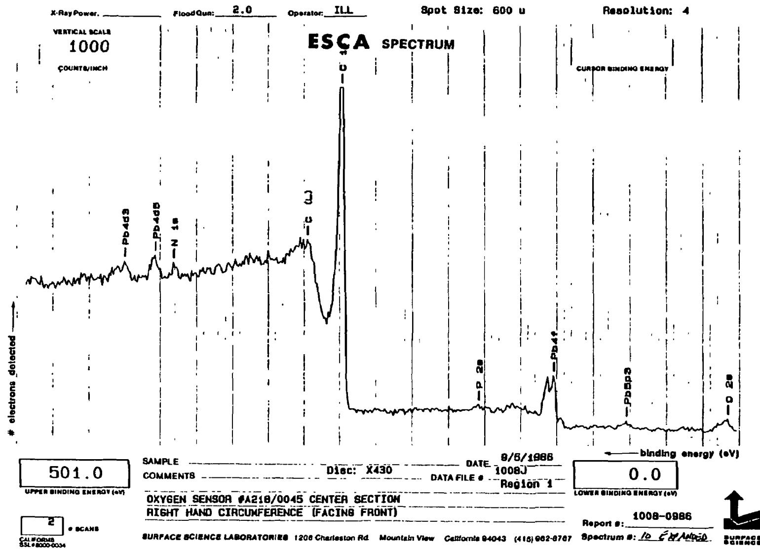
Figure I-13. ESCA Spectrum of Oxygen Sensor A218/0045 from 0 eV to 501 eV (Location 6)
