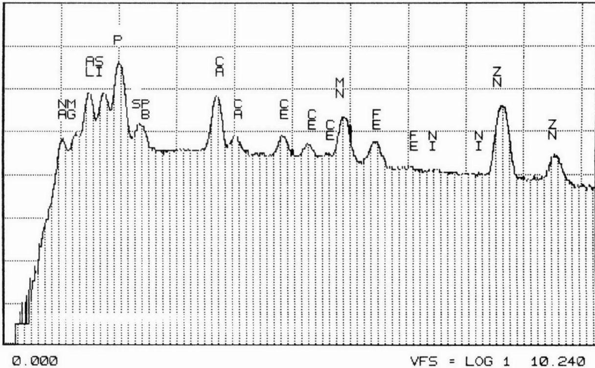
Figure D-211. SEM/EDX Spectrum of Converter A155/0941-1
