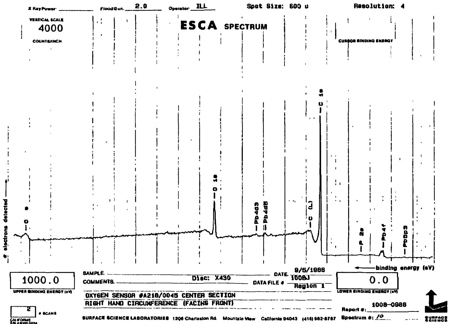
Figure I-12. ESCA Spectrum of Oxygen Sensor A218/0045 from 0 eV to 1000 eV (Location 6)
