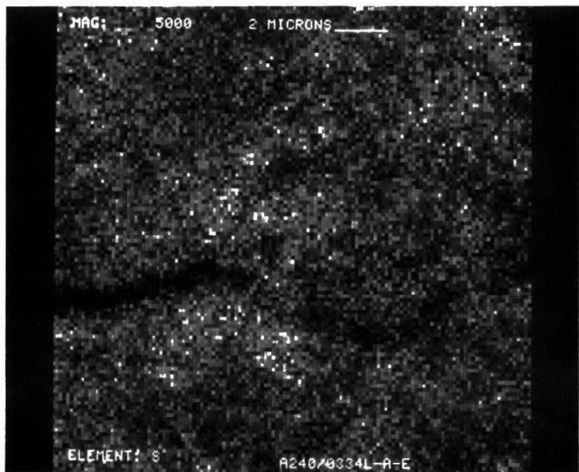
Figure D-168. Sulfur Dot Map at X5000 of Converter A240/0334L
