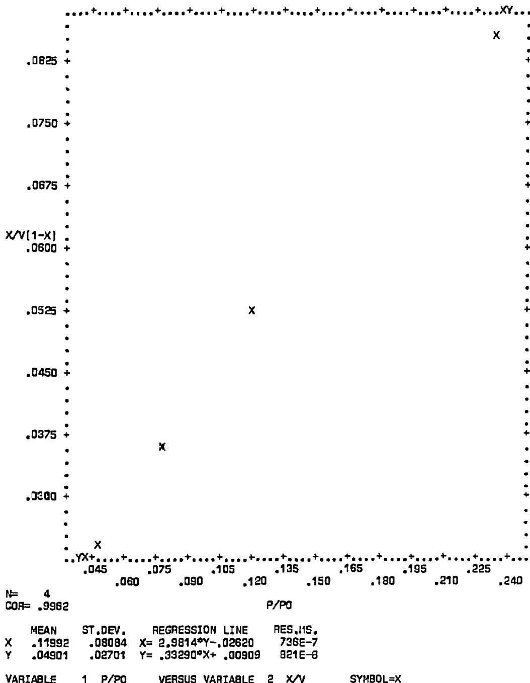
Figure C-49. Plot of BET equation versus relative pressure for Converter A230/0636X-A - Front Face
