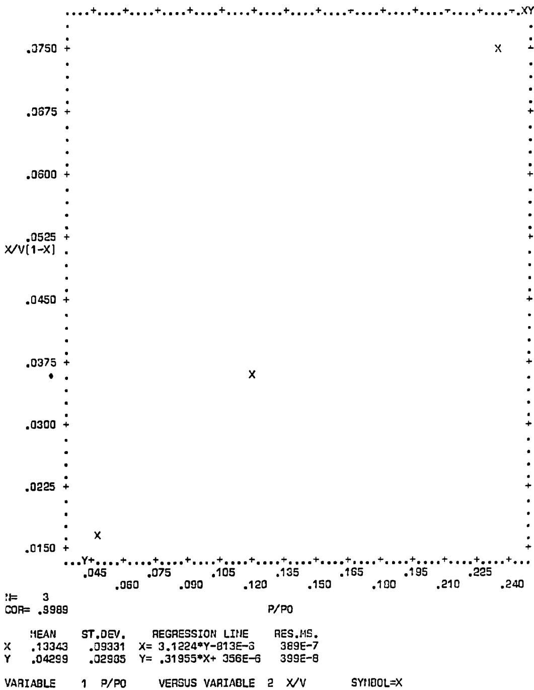
Figure C-71. Plot of BET equation versus relative pressure for Converter A240/0153-B - Bulk
