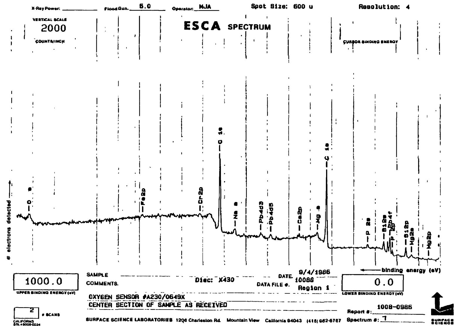
Figure G-11. ESCA Spectrum of Oxygen Sensor A230/0649X from 0 eV to 1000 eV (Exterior Surface)
