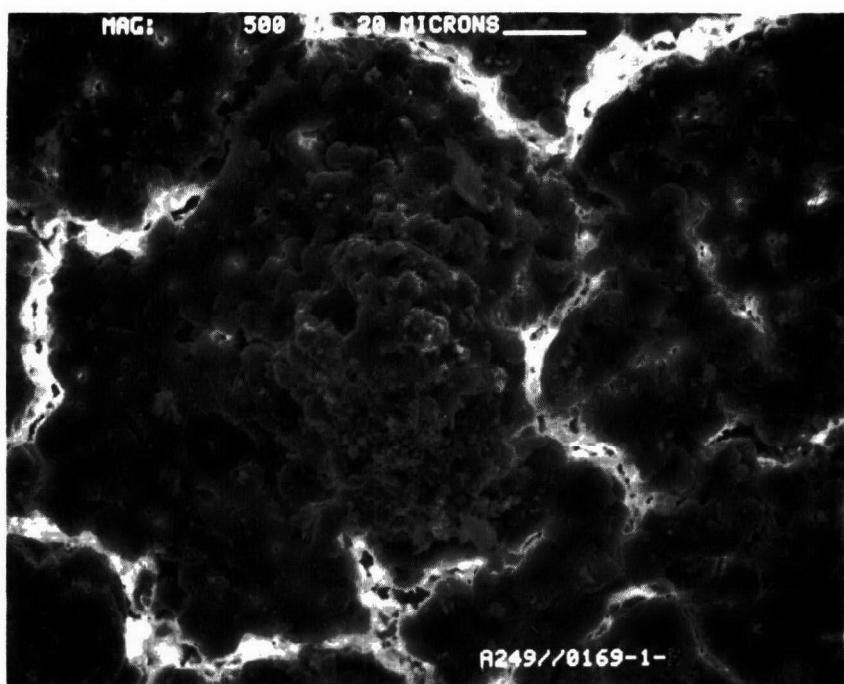
Figure D-282. Scanning Electron Micrograph at X500 of Converter A249/0169-1-Rear Face
