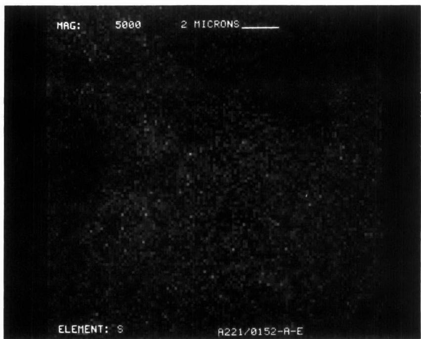
Figure D-78. Sulfur Dot Map at X5000 of Converter A221/0152
