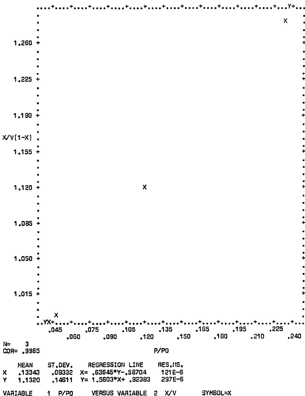
**Figure F-1.** Plot of BET equation versus relative pressure for Oxygen Sensor A220/0660
