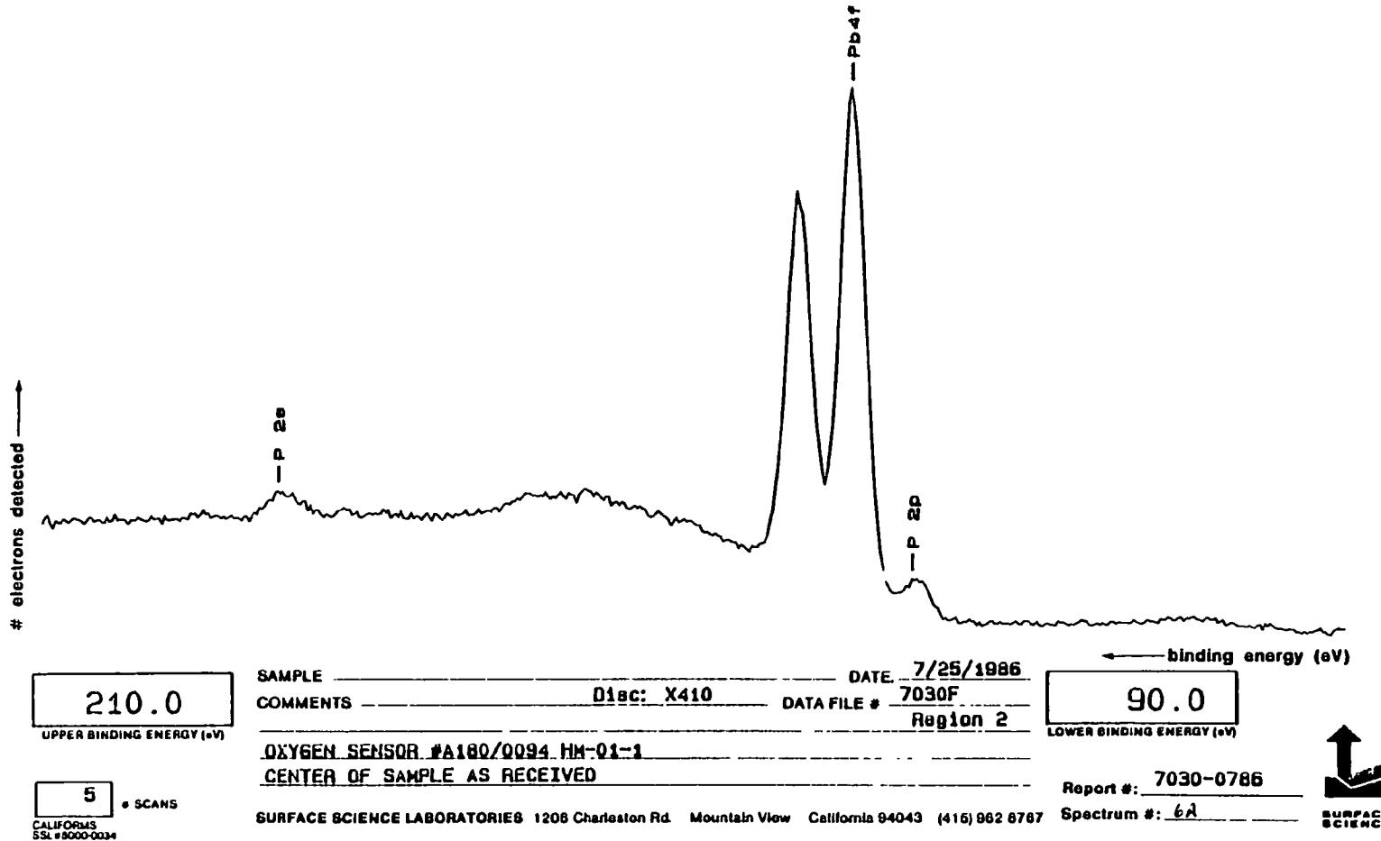
Figure G-19. ESCA Spectrum of Oxygen Sensor A180/0094 from 90 eV to 210 eV (Exterior Surface)
