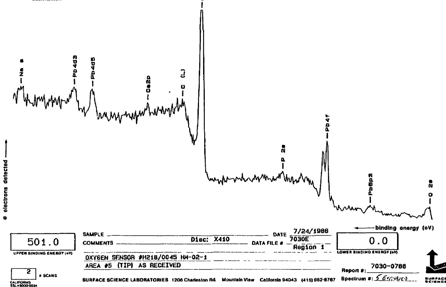
Figure I-11. ESCA Spectrum of Oxygen Sensor A218/0045 from 0 eV to 501 eV (Location 5)
