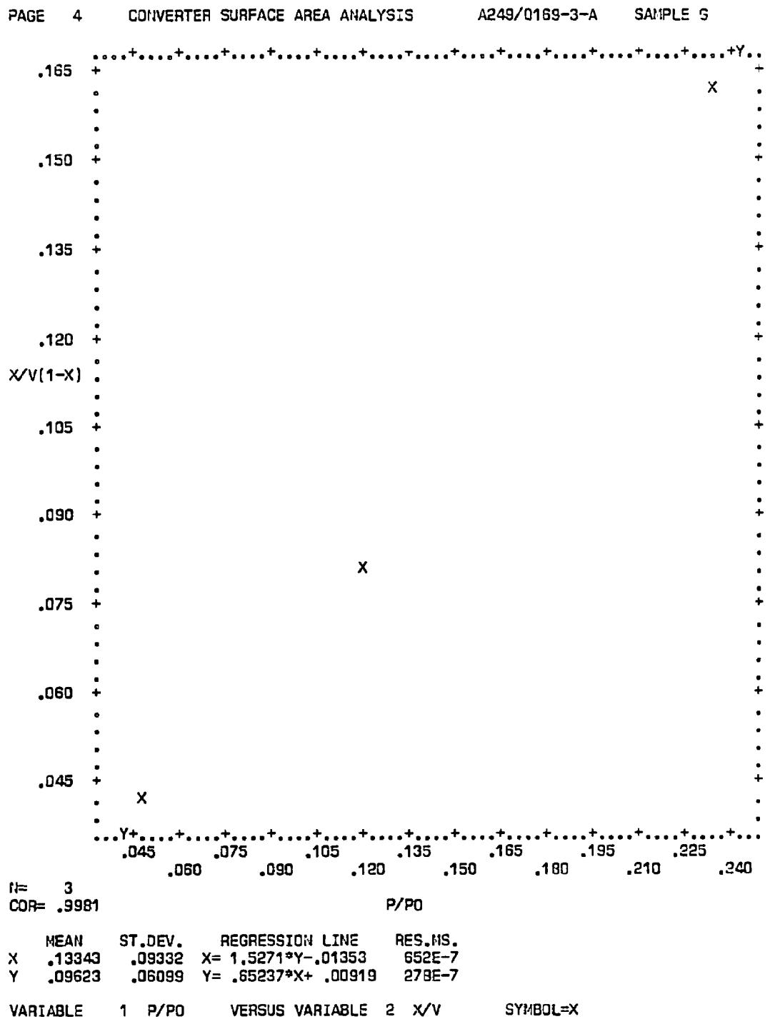
Figure C-86. Plot of BET equation versus relative pressure for Converter A249/0169-3-A - Rear Face
