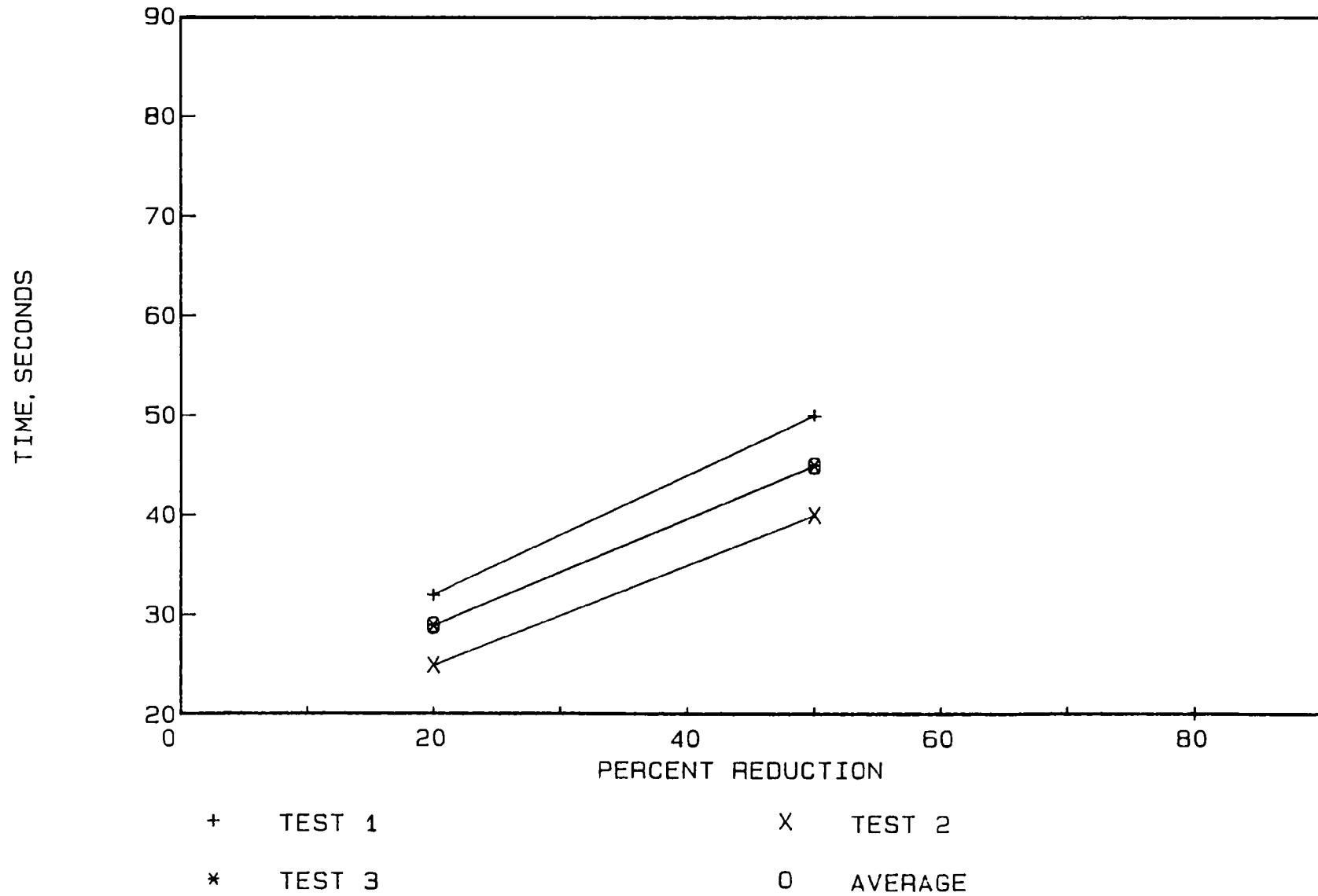
Figure 6. Percent reduction of NO<sub>x</sub> from the light-off test for Converter EPA 1174R
