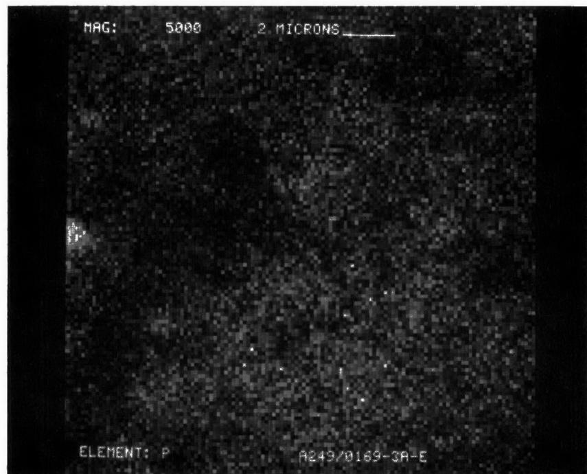
Figure D-200. Phosphorus Dot Map at X5000 of Converter A249/0169-3
