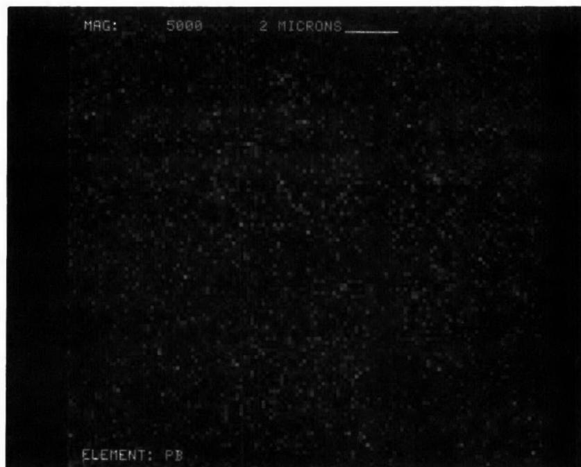
Figure D-27. Lead Dot Map at X5000 of Converter A218/0045
