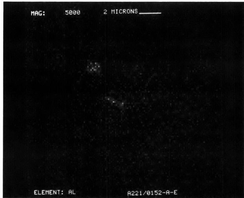
Figure D-75. Aluminum Dot Map at X5000 of Converter A221/0152
