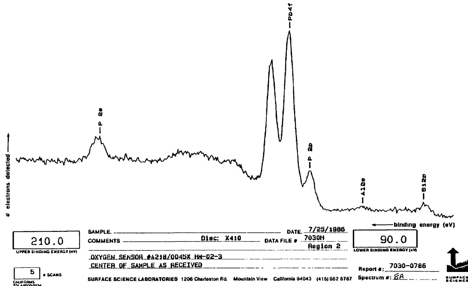
Figure G-25. ESCA Spectrum of Oxygen Sensor A218/0045X from 90 eV to 210 eV (Exterior Surface)
