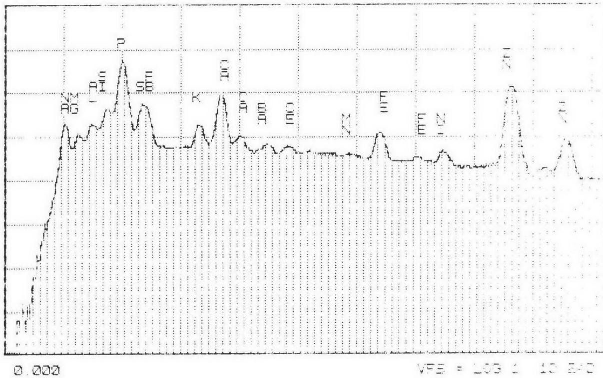
Figure D-61. SEM/EDX Spectrum of Converter A220/0810
