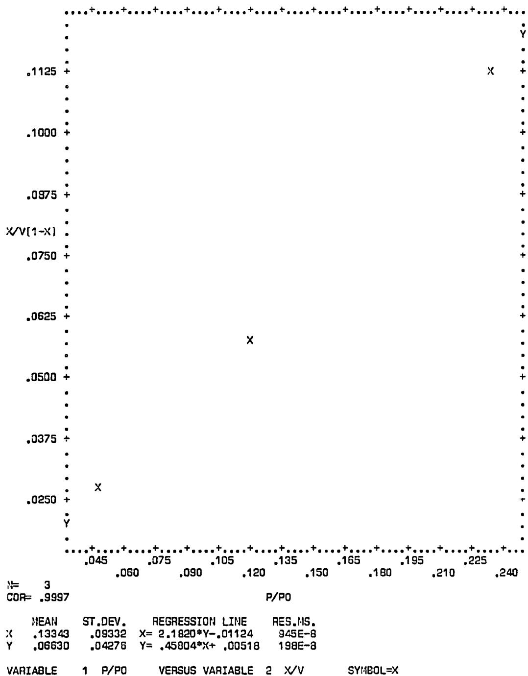
**Figure C-26. Plot of BET equation versus relative pressure for Converter A220/0810-B - Bulk**
