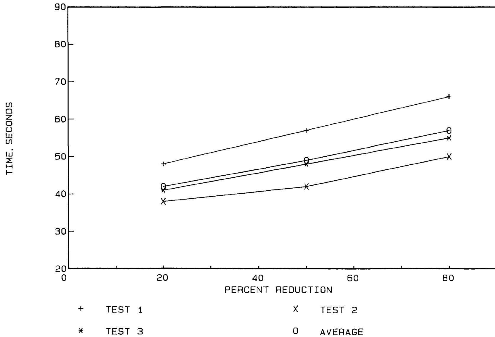
Figure 5. Percent reduction of CO from the light-off test for Converter EPA 1174R
