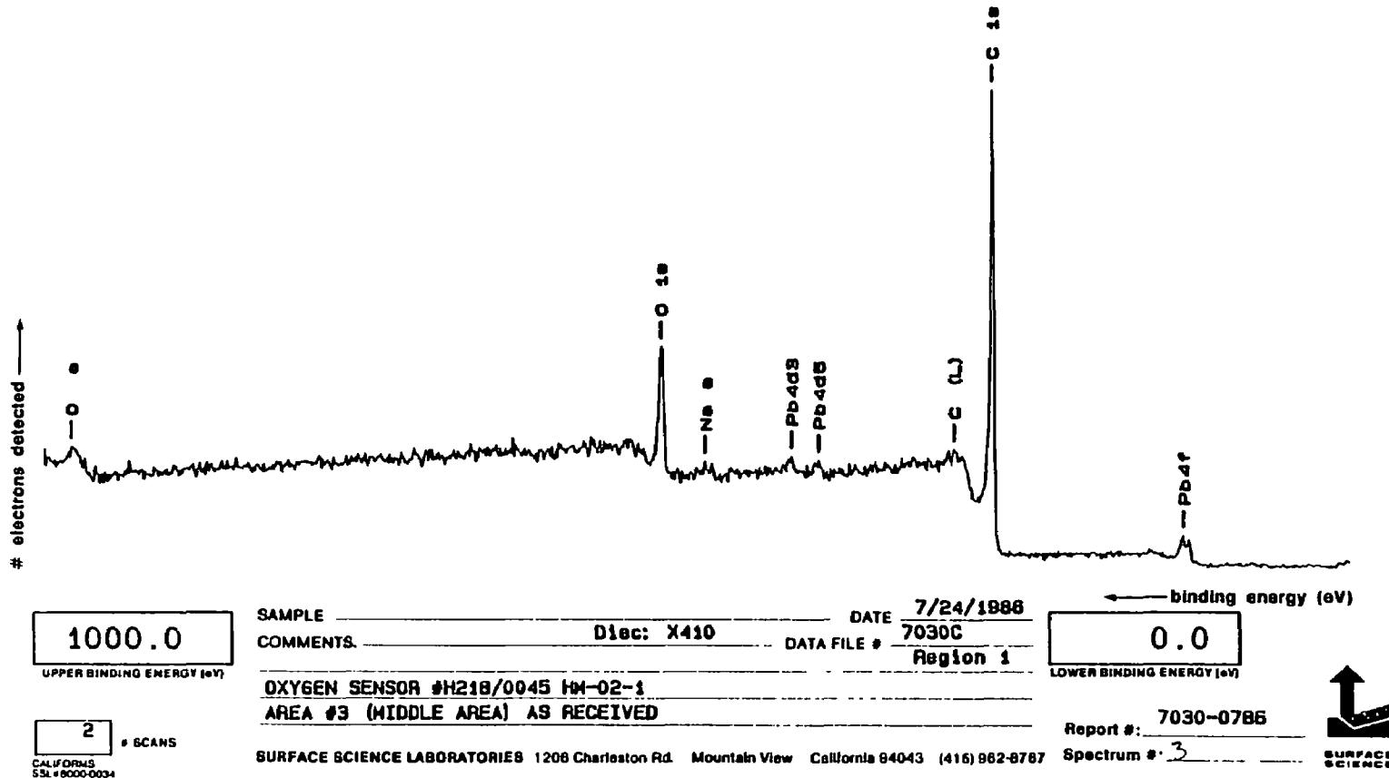
Figure I-5. ESCA Spectrum of Oxygen Sensor A218/0045 from 0 eV to 1000 eV (Location 3)
