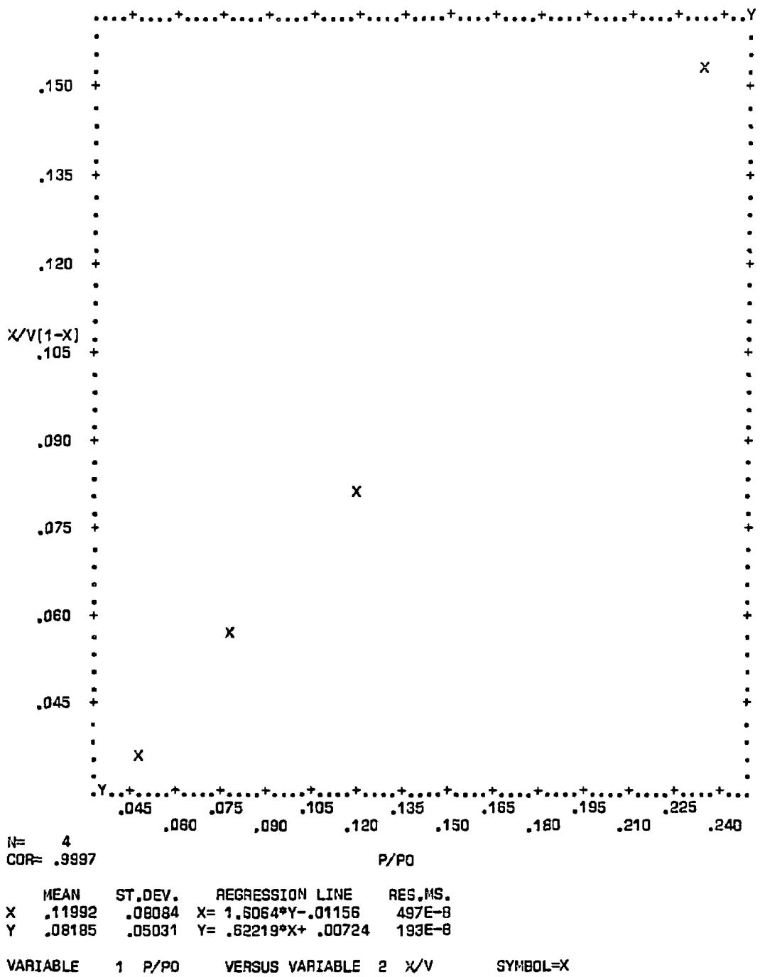
Figure C-97. Plot of BET equation versus relative pressure for Converter A155/0941-1-B - Bulk
