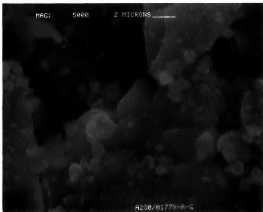
Figure D-274. Scanning Electron Micrograph at X5000 of Converter A230/0177X-Rear Face
