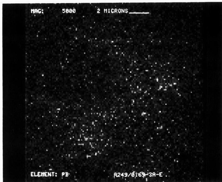
Figure D-197. Lead Dot Map at X5000 of Converter A249/0169-3
