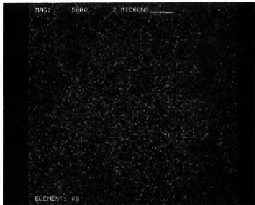
Figure D-47. Lead Dot Map at X5000 of Converter A218/0068
