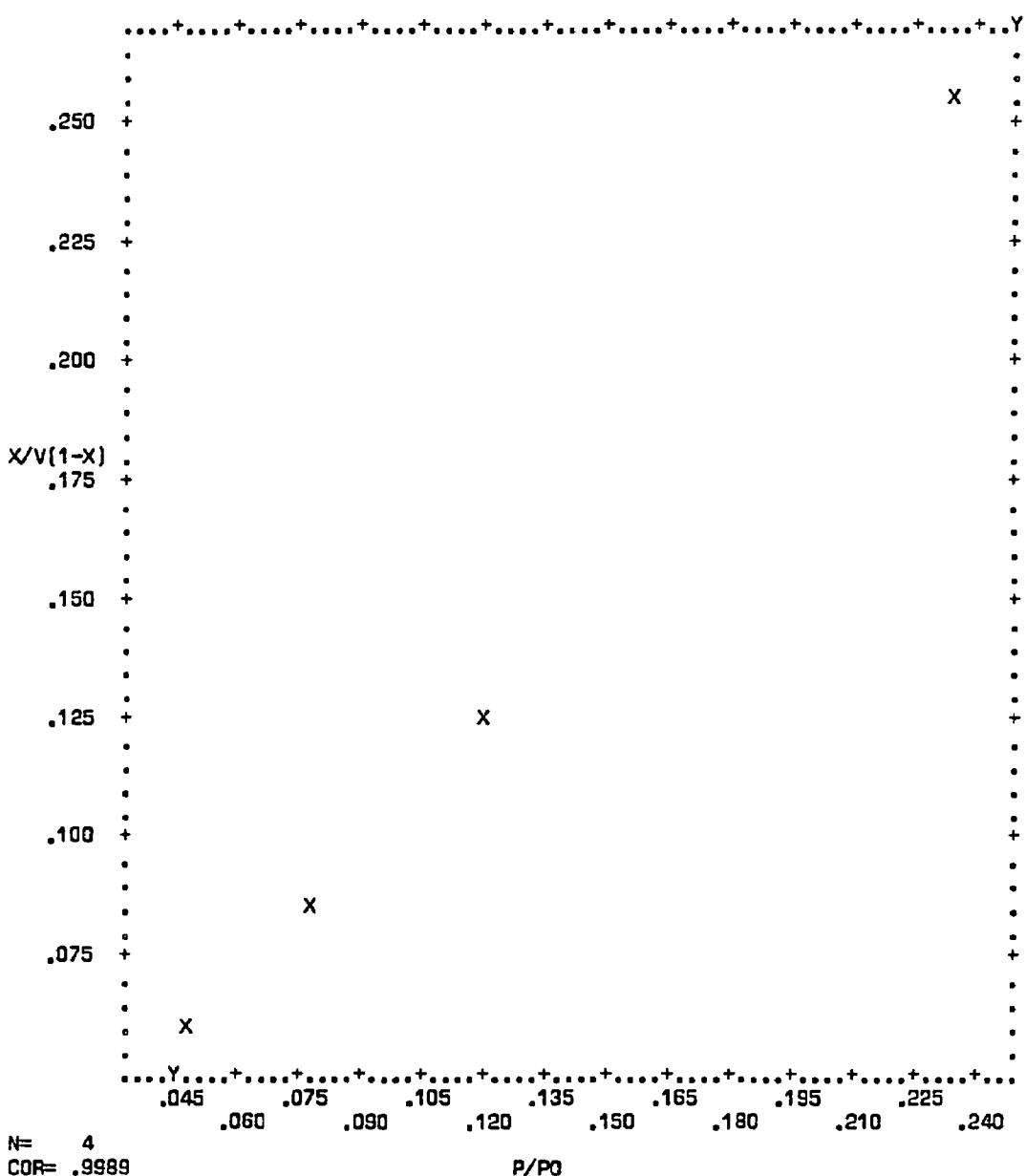
**Figure C-102.** Plot of BET equation versus relative pressure for Converter A155/0941-2-B - Bulk
