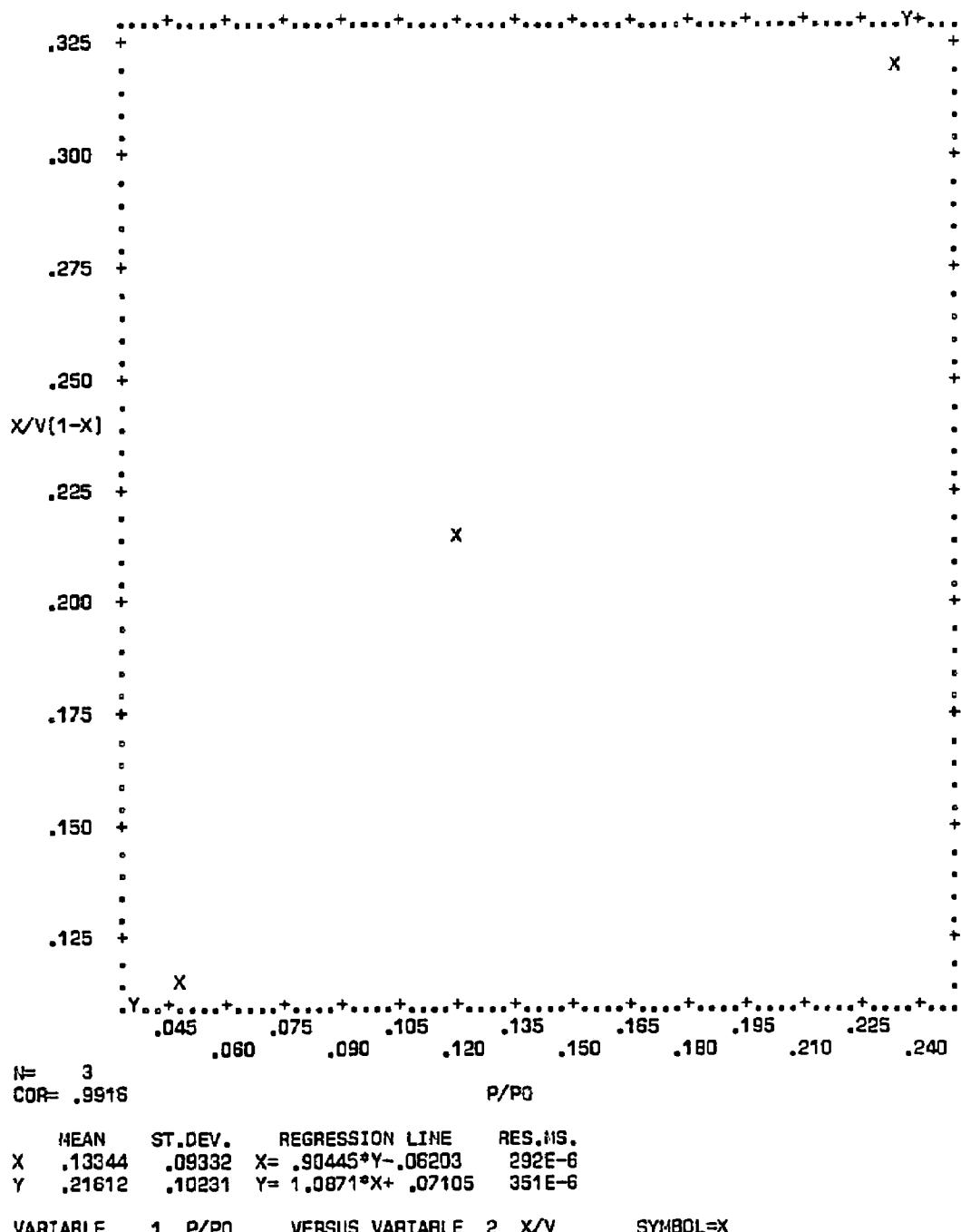
Figure C-88. Plot of BET equation versus relative pressure for Converter A249/0169-3-B - Front Face
