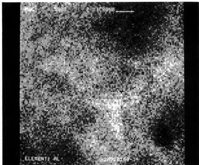
Figure D-175. Aluminum Dot Map at X5000 of Converter A249/0169-1
