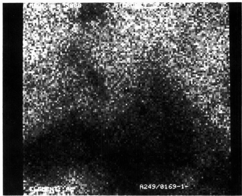
Figure D-285. Aluminum Dot Map at X5000 of Converter A249/0169-1-Rear Face
