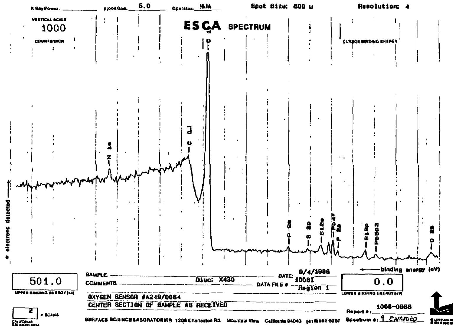
Figure G-14. ESCA Spectrum of Oxygen Sensor A249/0064 from 0 eV to 501 eV (Exterior Surface)
