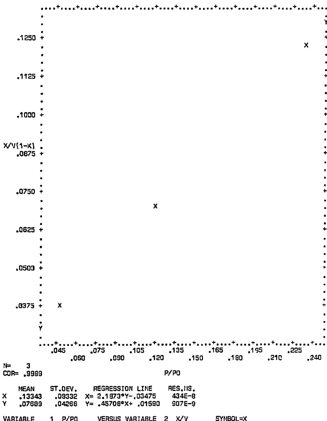
Figure C-91. Plot of BET equation versus relative pressure for Converter A280/0001L-A - Rear Face
