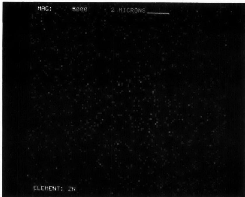
Figure D-189. Zinc Dot Map at X5000 of Converter A249/0169-2
