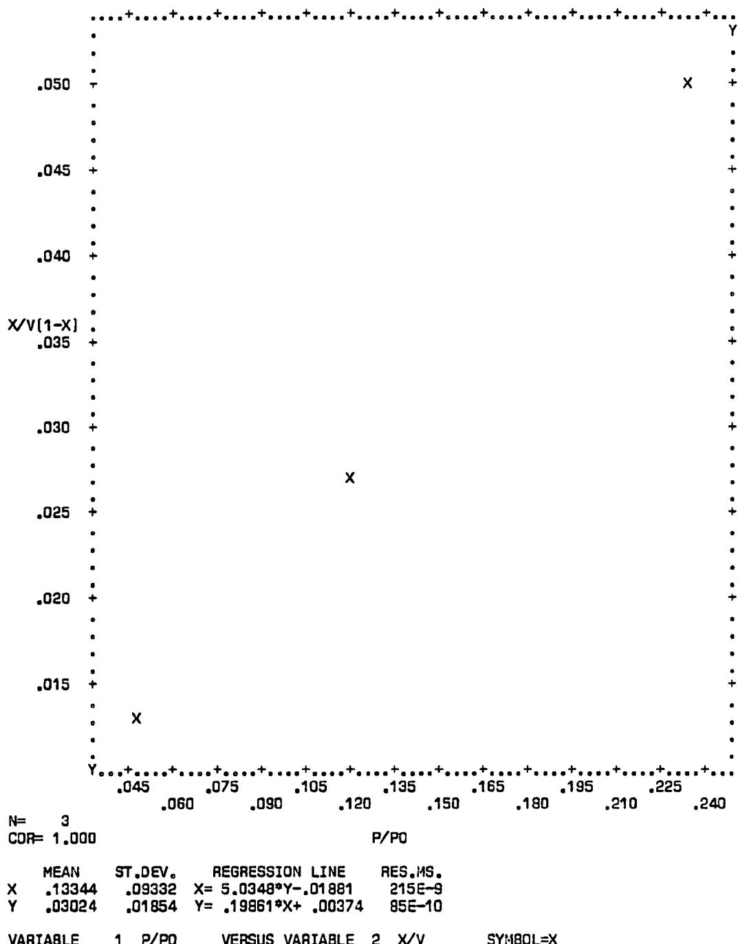
**Figure C-54. Plot of BET equation versus relative pressure for Converter A240/0016L-A - Front Face**
