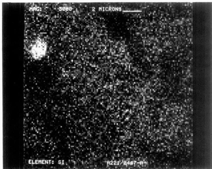
Figure D-266. Silicon Dot Map at X5000 of Converter A221/0447-Rear Face
