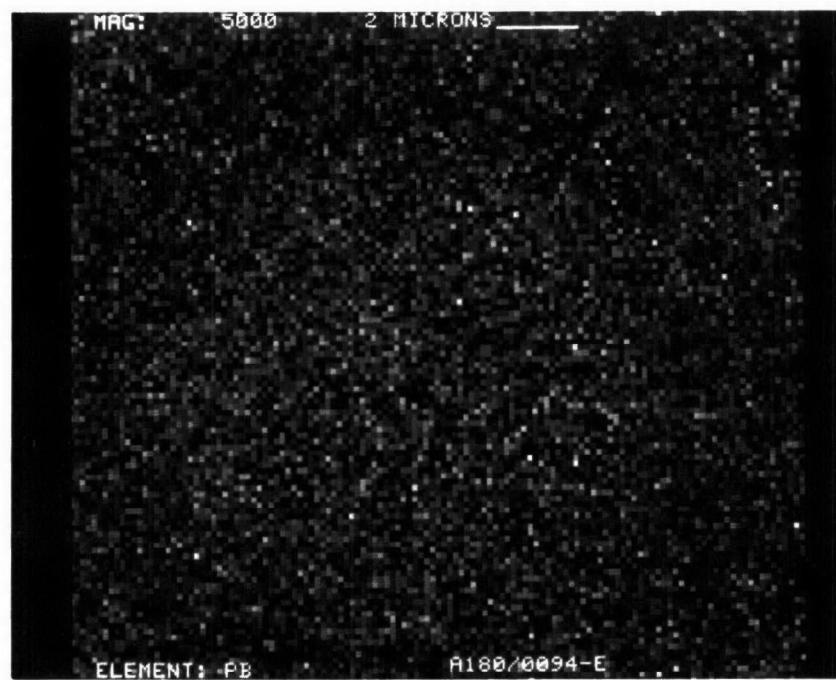
Figure D-7. Lead Dot Map at X5000 of Converter A180/0094
