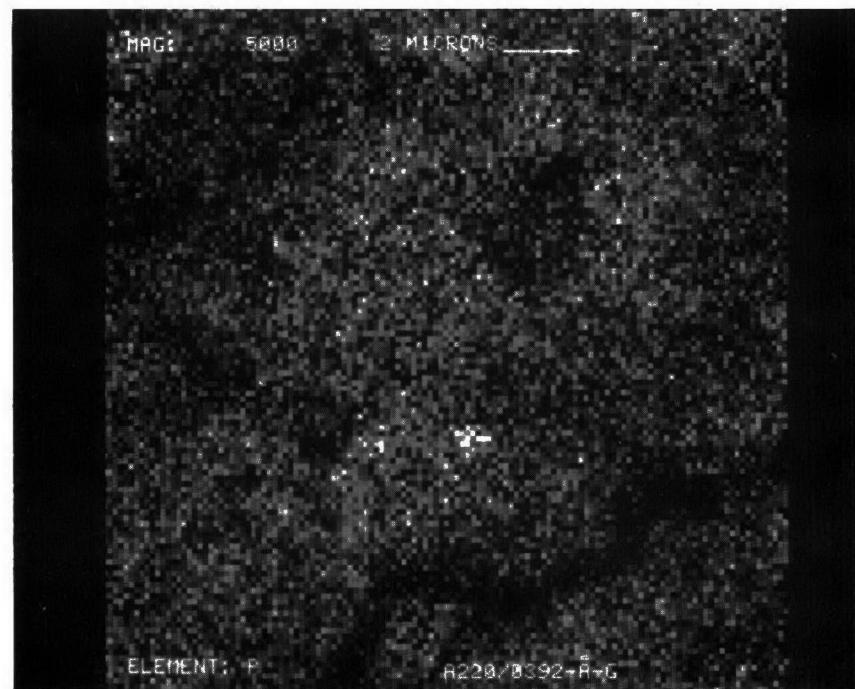
Figure D-260. Phosphorus Dot Map at X5000 of Converter A220/0392-Rear Face
