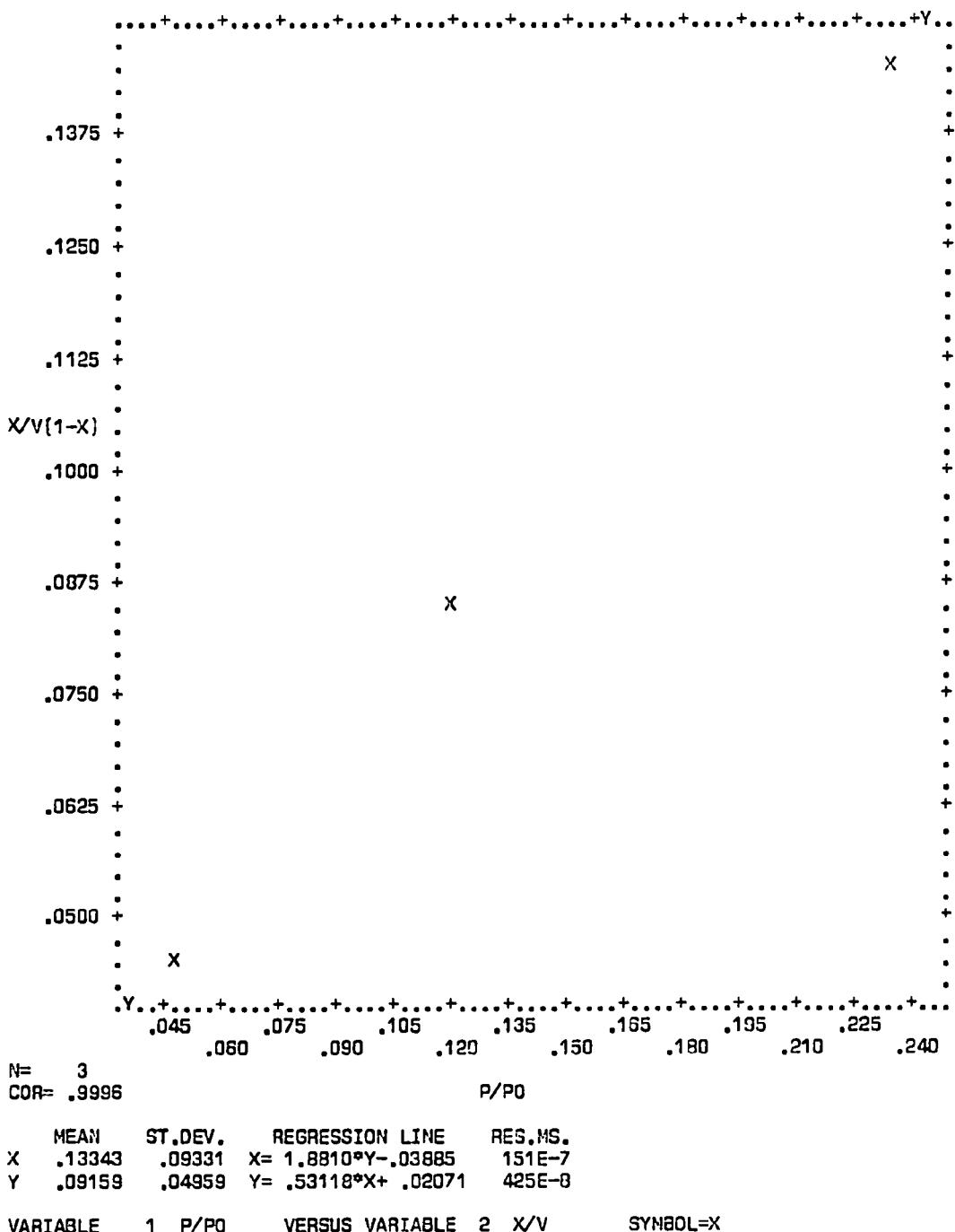
**Figure C-85. Plot of BET equation versus relative pressure for Converter A249/0169-3-A - Front Face**
