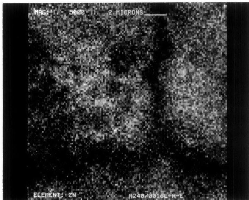
Figure D-129. Zinc Dot Map at X5000 of Converter A240/0016L
