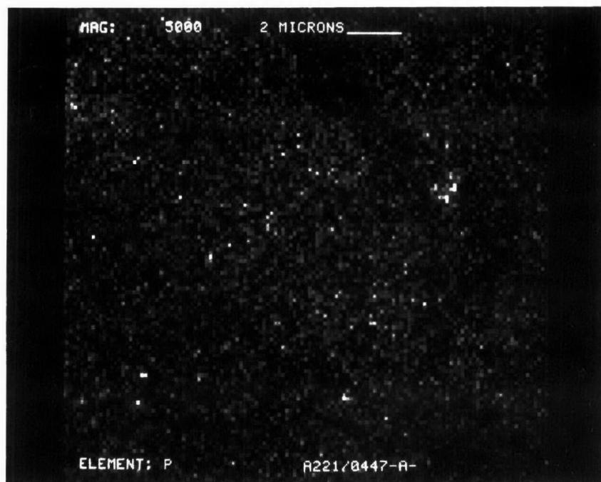
Figure D-270. Phosphorus Dot Map at X5000 of Converter A221/0447-Rear Face
