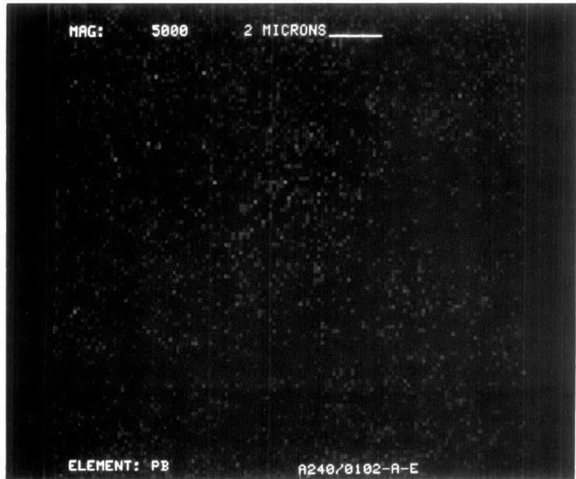
Figure D-137. Lead Dot Map at X5000 of Converter A240/0102
