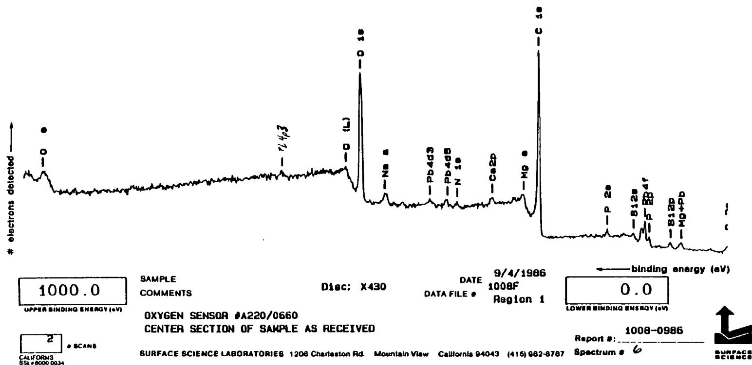
Figure G-1. ESCA Spectrum of Oxygen Sensor A220/0660 from 0 eV to 1000 eV (Exterior Surface)
