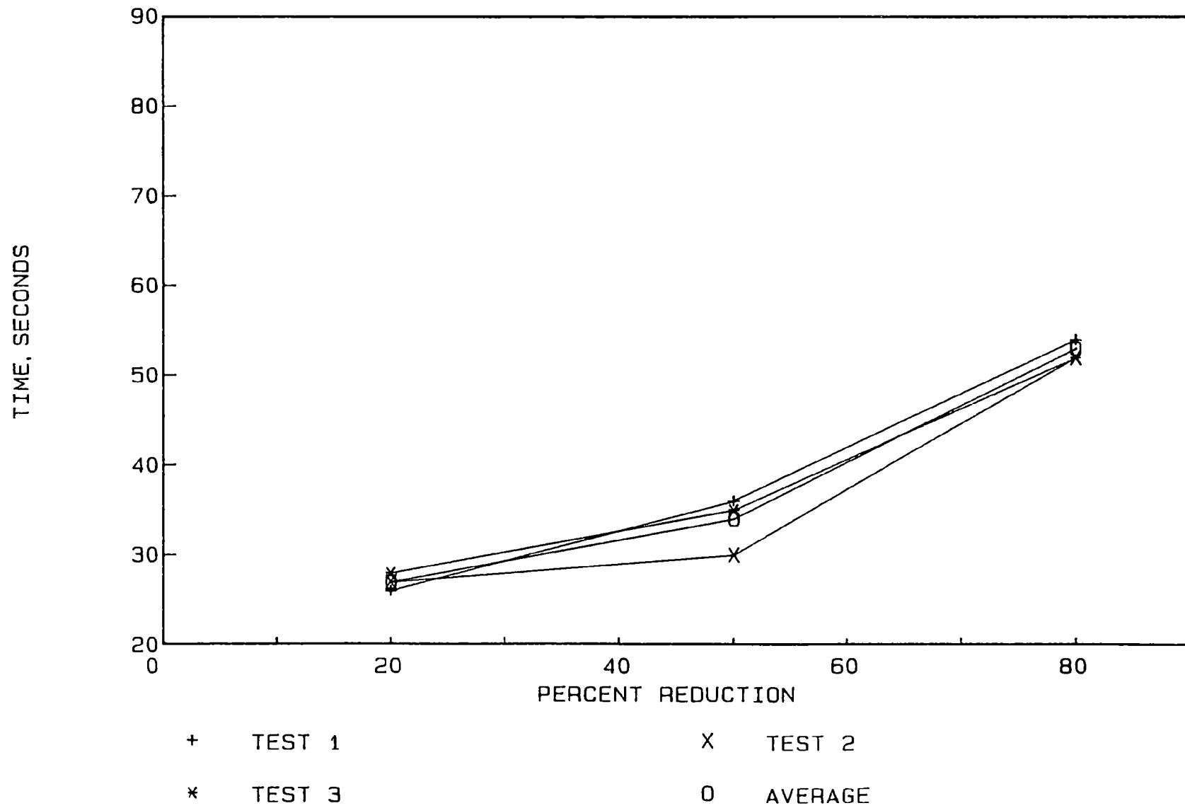
Figure 2. Percent reduction of HC from the light-off test for Converter A215/0201R
