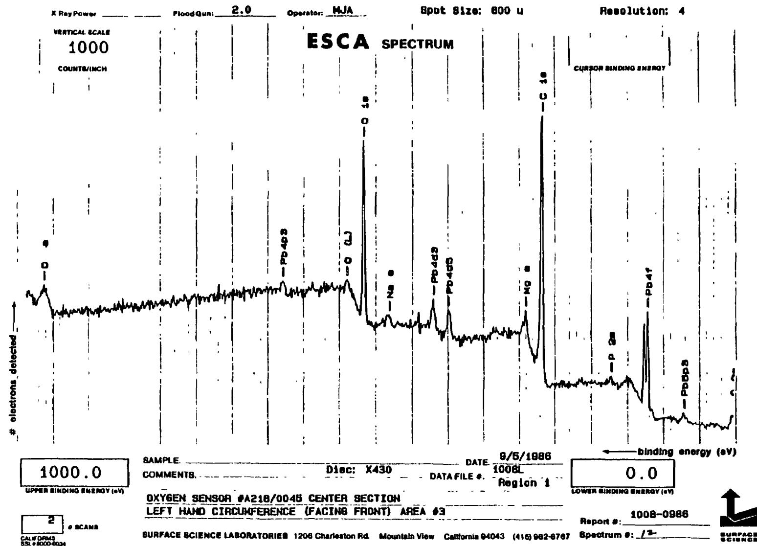
Figure I-16. ESCA Spectrum of Oxygen Sensor A218/0045 from 0 eV to 1000 eV (Location 8)
