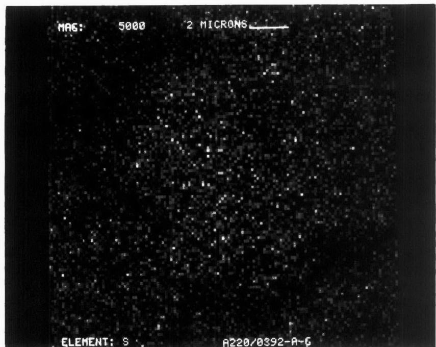
Figure D-258. Sulfur Dot Map at X5000 of Converter A220/0392-Rear Face
