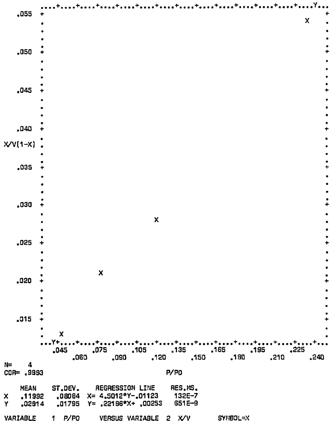
Figure C-20. Plot of BET equation versus relative pressure for Converter A220/0392-A - Rear Face
