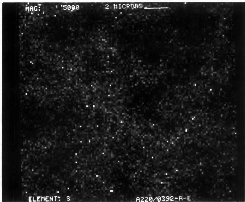
Figure D-58. Sulfur Dot Map at X5000 of Converter A220/0392
