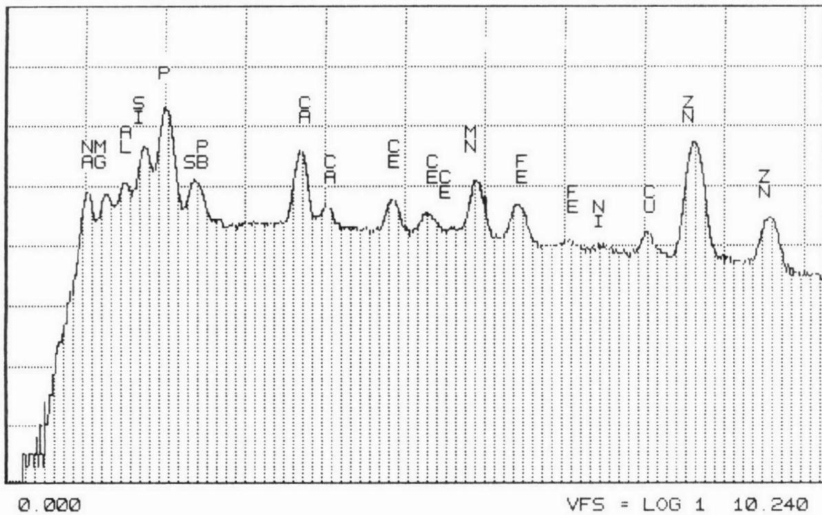
Figure D-201. SEM/EDX Spectrum of Converter A280/0001L
