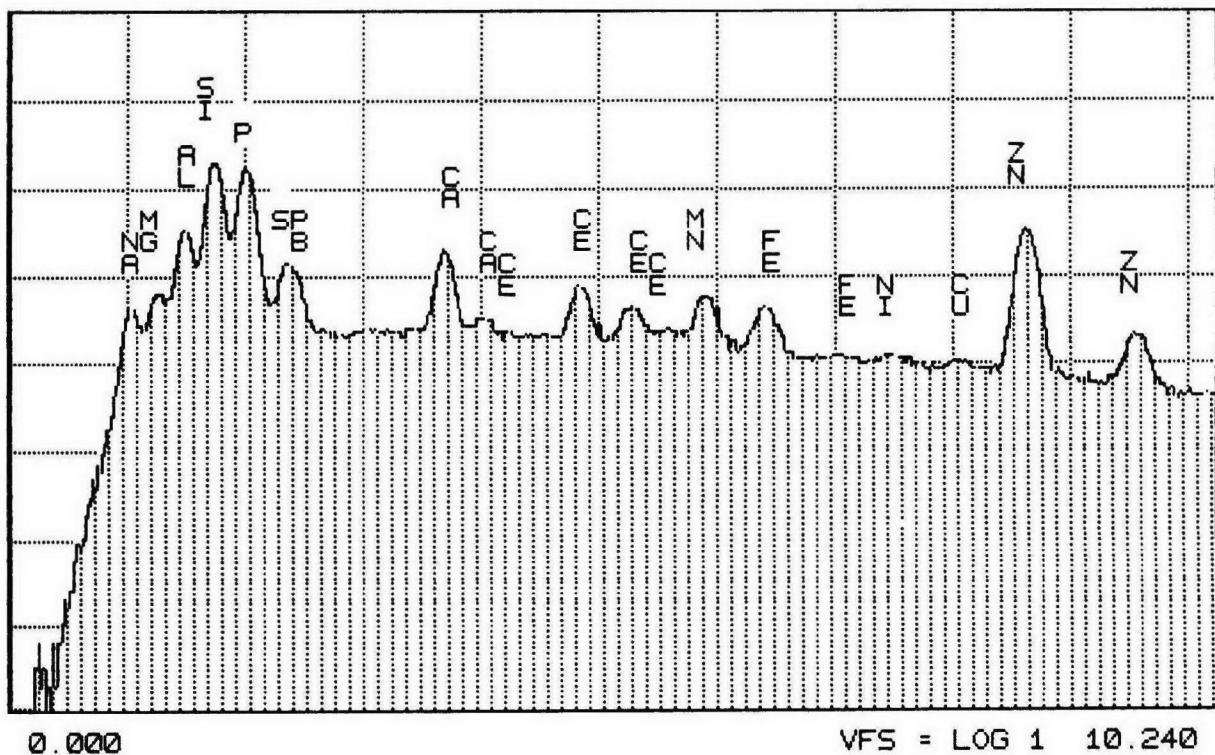
Figure D-11. SEM/EDX Spectrum of Converter A193/0908
