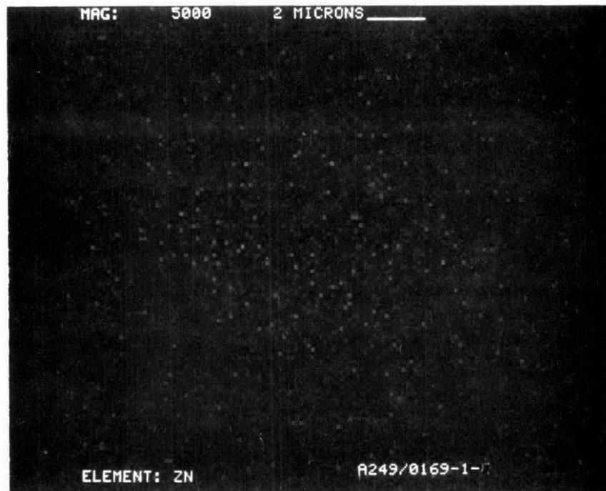
Figure D-289. Zinc Dot Map at X5000 of Converter A249/0169-1-Rear Face
