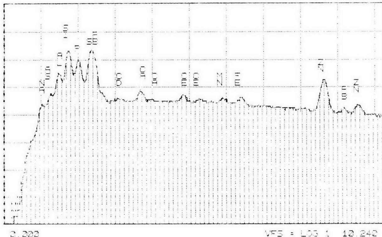
Figure D-91. SEM/EDX Spectrum of Converter A221/0447
