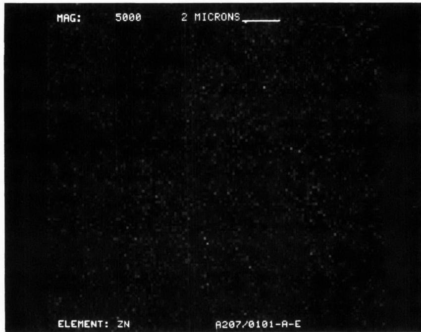
Figure D-239. Zinc Dot Map at X5000 of Converter A207/0101
