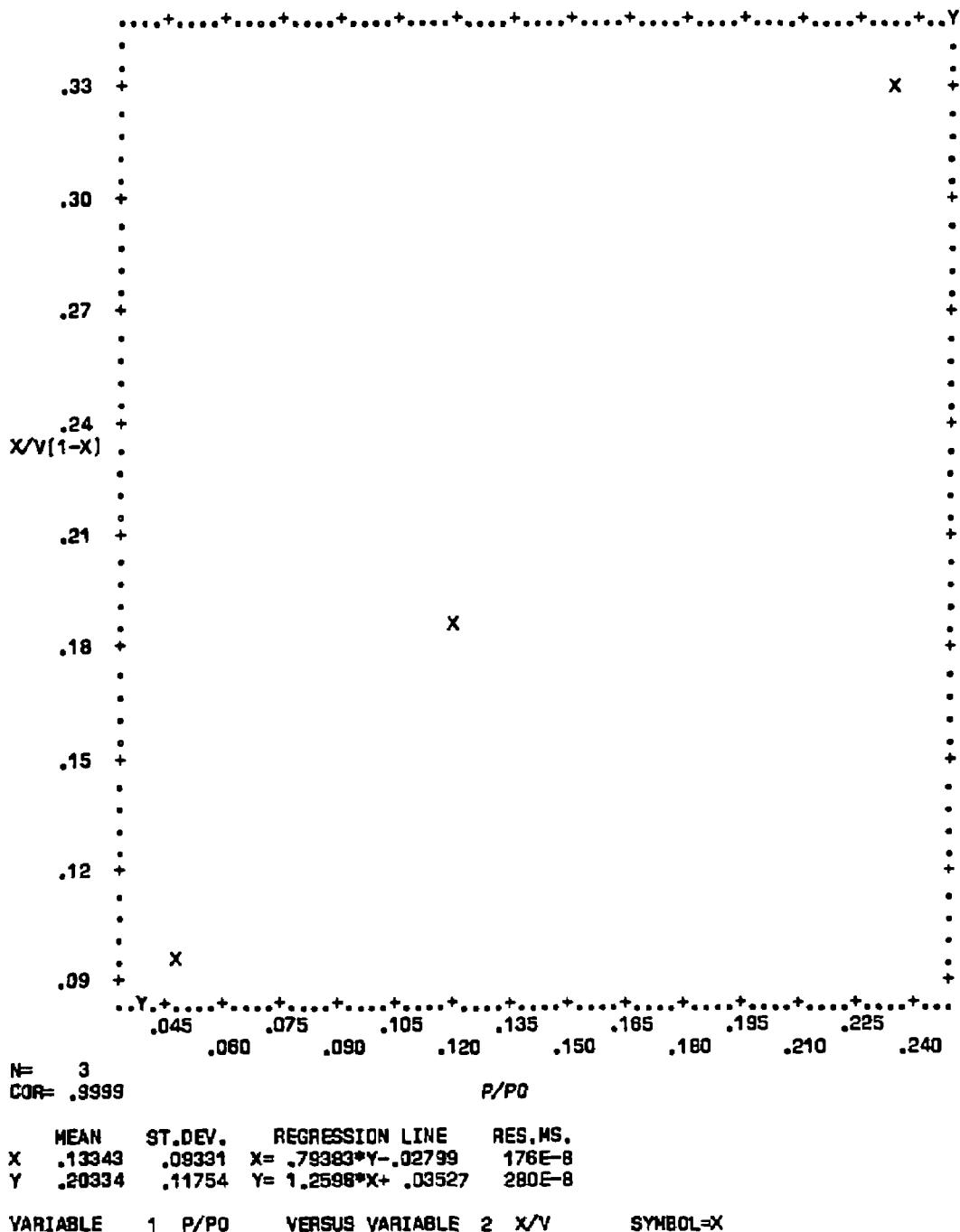
Figure C-7. Plot of BET equation versus relative pressure for Converter A193/0908-B - Bulk
