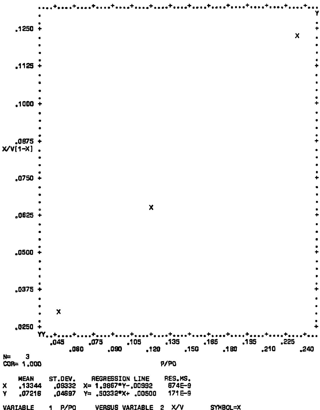
Figure C-76. Plot of BET equation versus relative pressure for Converter A240/0334L-B - Bulk
