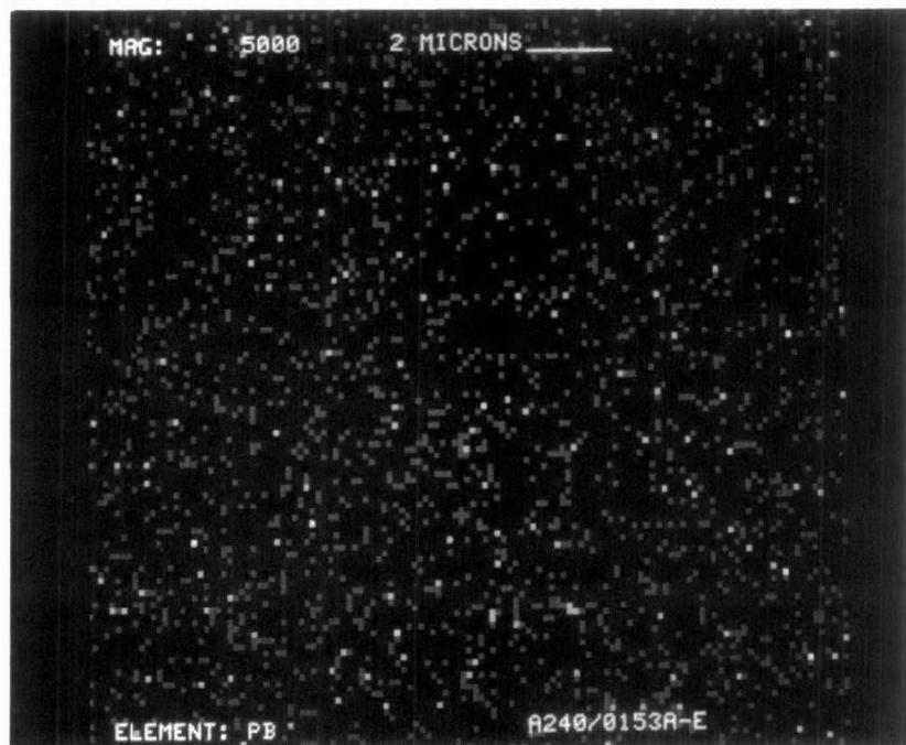
Figure D-157. Lead Dot Map at X5000 of Converter A240/0153
