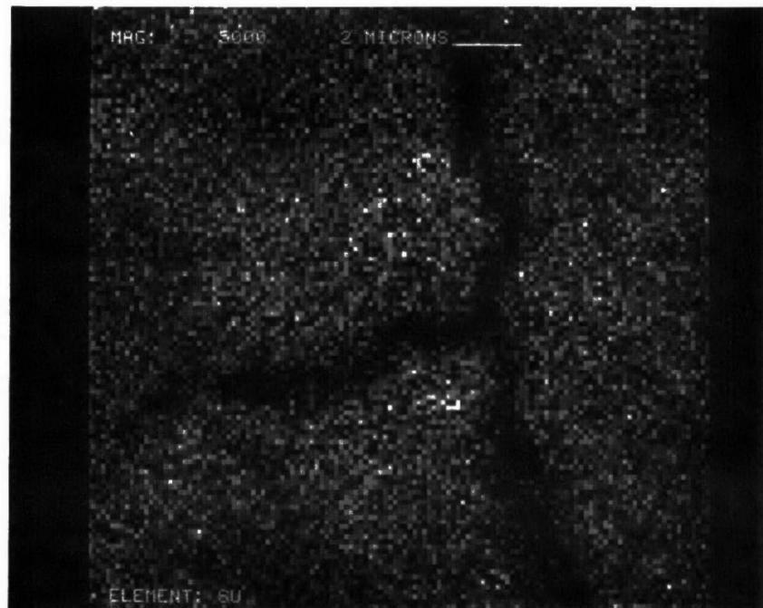
Figure D-28. Sulfur Dot Map at X5000 of Converter A218/0045
