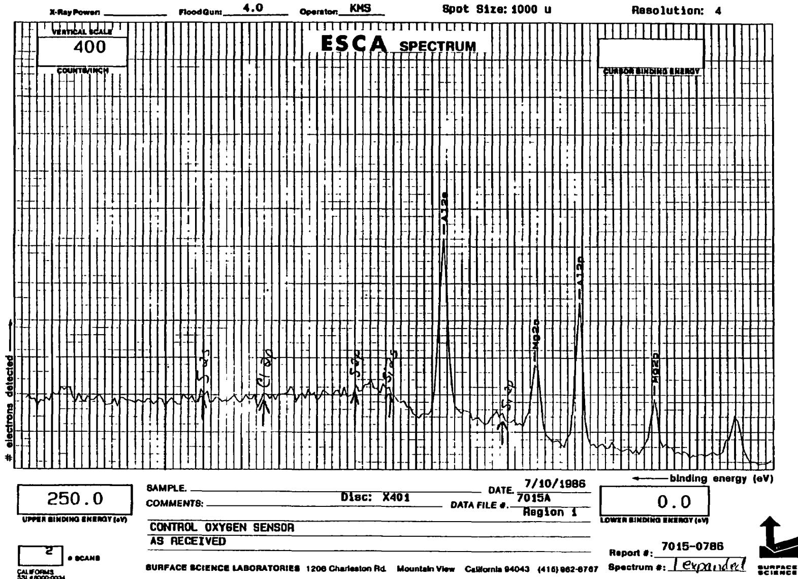
Figure G-30. ESCA Spectrum of New Chrysler Sensor from 0 eV to 250 eV (Exterior Surface)
