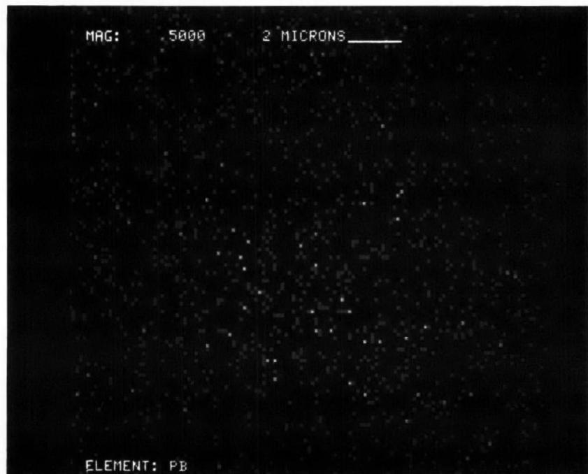
Figure D-187. Lead Dot Map at X5000 of Converter A249/0169-2
