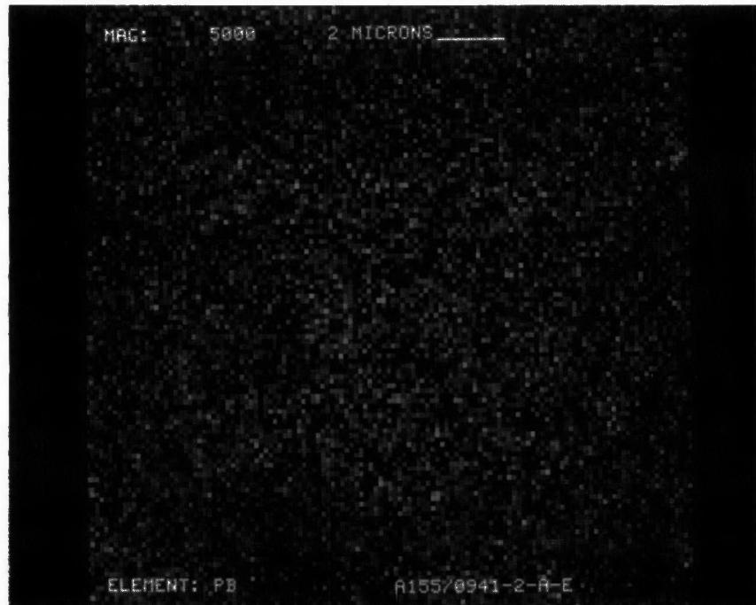
Figure D-227. Lead Dot Map at X5000 of Converter A155/0941-2
