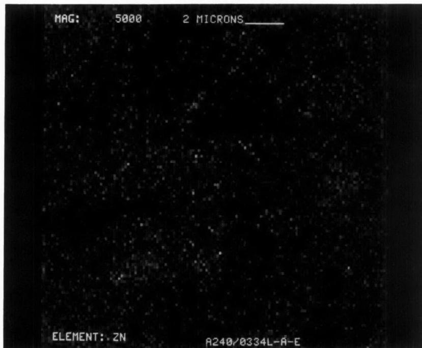
Figure D-169. Zinc Dot Map at X5000 of Converter A240/0334L
