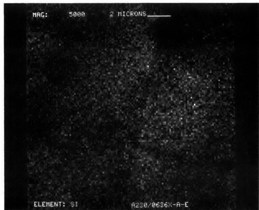
Figure D-116. Silicon Dot Map at X5000 of Converter A230/0636X
