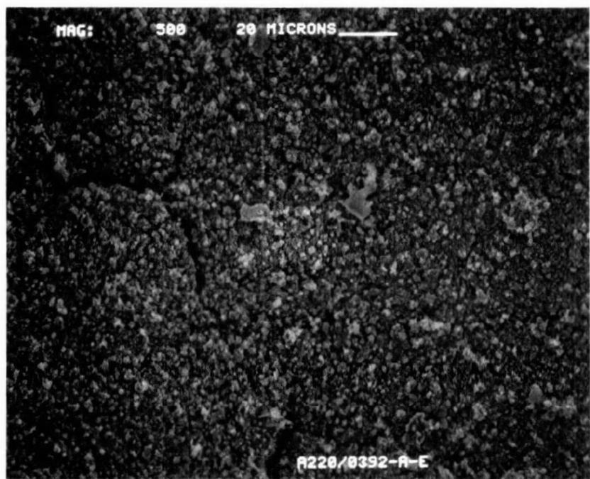
Figure D-52. Scanning Electron Micrograph at X500 of Converter A220/0392
