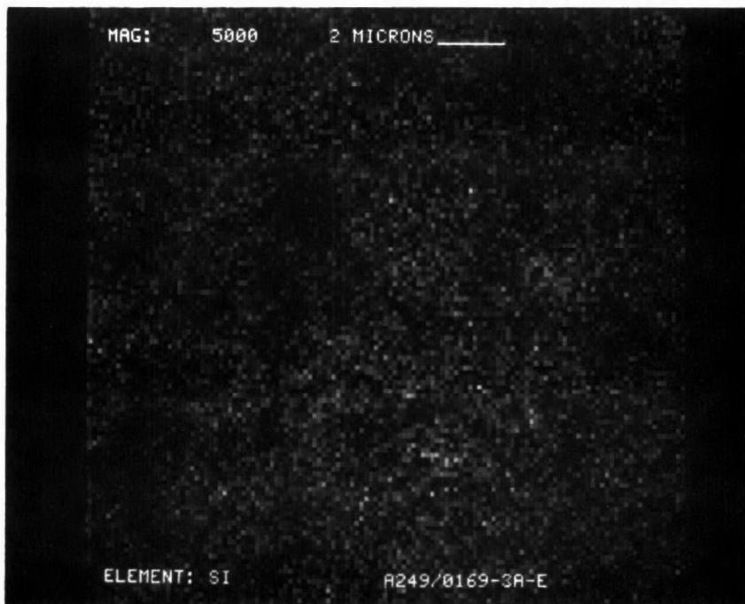
Figure D-196. Silicon Dot Map at X5000 of Converter A249/0169-3
