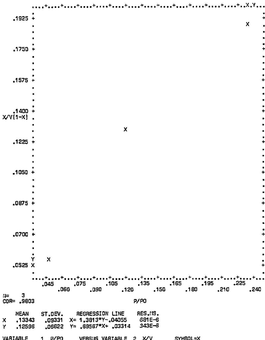
Figure C-96. Plot of BET equation versus relative pressure for Converter A155/0941-1-A - Rear Face
