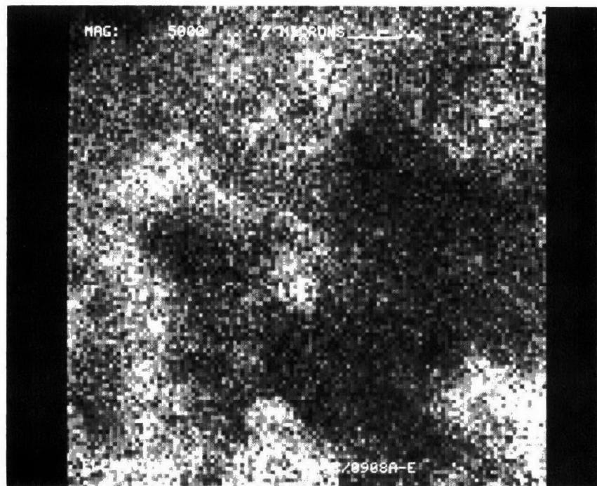
Figure D-20. Phosphorus Dot Map at X5000 of Converter A193/0908
