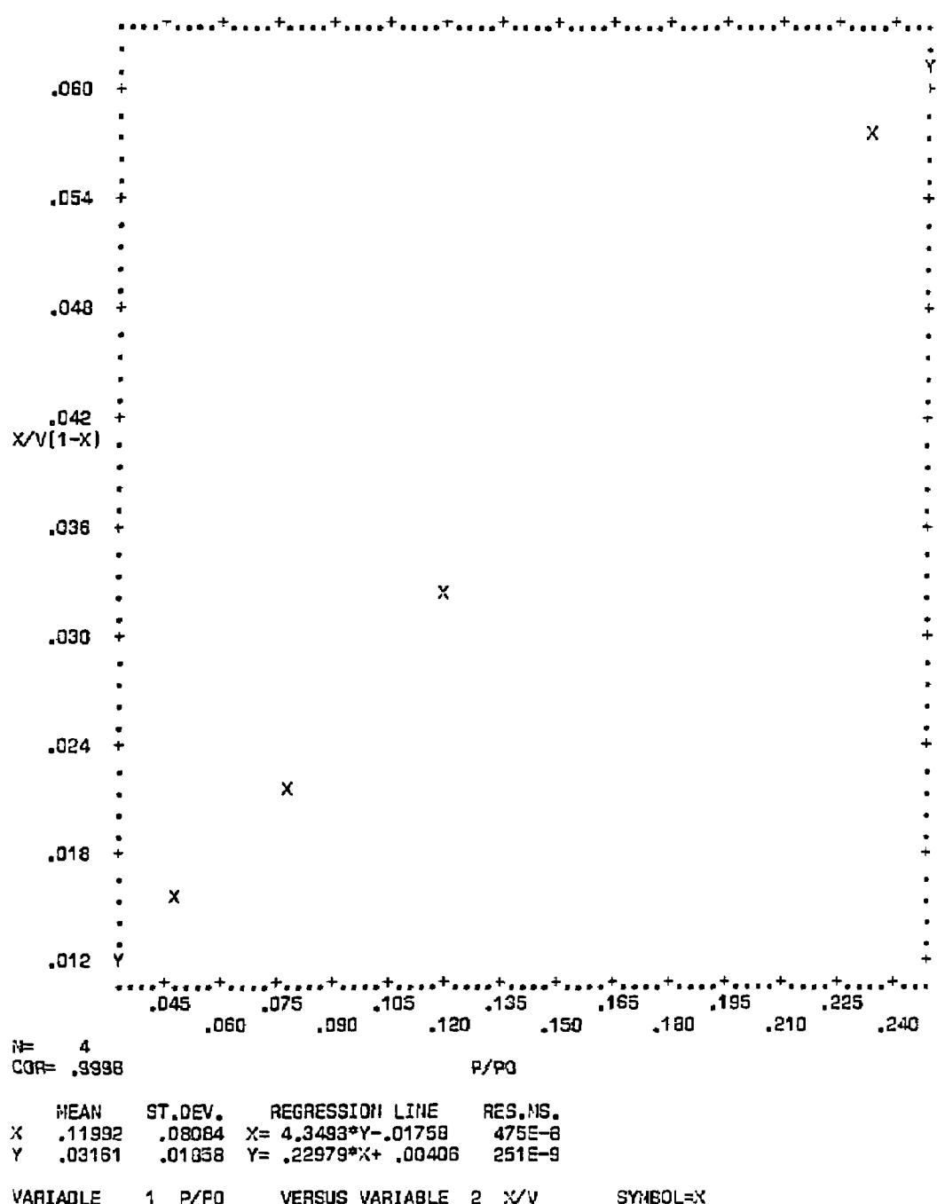
**Figure C-47. Plot of BET equation versus relative pressure for Converter A230/0177X-B - Front Face**
