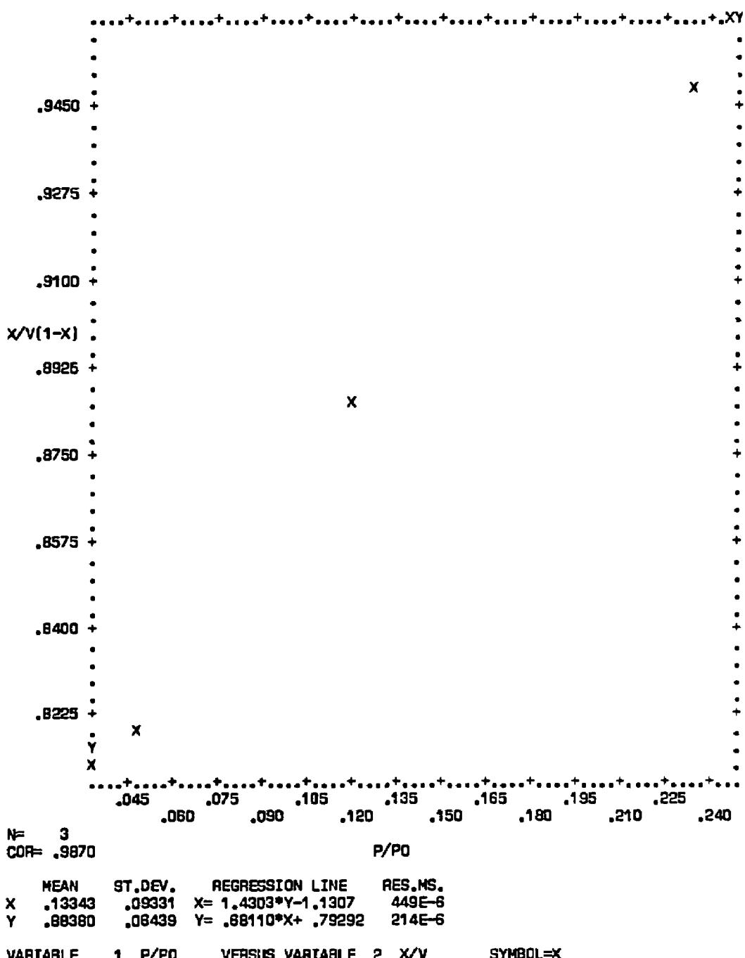
Figure F-13. Plot of BET equation versus relative pressure
