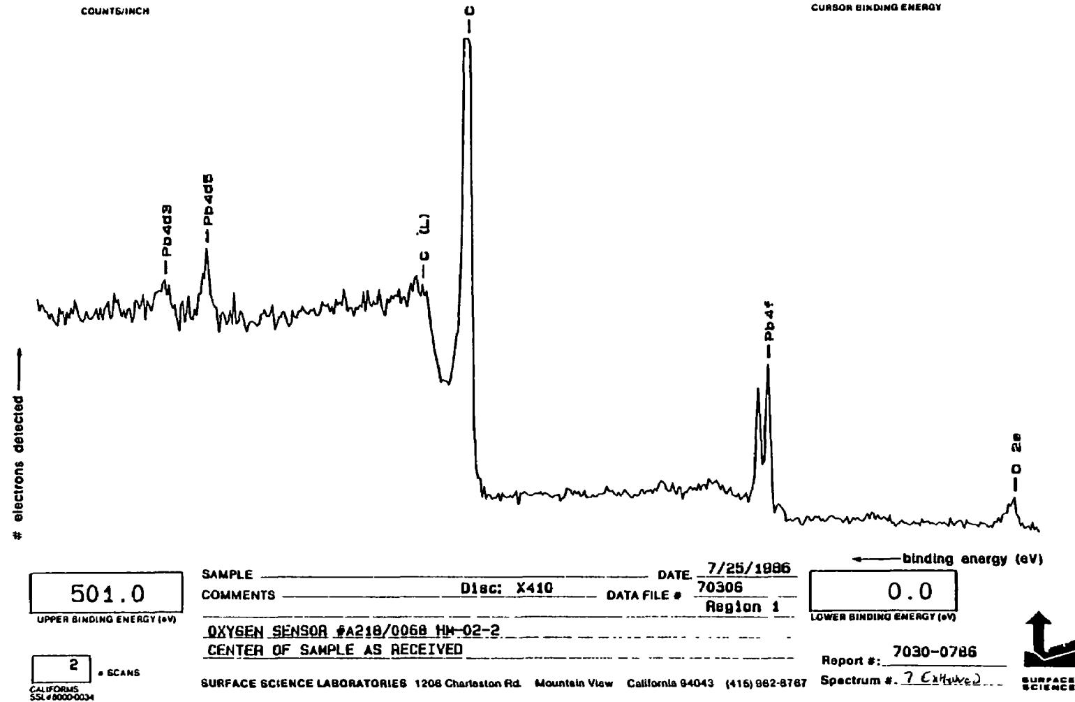
Figure G-27. ESCA Spectrum of Oxygen Sensor A218/0068 from 0 eV to 501 eV (Exterior Surface)
