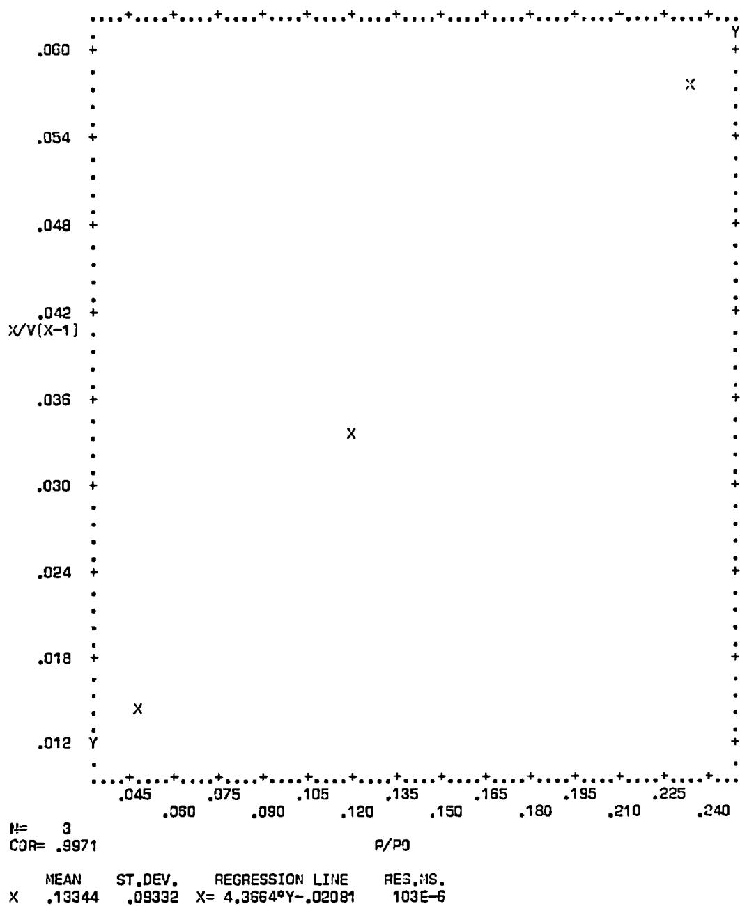
Figure C-77. Plot of BET equation versus relative pressure for Converter A240/0334L-B - Front Face
