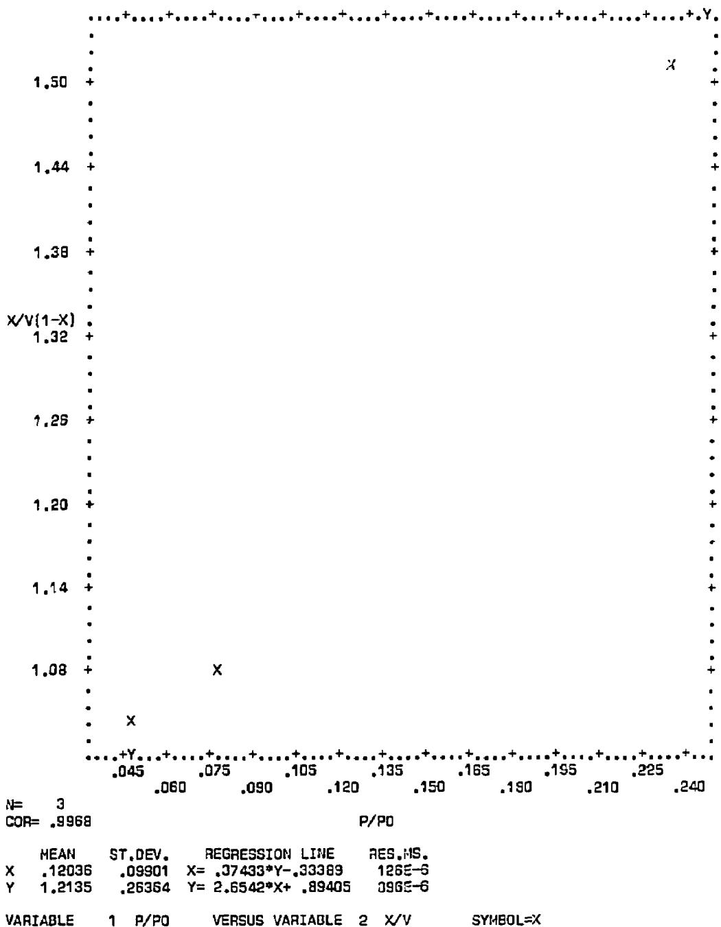
Figure F-5. Plot of BET equation versus relative pressure
