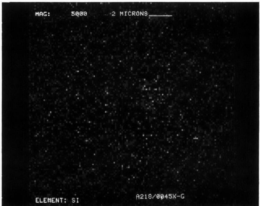
Figure D-246. Silicon Dot Map at X5000 of Converter A218/0045X-Rear Face
