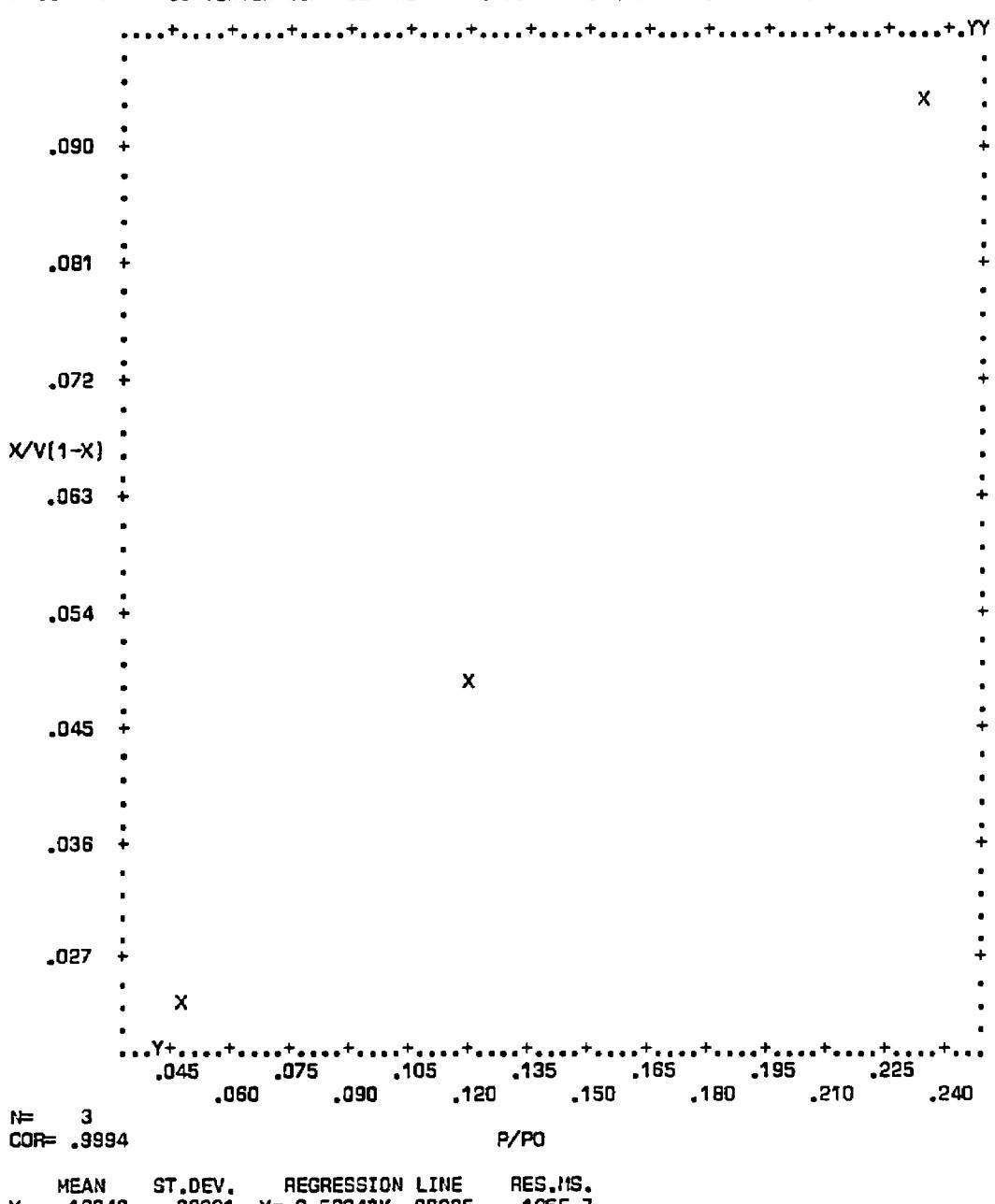
Figure C-51. Plot of BET equation versus relative pressure for Converter A230/0636X-B - Bulk
