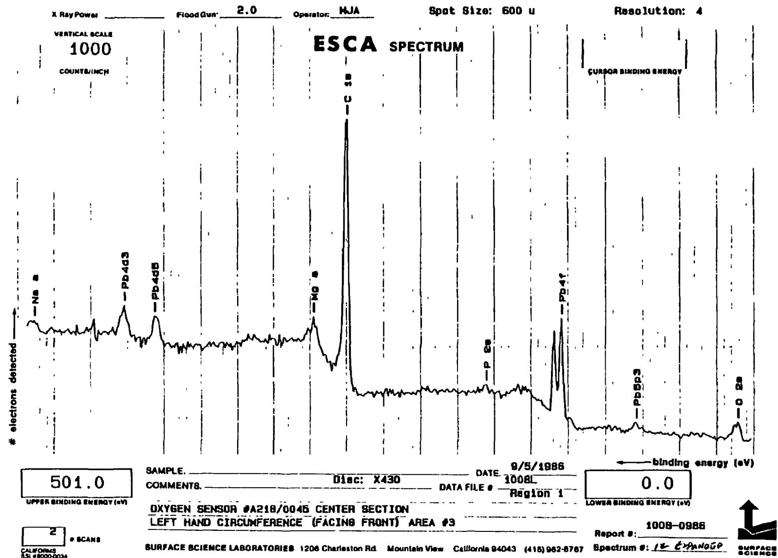
Figure I-17. ESCA Spectrum of Oxygen Sensor A218/0045 from 0 eV to 501 eV (Location 8)
