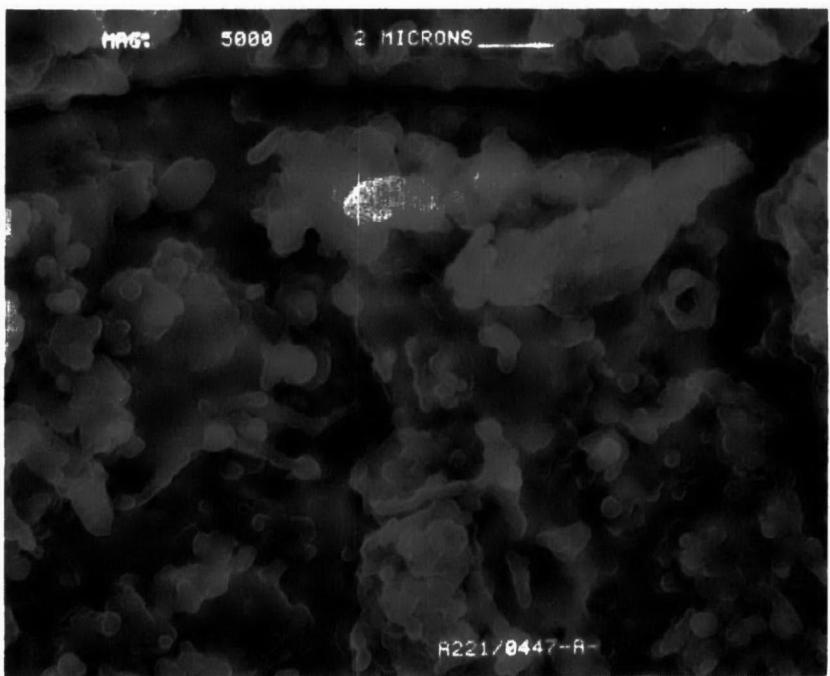
Figure D-94. Scanning Electron Micrograph at X5000 of Converter A221/0447
