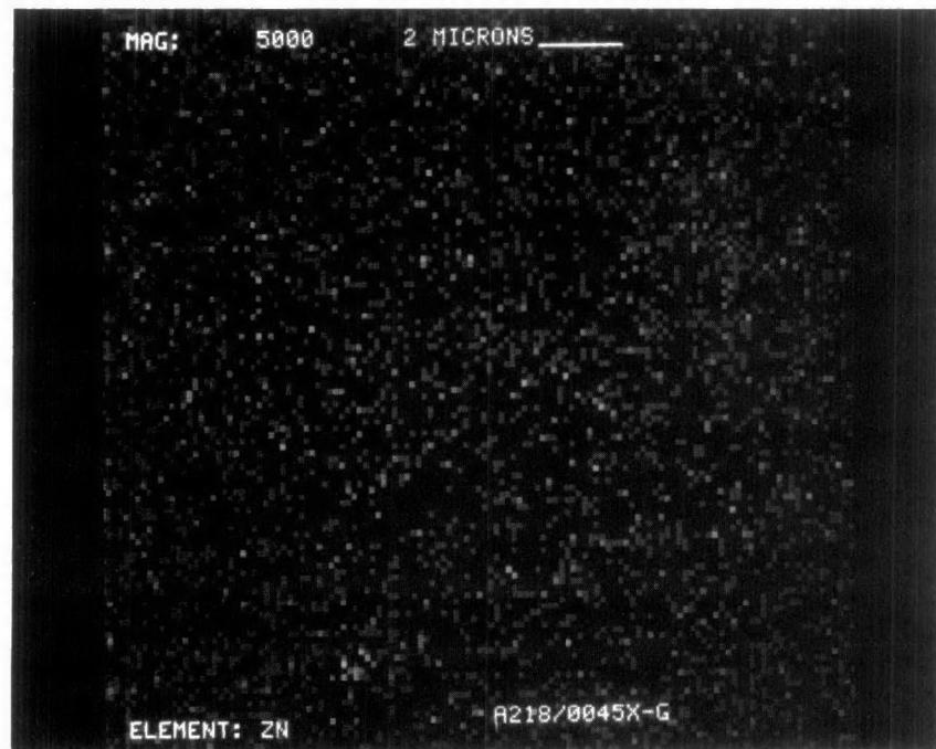
Figure D-249. Zinc Dot Map at X5000 of Converter A218/0045X-Rear Face
