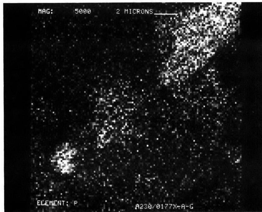
Figure D-280. Phosphorus Dot Map at X5000 of Converter A230/0177X-Rear Face
