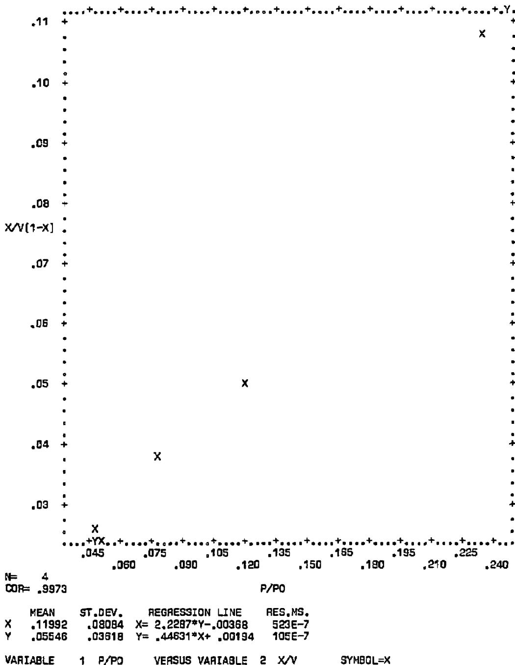
Figure C-66. Plot of BET equation versus relative pressure for Converter A240/0141L-B - Bulk
