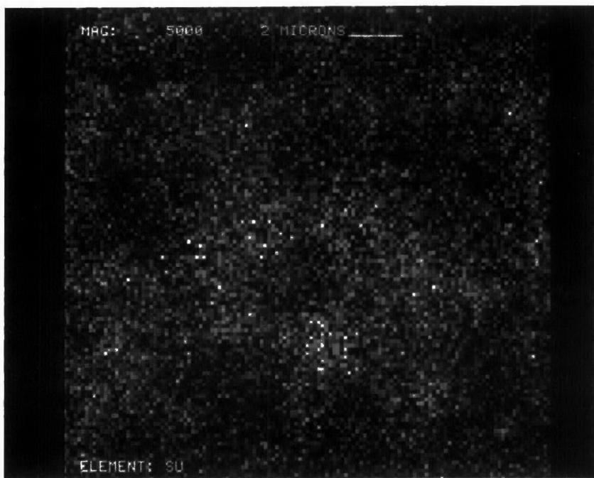
Figure D-38. Sulfur Dot Map at X5000 of Converter A218/0045X
