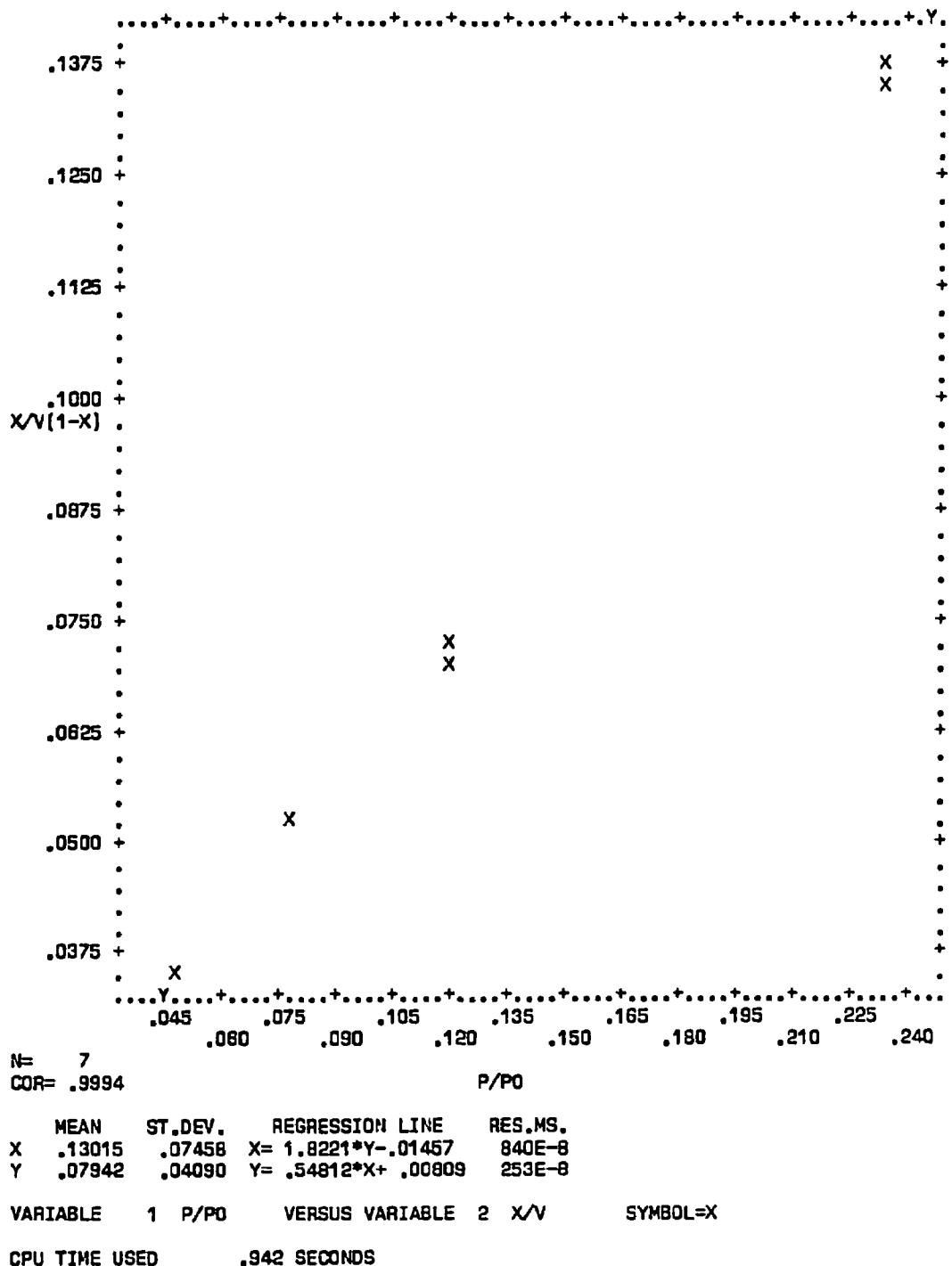
**Figure C-79. Plot of BET equation versus relative pressure for Converter A249/0169-1 - Front Face**
