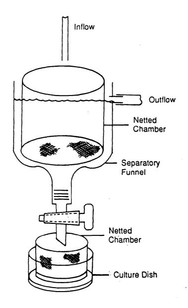
Figure 2. Apparatus for collection of postlarval mysids from gravid females. From Lussier et al., 1988.
