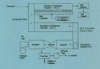
Figure 1. Peak oil Incineration unit process diagram.
