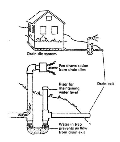
Figure 8.2. Individual pipe variation of sub-slab ventilation.(3)
