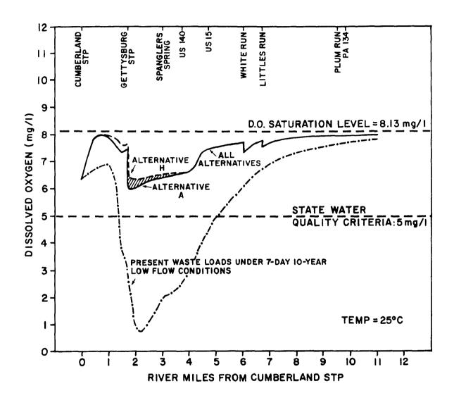
FIGURE Y-I PROJECTED DISSOLVED OXYGEN PROFILES UNDER 7-DAY 10-YEAR LOW FLOW CONDITIONS
