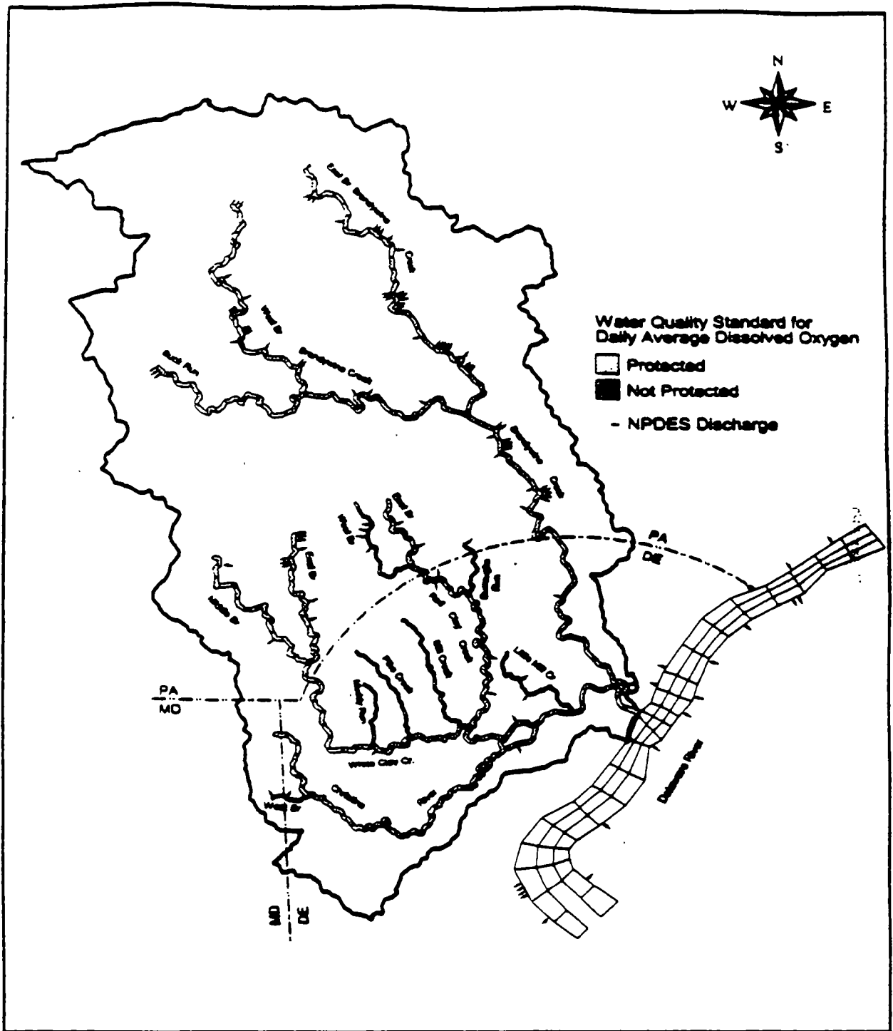
Figure 11. Modeled stream segments which violate daily average dissolved oxygen water quality criteria based on the Level 1 allocation analysis.
