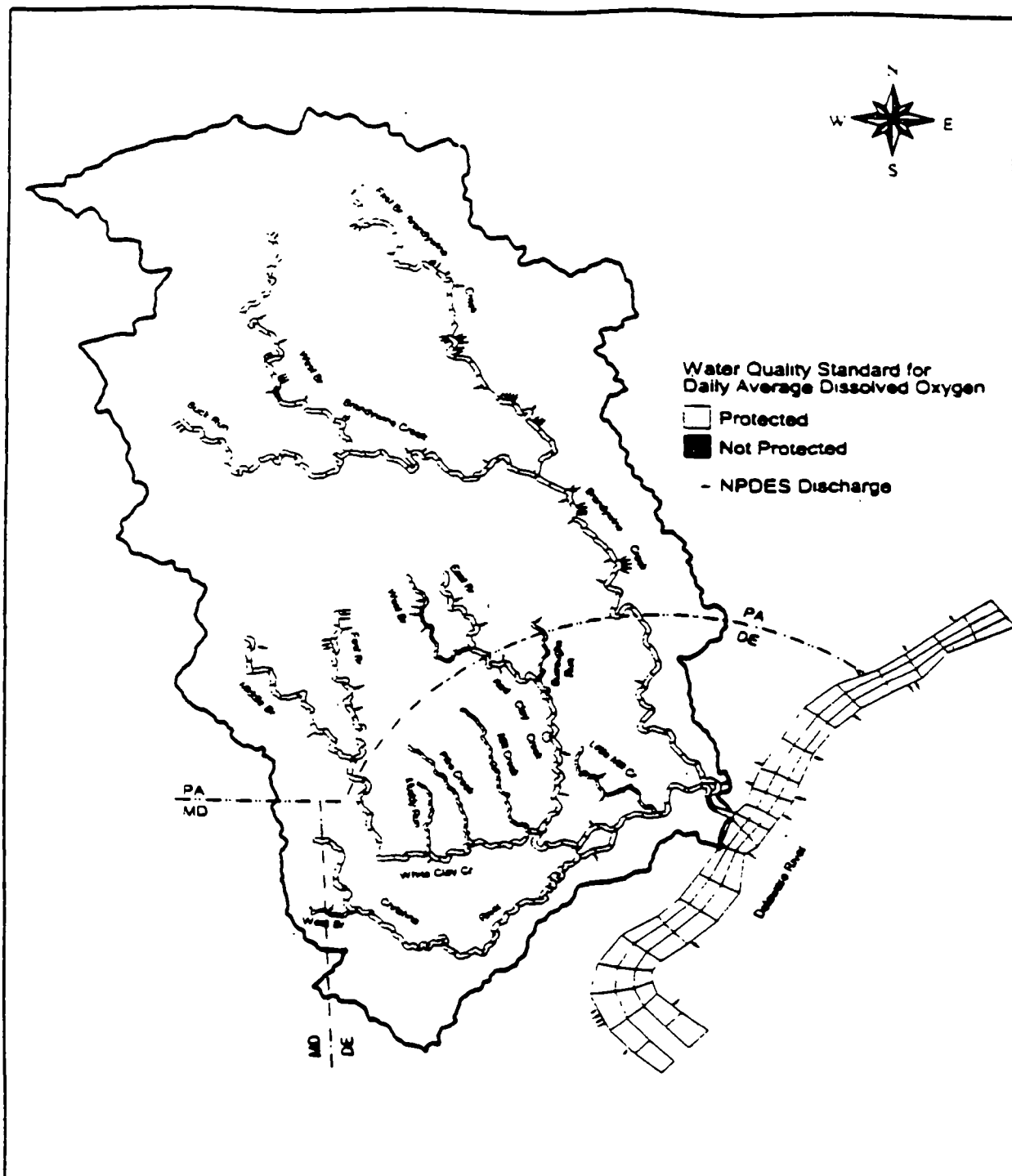
Figure 8 Modeled stream segments violating daily average dissolved oxygen water quality criteria based on the EFDC model during critical conditions.
