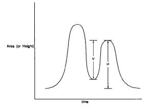
For pesticide analysis the X-axis shall be displayed such that a data reviewer can calculate the % Resolution.
