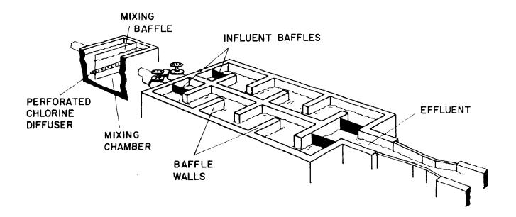
The operator can evaluate the contact tank more accurately for both flow patterns and contact times by conducting a dye test. Rhodamine WT is a fluorescent dye which is typically used. The dye is added to the wastewater at the point of chlorine injection (or at the next convenient upstream point). If the dye is obtained in solid form, it should be dissolved in water prior to use.
