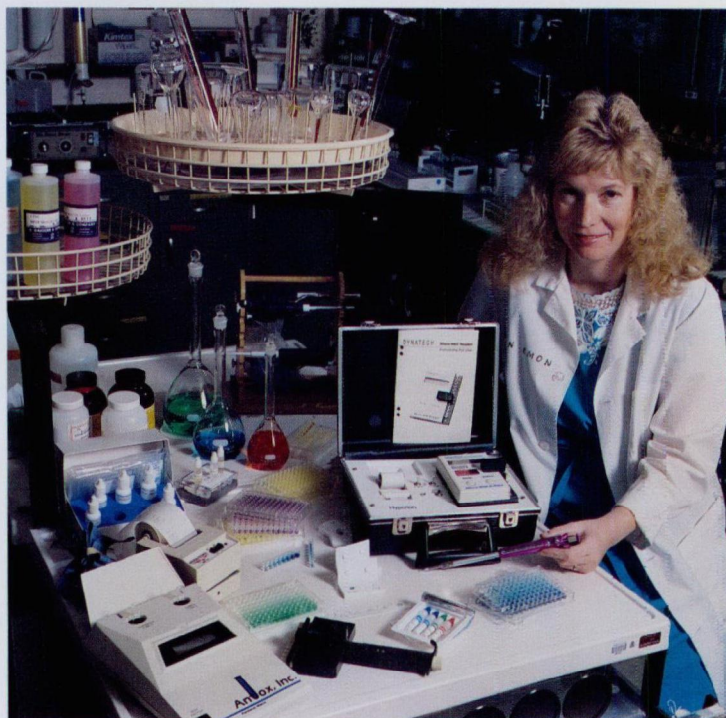
Field Portable Test Kit for Immunochemical Environmental Monitoring
