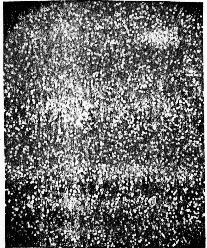
FIELD BLANK - note absence of mineral and carbon particles. Shows light contamination from handling.
