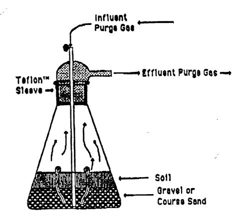
FIGURE 2. LABORATORY FLASK APPARATUS USED FOR SOIL VENTING EVALUATION
