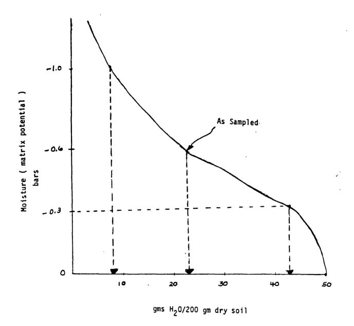
FIGURE 5. SOIL MOISTURE CHARACTERISTIC CURVE
