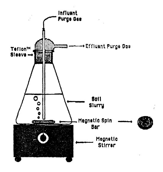
FIGURE 3. LABORATORY FLASK APPARATUS USED FOR SLURRY TAPE MATERIAL
