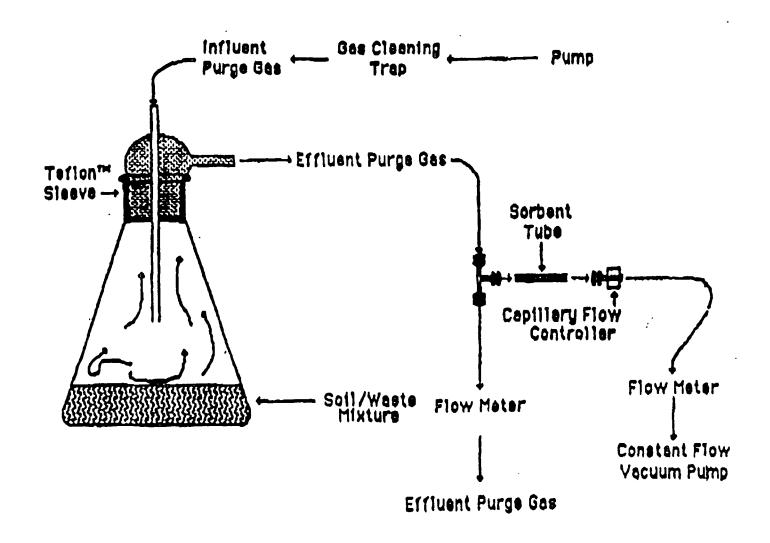
Figure 1. LABORATORY FLASK APPARATUS USED FOR MASS BALANCE MEASUREMENTS
