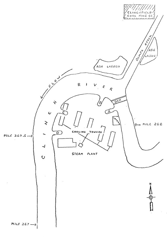
FIGURE 1. DIAGRAMMATIC MAP OF THE APPALACHIAN POWER COMPANY STEAM PLANT AND A PORTION OF THE CLINCH RIVER, VIRGINIA (Symbols A, B, C, and D indicate steam plant effluents)
