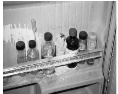
Air and water reactive chemicals stored in refrigerator – even small containers can be big problems.
