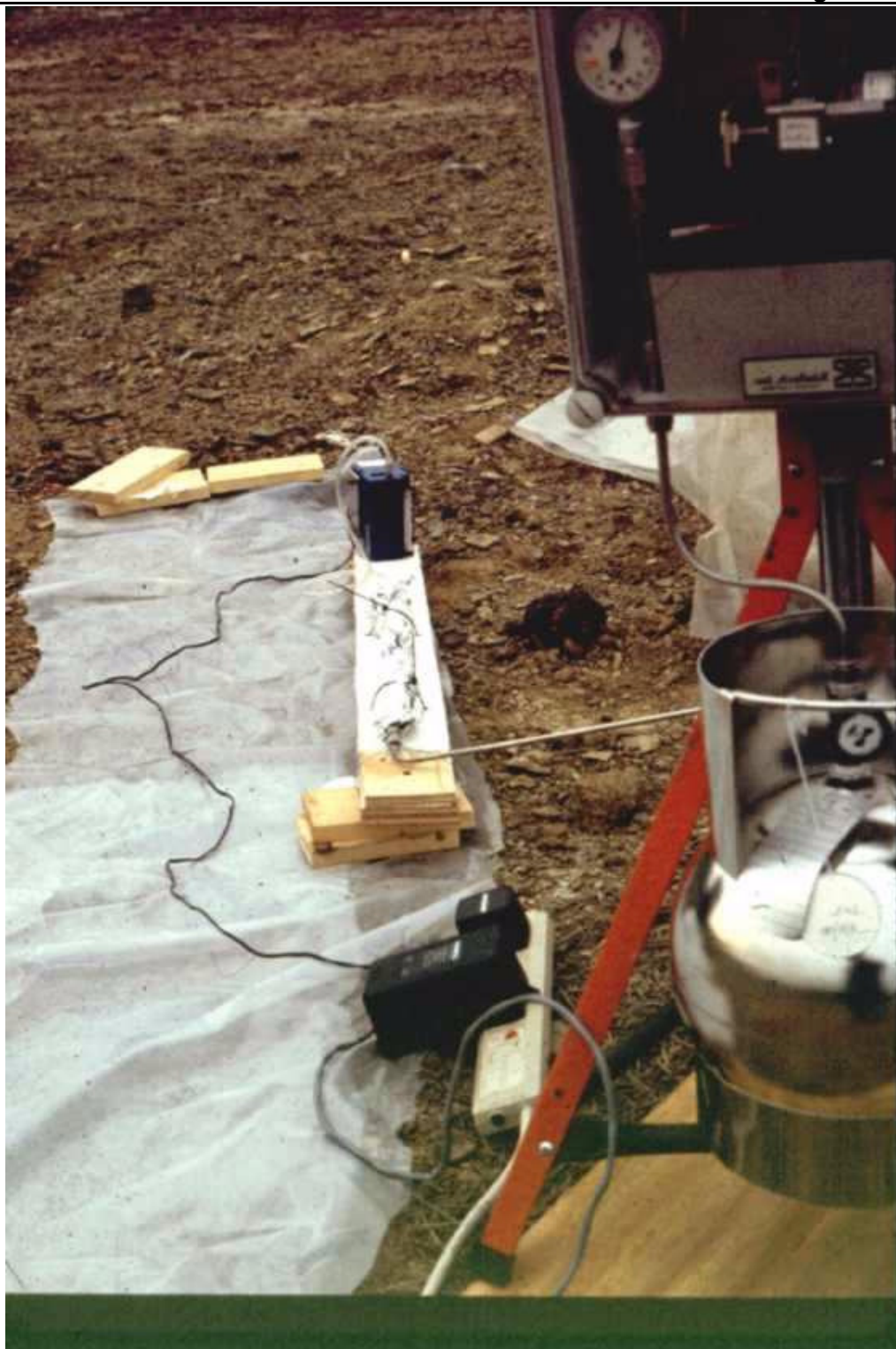
Figure A-11. Application of Compendium Method TO-10A (Semi-volatiles, PCBs) and Compendium Method TO-15 (Methane, NMOCs, VOCs) Sampling at a MSW Landfill.
