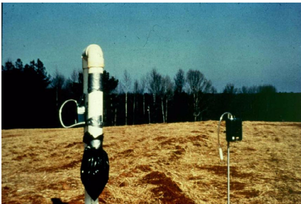
Figure A-12. Encapsulated Vent Tube Sampling for PCBs Utilizing EPA Compendium Method TO-10A. (Note Portable Monitor to the Right of the Vent Tube for Ambient Monitoring of Emissions During Normal Vent Tube Emissions.)
