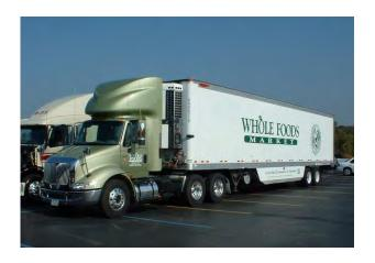
Whole Foods MWD projects savings of 4% on total fuel costs due to the fairings. Projected yearly savings are 16,931 gallons, based on 2,582,032 miles traveled by the fleet. At \$2.50 per gallon of diesel, this equates to \$42,328 saved per year. Each gallon saved will reduce carbon dioxide emissions by 22 lbs, saving Whole Foods MWD a total of 186 tons per year. Through improved fuel economy, Whole Foods also expects reductions in particulate matter and nitrogen oxide emissions.
