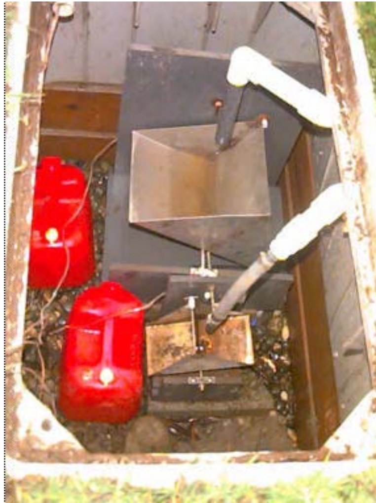
Figure 2-5. Picture of the tipping bucket installation for monitoring surface runoff and subsurface flows at the University of Washington Center for Urban Horticulture
