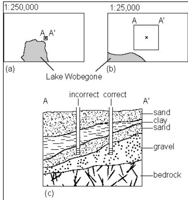
In Exhibit 1.5, X indicates the location of a well with known areal coordinates and depth. On the smaller scale map, (a), precise plotting of the well's location is impossible. The larger scale map, (b), shows the location of X with much greater precision. Cross-section (c) shows a correct identification, based on map (b), of the well's aquifer as gravel (a sensitive aquifer) and an incorrect identification, based on map (a), of the well's aquifer as sand (a non-sensitive aquifer).
