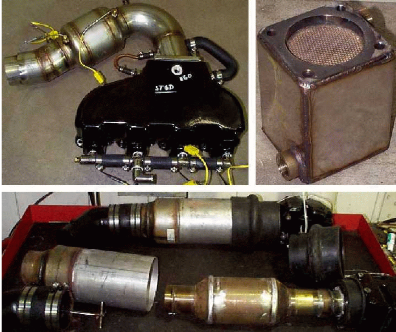
Figure 4.5-1: Three Catalyst Configurations Used in SD/I Test Program
