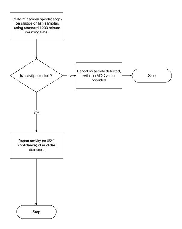
Each laboratory will report the minimum detectable concentration (MDC) for all nuclides of interest which are not detected in a sample. The instrument signal is compared to a critical level (Lc) which is the value of the net signal (e.g., count rate) that has a 5% probability of being exceeded when a blank sample is analyzed. It is used as a threshold value for deciding whether a sample contains the analyte of interest.
