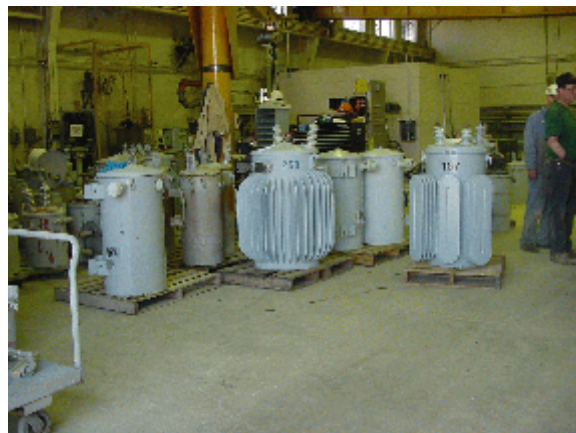
Figure 2-3. PCB Transformers in storage.
