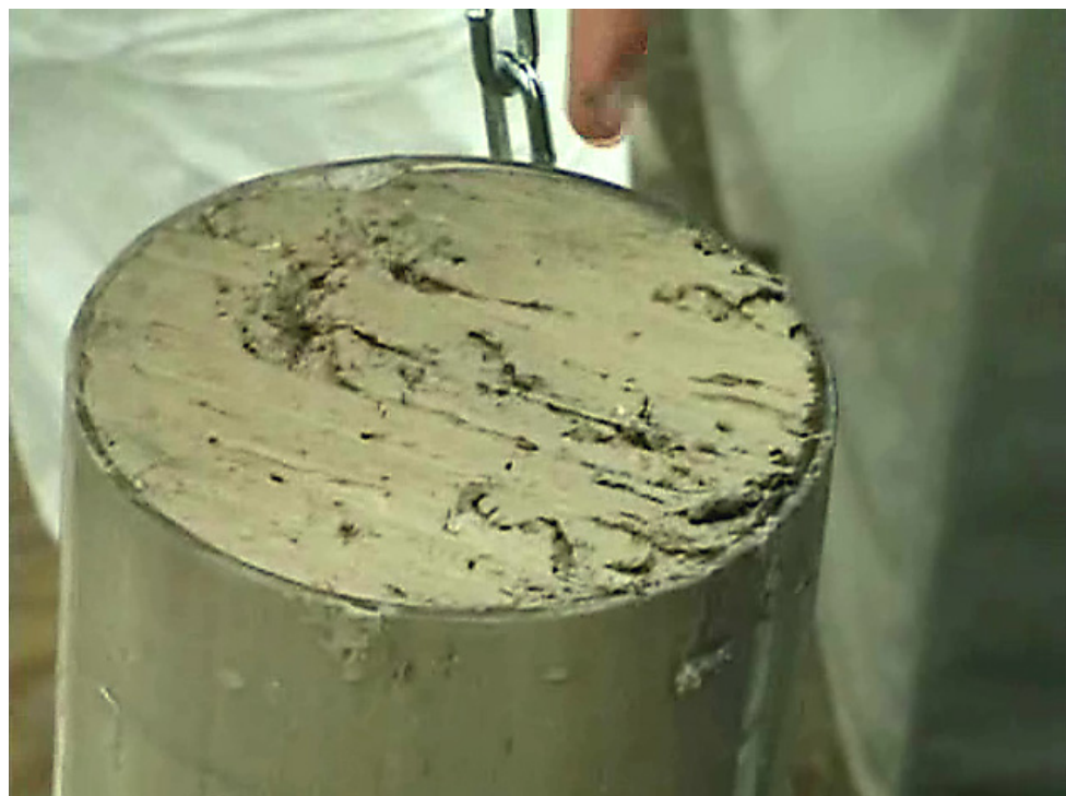
Figure 31. Sediment in Tube after Sub-sampling Surface Layer.
