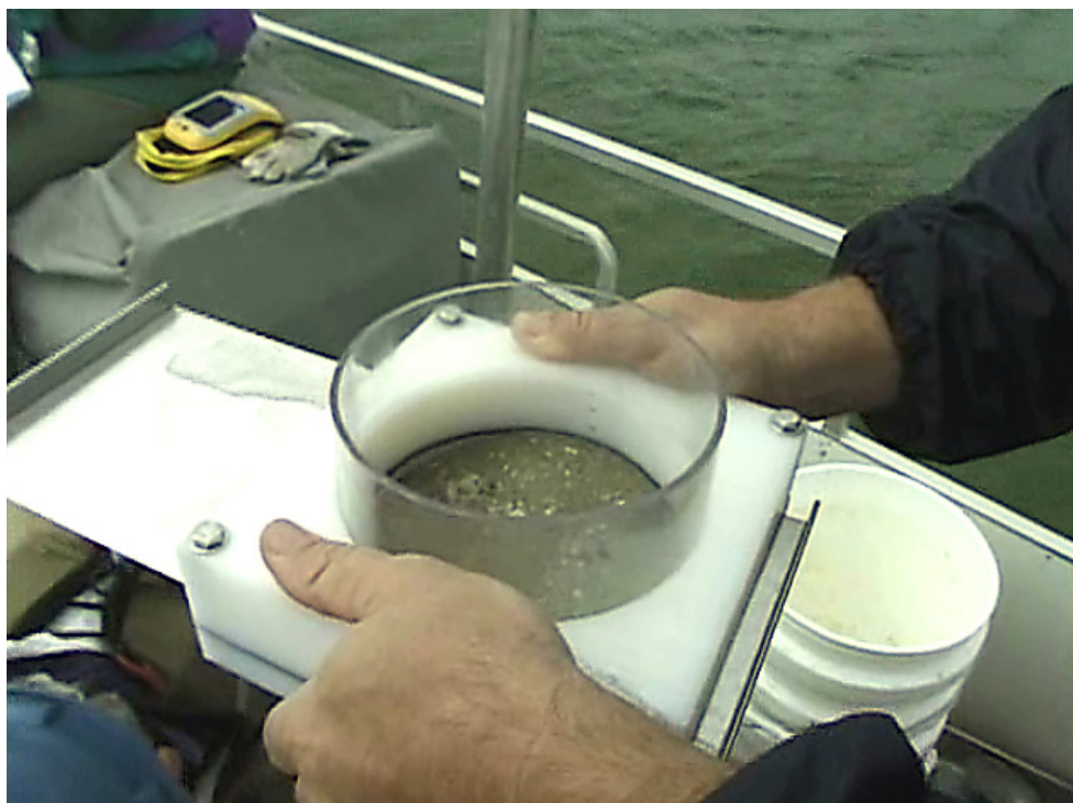
Figure 30. Slicer Block Assembly on Core Tube for Sub-sampling
