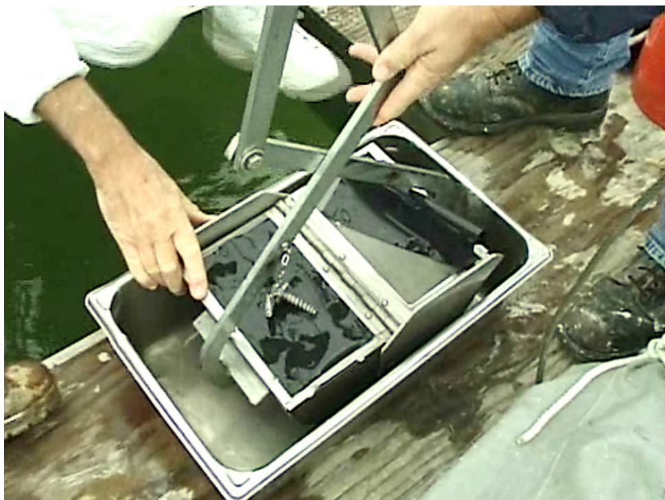
Figure 26. Removal of Sediment from Ponar Sampler
