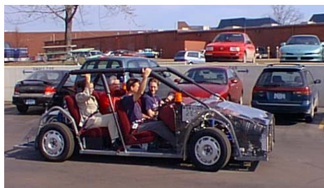
EPA's proof-of-concept test chassis demonstrating hydraulic hybrid technology.
