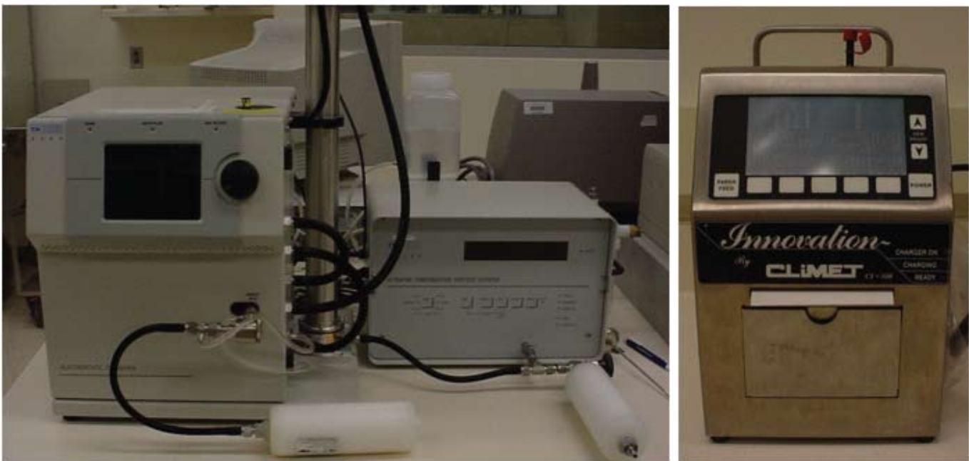
Figure 3-1. Aerosol Sampling Instruments, TSI SMPS (left) and Climet CI-500 (right)
