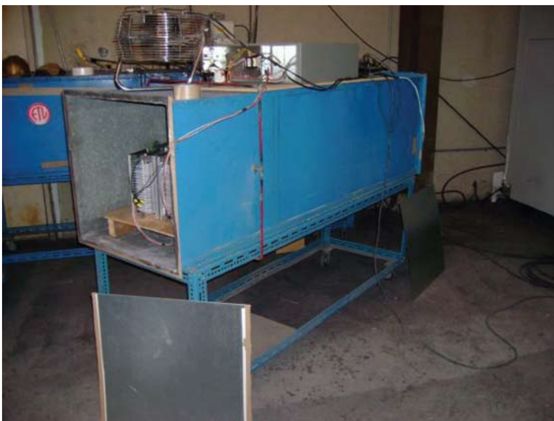
Figure D-5. Photograph (side view) of the Test Fixture Used During the Silicon Vapor Exposures of the Electronic Air Cleaners
