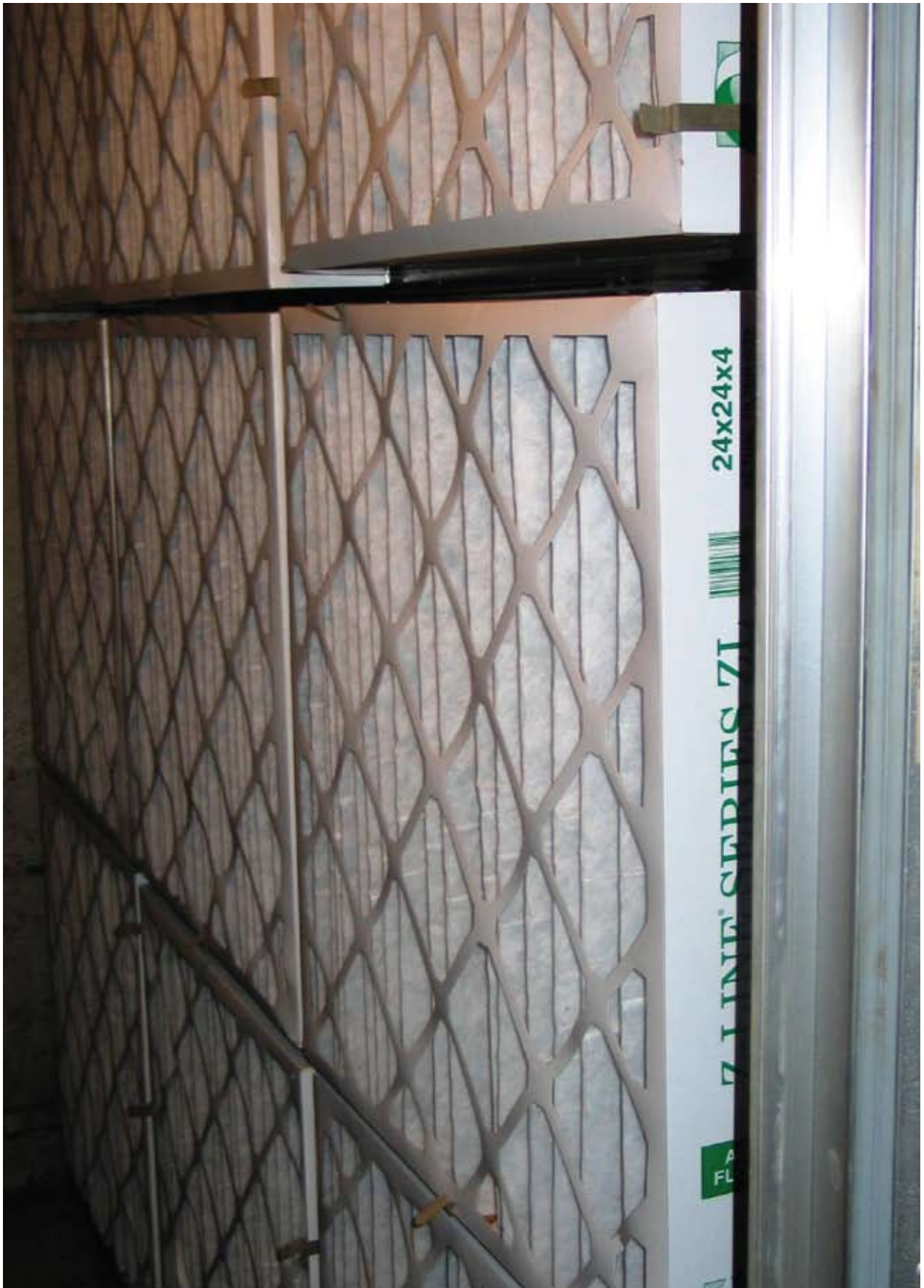
Figure C-6. Photograph of the 9-Filter Commercial HVAC System Used to Age Filters C14PCS and C11GM-16 (The test filters are behind the prefilters.)
