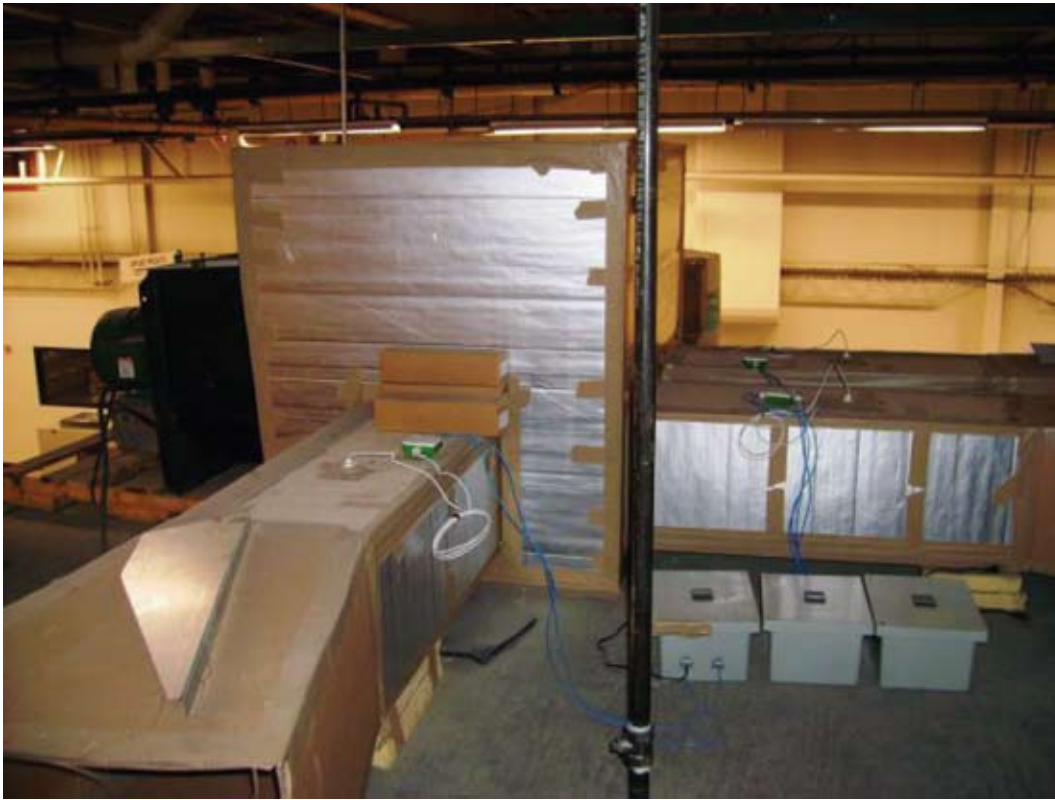
Figure D-8. Photograph of the Upstream Side of the Test Fixture and Airflow Controllers Used During the Ambient Aging of the Electronic Air Cleaners
