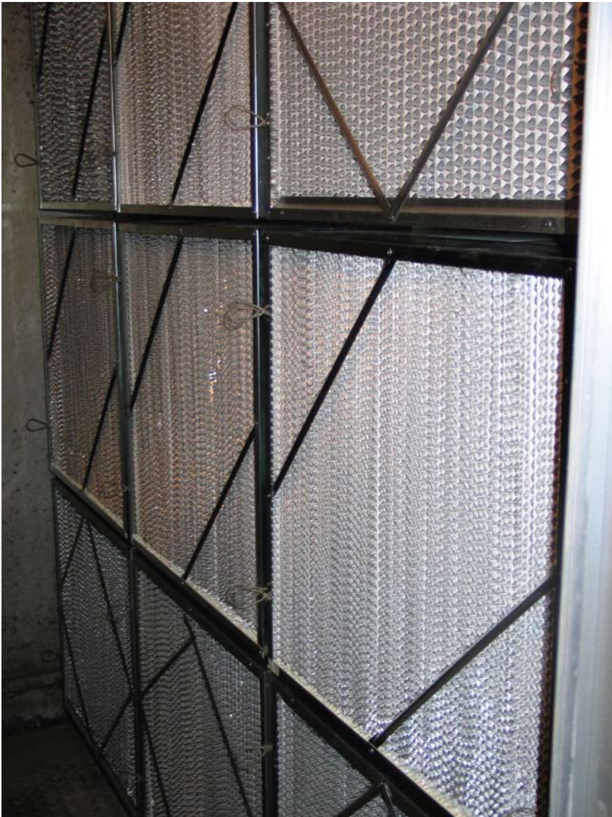
Figure C-5. Photograph of the 9-Filter Commercial HVAC System Used to Age Filters C14PCS and C11GM-16 (The test filters are shown before the prefilters were installed.)
