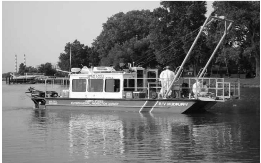
*EPA's research vessel Mudpuppy can enter shallow inlets on the Great Lakes to test for contaminated sediment.*
