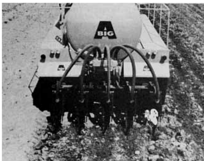
Figure 14-9. Tank truck with liquid sludge tillage injectors (courtesy of Rickel Manufacturing Company).
