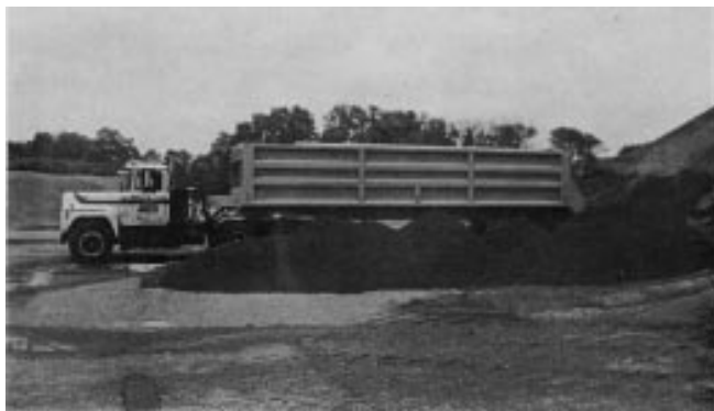
Figure 14-2c. A 25-cubic-yard dewatered sludge haul truck (courtesy of Convento Manufacturing Company).
