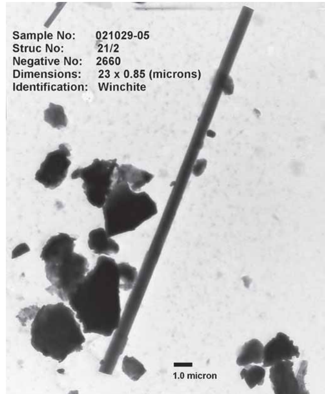
Figure 7. Asbestos Fiber on Air Filter Derived from Soil 12 in Phase II Viewed by TEM
