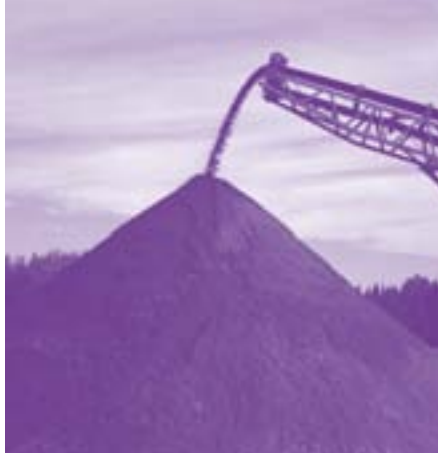
Crushed asphalt on conveyer belt.
