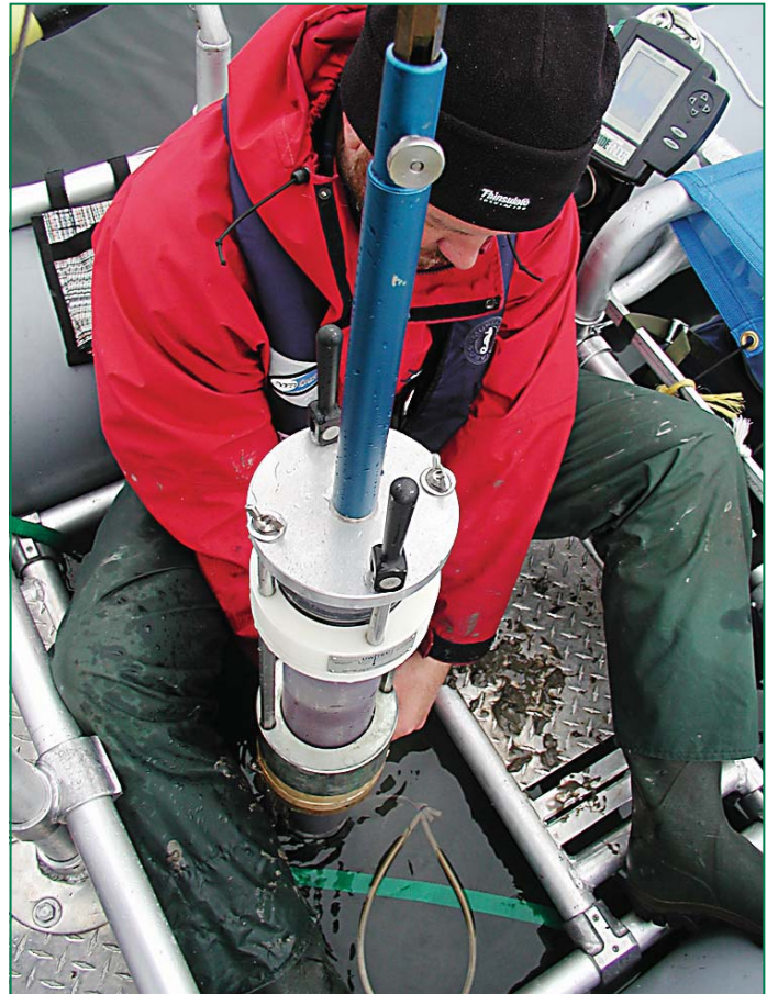
A WACAP researcher operates the lake sediment sampler.
