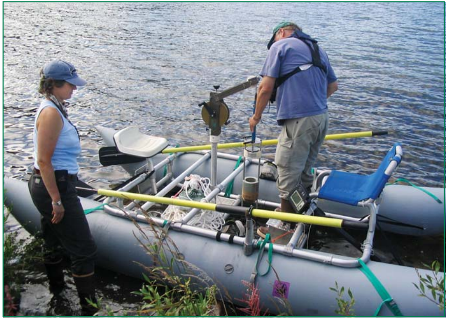
A special inflatable raft is used for the sediment coring device, shown being prepared by Dr. Dixon Landers.
