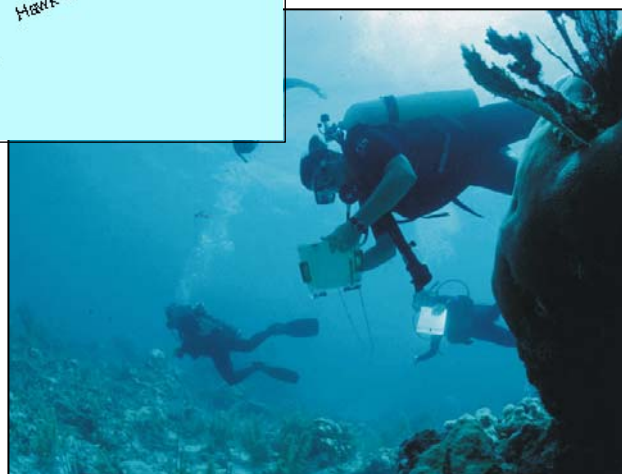
Figure 12-5. Using SCUBA, surveyors count and identify each colony in a 113m 2 radial belt transect and examine each for evidence of bleaching and disease.
