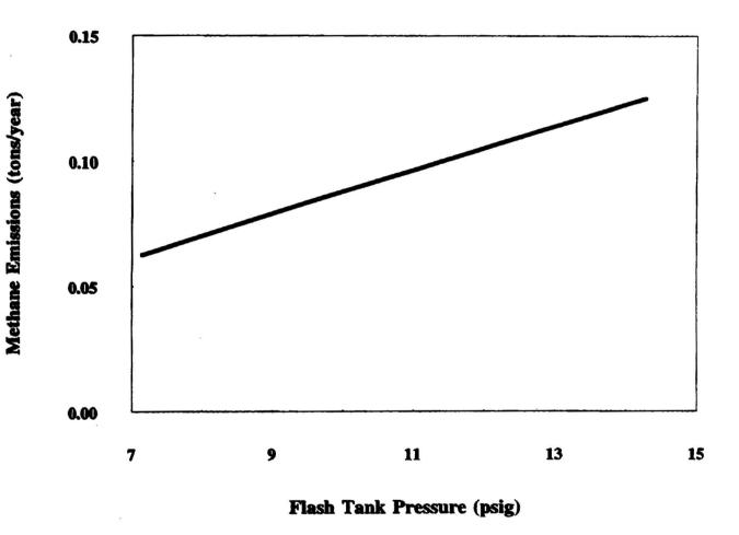
Figure 5-3. Methane Emissions - Glycol Regenerator Effect on Flash Tank Pressure
