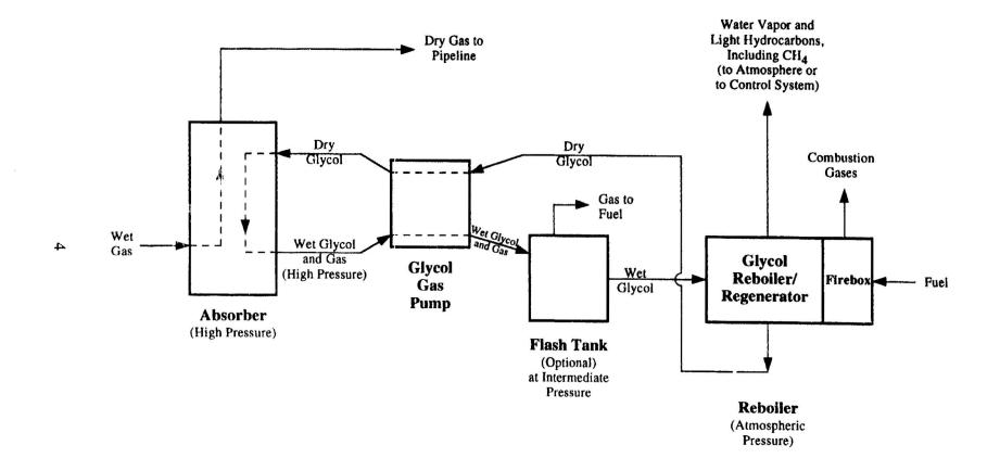
Figure 3-1. Block Process Flow Diagram of a Typical Glycol Dehydrator
