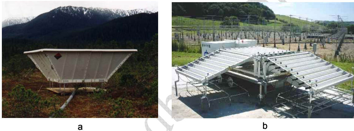
Figure 8.7 Photographs of Several Types of Radar Wind Profilers: (a) Phased-Array System and (b) Fixed-Axis Antenna System
