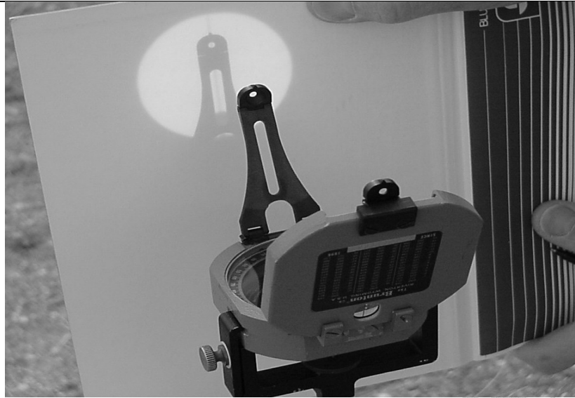
Figure 2.14 Projection of Sun's Reflection Using a Brunton Pocket Transit
