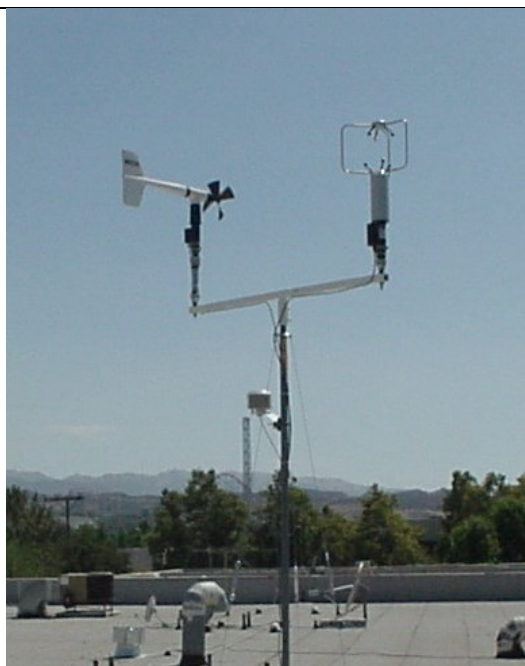
Figure 2.16 Sensor Mounting for the Testing and Evaluation of the Audit Wind Sensor Against a Sonic Anemometer
