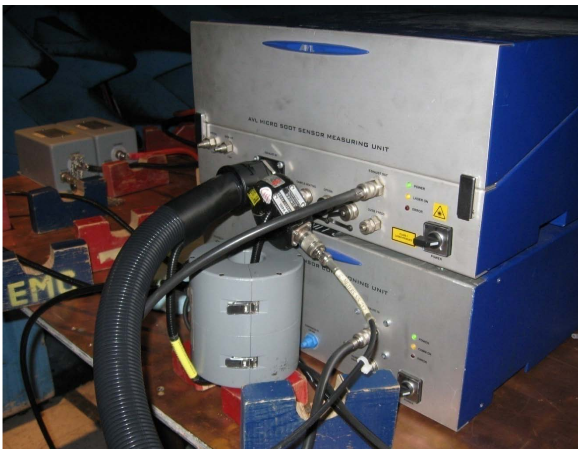
FIGURE 111. AVL SETUP DURING BULK CURRENT INJECTION TESTING
