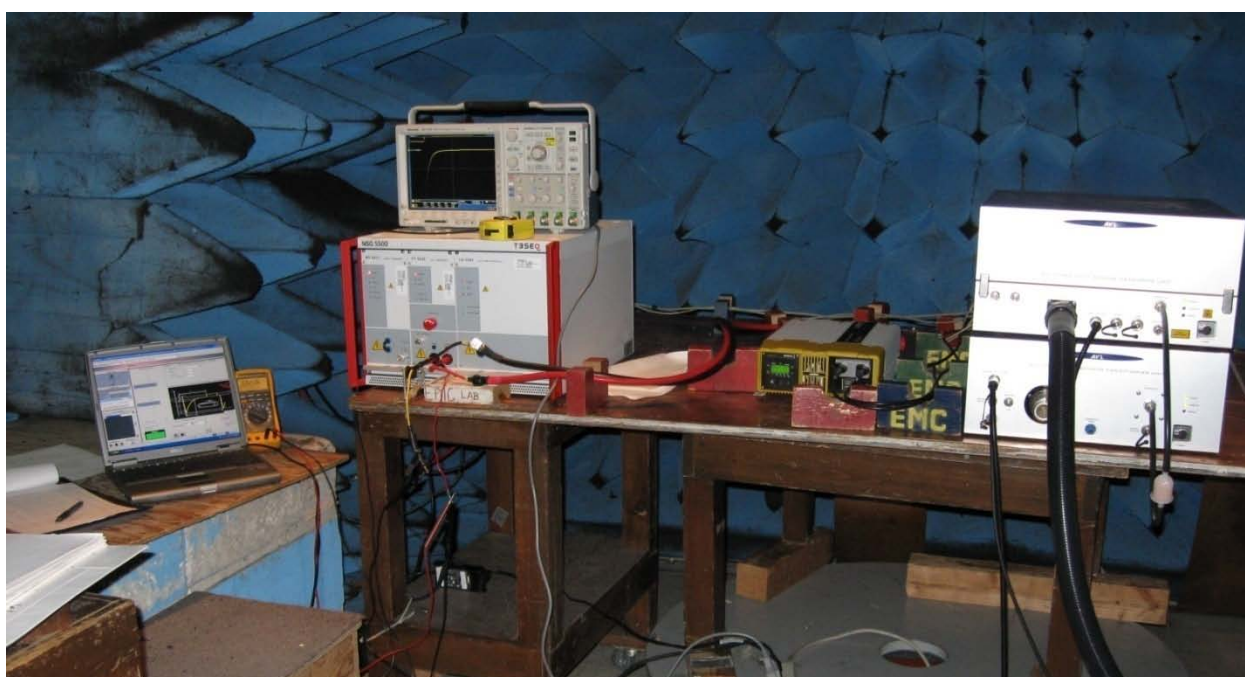
FIGURE 121. AVL SETUP DURING CONDUCTED TRANSIENTS TESTING
