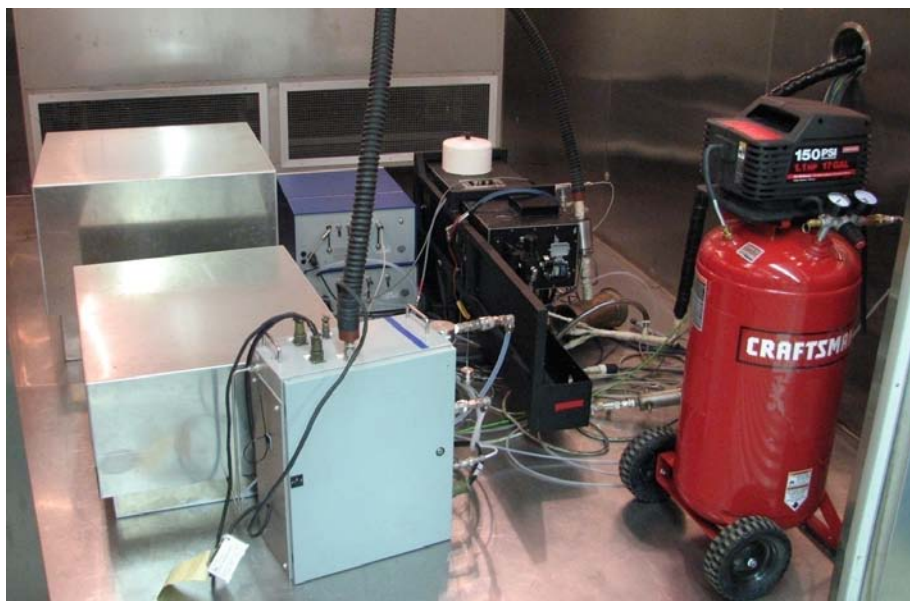
FIGURE 97. PEMS INSTALLED IN THE TEMPERATURE AND HUMIDITY CHAMBER
