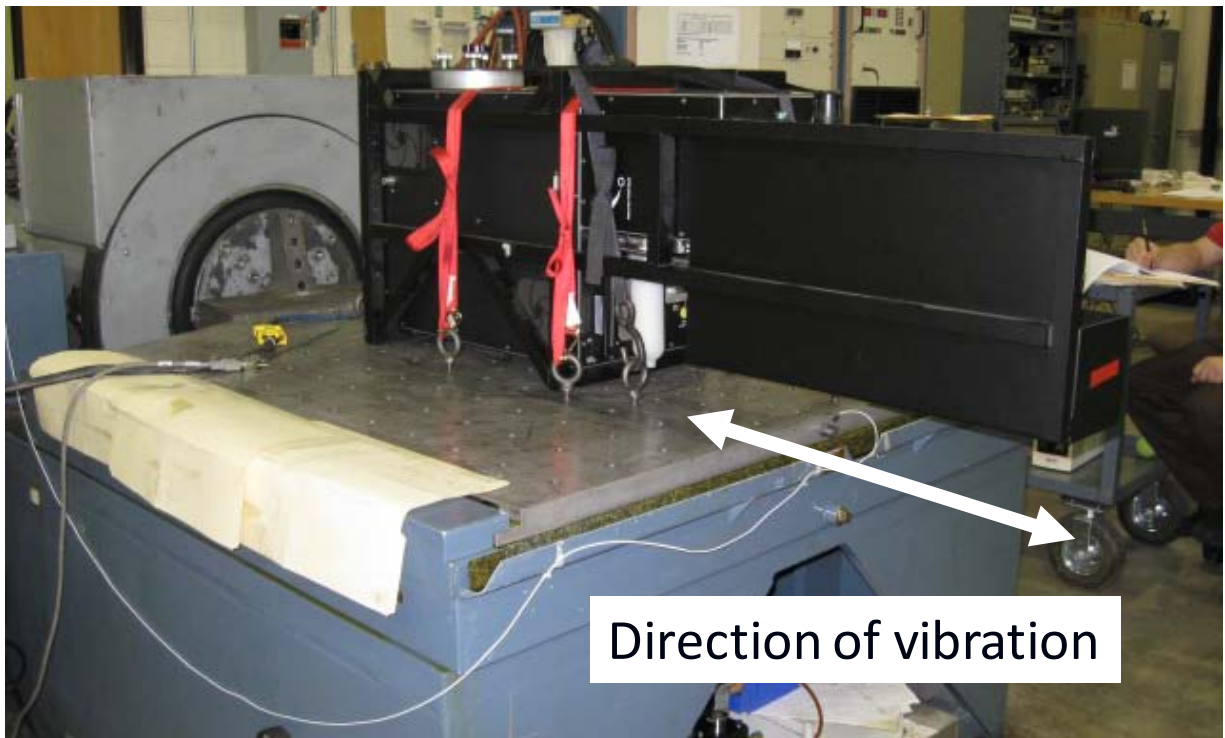
FIGURE 123. SENSORS PEMS MOUNTED FOR LONGITUDINAL HORIZONTAL VIBRATION
