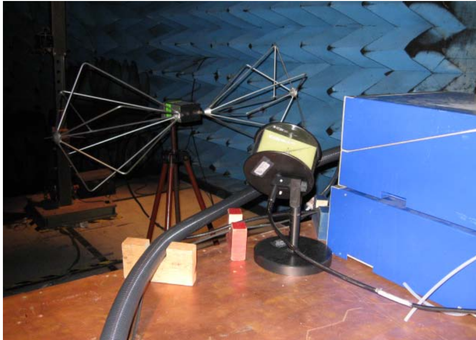
FIGURE 117. AVL PEMS SETUP DURING RADIATED IMMUNITY TESTING
