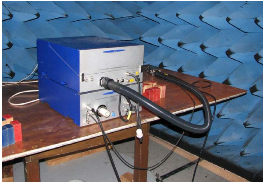
FIGURE 107. AVL PEMS IN THE RADIATION CHAMBER FOR EMI AND RFI TESTING
