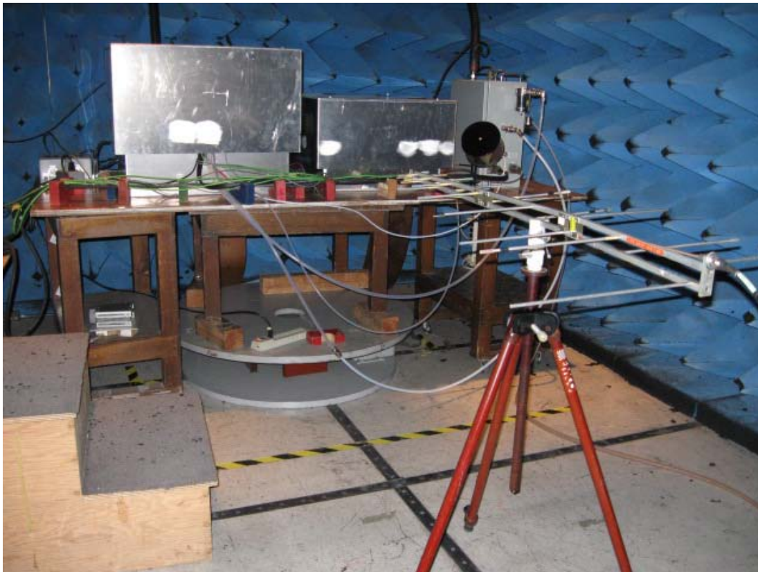
FIGURE 115. HORIBA PEMS SETUP DURING RADIATED IMMUNITY TESTING
