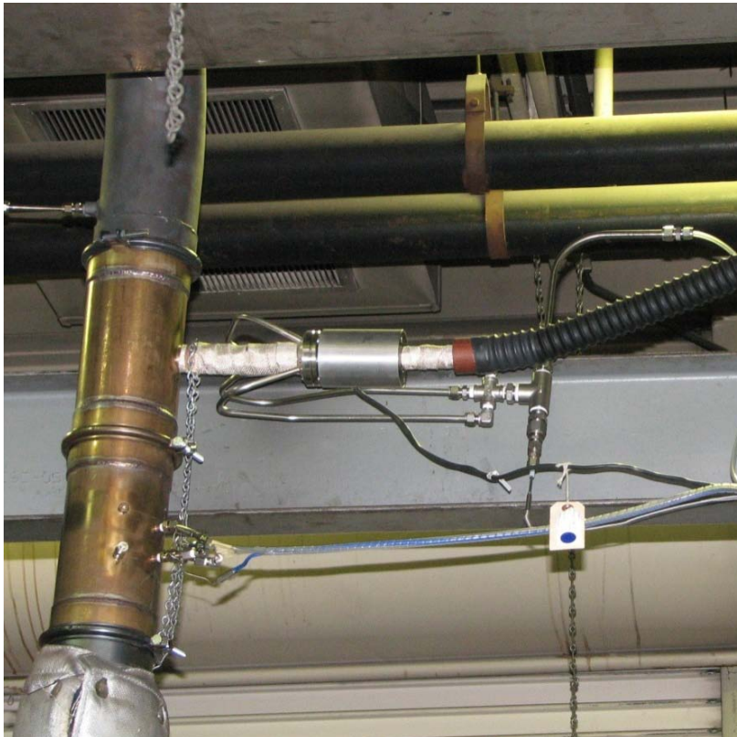
FIGURE 21. THE PROBE AND TPA FOR THE HORIBA OBS-TRPM
