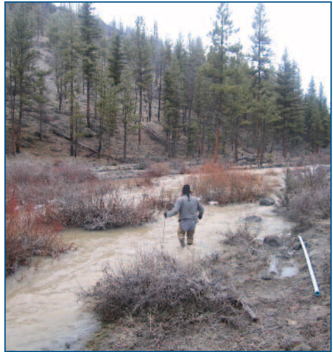
Roland Kalama CTWS water technician removing a data sonde from Coyote Creek during a flash event that moves large amounts of sediment downstream into Beaver Creek. This is an area that is highly disturbed from legacy forestry prescriptions and a large wildfire in 2007. Photo by Brenda Sanchez
