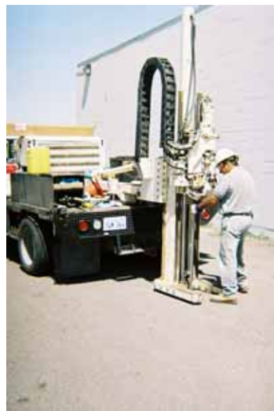
Figure 3-2. Large Direct-Push Rig
