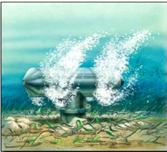
Figure 7-17. Cylindrical Wedgewire Screen with Air Sparging (Johnson Screens)
