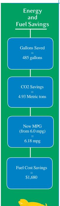
Synthetic lubricants in the engine crankcase, rear axle, and transmission can improve fuel economy by about 3 percent, saving nearly 485 gallons of fuel and eliminating 5 metric tons of greenhouse gas emissions for a typical combination truck each year.
