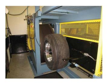
Rolling resistance is measured on a specialized road wheel in a controlled laboratory setting. Target values for SmartWay-verified tires are based on laboratory tests and modelling simulations. *Photo courtesy of Smithers Scientific's Rayenna Laboratory*
