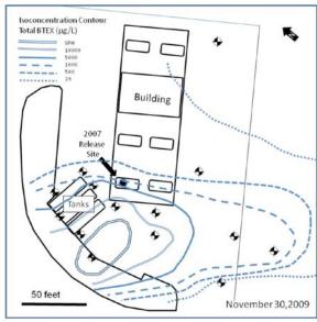
FIGURES 2A, 2B, 2C. Site diagrams show plume size prior to 2007 release, shortly after discovery of 2007 release, and more than two years after 2007 release. Note increasing size of plume and area of separate-phase hydrocarbons.
