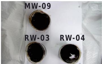
**FIGURE 3.** Top: Light-colored LNAPL from tank field wells (2007 release); Bottom: Dark, weathered product from source zone wells (1988 release).
