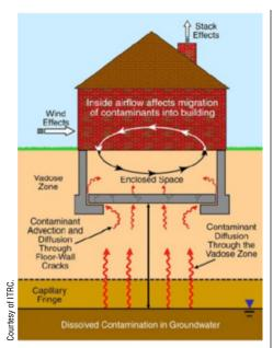
FIGURE 2. Vapor intrusion cross-section.
