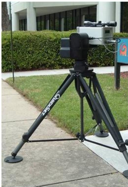
**Figure 1-5. Scanning Boreal Laser GasFinder 2.0 System**
