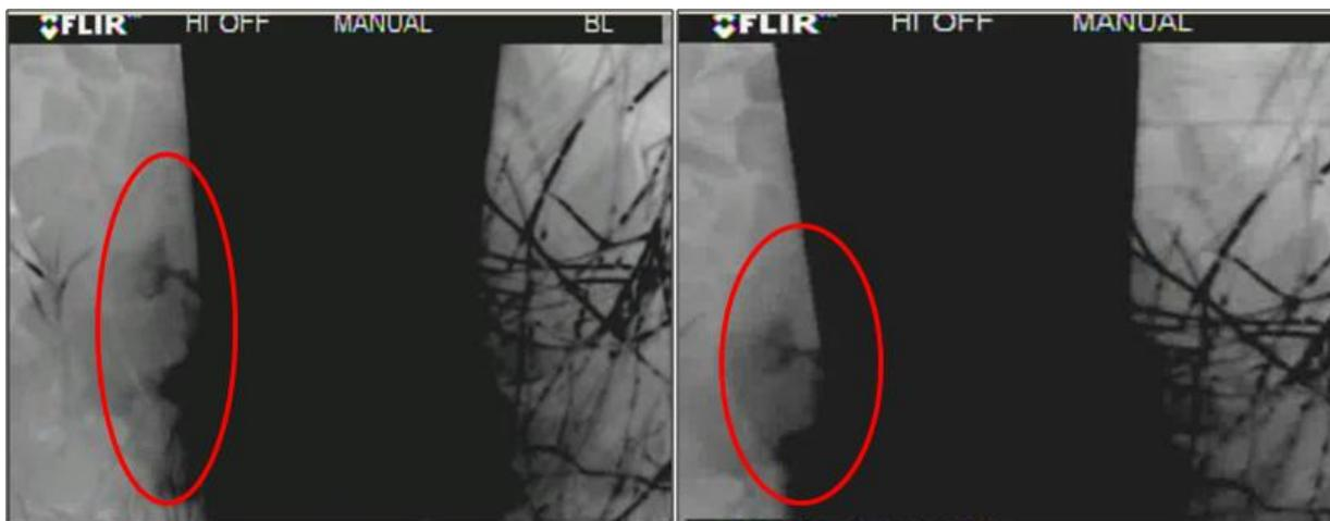
**Figure 3-8. Additional Screenshots from FLIR Camera of Fugitive Leaks from Base of Gas Wells at Site A.**
