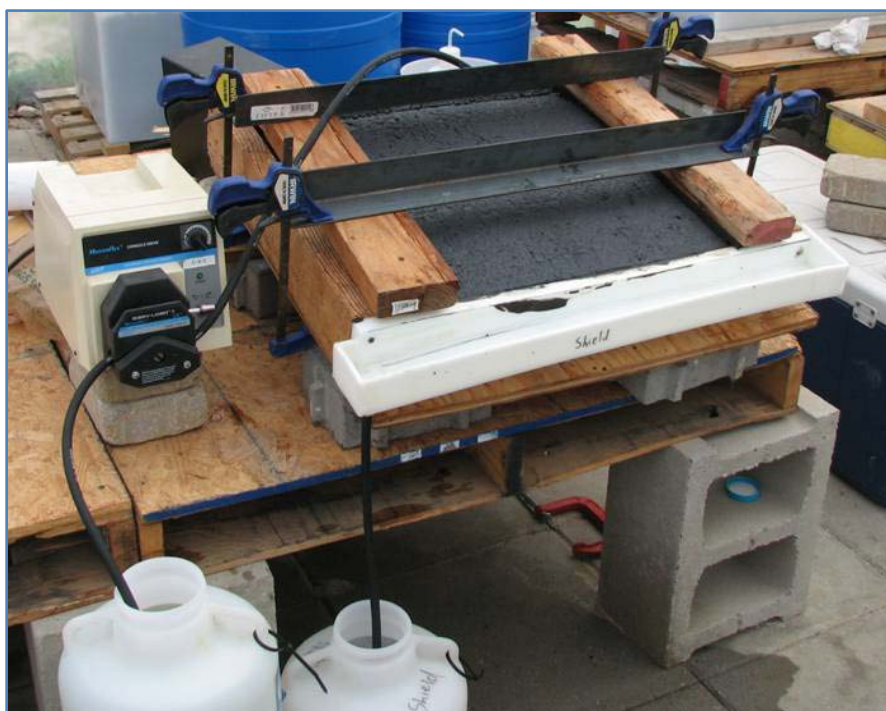
Figure 3. Sealed asphalt panel with rainwater delivery apparatus, angled to promote runoff.
