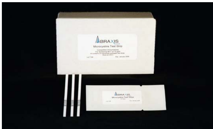
Figure 2. Microcystin Strip Test
