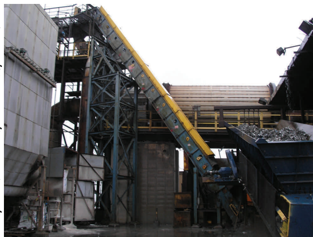
Scrap being loaded into one of the two scrap dryers at Spectro Alloys
