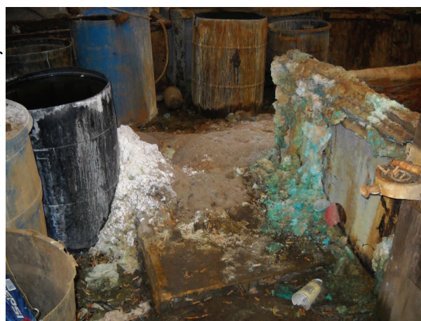
Vats, caustics and precipitate. Note the “drag out” from years of electroplating. Hazardous waste from the business had never been properly disposed of by the defendant, despite operating the company for over 14 years.
