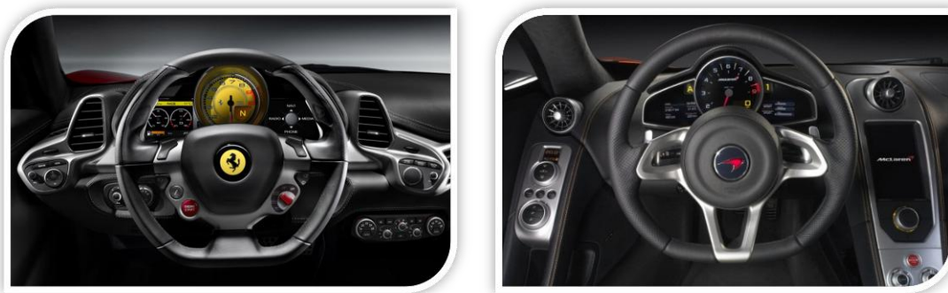
Image F.5-32: VFT Airbag used in Ferrari 458 Italia (left) and McLaren MP4-12C (right)
