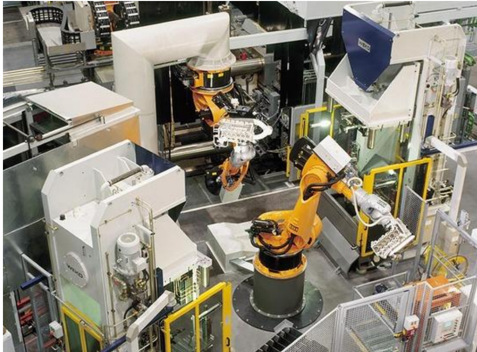
Image F.2-25: Die Casting - Aluminum Cylinder Insert
