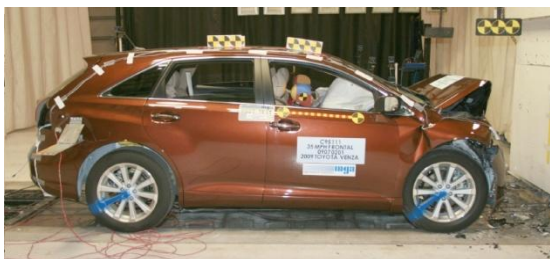
Figure D.3-26: Deformation Mode Comparison: Left Side View @ 80msec
