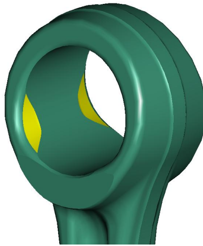
Image F.2-16: Forged In Oil Pockets (Lightweighted)
