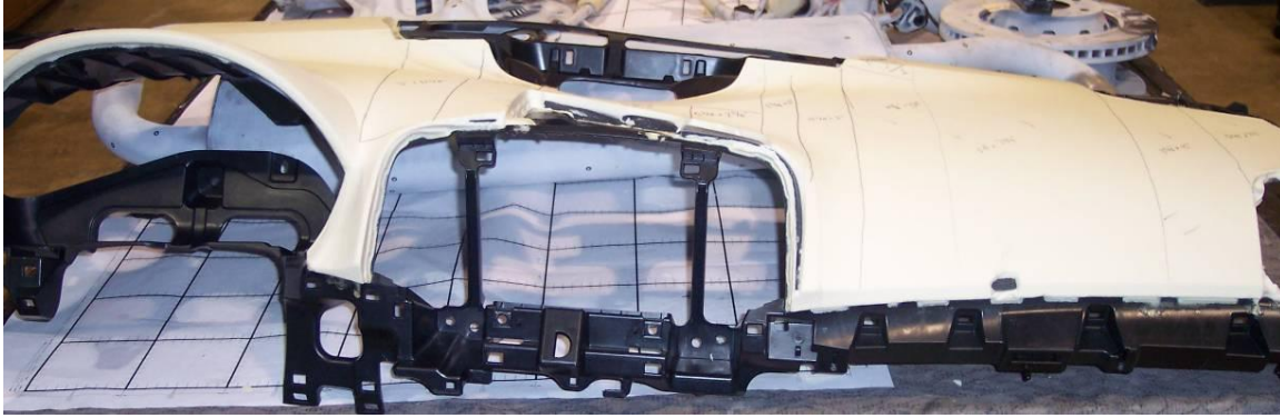
Image F.5-24: Dash, IP Base with Skin Cover Removed
