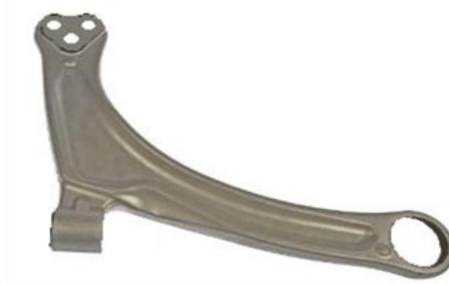
Image F.9-22: Front Control Arm Mass Reduced Component Example
