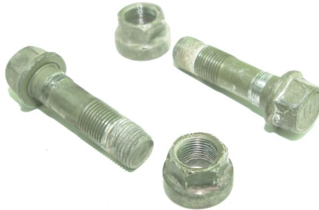
Image F.9-76: Rear & Front Mount Fasteners Mass Reduced Component Examples
