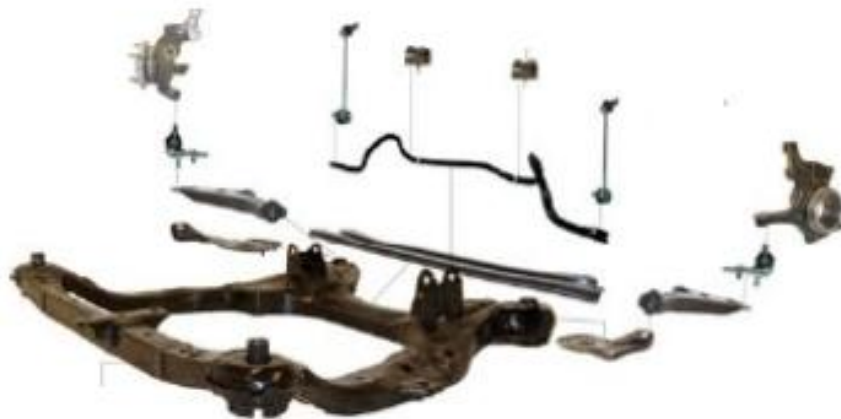
Image F.9-1: Front Suspension Subsystem Relative Location Diagram
