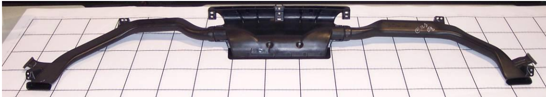
Image F.16-9: Toyota Venza's Defroster Duct Assembly Including Two Center Manifolds and Two Side Ducts
