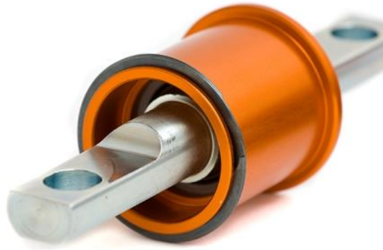
Image F.9-23: Front Control Arm Mounting Shaft Mass Reduced Example
