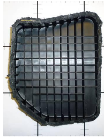
Image F.2-57: Air Intake Cover MuCell – 9% Mass Savings
