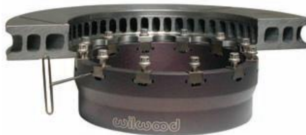
Image F.11-10: Front Rotor Mass Reduced Component
