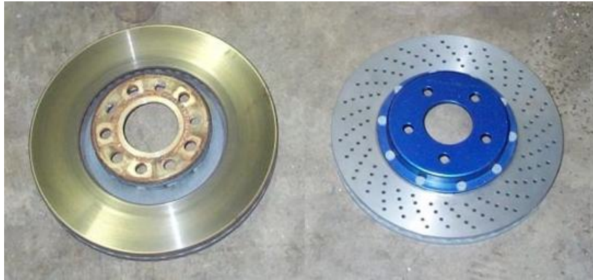
Image F.11-16: Front Rotor Size Normalization Mass Reduced Component
