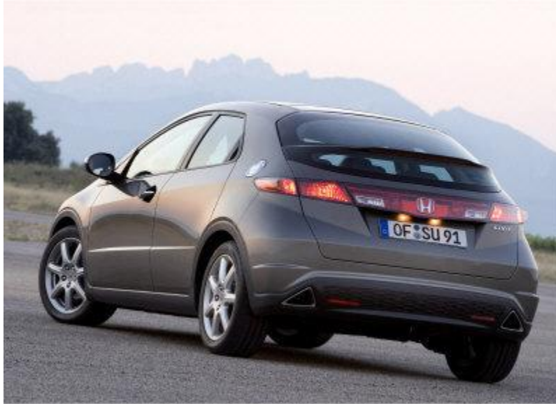
Image F.7-3: European Honda Civic Backlight/Spoiler Integration through Use of Polycarbonate
