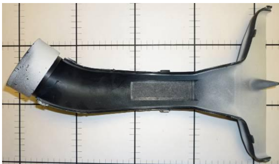
Image F.2-60: Air Intake Duct MuCell - 9% Mass Savings
