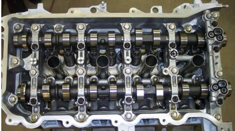
Image F.2-34: Valvetrain Assembly (Phasers removed)
