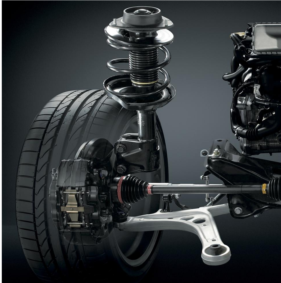
Image F.9-17: Front Suspension Rotor Mass Reduced System Example
