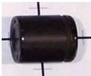
Image F.11-54: Rear Caliper Piston Mass Reduced Component
