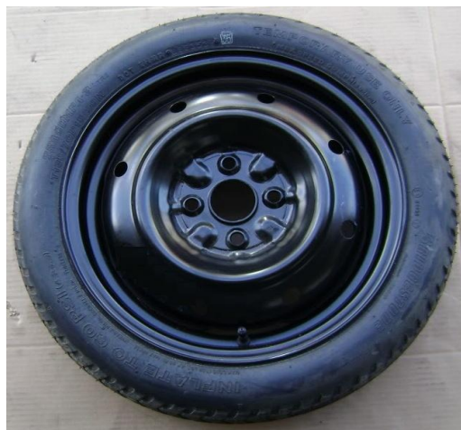
Image F.9-86: Spare Wheel & Tire Current Assembly Example
