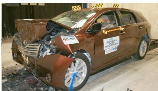
Figure D.3-28: Deformation Mode Comparison: ISO View @ 80msec
