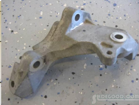
Image F.2-82: [New Technology] AC Comp Bracket (Nissan 350z)
