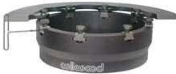
Image F.11-38: Rear Rotor Mass Reduced Component
