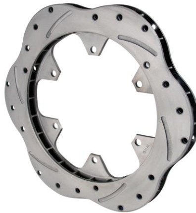
Image F.11-17: Front Rotor Mass Reduced Component
