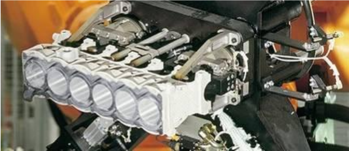
Image F.2-23: Aluminum Cylinder Insert with Integrated Water Jacket and Bulkheads
