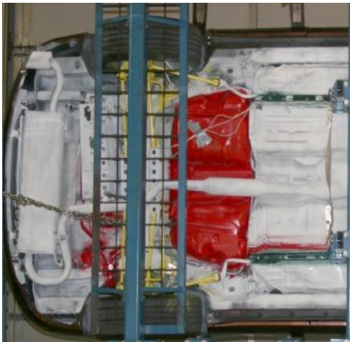
Figure D.3-29: Deformation Mode Comparison: Bottom View Front Area @80msec
