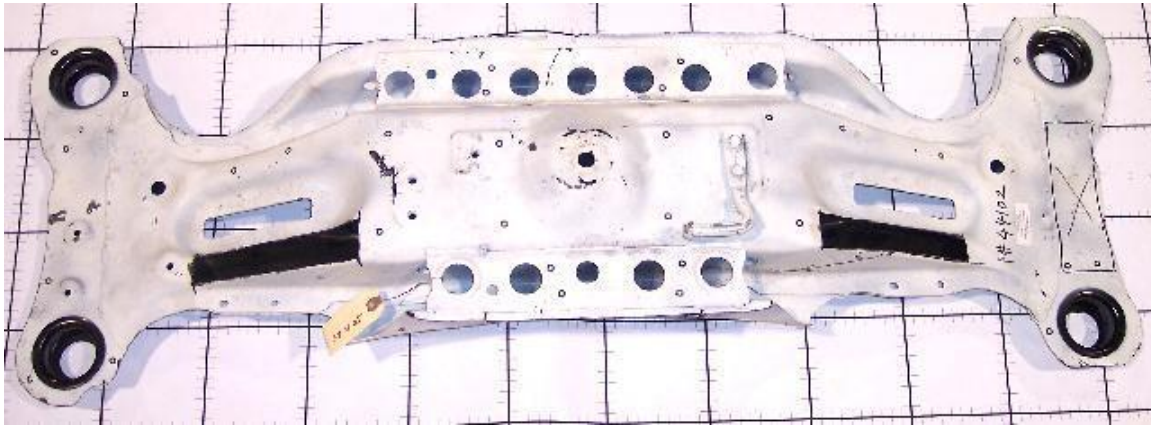
Image F.12-15: Rear Frame Assembly
