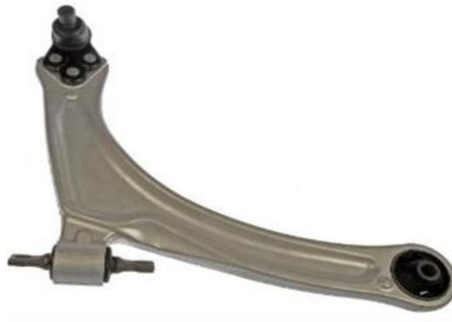
Image F.9-18: Front Control Arm Mass Reduced Assembly Example
