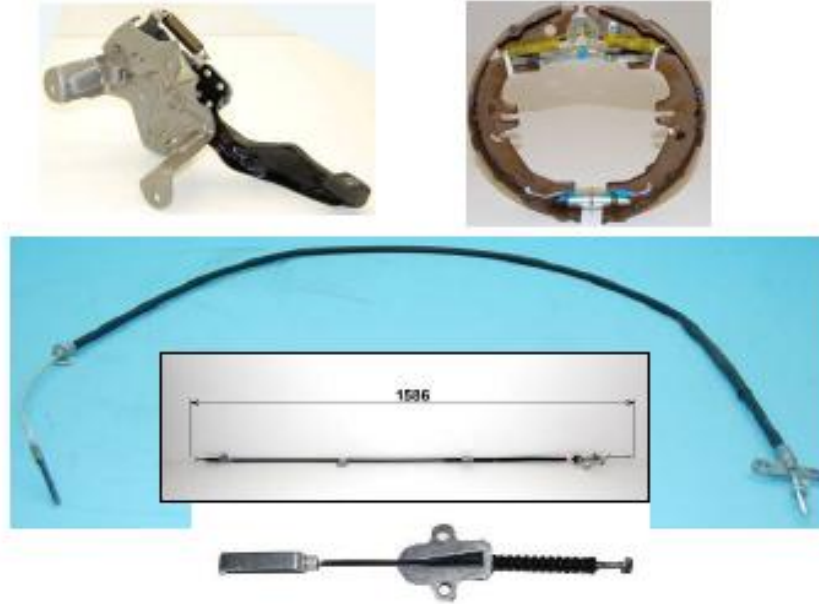
Image F.11-57: Parking Brake and Actuation Subsystem Current Sub-assemblies
