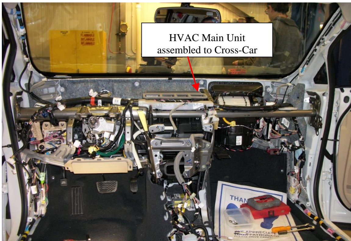
Image F.16-3: Toyota Venza Instrument Panel with Interior Trim Removed
