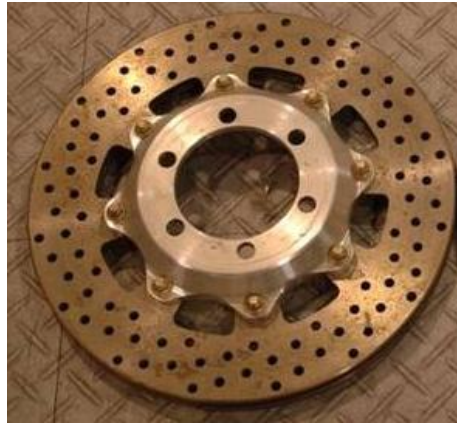
Image F.11-18: Front Rotor Mass Reduced Component
