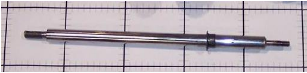
Image F.9-61: Rear & Front Strut Piston Shaft Current Component Example
