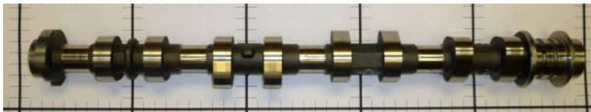
Image F.2-38: [Base Technology] Solid Cast Camshaft
