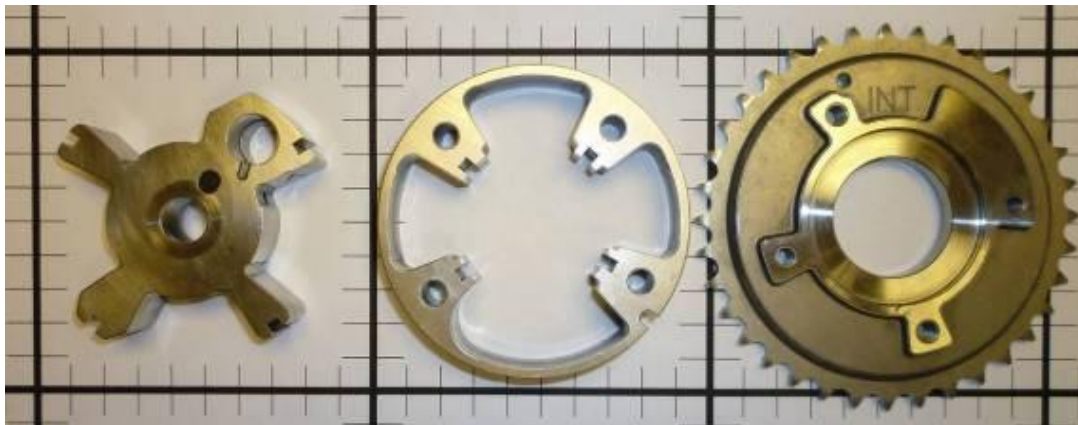
Image F.2-40: [Base Technology] Sintered Iron Cam Phaser Rotor, Stator, Sprocket
