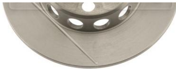
Image F.11-46: Rear Rotor Mass Reduced Component
