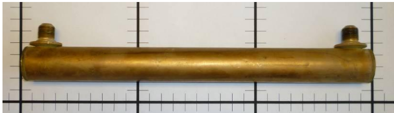
Image F.2-74: Transmission Heat Transfer Element – Copper Alloy
