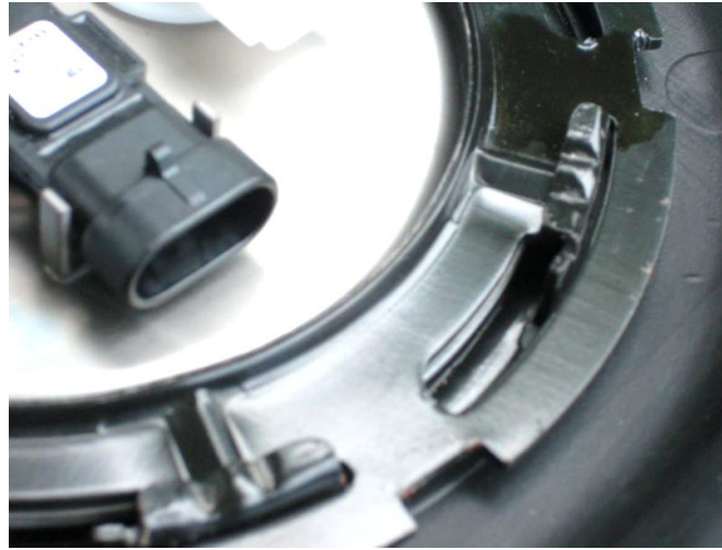
Image F.14-13: Fuel Pump Retaining Bracket “Twist Lock” Design
