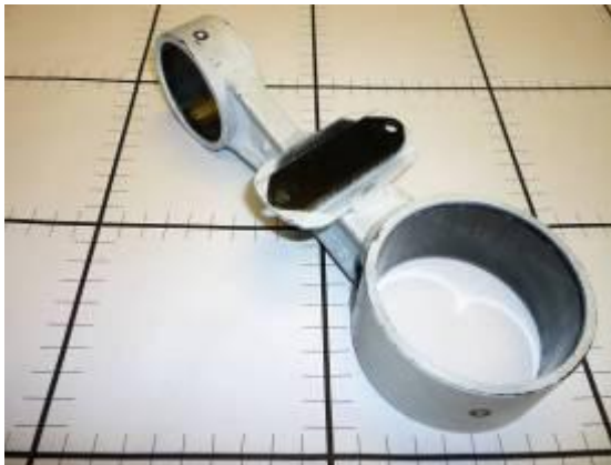
Image F.2-7: Torsion Strut Link
