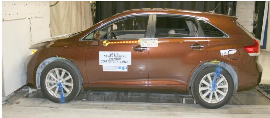
Image D.3-5: FMVSS 208 35 MPH Flat Frontal Crash Test Setup
