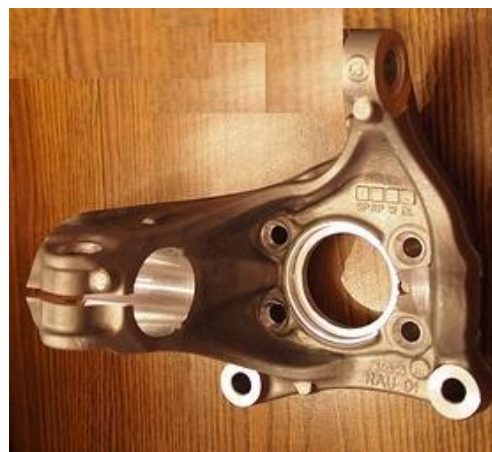
Image F.9-46 (Left): Rear Carrier Alfa Romeo (Source: Lotus – 2010 March EPA Report)
