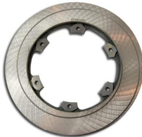
Image F.11-40: Rear Rotor Mass Reduced Component
