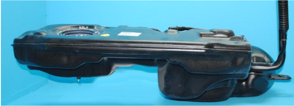
Image F.14-11: Plastic (HDPE) Fuel Tank
