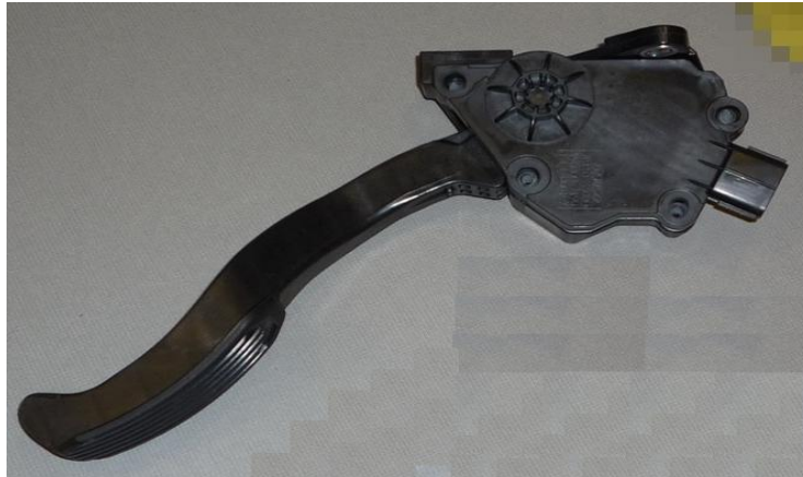
Image F.11-79: Accelerator Pedal Actuator Mass Reduced Sub-assembly Example
