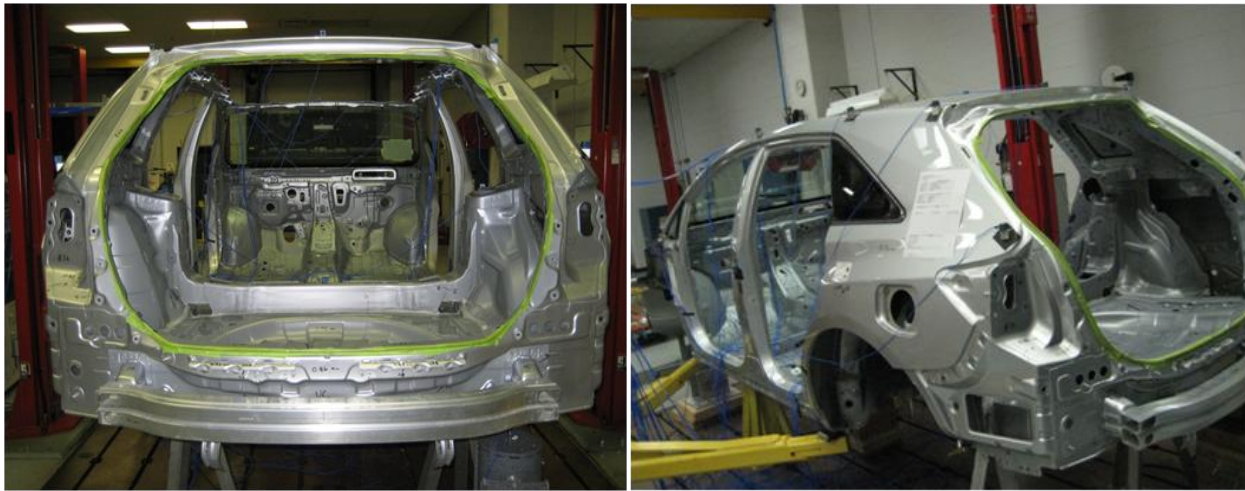
Image D.3-3: Dynamic Modal Test Setup
