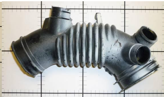
Image F.2-59 : Main Intake Hose MuCell - 9% Mass Savings
