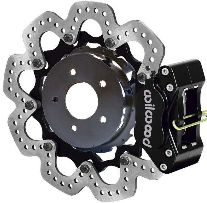
Image F.11-56: Rear Brake System Mass Reduced Assembly Example
