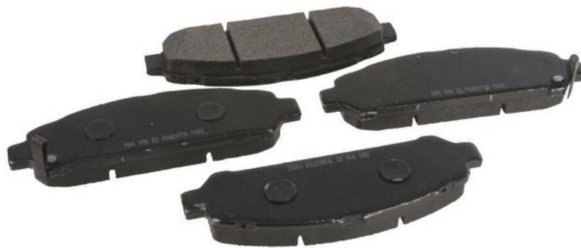
Image F.11-26: Front Caliper Brake Pad Mass Reduced Components
