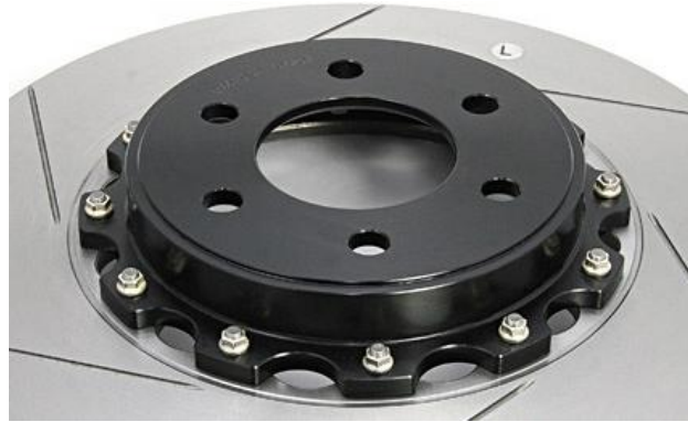
Image F.11-39: Rear Rotor Mass Reduced Component
