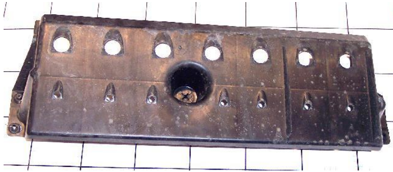
Image F.14-22: Vapor Canister Cover
