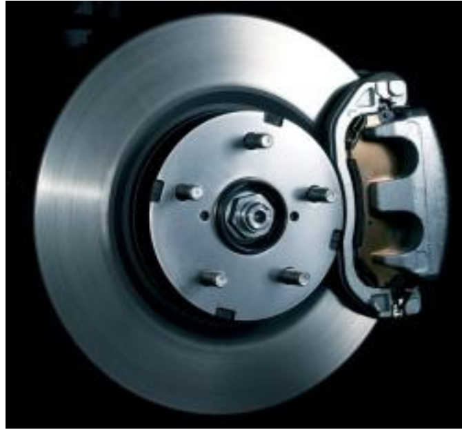
Image F.11-30: Rear Brake System Assembly Example
