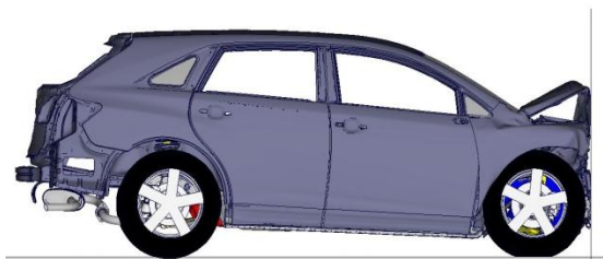
Figure D.3-26: Deformation Mode Comparison: Left Side View @ 80msec
