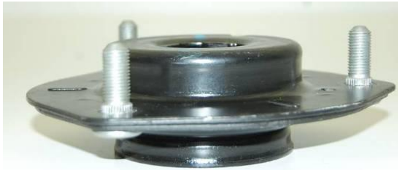
Image F.9-70: Front Strut Top Mount Current Sub-Assembly Example
