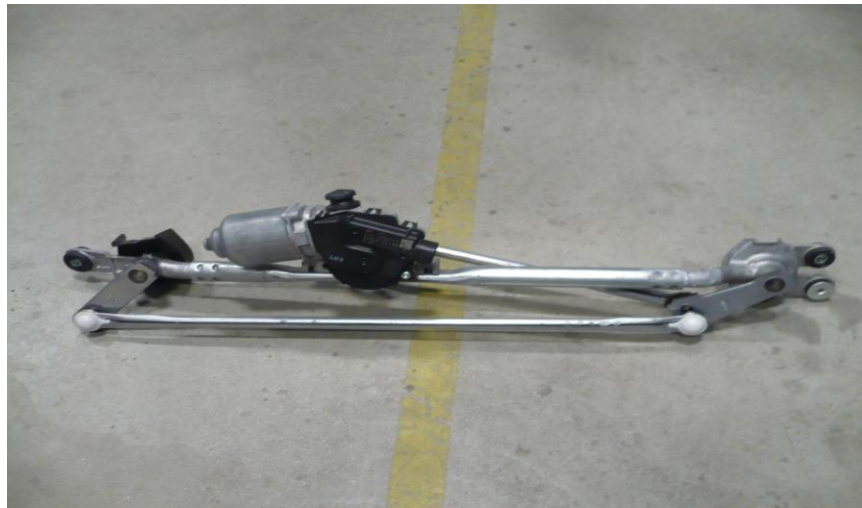
Image F.7-7: Front Wiper Assembly
