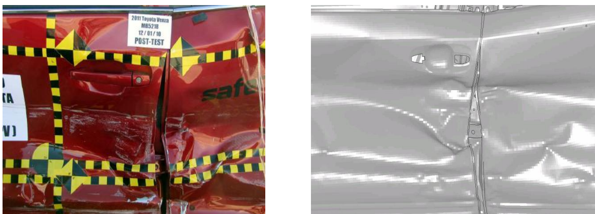
Figure D.3-40: Doors Deformation Mode Comparison
