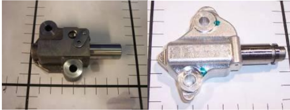
Image F.2-48: [Base Technology] Tensioner Housing – Cast Iron (Source: FEV, Inc. photo)
