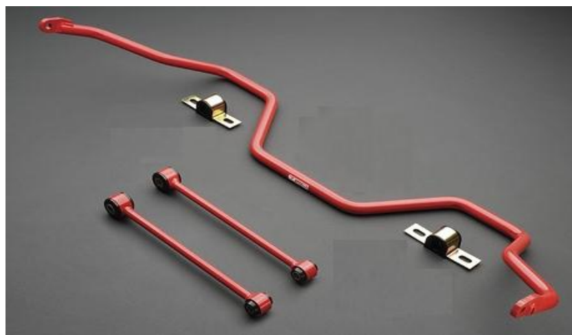
Image F.9-49: Stabilizer Bar System Mass Reduced System Example
