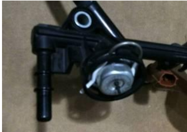
Image F.2-64: Fuel Rail with Integrated Pulsation Dampener
