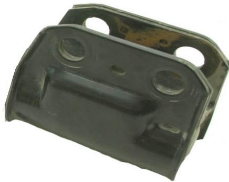
Image F.9-62: Rear & Front Strut Lower Mount Current Component Example
