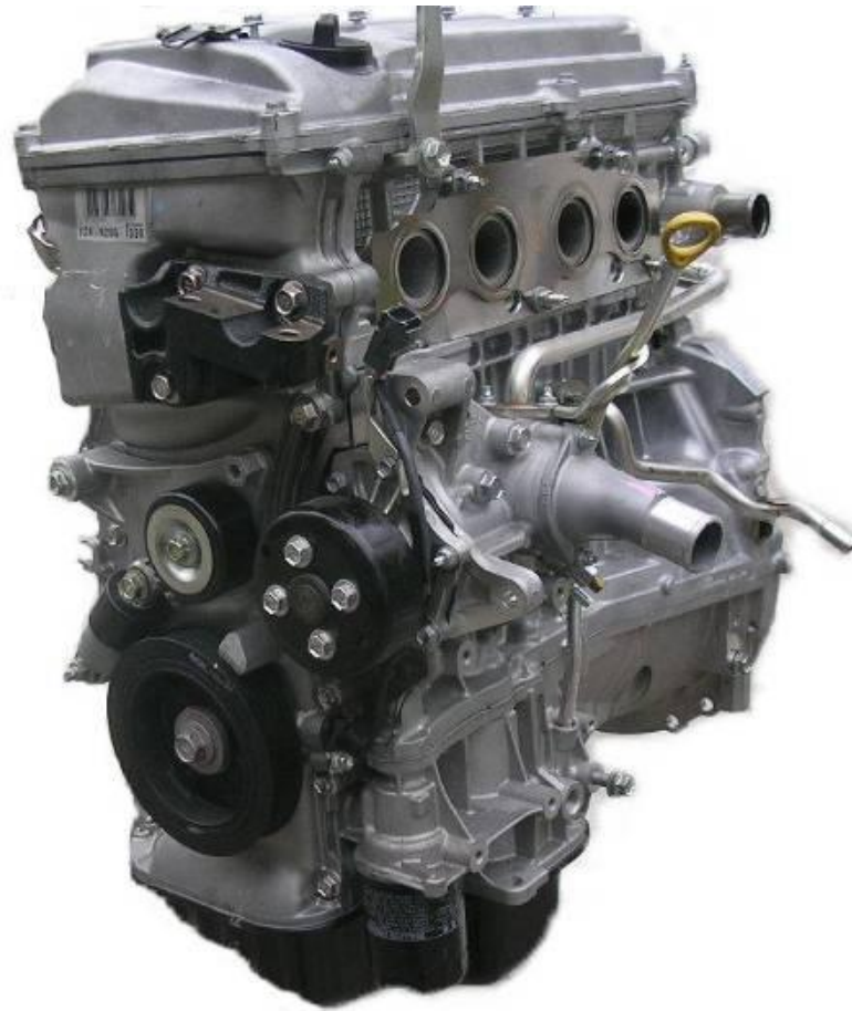
Image F.2-2: Engine Downsize Selection (Toyota 2.4L 2AZ-FE)
