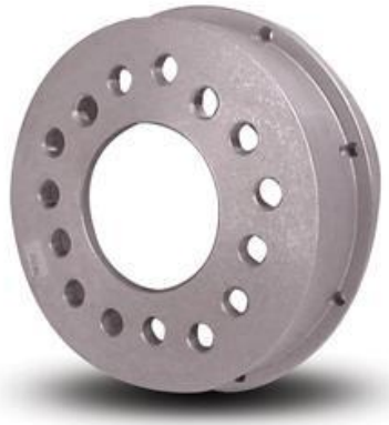
Image F.11-20: Front Rotor Mass Reduced Component
