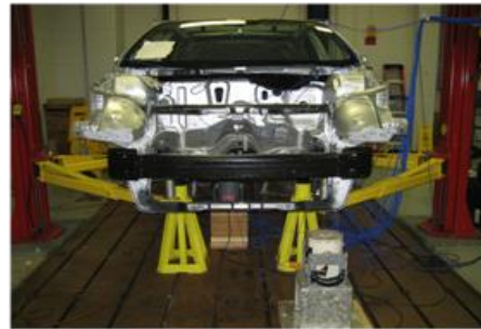
Image D.3-2: Torsion Stiffness Testing Setup
