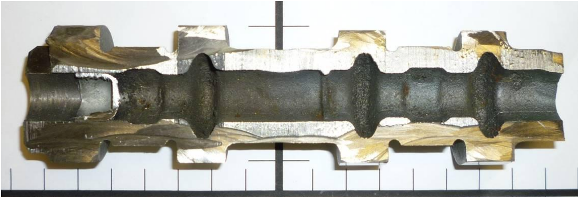
Image F.2-35: Hollow Cast Camshaft – 1.4L Ecotec
