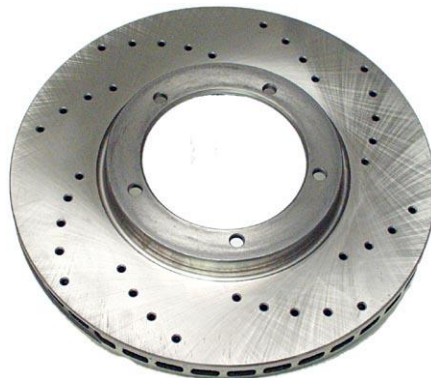
Image F.11-42: Rear Rotor Mass Reduced Component
