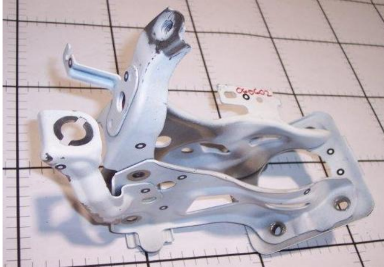
Image F.11-70: Brake Pedal Arm Frame Current Sub-assembly
