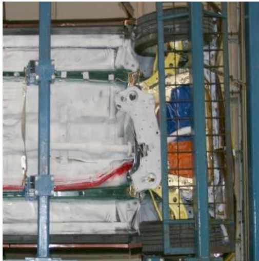
Figure D.3-29: Deformation Mode Comparison: Bottom View Front Area @80msec
