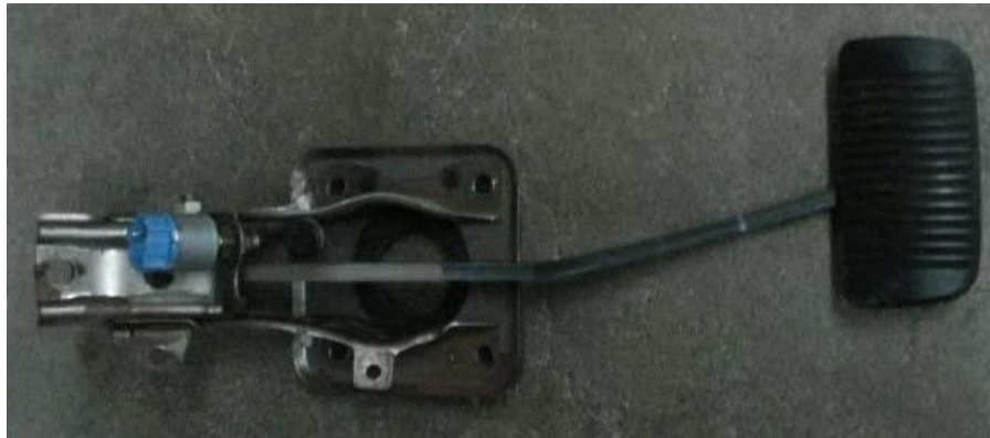
Image F.11-69: Brake Pedal Actuator Current Sub-assembly
