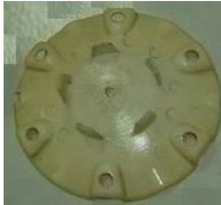
Image F.11-93: Vacuum Booster Diaphragm Backing Plate Mass Reduced Component Example
