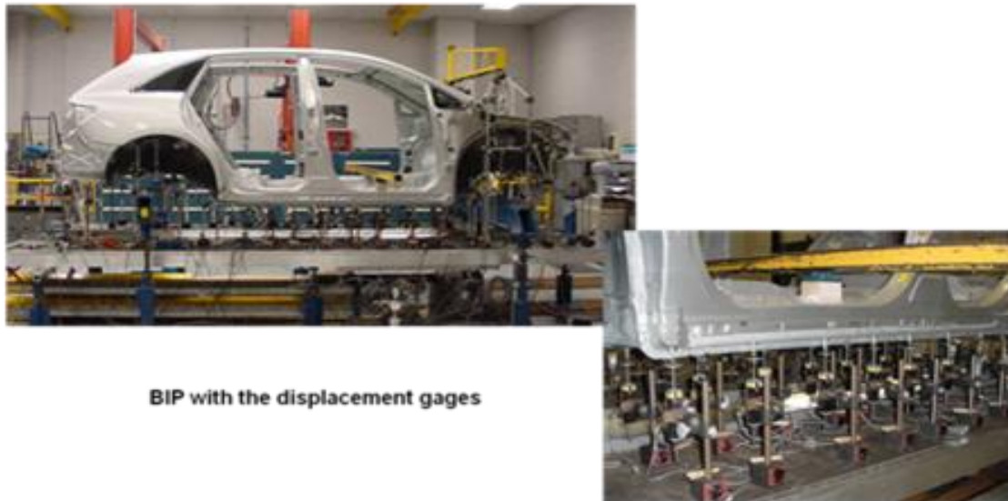
Image D.3-1: Bending Stiffness Testing Setup
