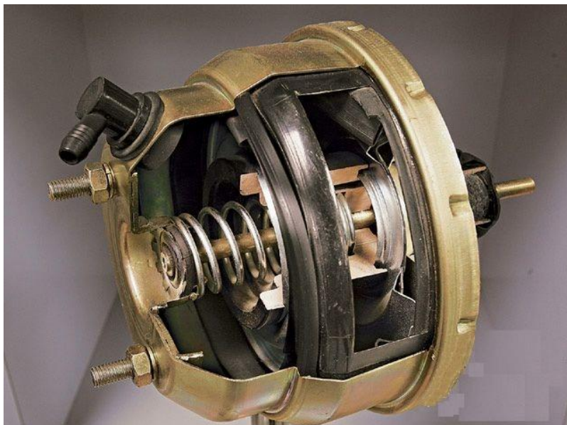
Image F.11-80: Brake Power Brake Subsystem Major Sub-assembly Example
