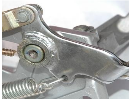
Image F.11-77: Brake Pedal Arm Frame Reduced Mass Sub-assembly Example
