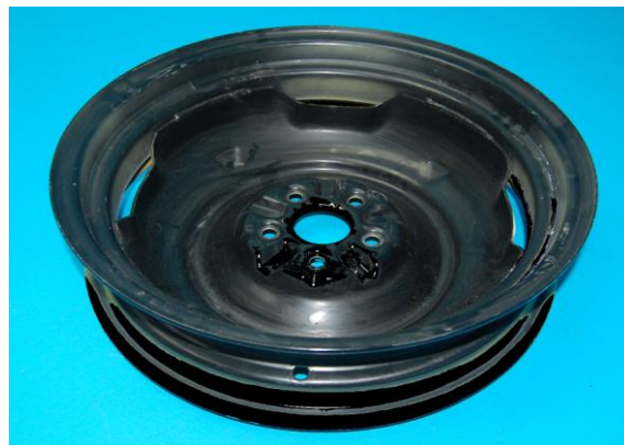
Image F.9-94: Spare Wheel Mass Reduced Assembly
