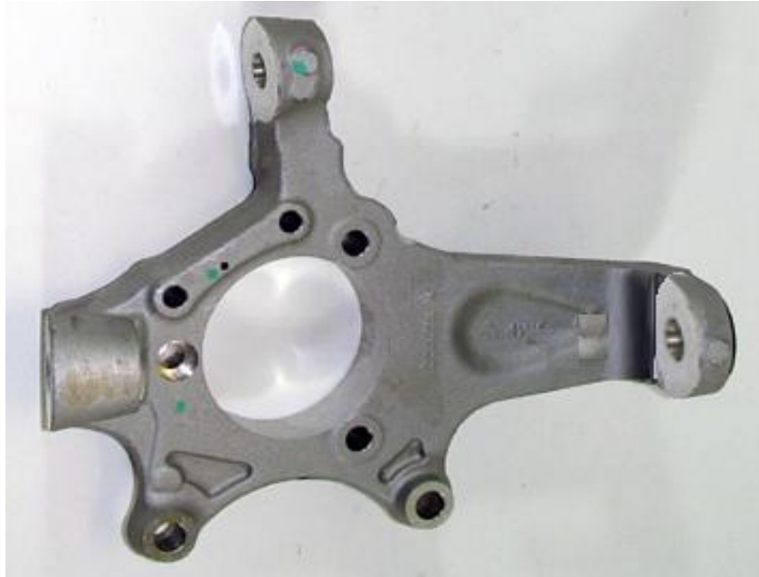
Image F.9-48: Rear Bearing Carrier Knuckle Mass Reduced Component Example
