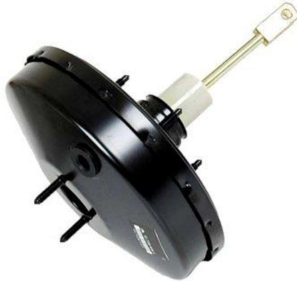
Image F.11-88: Vacuum Booster Mass Reduced Sub-assembly Example
