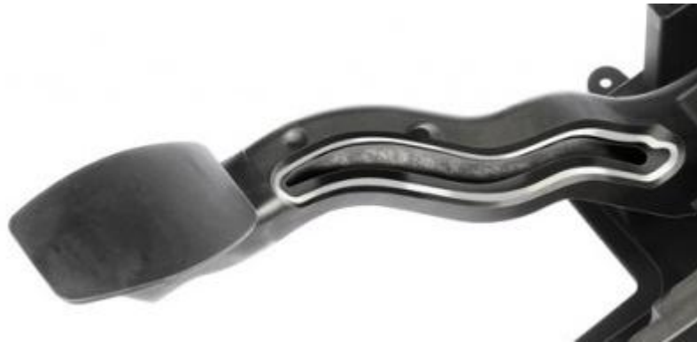
Image F.11-78: Brake Pedal Arm Mass Reduced Sub-assembly Example
