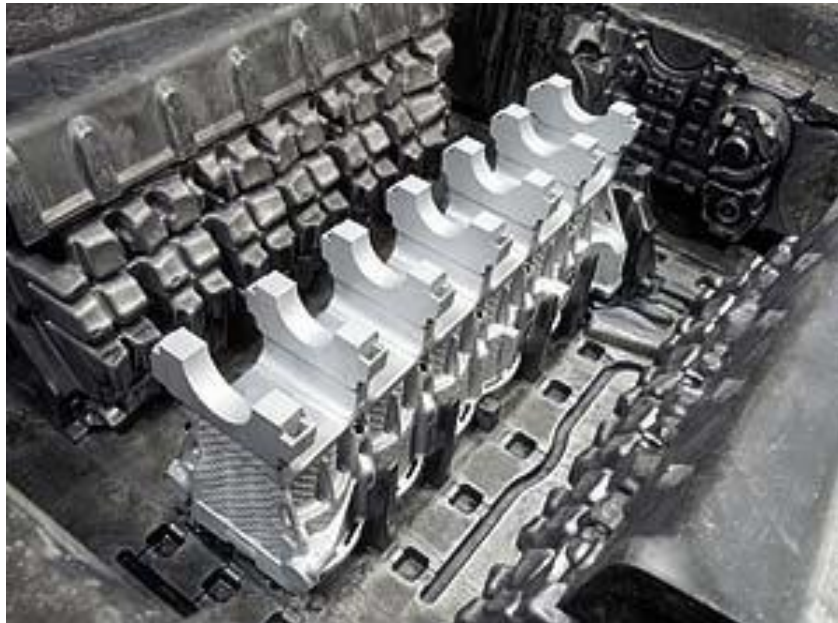
Image F.2-24: Die Casting - Aluminum Cylinder Insert
