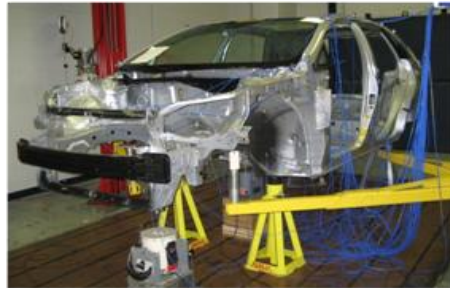
BIP instrumented with accelerometers
