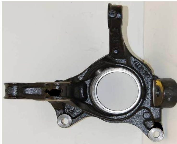
Image F.9-10: Front Steering Knuckle Current Component
