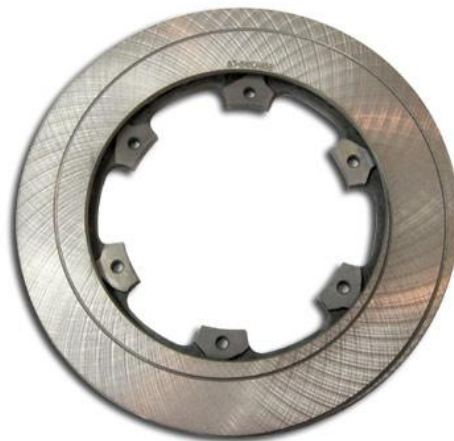
Image F.11-12: Front Rotor Mass Reduced Component
