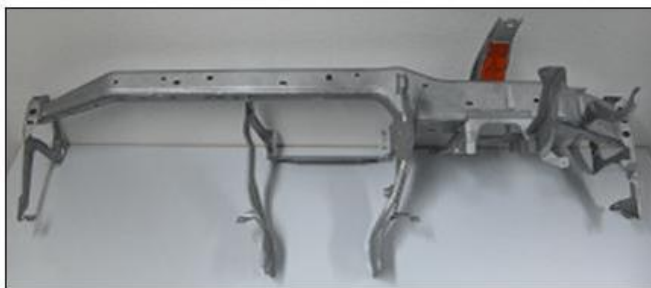
Image F.5-26: CCB Examples Compared by the Stolfig® Group
