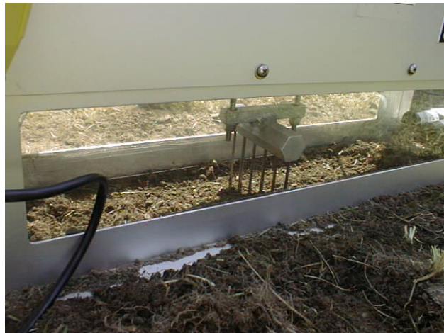
Figure 1. Releasable asbestos field sampler a) Instrument during sample collection b) Instrument rakes agitating the top soil (U.S. Patent Number 7,758,813)
