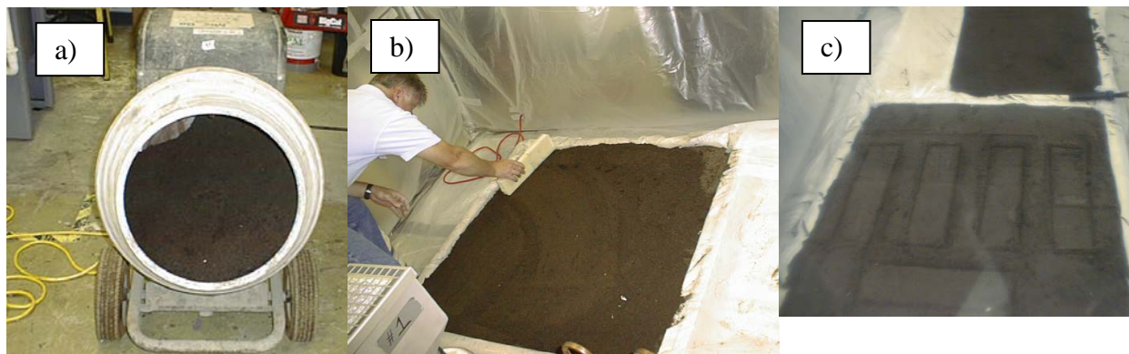
Figure 8. Soil and wooden frame preparation, a) Soil, sand and water being mixed, b) Wooden frame being packed and leveled, c) RAFTS footprint impressions
