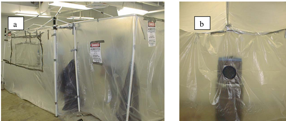
Figure 2. Tent for asbestos laboratory test showing, a) Working and decontamination area, and b) HEPA filter vacuum pump in wall of tent
