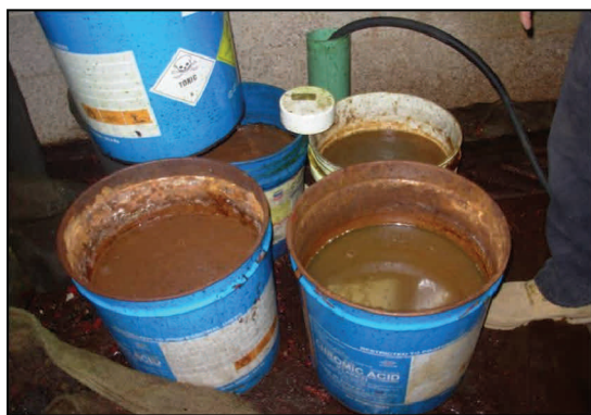
Accumulated wastewater at Smith Chrome Plating that was being discharged to the sewer from the hose shown above
