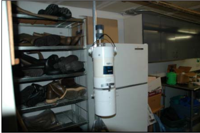
Figure 16 Mini-volumetric Sampler in Equipment Room
