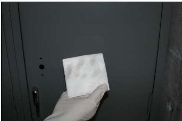
Figure 6 Equipment Room Locker Door Wipe Sample (0.3 µg PCBs)
