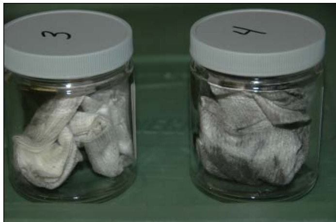
Figure 9 Vent Cover Wipe Samples (#3-inside room, #4-outside room)
