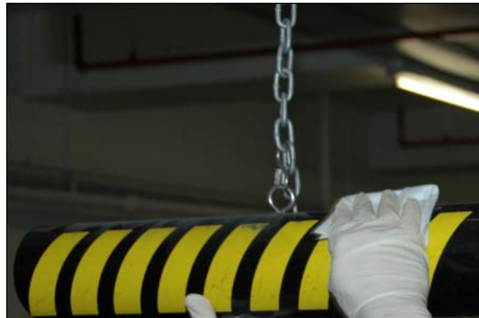
Figure 14 Sampling of Height Limit Bar (some dust visible)
